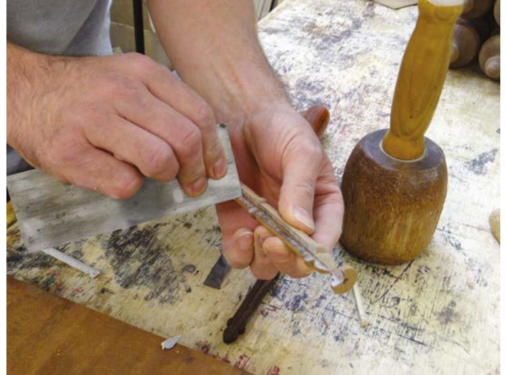
Using a cabinet scraper to remove the newspaper backing
