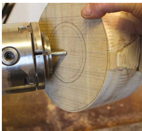
Mounting timber on a screw chuck
