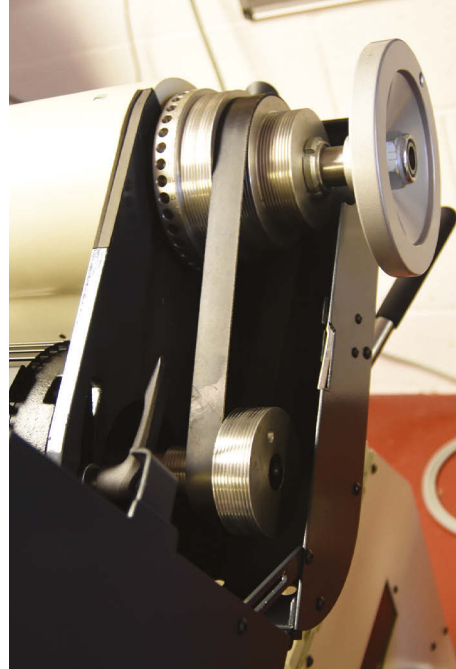
The pulleys and indexing ring in the housing
