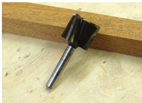
The tenon cutter I use to cut clean rebates
