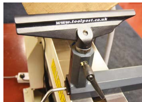
Toolrest with height adjustment collar to set at your preferred position
