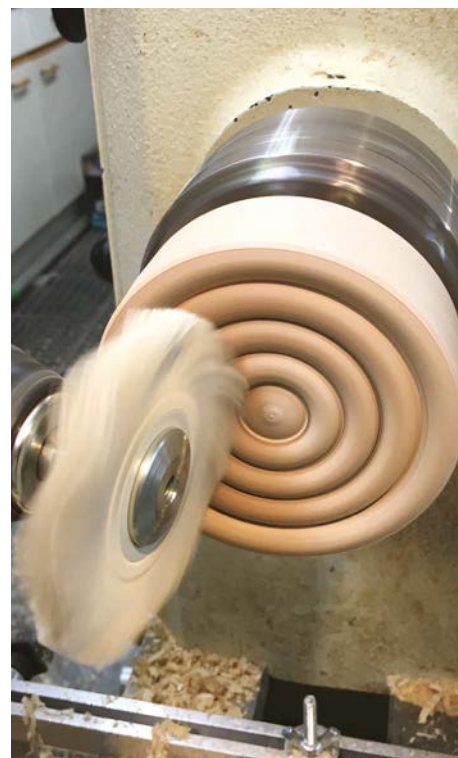
Cleaning up the surface of chatter work
