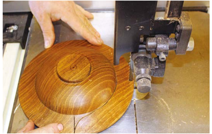
Cutting the waste away on the bandsaw
