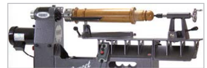
Gap section extends bed for long spindles
