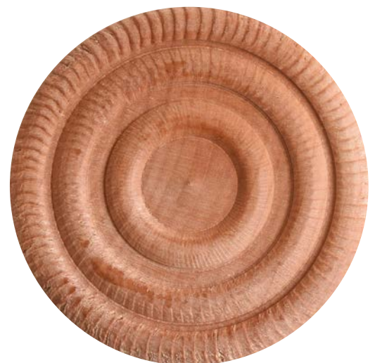
Example of damage due to not pre-shaping the beads and using too much pressure and too long a cutter projection
