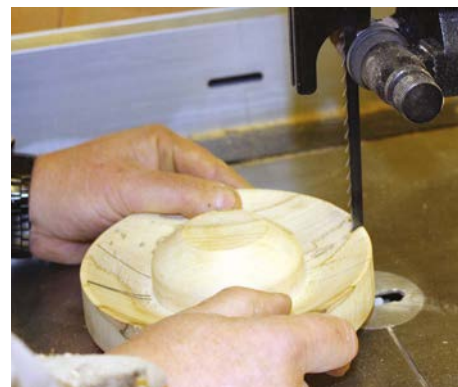
Removing waste on the bandsaw
