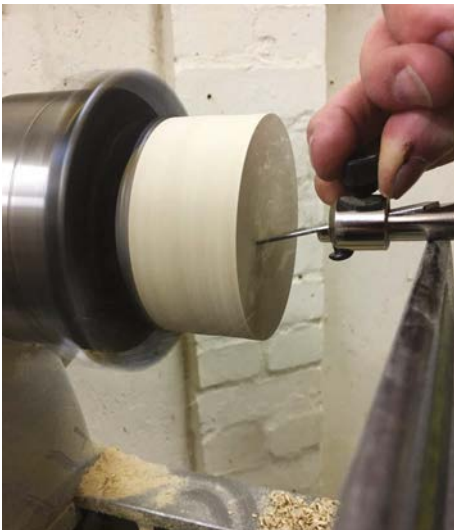
The square-end cutter being used square on to the work, but at a negative rake/trailing angle
