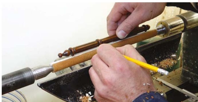
Transferring details from the original spindle
