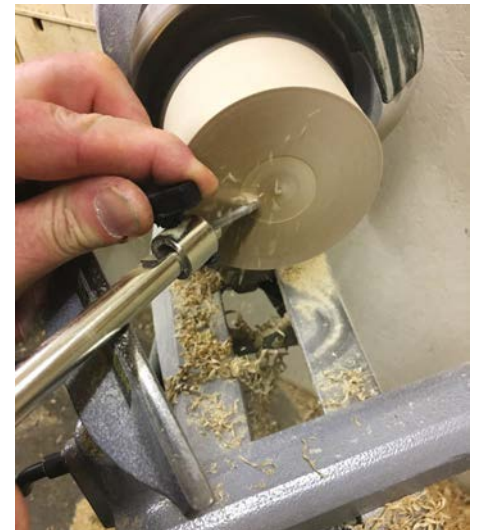
The diamond-shaped cutter is being used but note how the handle is rotated so the cutting edge is pointing at about 40° to the work
