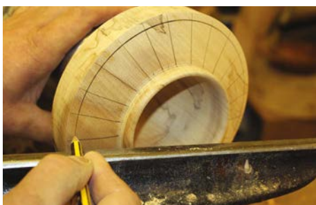
Using the indexing facility to mark equal segments on rim
