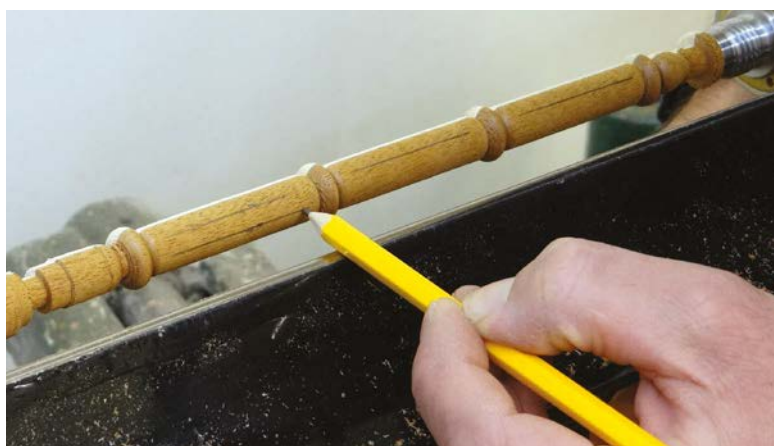
Marking the flutes using the toolrest as a guide
