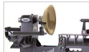
Gap section moved to side for large bowls and platters
