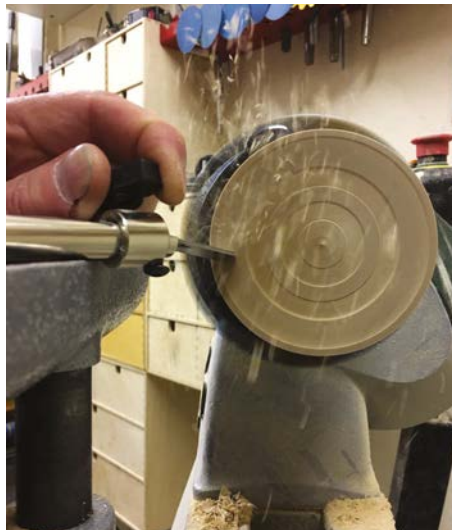
The diamond-shaped cutter being traversed along the work, but cutting below centreline
