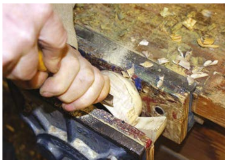
Cleaning up the waste cuts with a carving chisel
