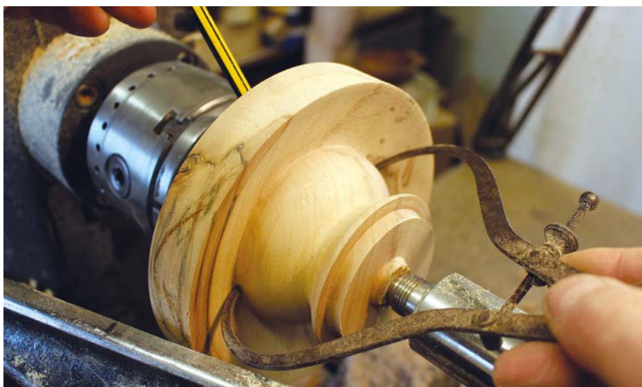
Checking dimensions above and below the wing
