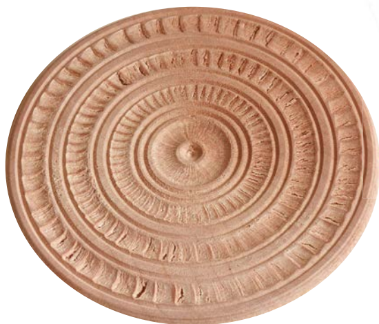
The result of too much blade projection in conjunction with too much pressure applied during the cut
