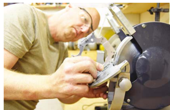
The gauges being used to set the platform prior to sharpening
