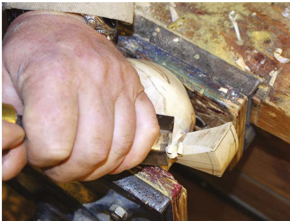
Cutting the arris with a bench chisel
