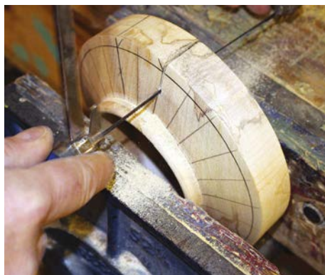
Removing waste with a coping saw
