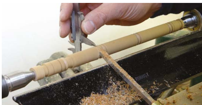
Sizing the spindle with Vernier callipers
