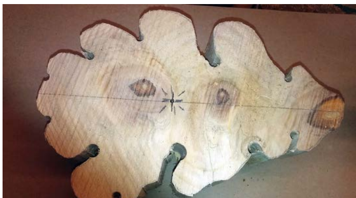
For oak leaves, draw a centreline along its length and halve this to find the centre. Then, offset the mark by about 20mm to offset the imbalance in the shape
