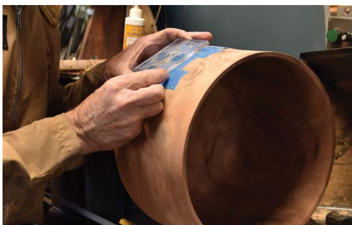
Careful alignment is required
