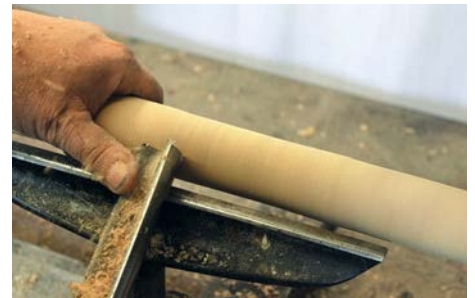
An overhand grip is used to help reduce bounce in the workpiece
