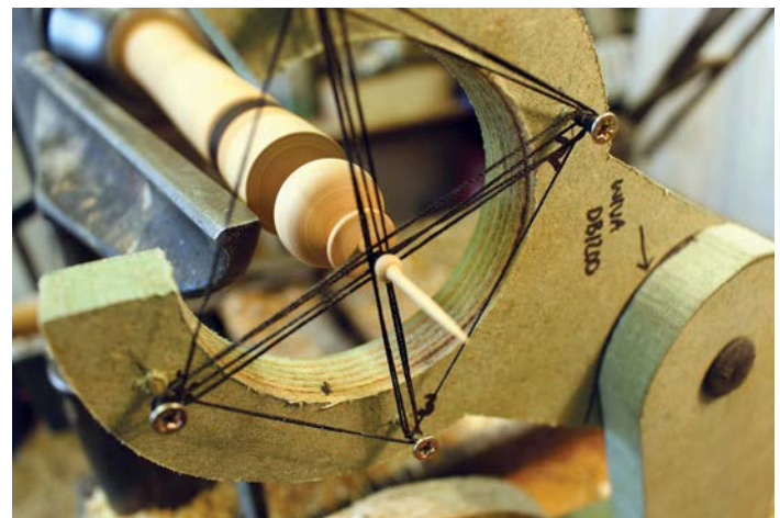
String steady tied off
