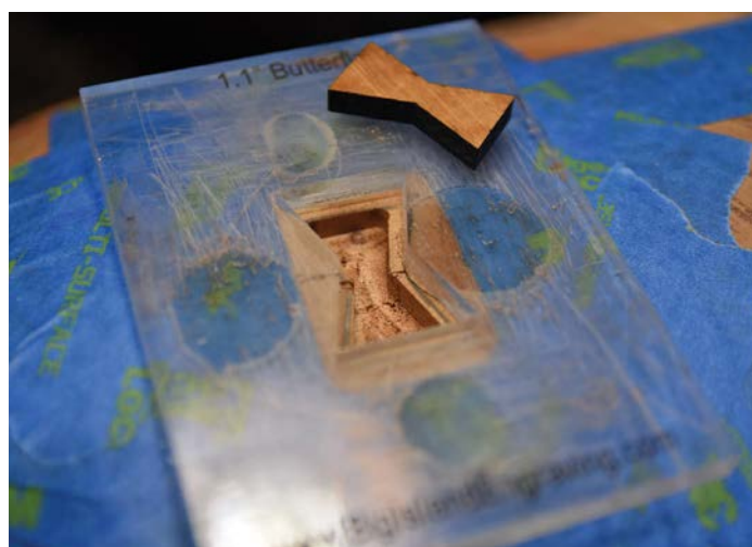
Here is the fill depth recess and the corresponding pewa to be inset
