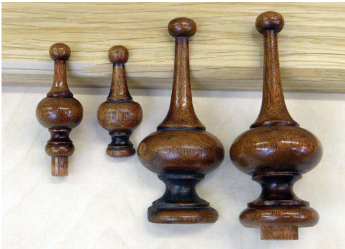
After the lacquer is dry they just need cutting back and a final polish
