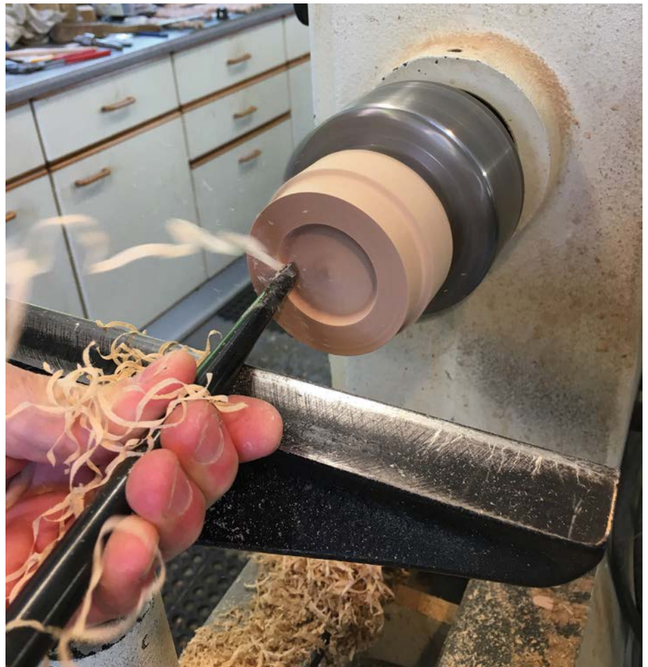
The straight probe removing waste on the inside of a box
