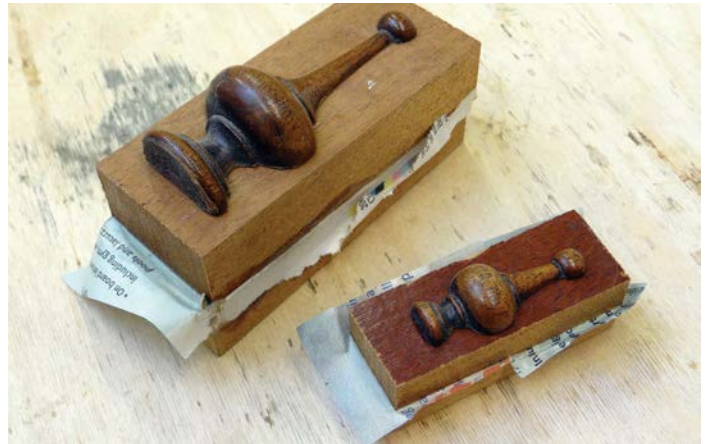
The finials on the blocks ready for turning
