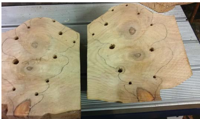
The oak leaf patterns with drill holes to make bandsawing easier
