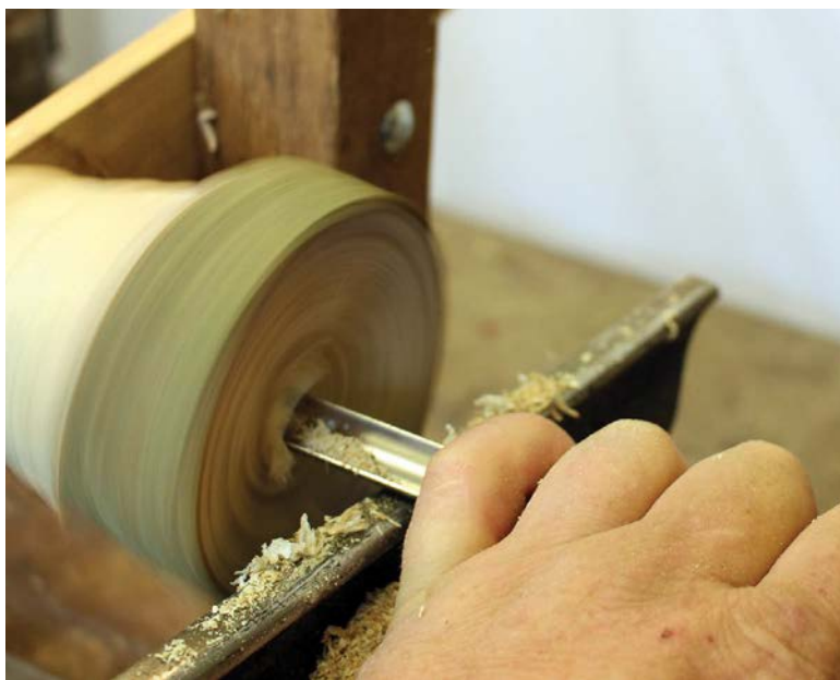
Using the simple steady to support the end of the workpiece
