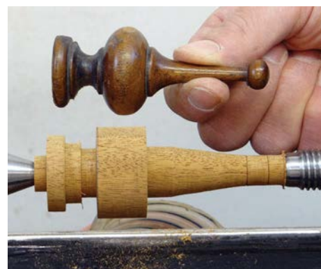
Blocked out and ready for the details to be turned
