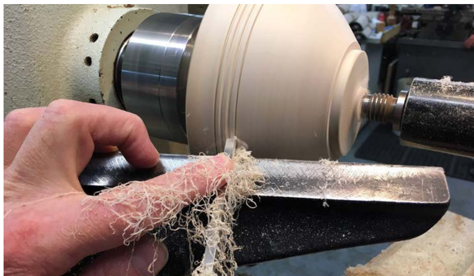
The bead-forming tool being used, showing the starting position with the handle lower than the tip and the finish position with the handle just off horizontal
