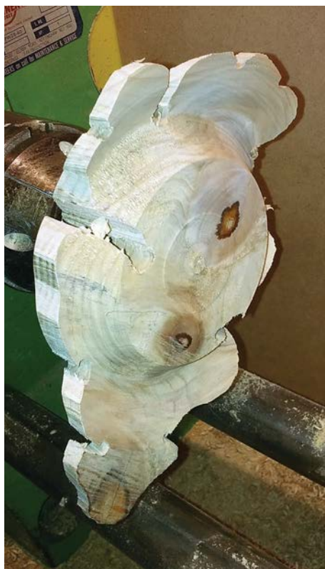
Turning the irregular edge areas before dealing with the centre section
