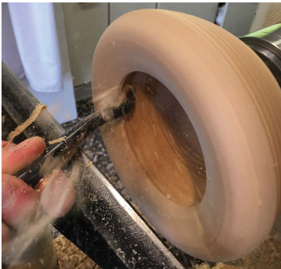
The offset Probe working on the undercut rim of a bowl
