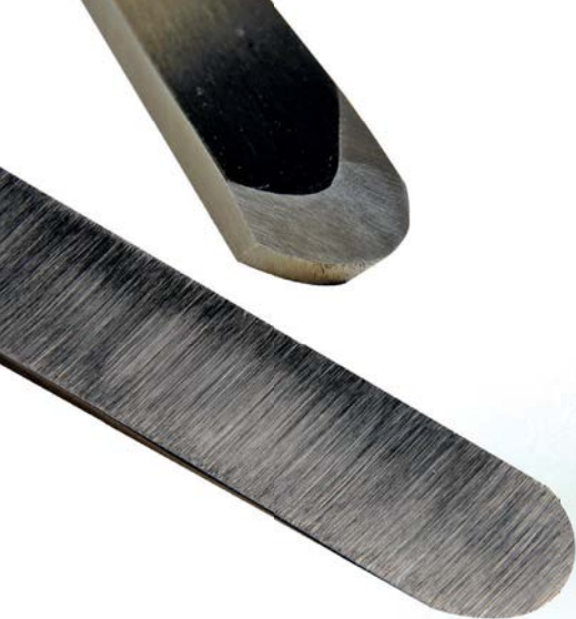
A negative rake scraper (top) shaped to cut a cove and a standard scraper profiled to cut a cove
