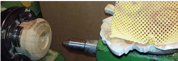
Jam chuck mounted in the lathe and the inner face of the bowl with non-marring non-slip router mat on it ready for placing against the jam chuck
