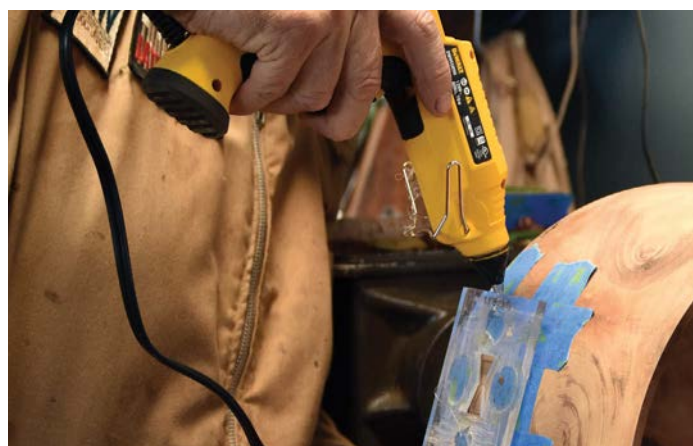
Bridging the gaps with hot-melt glue to provide stability
