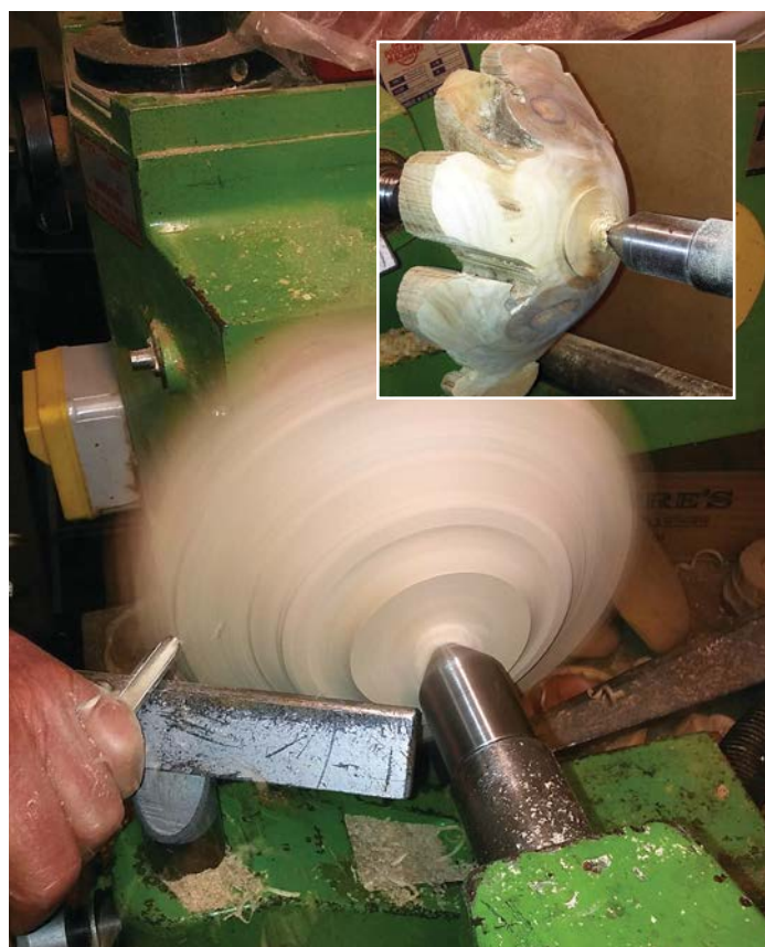
The blank mounted between centres and the irregular bandsawn edge area is turned against the grain to minimise breakage and tearout of the irregular edges
