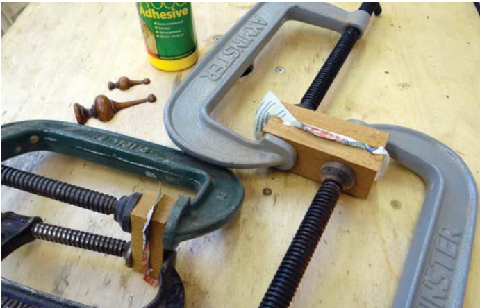
The blanks are clamped up overnight to dry
