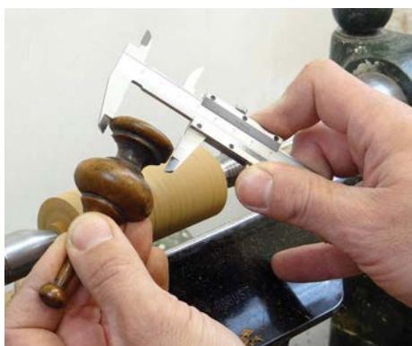
I take my measurements directly from the original
