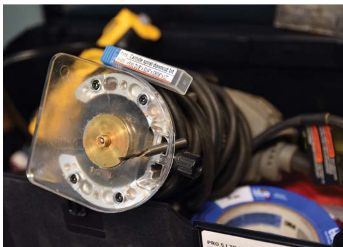
The picture shows the router with guide bush and bit attached and a spare router bit to show what is being used to cut the wood
