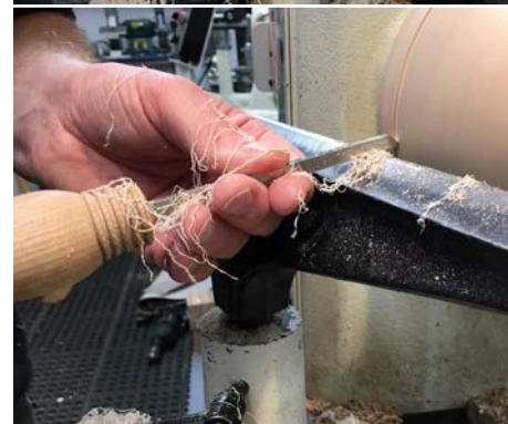
The bead-forming tool being used, showing the starting position with the handle lower than the tip and the finish position with the handle just off horizontal
