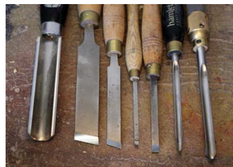
From left to right: Spindle roughing gouge, three sizes of skew chisel, bedan, pointed-grind 10mm spindle gouge, 15mm spindle gouge
