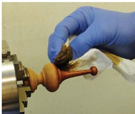
Applying the first coat of stain
