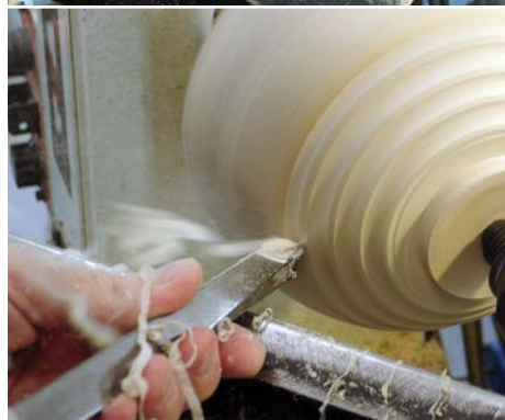
Using a forming tool to cut the coves
