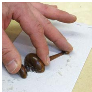
Rubbing against a flat piece of abrasive to remove the paper backing
