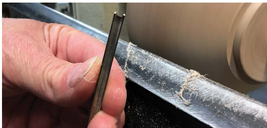
The points of the forming tool flattened/reduced in length just a little BELOW: Cutting multiple beads
