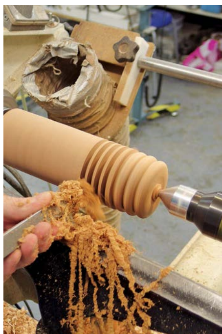
Pictures showing the various cones supporting work. But likewise the ring on the revolving can be used on its own to support work too
