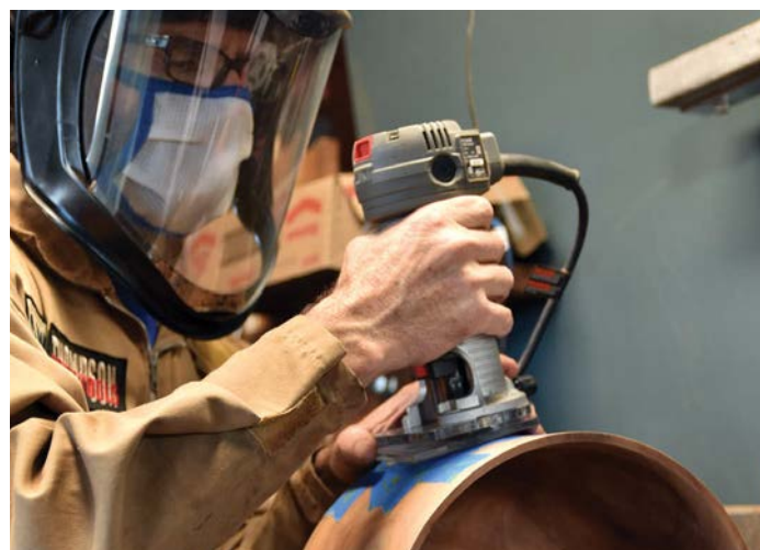
Wearing appropriate PPE and RPE and keeping the router firmly against the template, make gentle cuts, incrementally deeper until the required depth is achieved
