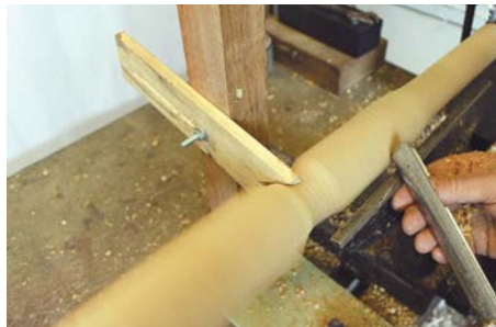
Simple steady used to reduce flex during roughing down
