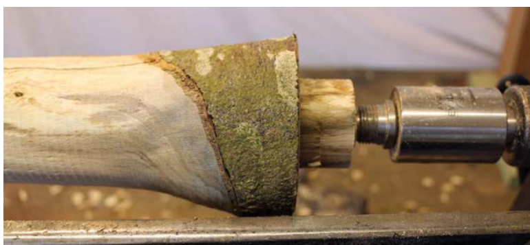
Preparing the long tenon
