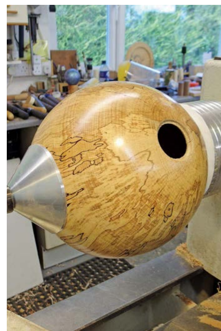
Pictures showing the various cones supporting work. But likewise the ring on the revolving can be used on its own to support work too
