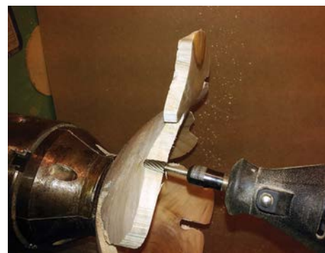
Using a rotary carving tool with a burr to refine the leaf-shaped edges
