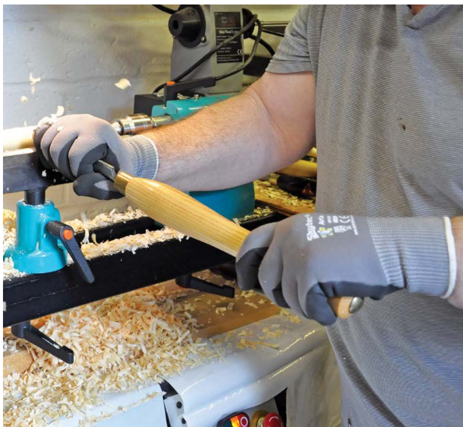
Gloves being used while roughing one of 100 presentation honey dippers for a local country club – green beech from its estate, rough turned to allow drying. I turn left and right-handed to vary posture and access, wear protective gloves, remove my watch and use extended jaws with no projections. Plastic sheet protects the lathe from the worst of the flying sap
