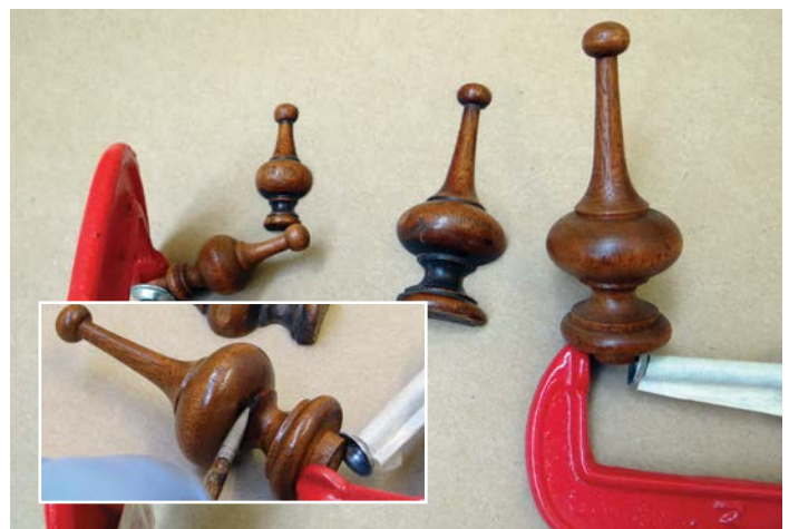
After the blush lacquer the colour is really getting close INSET: Adding the darker areas with a small brush and solvent-based stain
