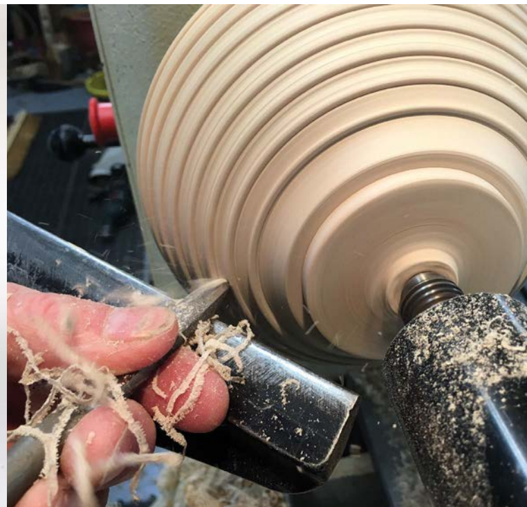
Using a cove-forming tool for cutting coves between beads
