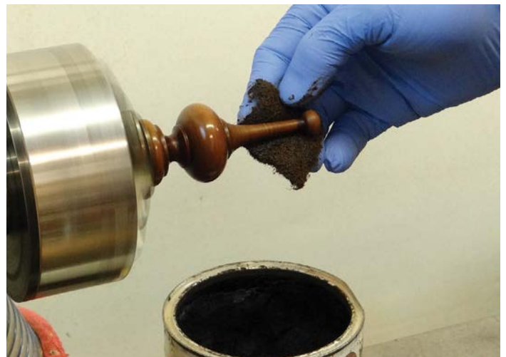
Gently applying coloured wax with an abrasive pad
