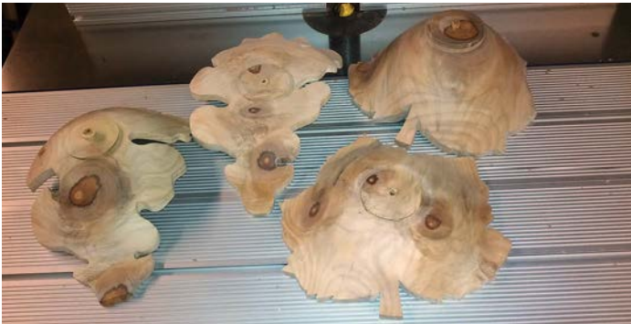
Here is a selection of leaf-shaped bowls ready for the bottom to be refined
