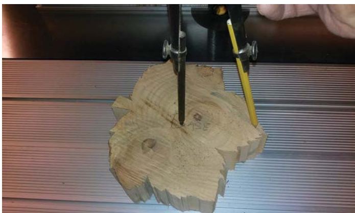
Finding the centre of the maple leaf using a compass
