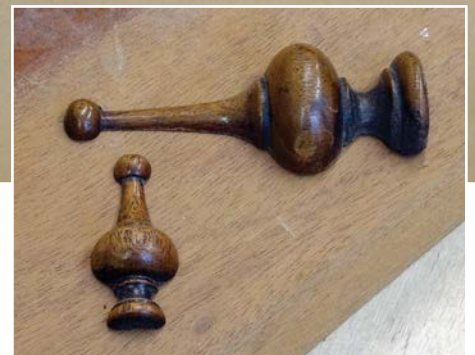
The original half finials with the reclaimed mahogany I used for the new finials
