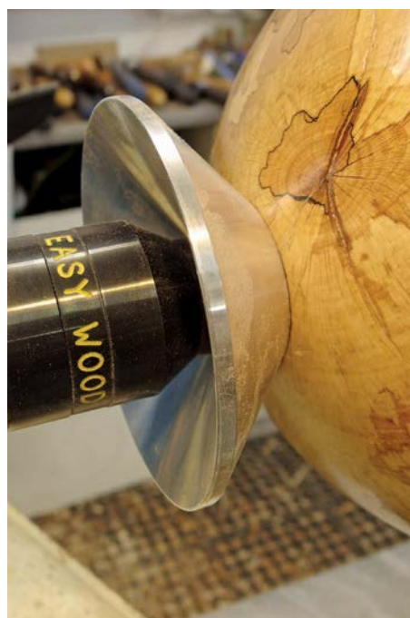
Pictures showing the various cones supporting work. But likewise the ring on the revolving can be used on its own to support work too
