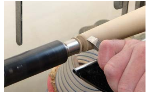
Rounding the bottom of the leg with my beading and parting tool
