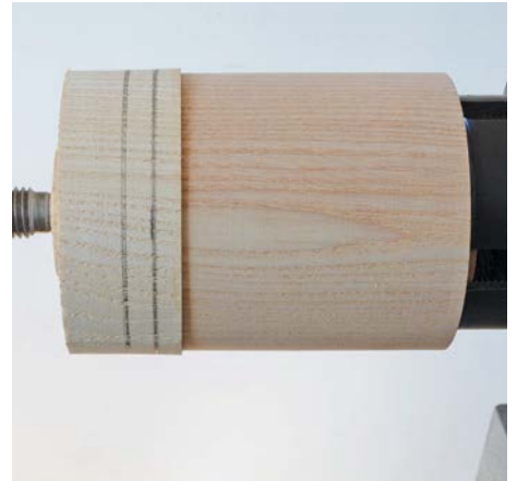
Lid jam-chucked on to the base with tailstock used for support while the top shape is created
