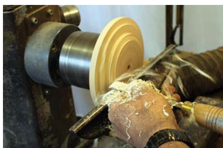
Preparing a jam chuck from scrap wood
