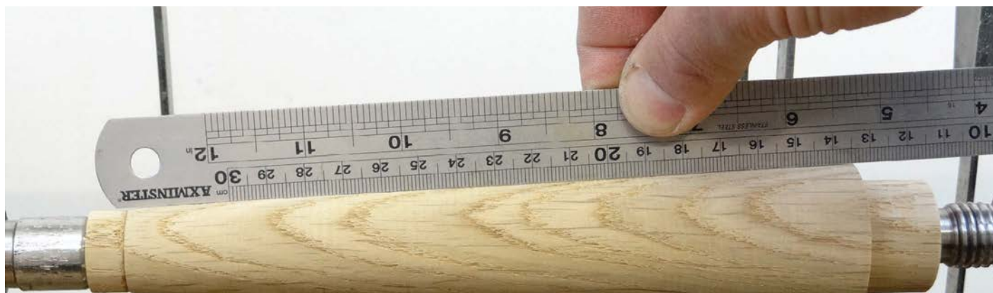
The straight edge is just as important on the small tapers as it is for the large legs
