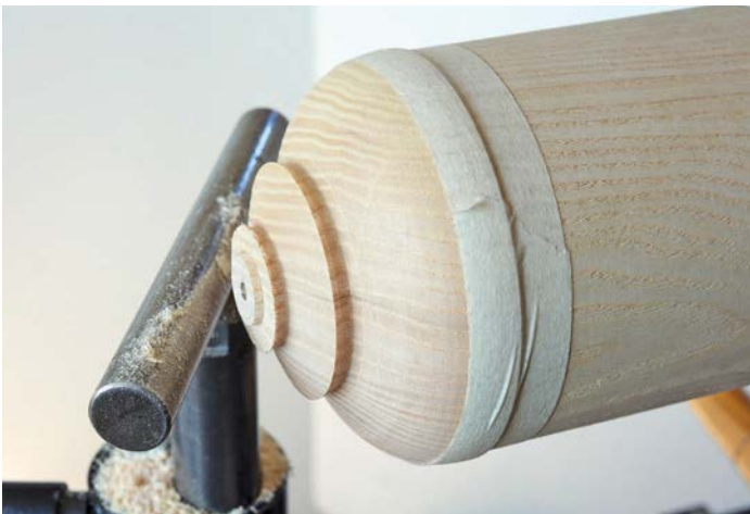
Using masking tape as insurance against base and lid parting company
