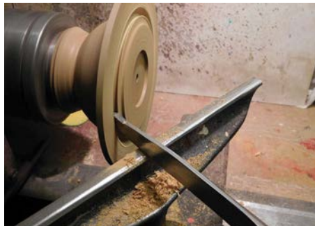
Using the slicer to core
