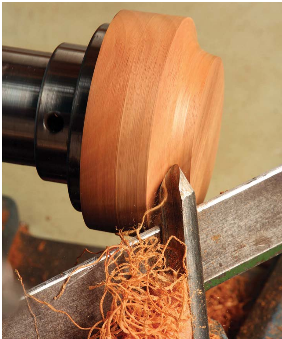
A concave moulding being turned with the detail gouge in the desirable steep presentation
