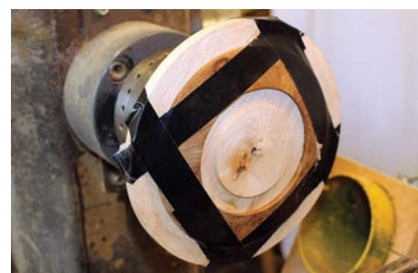
Extra security from duct tape
