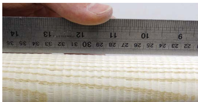
The straight edge shows a low spot
