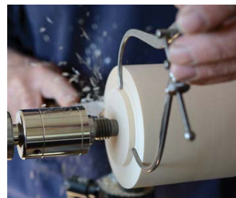
The base turned into a cylinder between centres, measuring while cutting the chuck spigot
