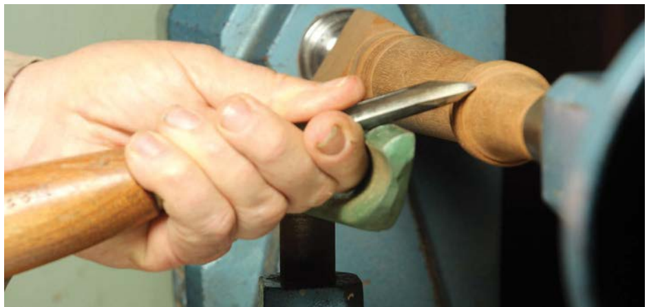
The underhand left-hand grip. The left hand is merely resting against the toolrest
