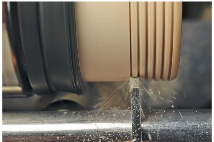
For uniformity, the beads on the non-domed lid are cut with a 3mm beading tool
