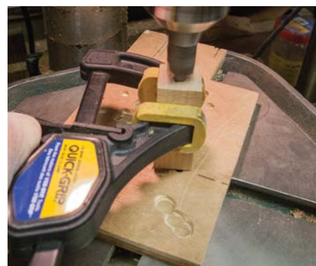
Using a slow speed and piloting on the tube's inner diameter, the pen mill will create a perpendicular face
