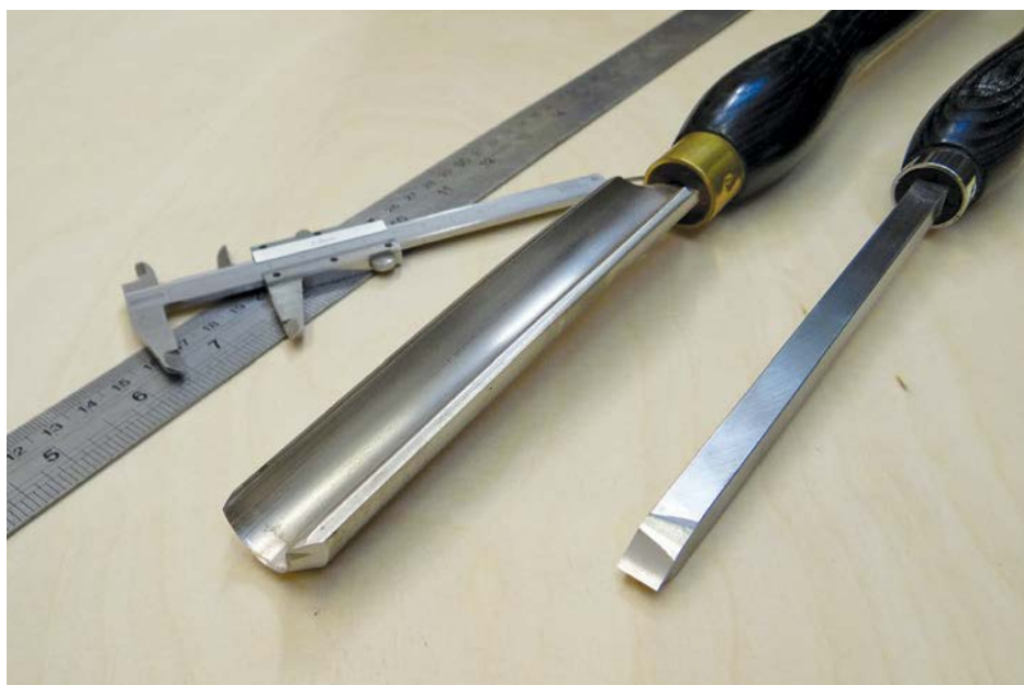
The tools for the job: spindle roughing gouge, beading and parting tool, Vernier callipers and a straight edge
