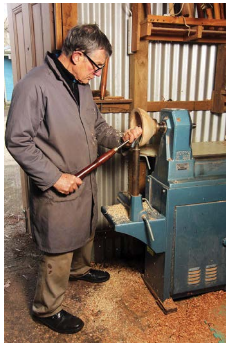
Turning outboard. I'm free to place my body where I wish, and can use a steep tool presentation if I like. Ideally there should be a duplicate (or triplicate) set of lathe controls located to suit outboard turning. Note: The lathe is turned off in this picture
