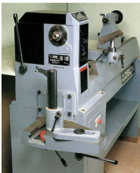
A nicely machined outboard turning facility
