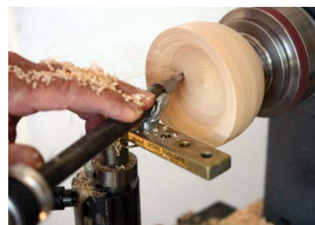
Using a hollowing gate as a stable pivot point
