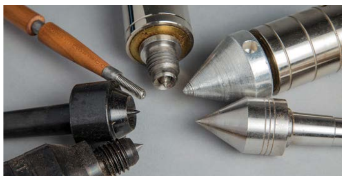
Tailstock centres have a variety of nose angles. This causes problems with the standard pen mandrel
