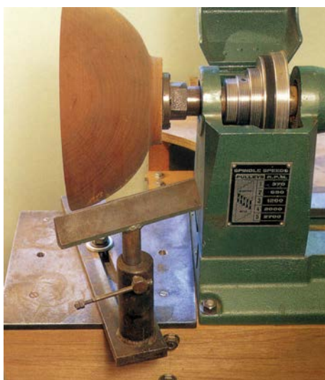
A cheap but excellent outboard facility for a bench lathe. The wooden bearers are continued past the left-hand end of the headstock, and a steel plate is mounted on them. You may need to obtain a banjo manufactured for a lathe with suitable high centre-height, or have a tall projecting from the right-hand side of the banjo neck banjo made
