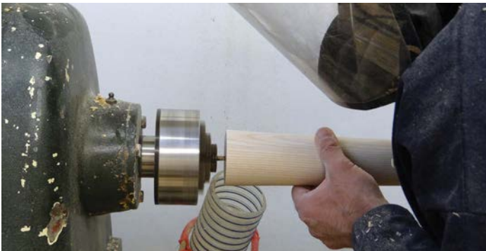
Drilling the pilot hole using tailstock support to ensure perfect concentricity
