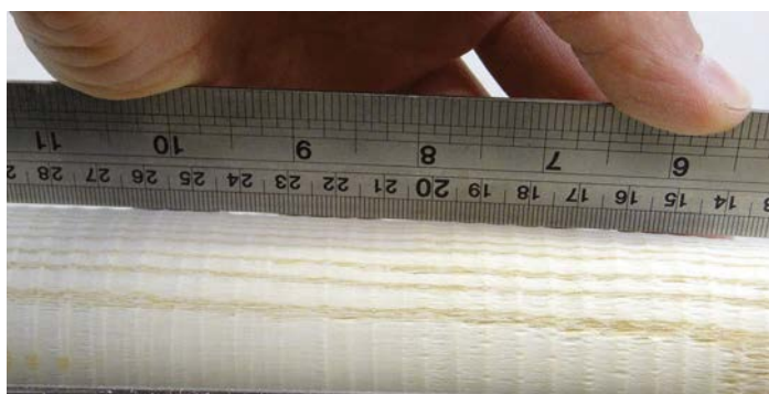
The straight edge shows a high point at 190mm
