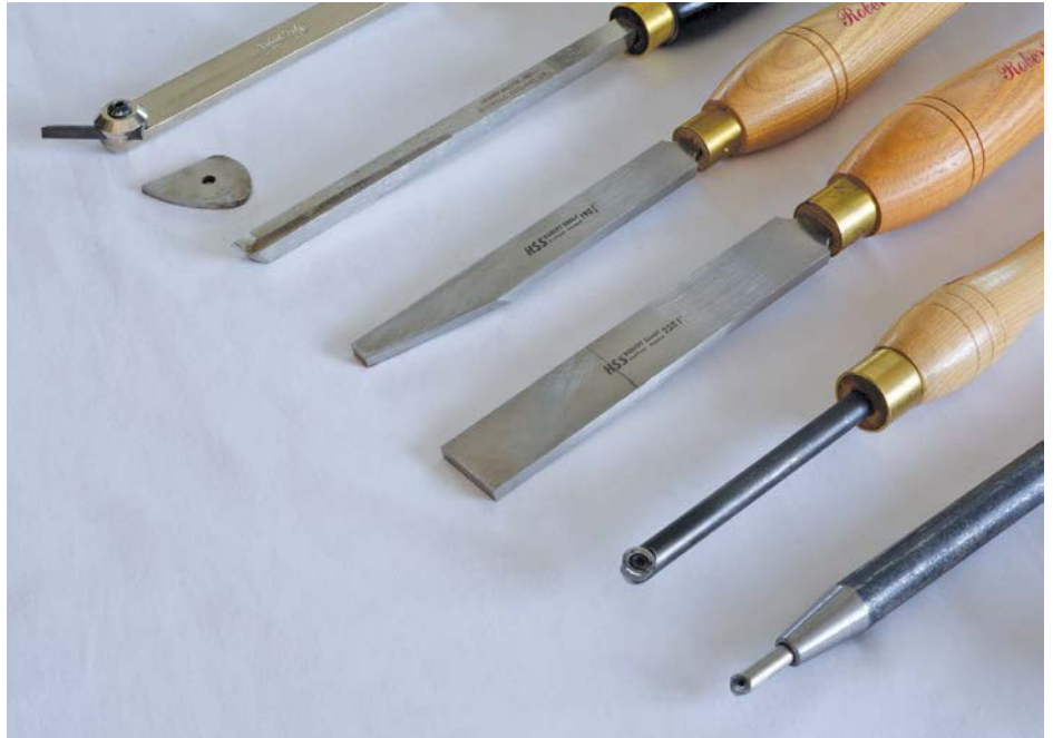
A selection of some of the typical hollowing tools for boxes. From bottom right to top left: two tungsten carbide tipped tools, 25mm square-end scraper, side-cut box scraper, a side and end cutting negative-rake scraper and a multi-purpose tipped hollowing tool with scraper head
