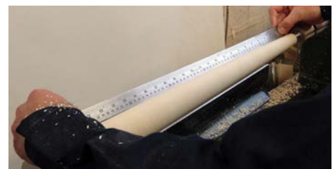
Using the straight edge with the lathe running
