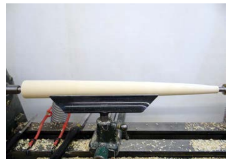
The roughed out taper, showing three clear facets
