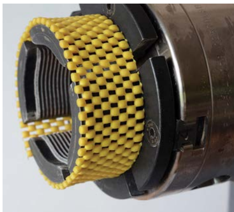
Chuck jaws with router matting to protect inside of base when re-chucking
