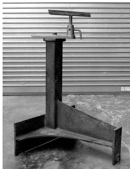
A fabricated outboard stand, banjo and toolrest
