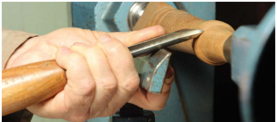
The tied-underhand left-hand grip. The left hand is actively gripping both the tool and the toolrest, and is therefore enabled to take a more active part in manipulating the turning tool. In particular, the left forefinger can move traverse the tool along the toolrest either to the left or the right. Also, because the left hand should be securely gripping the tool blade, the left hand can apply axial thrust and can rotate the tool
