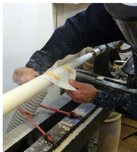
Sanding the large tapered legs with a strip of abrasive, keeping arms and clothing well away from the work
