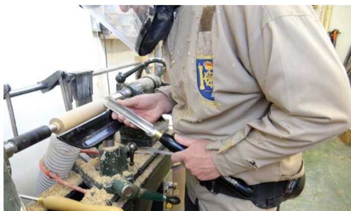
Beginning the cut with the tool handle low
