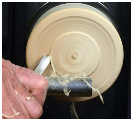
Final action on the base, dishing the bottom with a spindle gauge
