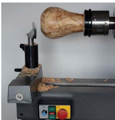
Lathe set-up for ideal hollowing position
