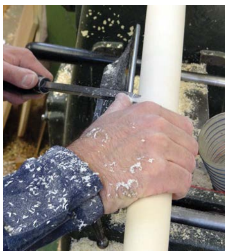
Planing the timber and offering support to the work with my front hand
