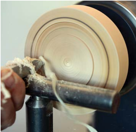
Creating a recess in the underside of a lid with a parting tool. Note the pencil line to define maximum width, leaving sufficient material to finish
