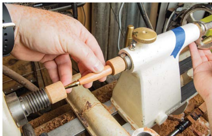
The best assembly tool is your lathe. A couple of wood blocks work well
