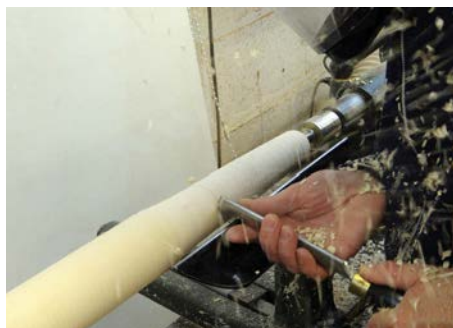
Beginning the initial shaping stage at the bottom of the leg
