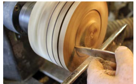
Edge cut made, face cut started
