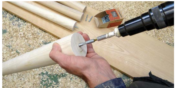
Fitting the stud screw into the ash legs
