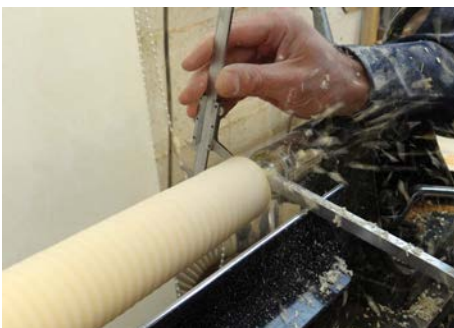
Sizing the bottom of the leg
