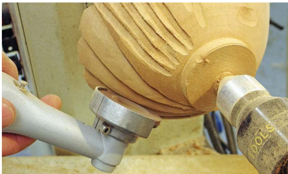
Using the sanding pads to clean up some cuts
