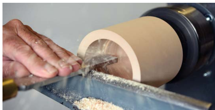
Plunge cutting with the square end scraper to establish wall thickness and clean up
