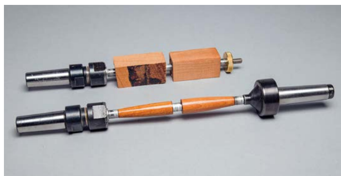
A mandrel saver swallows the shaft putting all of the force on the bushings and brass tubes
