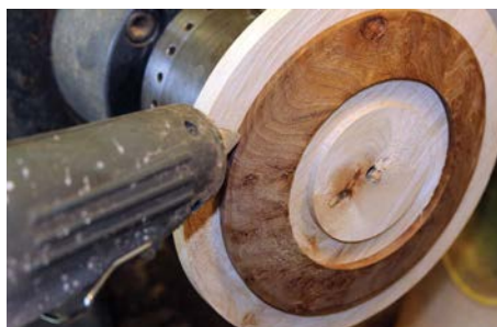
Extra security from hot-melt glue
