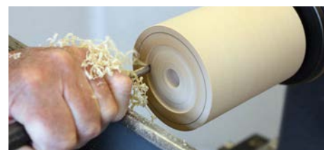
Initial hollowing cutting from the centre outwards
