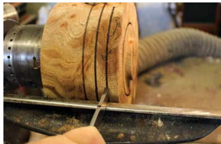
Blank marked off and tool position
