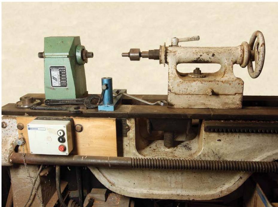
A bed with a gap, here with the infill in place. The bed and tailstock are from a 19th-century engineer's lathe. The woodturning lathe headstock has an outboard nose with a left-hand thread, and is mounted so that a banjo on the bed projecting to the left can be used for outboard turning. The inboard spindle nose has a hexagonal boss which can be locked with a spanner for chuck mounting or removal
