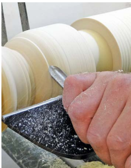
Turning the sphere detail with the spindle gouge
