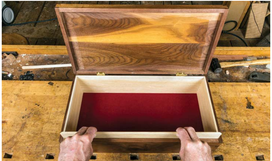
I do not glue the liners but fit them so well with a plane and a shooting board that they stay put. This makes repair of the box much easier. Here I am removing the newly fitted liners so I can drill the holes for the handle stems
