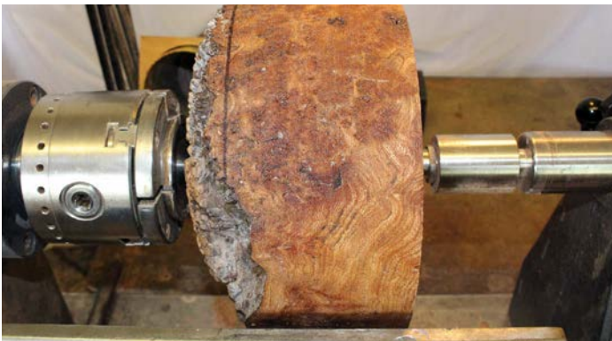
Blank mounted between centre perpendicular to lathe bed
