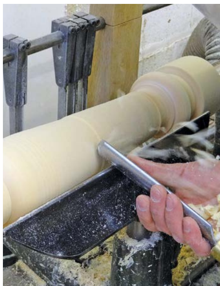
Defining the main shape with the roughing gouge
