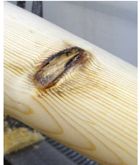
Knots and pine go hand in hand but, turned carefully, they shouldn't cause too much trouble. This knot shows the finish straight from the tool
