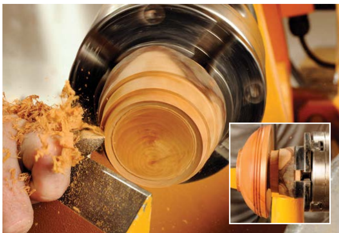
Cut a tenon on the waste wood so it is a snug fit for the size of hole in the work and check for fit with the lathe stopped
