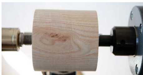
The blank turned into a cylinder shows the full extent of the defect and a decision needs to be made as to where the defect or feature will appear on the finished article
