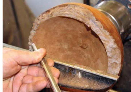
Making the entry cut into the natural edge
