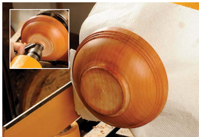
Place tissue paper over the tenon, fit the work on to the spigot cut and secure in place with a revolving centre in the tailstock, then shape the bottom
