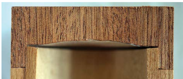
Basic over-fit lid with parallel spigot and recess, known as 'piston fit'
