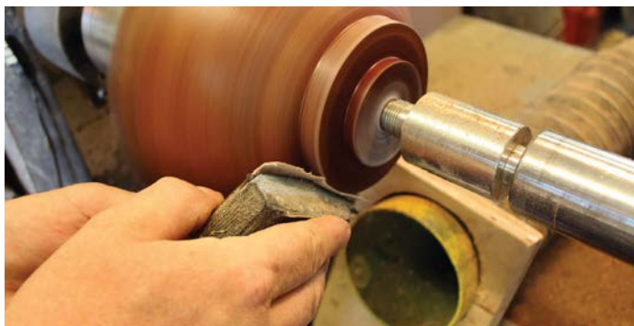
Abrading by hand using abrasive wrapped around a foam block
