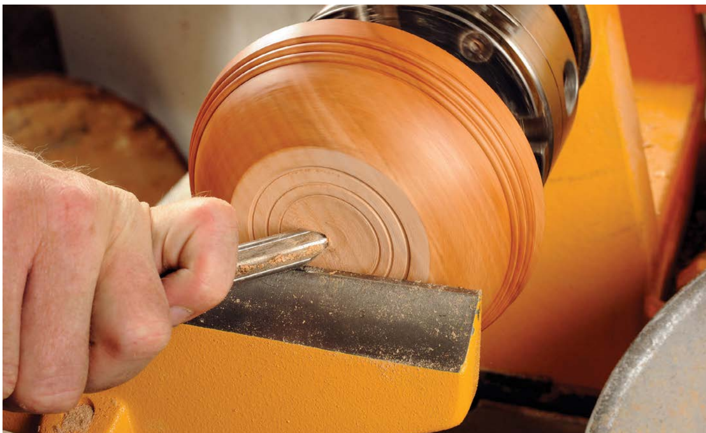
Once the underside is partially shaped, remove the tailstock and check the work is secure. If the hold is secure finish the bottom, if insecure, remove and hand finish
