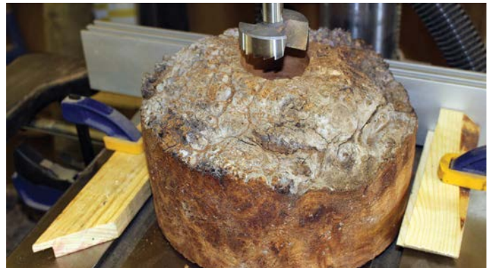
Cutting a mounting recess on the pillar drill
