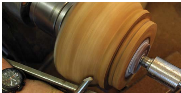
Sheer cut on lower wing of tool
