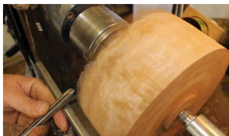
Cutting left to right to keep the natural edge intact
