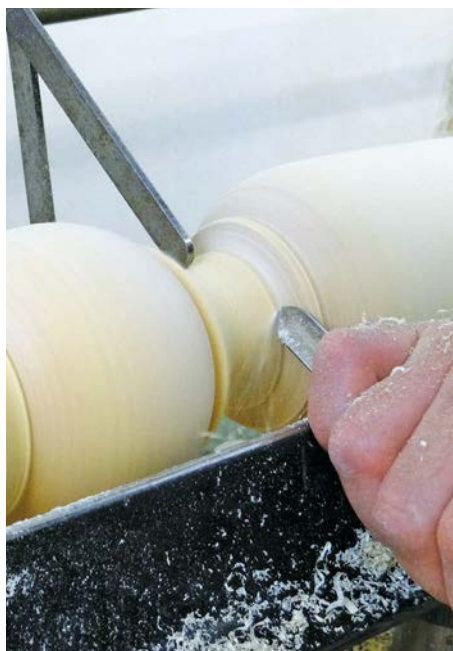
Forming the coves with the spindle gouge
