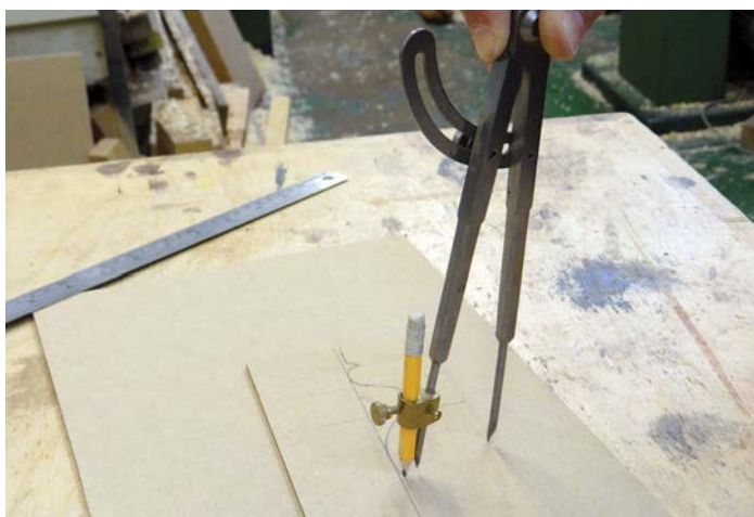
Using a pair of compasses to draw the spherical detail
