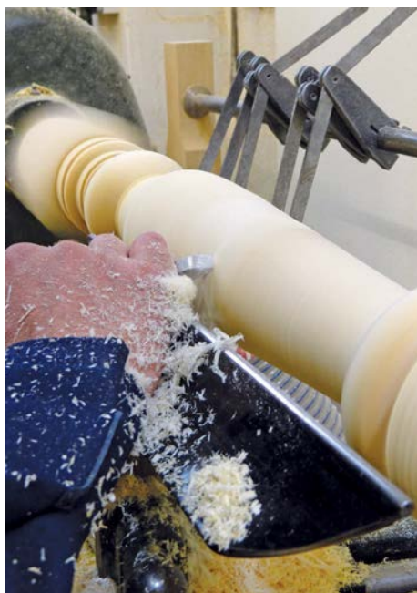
Planning cut with the beading and parting tool
