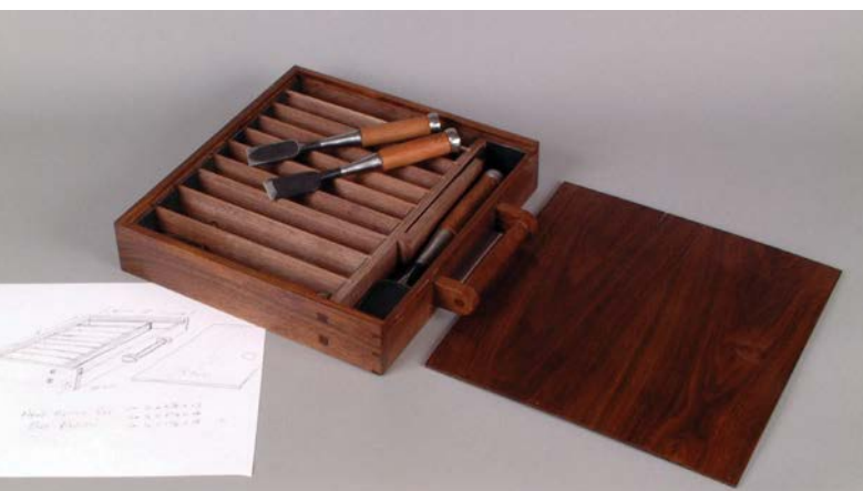
Custom box for author's Japanese chisels along with construction sketch
