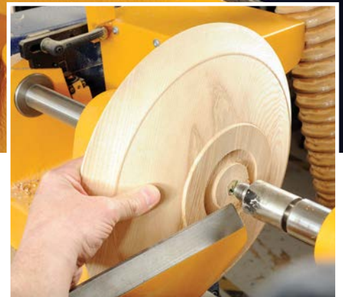
Bring up the tailstock revolving centre to support the work securely against the friction drive
