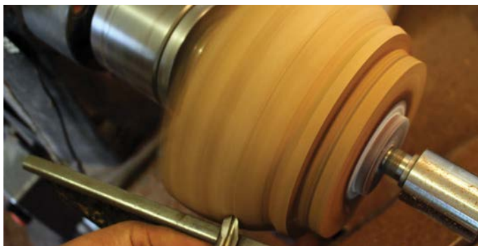
Bevel-supported push cut
