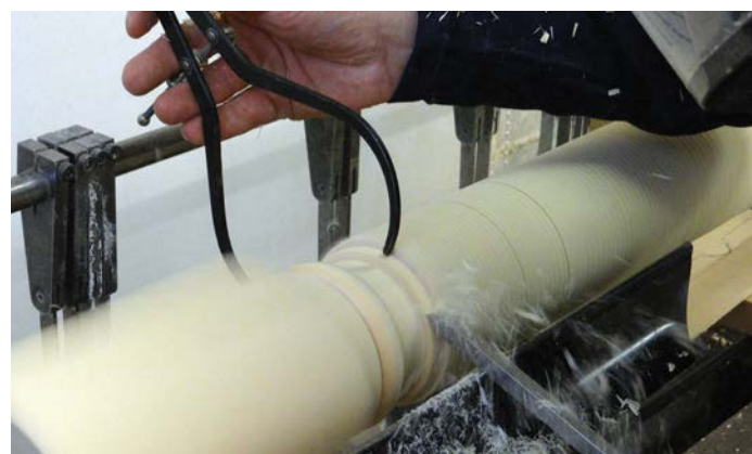
Sizing with spring callipers and my beading and parting tool
