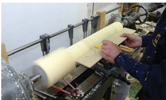
Using the template to mark the positions of the details
