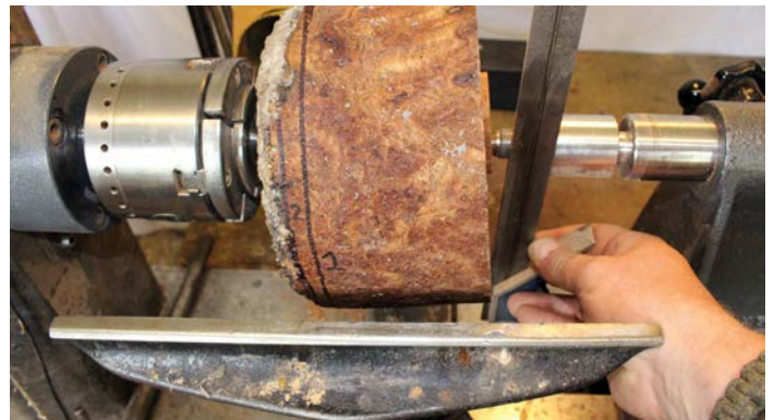
Blank mounted between centres at an offset
