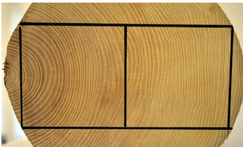
This was one quarter of an ash log highlighting what quarter-sawn timber looks like and marked out ready to saw two box blanks
