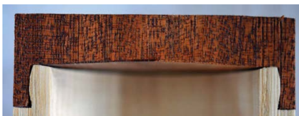
Over-fit lid made to pop off. Note the profile of the spigot which leaves a slim band of fibres around the middle which crush to ensure tight fit
