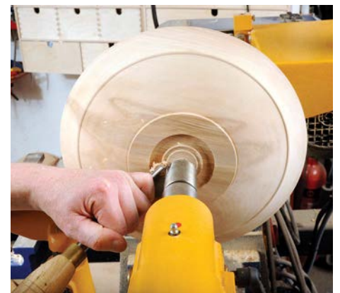
Turn away the waste and clean up the base leaving a small nub of wood under the revolving ring centre
