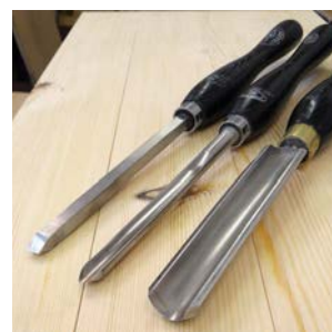
The tools used for this job: spindle roughing gouge, spindle gouge and a beading and parting tool
