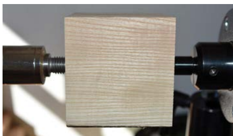
The outside piece of the log showing quarter-sawn straight grain. There was a very slight defect on the opposite side
