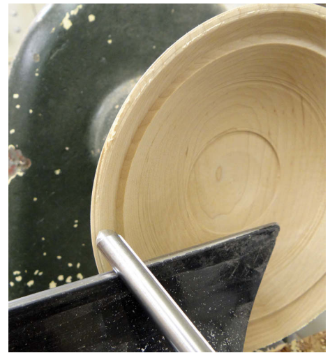
Catch with tool in place
