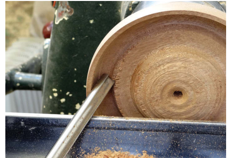
The wing of a traditional grind gouge is easy to catch
