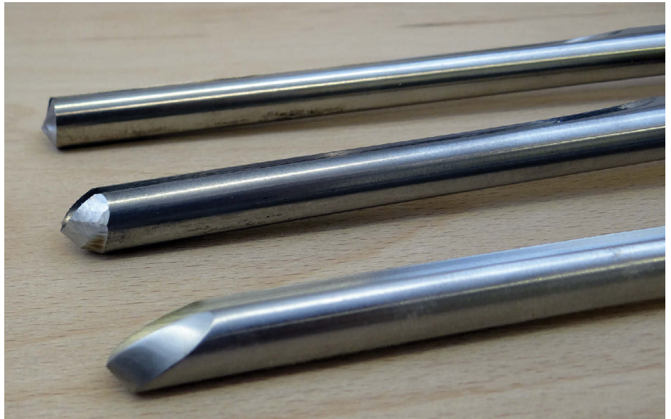
Three bowl gouge profiles: Top – traditional square grind, Bottom – long grind, Centre – my preferred long grind
