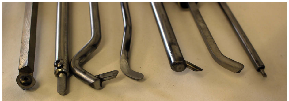
Simple straight, bent and cranked tools used for the initial hollowing out and if their shape allows some undercutting too
