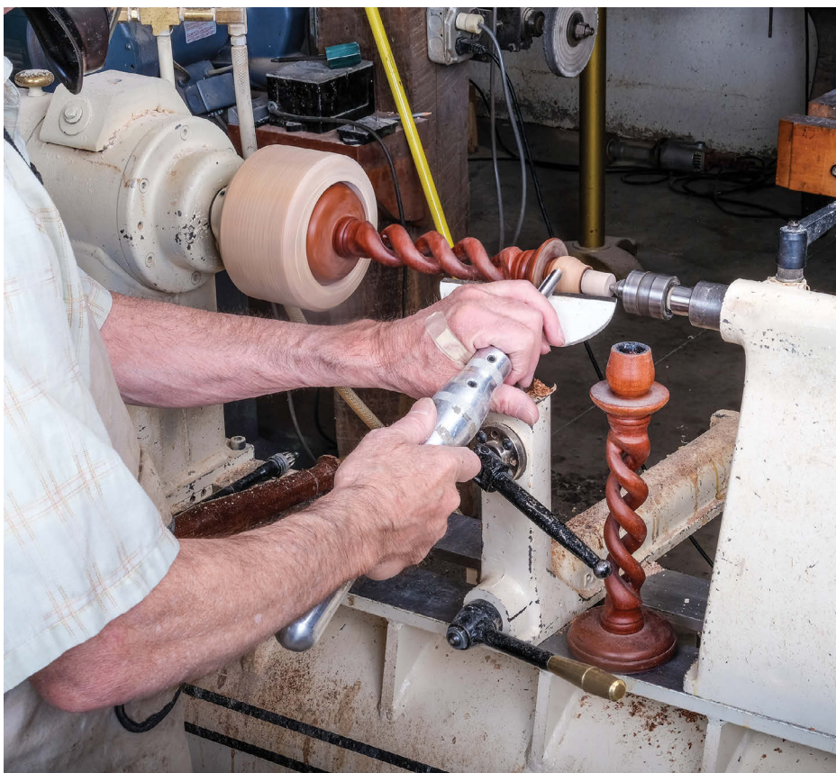
Repairing singed cups on barley twist candle made by author a decade ago. Although the cup was a separate piece it was quicker to catch the base in a jam chuck and centre the cup with a tapered mandrel. Metal inserts are now included
