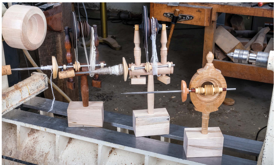
A reproduction bat head with two Miner, or accelerating, heads repaired by author, showing extremes of repair. The one at the left only needed a new spindle, pulley and whorl, while the only part saveable on the centre head is the countershaft. While spindle could be turned on a South Bend engineering lathe, it is quicker to chuck it in an electric drill and rotate it against the rotation of a bench grinding wheel
