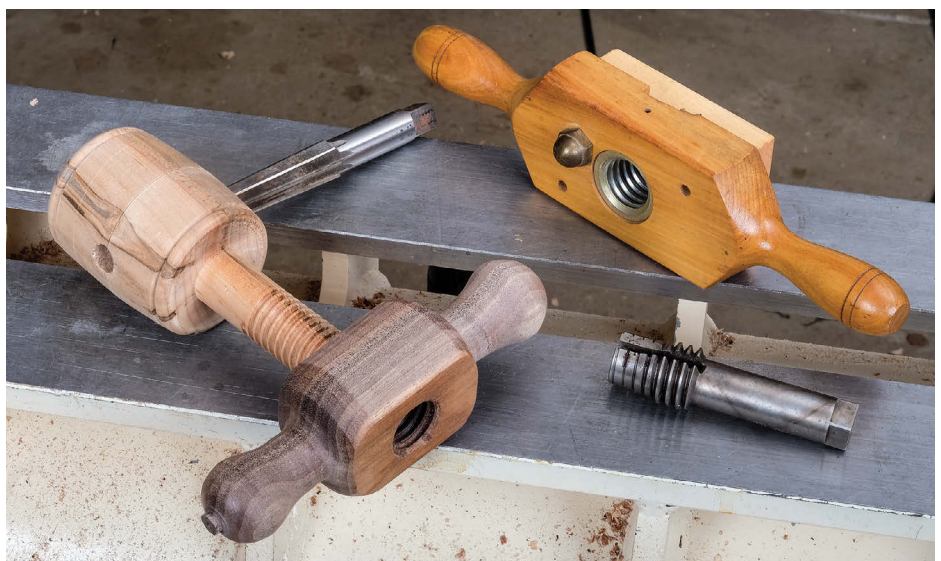
Threaded parts are common to spinning equipment in general. A 25mm threadbox was used to cut male threads on shaft while tap cut female threads in the wing nut. Standard No.2MT reamer was used to ream tapered hole from stepped 15mm-13mm hole
