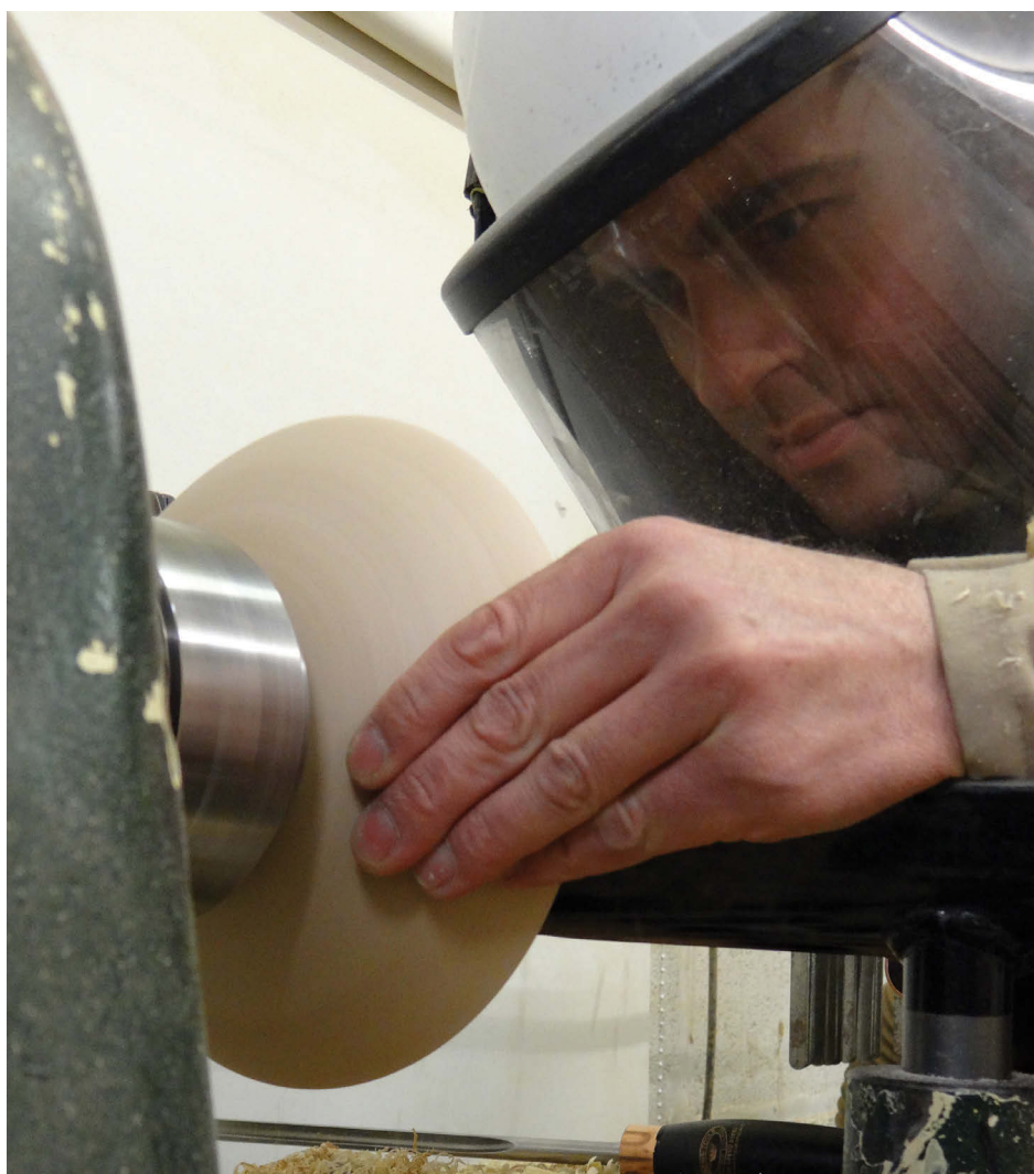
Concentrating on turning the inside of a bowl and supporting the bowl at the same time
