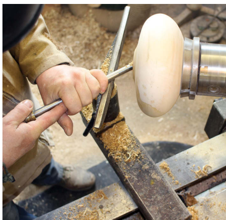
Headstock at 45° to bed for easier access
