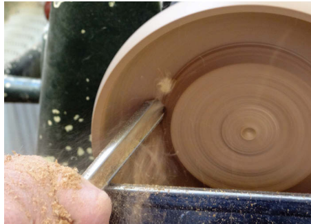
Cut is progressing well but the wing is getting close to a catch
