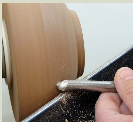
I was surprised how far I could rotate the tool before getting a catch
