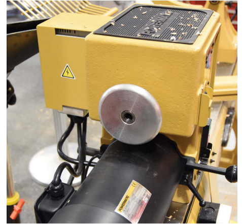
View of the end of the headstock. Note the threaded internal bore of the end of the spindle. This will accept vacuum-chuck attachments
