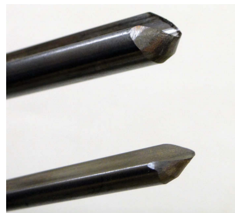
The difference in profile between a bowl gouge and a spindle gouge
