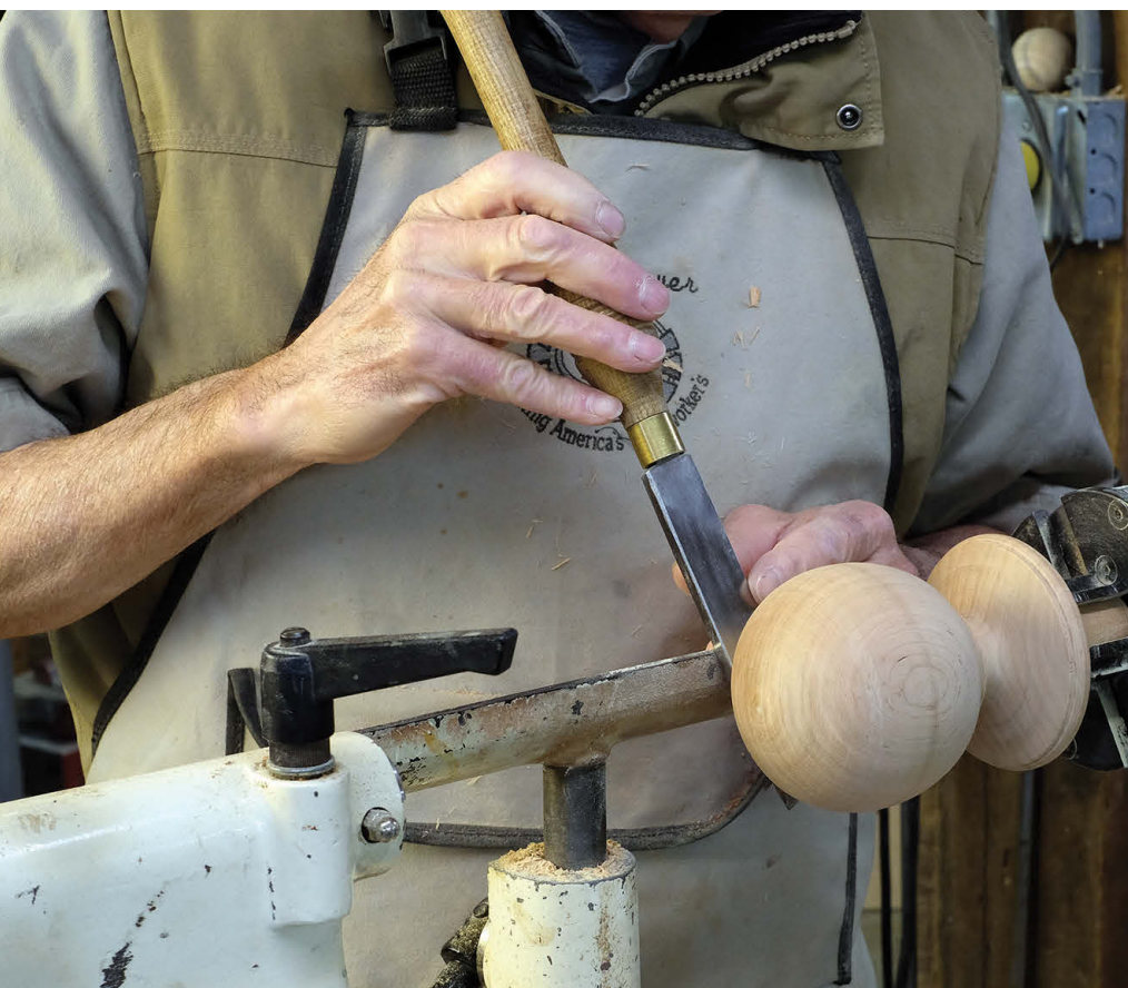
Making a duplicate of a stair newel post pediment. Turned almost entirely between centres the author used a four-jaw chuck to turn the centre mark at the very top away. By loosely grabbing it in the chuck and running the lathe slowly (50rpm) the piece was brought on perfect centre by applying pressure with the flat of a skew against it. The chuck was then fully tightened and the centre turned away
