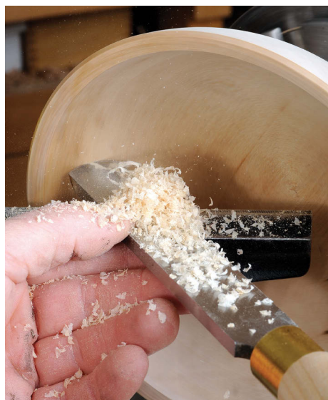
Using a scraper on the inside of a bowl
