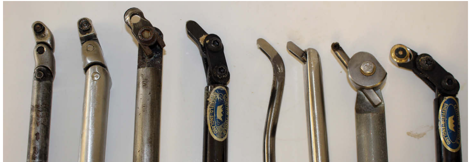
Shielded, cranked and multi-link tools can, depending on their design, be used for initial hollowing and for cutting under the shoulder of the hollow form
