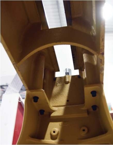
The webbing on the underside of the lathe bed
