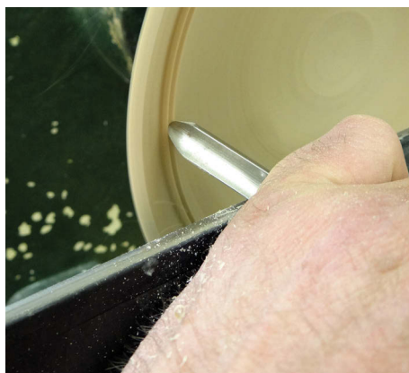
Using a spindle gouge to refine a detail rather than a bowl gouge
