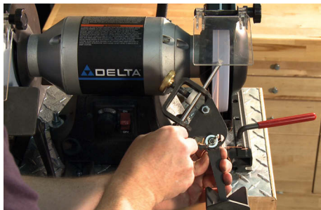
Using a jig to sharpen a gouge
