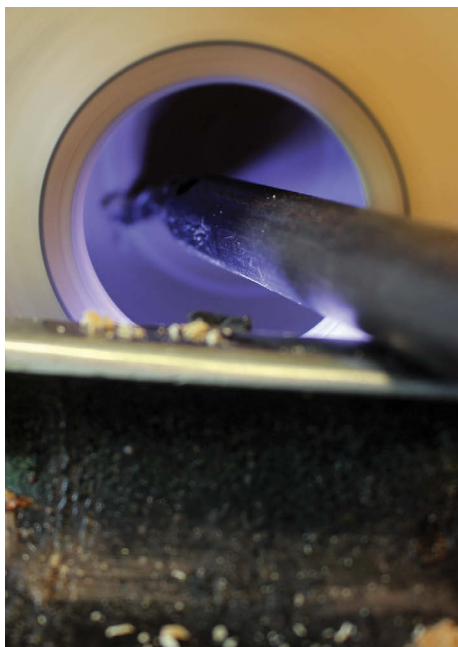
Delicate finishing and refining cuts
