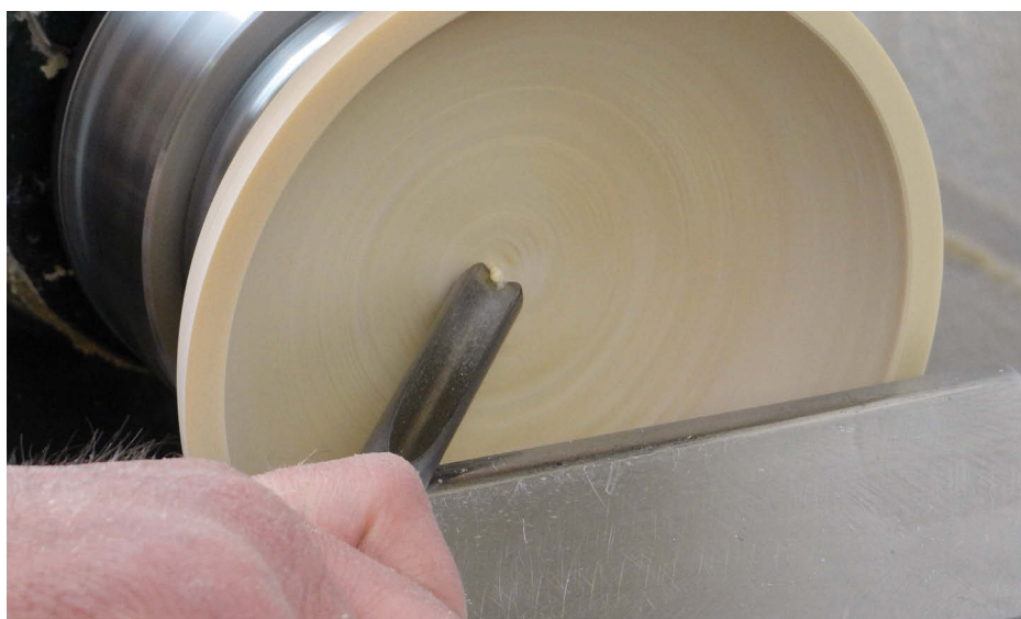
Correctly finishing the inside of a bowl
