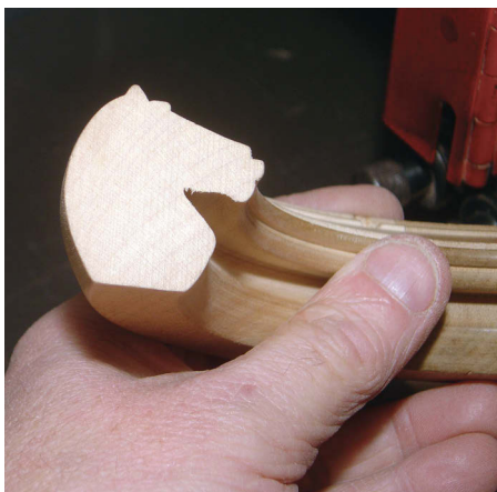
When it is cut the knight profile is revealed. The blank for the ring was made up of two halves, light sycamore and dark walnut, so both light and dark knights were produced from one blank.
