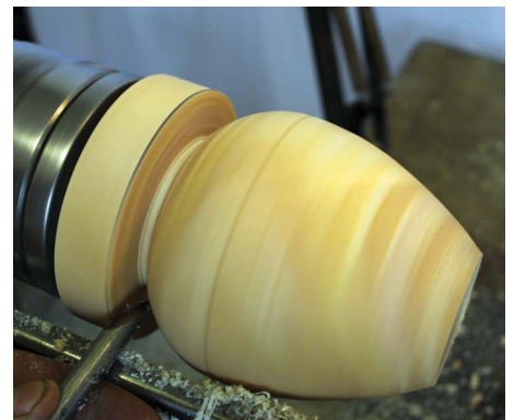
Rough shaping the exterior of the hollow form
