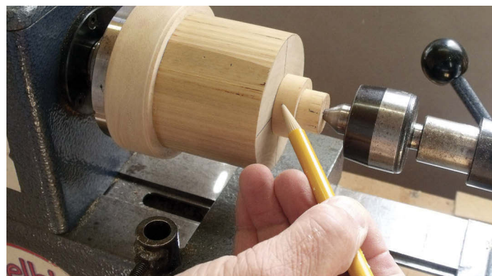
The parts are pushed together with pressure from the tailstock holding them until the glue cools.
