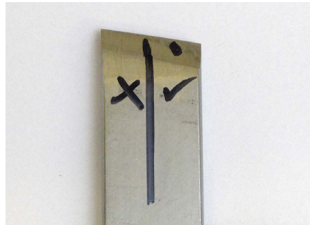
How to mark out a skew to help your planing technique
