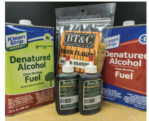
To create your own shellac, flakes and alcohol along with any colourants you wish to tailor the shade
