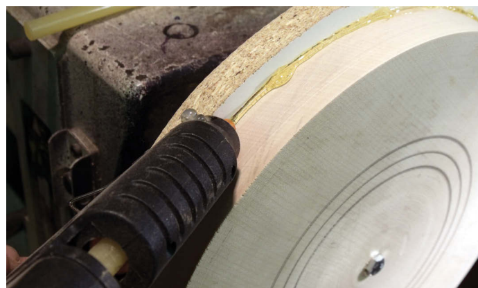
For larger pieces a hot melt glue weld will be enough to hold the work. Do make sure that the weld is substantial. When the turning is complete the weld can be picked off or the glue can be softened using a hot air gun.
