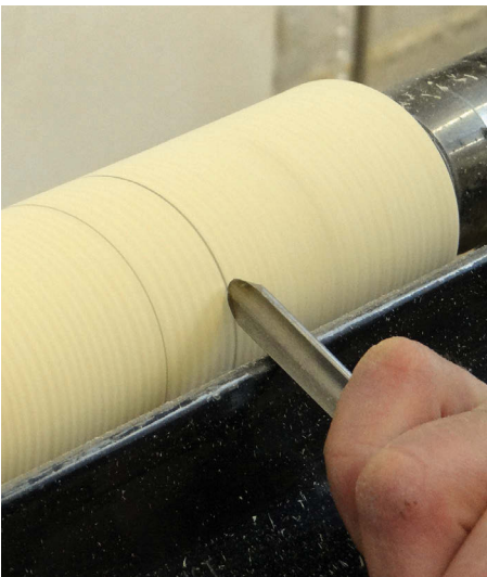
Beginning to cut into a cove, the flute here is too open and so a catch follows
