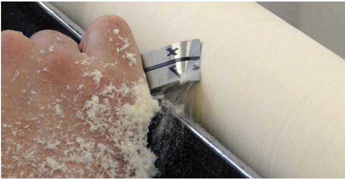
The correct planing position with a skew is in the lower quarter of the cutting edge
