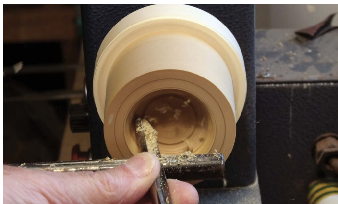
The wood can then be turned, but do take light cuts and wear a face shield. The joined parts can be separated if they are placed in a microwave on full power for 20-30 seconds. But take care – too much heat will cause the glue to become runny and it may soak into the grain.
