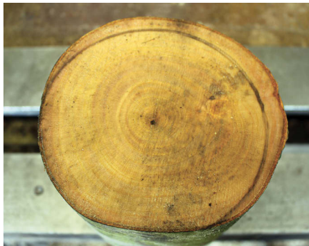
Bottom of the branch showing the location of the pith
