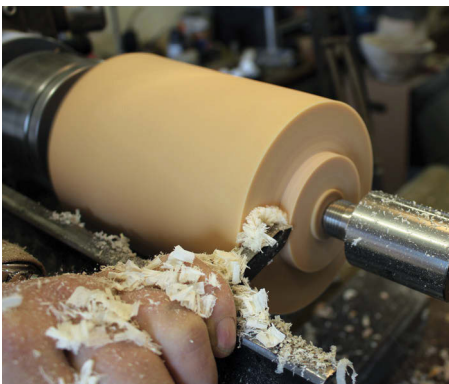
Cutting the tenon for the chuck
