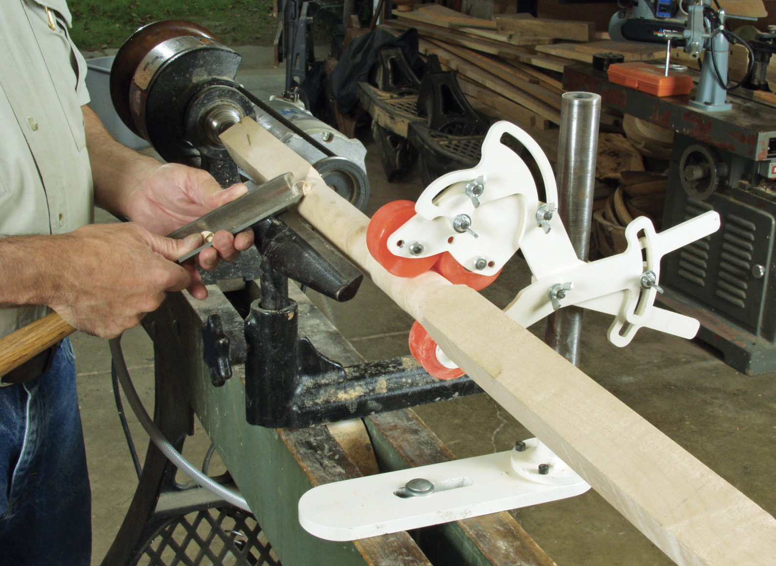
Turning slender spindles with a steady rest is a walk in the park
