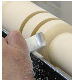
Cutting away from the point makes it virtually impossible to control the cut. This picture was taken a split second before a catch
