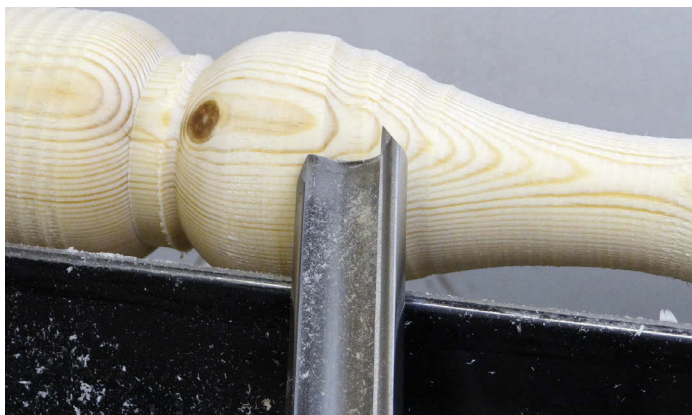
A roughing gouge catch, running up the hill
