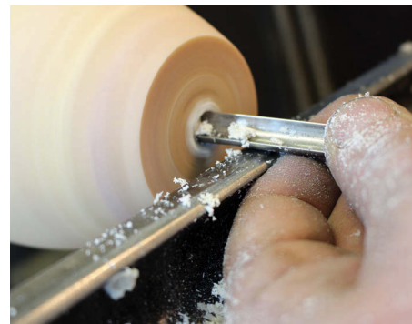
Using a spindle gouge to remove the waste wood
