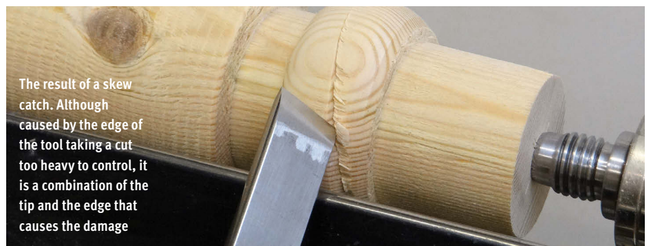
The results of a bead rolling catch with a skew
