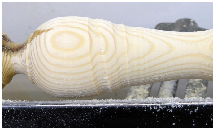
When a catch happens it happens quickly and is uncontrollable and the damage can be small or large
