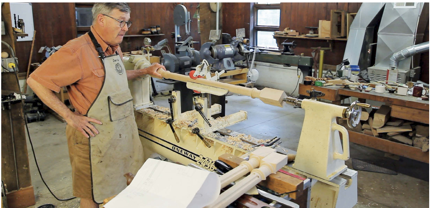
The advantage of having two banjos is enormous – necessary if you are going to tackle production spindle work
