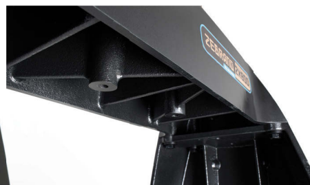
Cast webbing and support struts under the lathe bed
