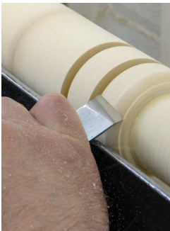
Correctly rolling a bead with the long point of the skew
