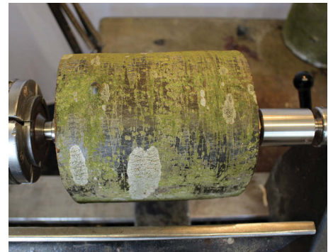
The branch mounted between centres
