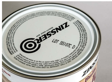
Depending on where you live, there might be date codes on ready-mixed formulations. Key to mfg. dates: second digit – last digit of year, third digit – month (1-9 plus O, N or D), fourth and fifth digits – day of month
