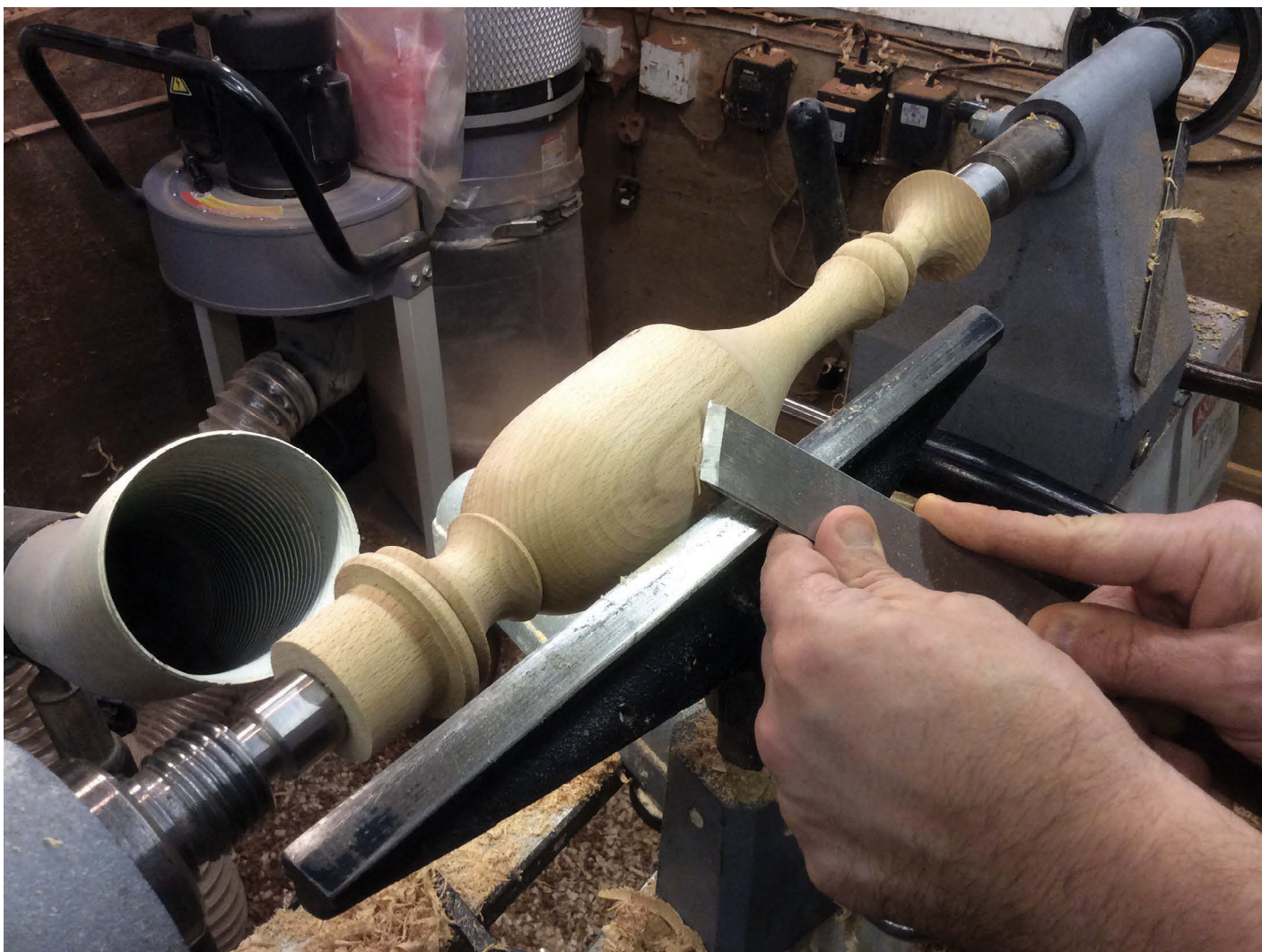
Refining a support column with a skew chisel
