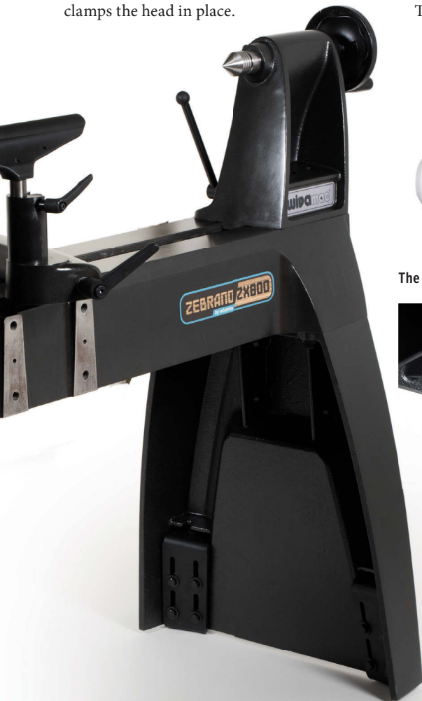
Cast webbing and support struts under the lathe bed
