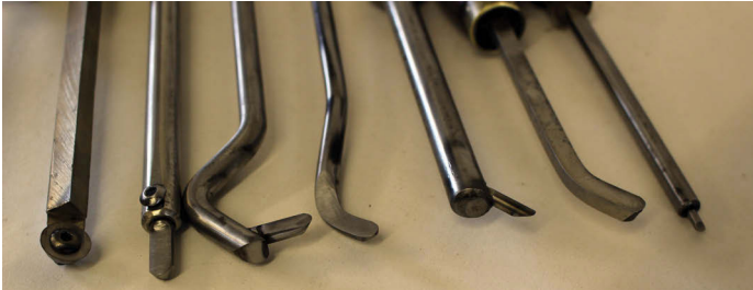
Basic hollowing tools, many of which are homemade
