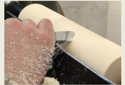
Raising the toolrest while planing can be a great help in learning to control the tool
