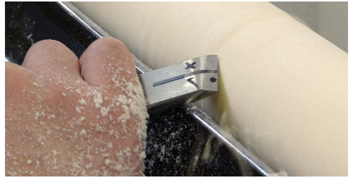
If the cut moves past the centre toward the top of the edge, a catch is sure to follow
