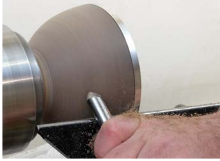
Cleaning the bowl and blending with the rim with my bowl gouge in shear cutting mode
