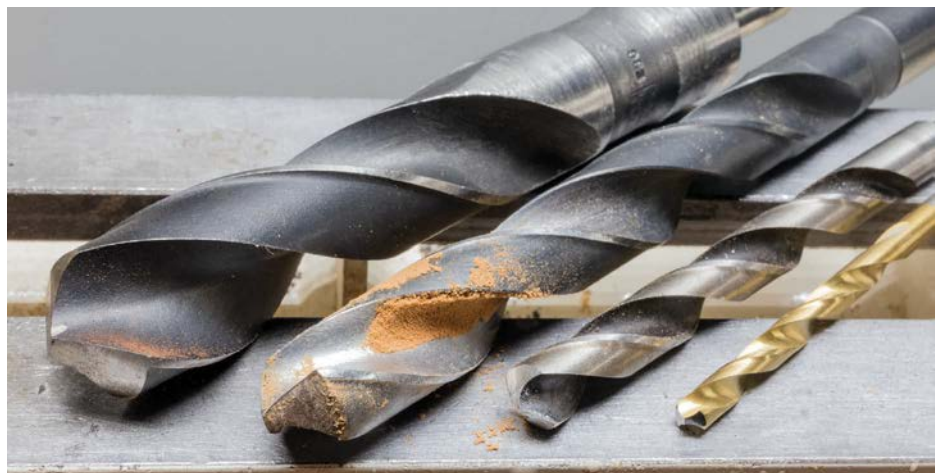
Start small and work your way up to the final size. The quality of the final hole will benefit from the process
