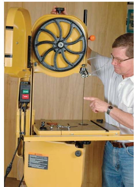
A properly tensioned blade should deflect about \frac{1}{4} in. under moderate finger pressure
