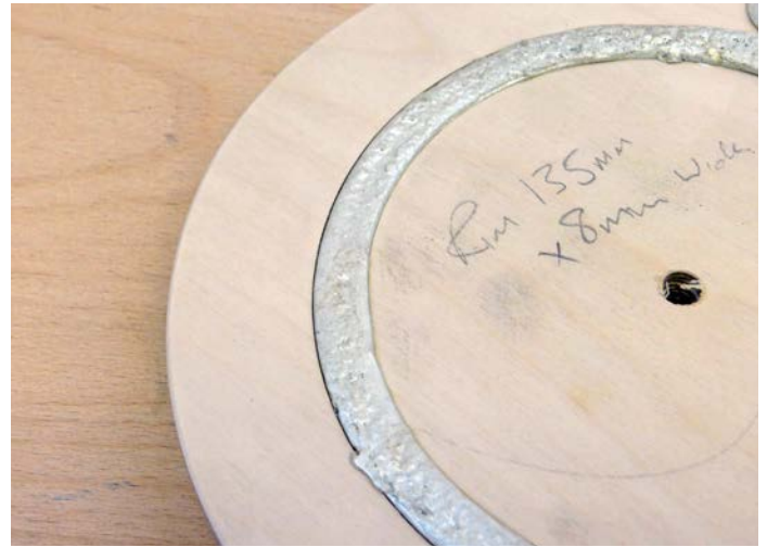
It looks like the cooled pewter has shrunk slightly in the mould
