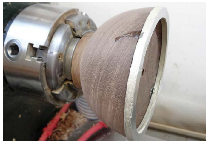
The following morning the epoxy is dry including the dribble down the edge of the bowl
