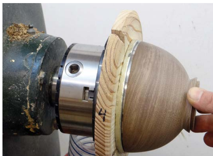
Test fitting the bowl to the pewter rim
