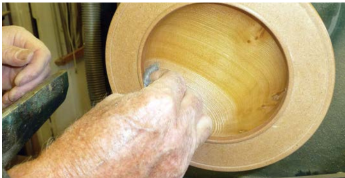
Figure 17. Buffing the inside of the bowl with '0000' wire wool
