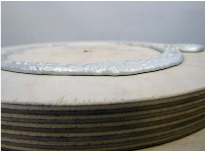
The cooled and cast pewter stands well proud of the mould
