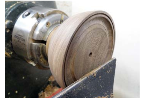
The bowl is turned and the next stage is casting the pewter
