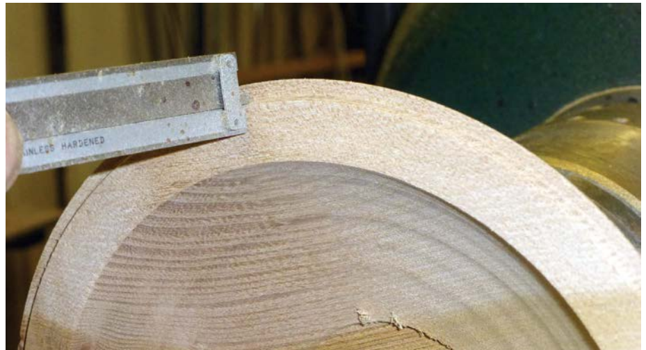
BELOW: Figure 9. Checking the depth of the step prior to fitting the rim
