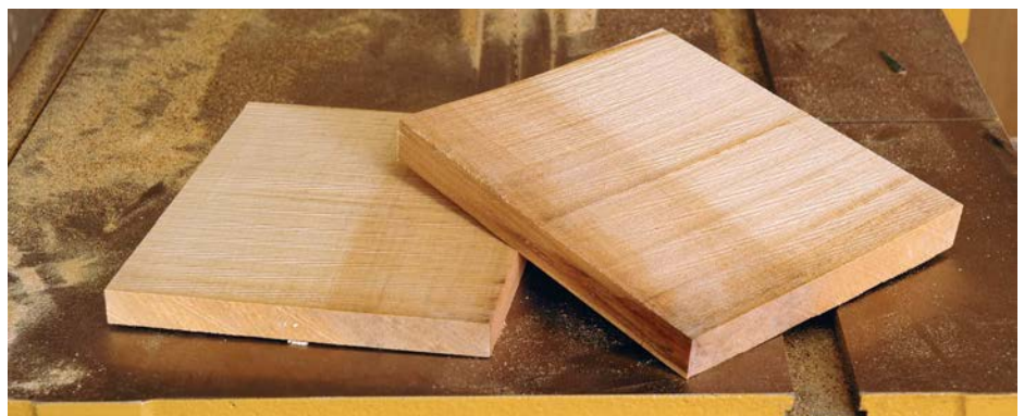
An unlucky combination of blade tension and feed rate can cause a rippled cut like this one
