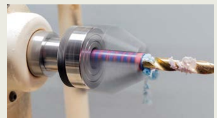
Don't be afraid to practise. Take scraps and drill holes. Try long lengths with thin walls and then check for uniformity
