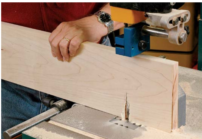
Non-coplaner thrust guides caused by poor adjustment or guidepost flex can cause blowout at the bottom of a cut
