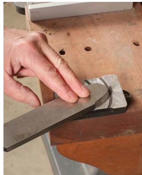
A burr can be burnished on HSS with a Veritas fixture that has a tungsten carbide cone to raise the burr.
