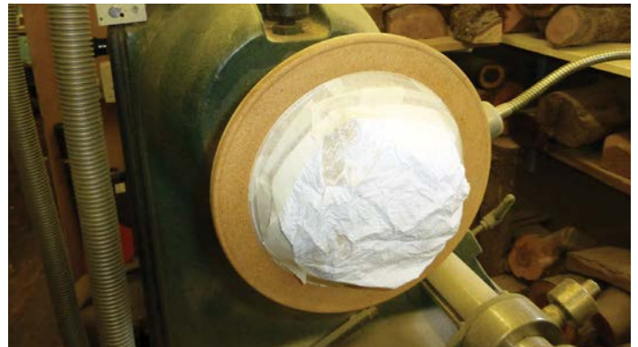
Figure 14. Masking tape after trimming with a skew chisel
