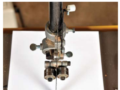
After installing a new blade, make several straight and curved test cuts to ensure that the blade tracks and cuts accurately
