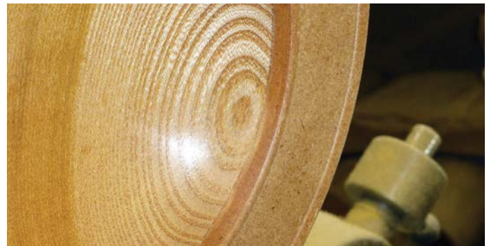
Figure 18. Join between wood and MDF rim with no gap
