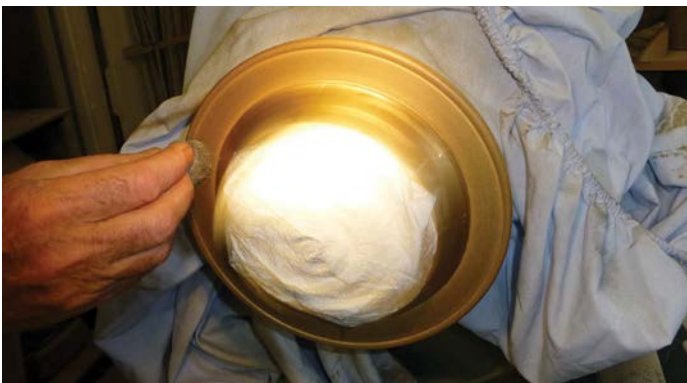
Figure 15. Buffing the gold lacquer with '0000' wire wool
