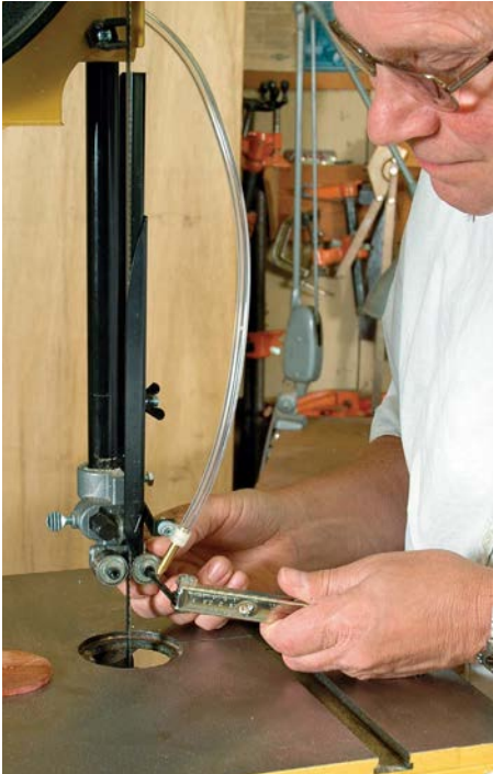
Before removing the old blade, retract the side guides and thrust bearing so they won't interfere when tracking the new blade
