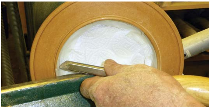
Figure 19. Rimming the masking tape with point of skew chisel
