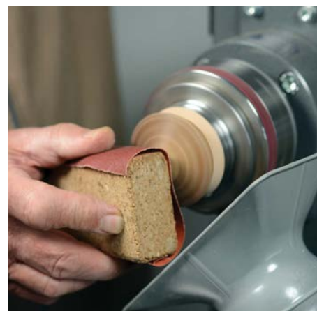
Sanding the lid with a block
