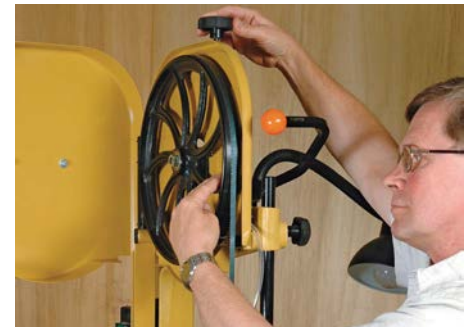
Simultaneously tension blade while rotating the upper wheel by hand
