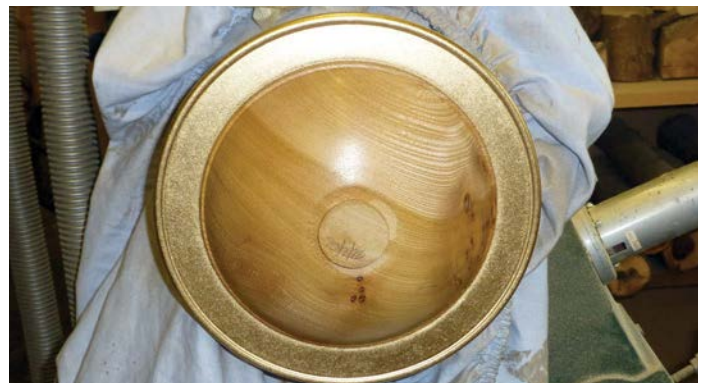
Figure 16. Finished underside of bowl with tape removed
