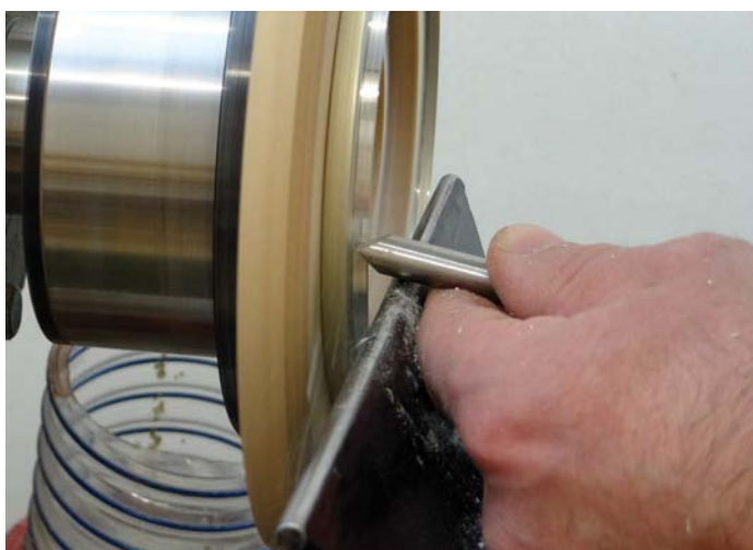
Beginning to shape the tongue on the pewter
