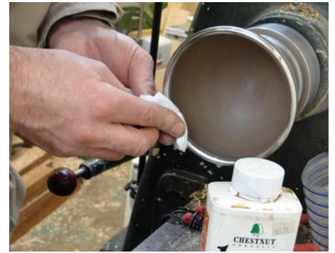
Burnishing the pewter – very carefully – to a high shine
