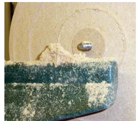
Figure 11. MDF finish straight from the tool
