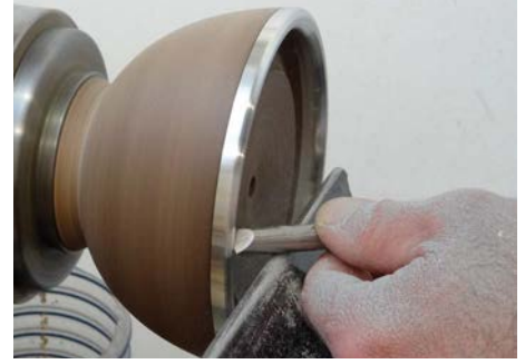
Shaping the pewter with my scraper – notice the metallic dust from the tool
