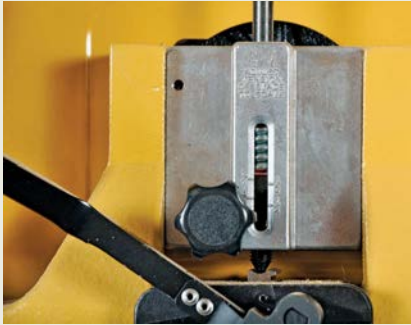
Completely compressing a tension spring as shown here can result in premature spring failure
