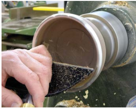
Turning the inside of the bowl
