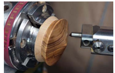
Setting the swing diameter outside
