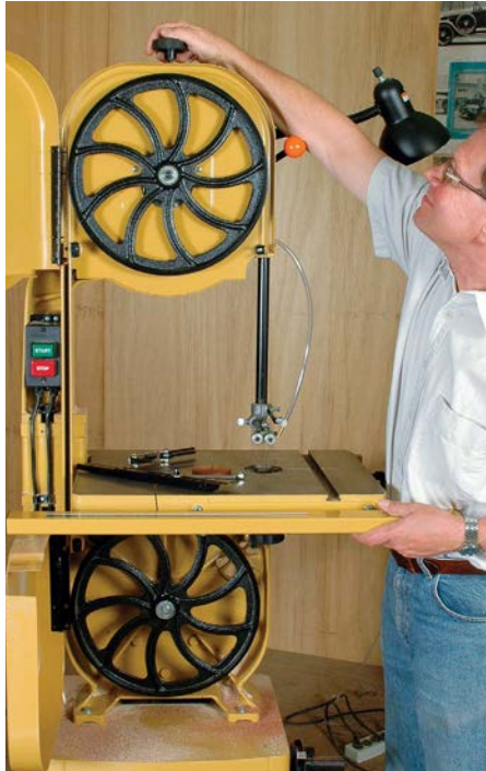
To release the old blade, first back off the tension adjustment knob, wheel, or lever
