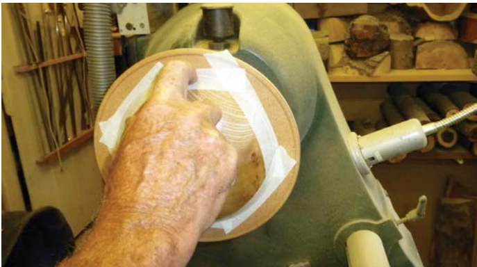
Figure 13. Bedding the masking tape with my finger
