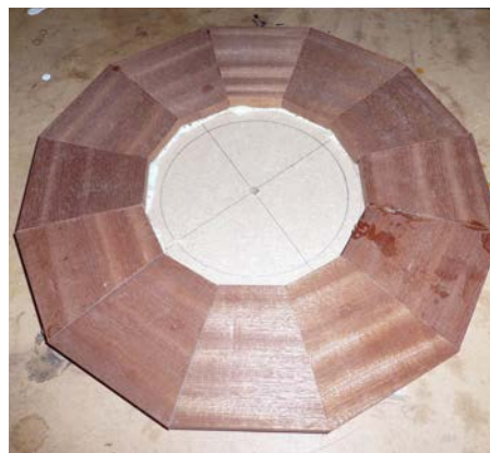
Figure 10. A wide rim made of segmented mahogany mounted on MDF prior to turning
