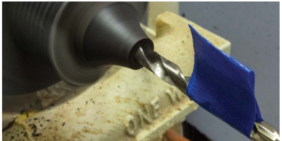
Every species and every orientation is liable to give you a slightly different final result. If needed, drill a test piece to find out
