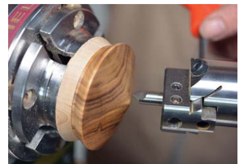
Setting the swing diameter inside
