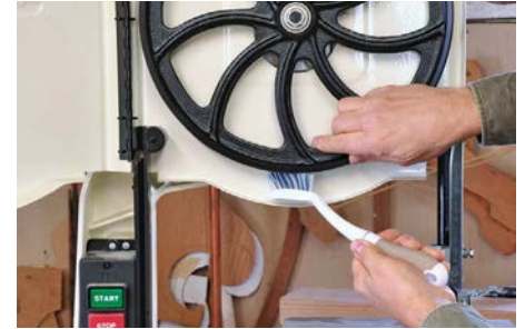
Clean debris from tires using a stiff nylon – or brass-bristle brush
