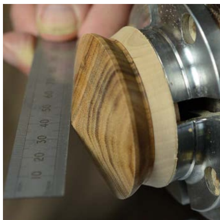
Checking the lid for flatness
