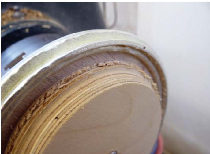
Turning the pewter from the ply mould
