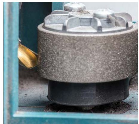
My drill sharpener accurately positions and presents the bit to the diamond wheel when it is running. Safety cover removed for visibility
