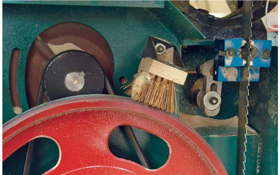
A stiff-bristle brush mounted in the lower wheel house helps clear sawdust off the tire.
