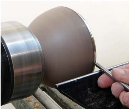
Adding the tiny V cut between the walnut and pewter
