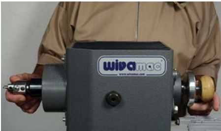
Inserting and securing the boring head
