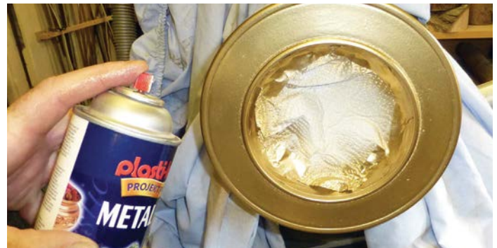
Figure 20. Gold base coat being applied
