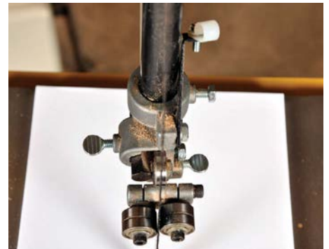
This misaligned guide assembly causes the side guides to be out of parallel to the blade. In the photo at far right, the guide assembly has been rotated on the guidepost to bring the guides into parallel with the blade
