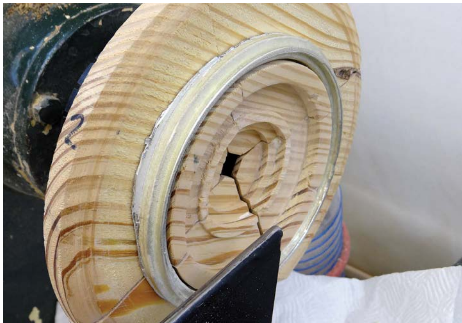
Holding the pewter ring with my wooden plate jaws in expansion mode
