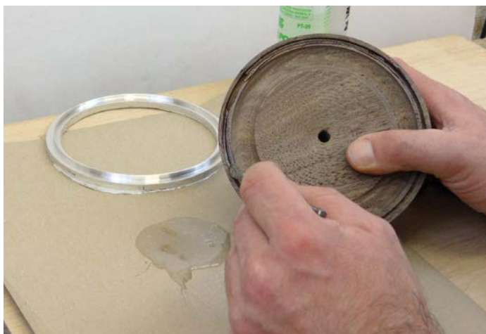
Carefully spreading the epoxy around the rim of the bowl
