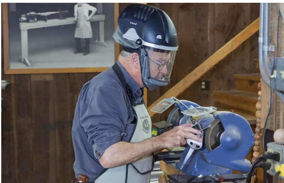
HSS can be ground with impunity because the temper created is not high enough to draw the temper.
