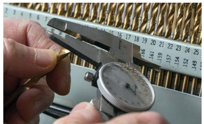
If size is important, measure! You measure a drill diameter across the edges that do the cutting
