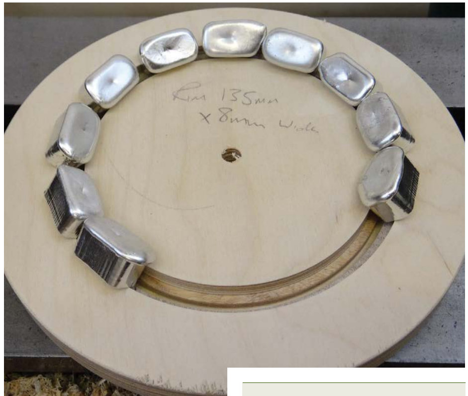
The mould with the pewter ingots
