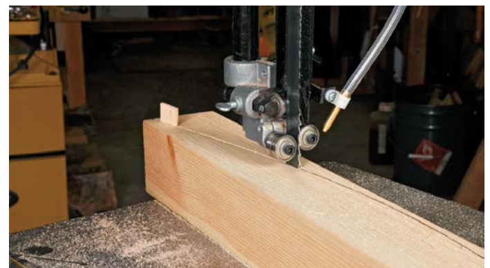
Blade binding in a cut can be eliminated by inserting a wedge into the cut
