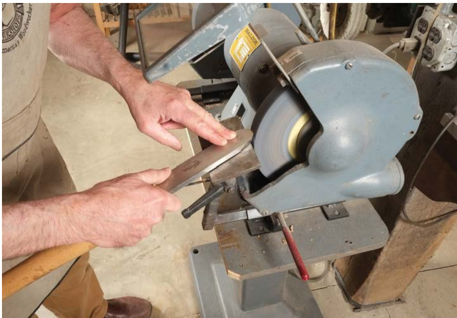
Grinding causes a burr to form through plastic deformation on the top and bottom about equally.
