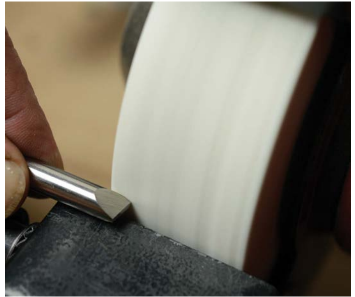
Relieving top of tool on grinder
