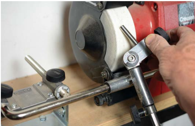
Tormek's jig is adapted for dry grinding
