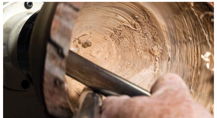
Not too common with the retailers any longer, my 25mm shaft bowl gouges have performed admirably
