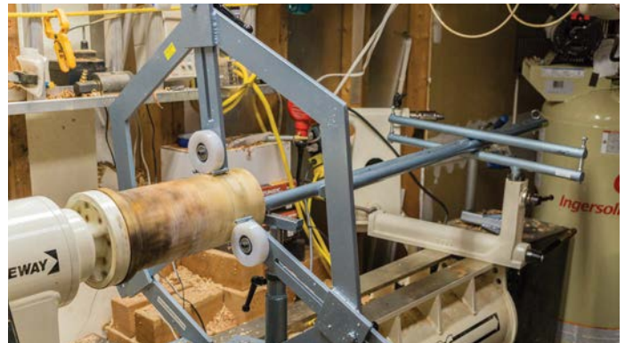
The huge mechanical advantage lies in the long, massive bar that is captured as well
