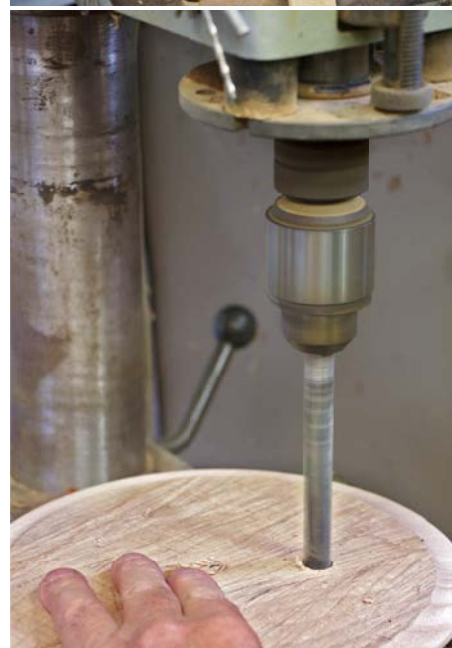
TOP: Using scrap that's equal in thickness to the proposed thickness of the plate, set the drill depth. BOTTOM: Drilling two depth holes will help you achieve a flat surface across the center of each plate
