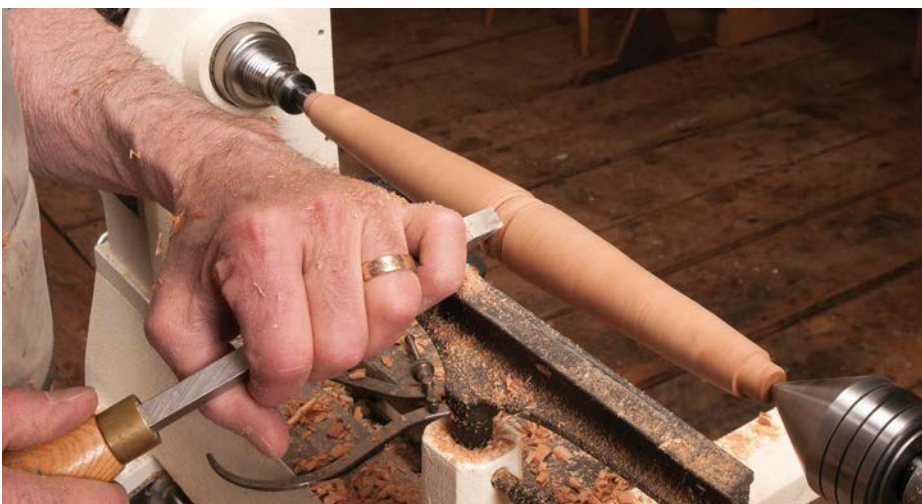
Turning between centres allows an infinite amount of re-chucking with no loss of concentricity
