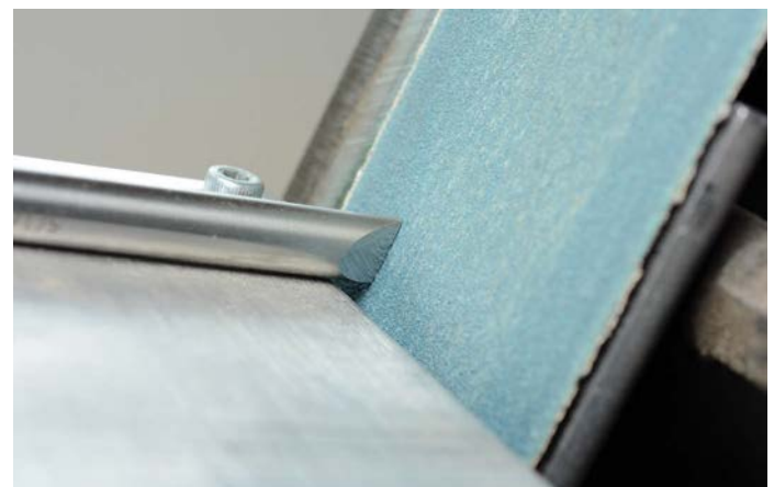
Truncating a point tool on pro-edge
