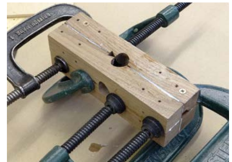
Glued up and ready for the last screws to be fitted before leaving to dry overnight
