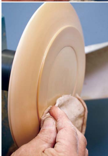
Sand and polish the base of the plate. I sand plates to 320 grit, finishing with a rotary sander to eliminate concentric sanding marks
