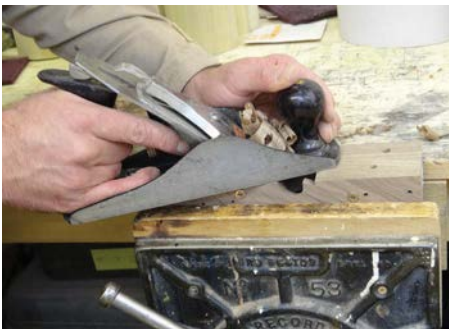
Flattening the pairs of quadrants to make sure I achieve a good tight join
