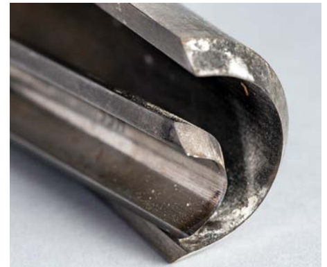
There are occasions when the smaller spindle roughing gouge is in order; less edge in the mix
