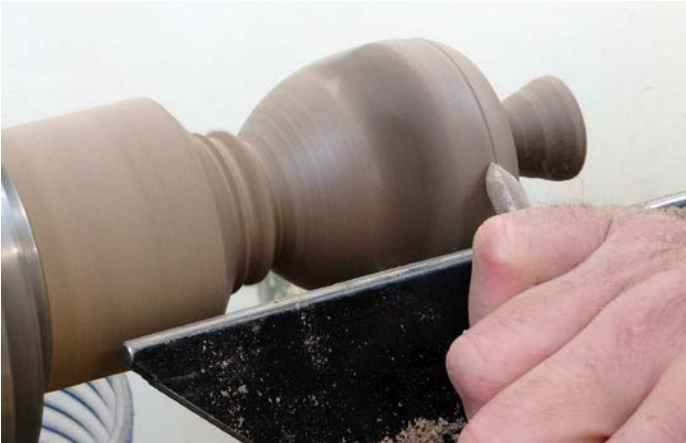
Developing the outer apple shape
