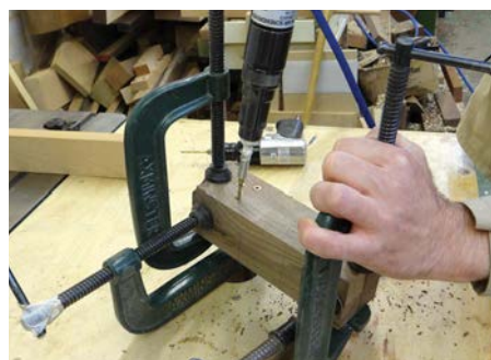
With the quadrants held securely with G-cramps I can drive in the securing screws
