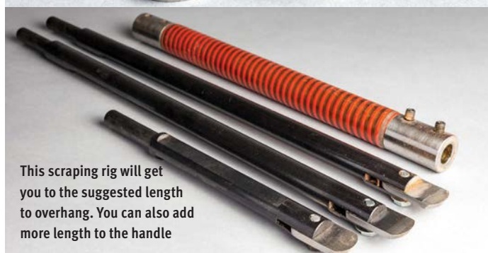
By design and manufacture, spindle roughing gouges are weakest right at the tool handle insertion point
