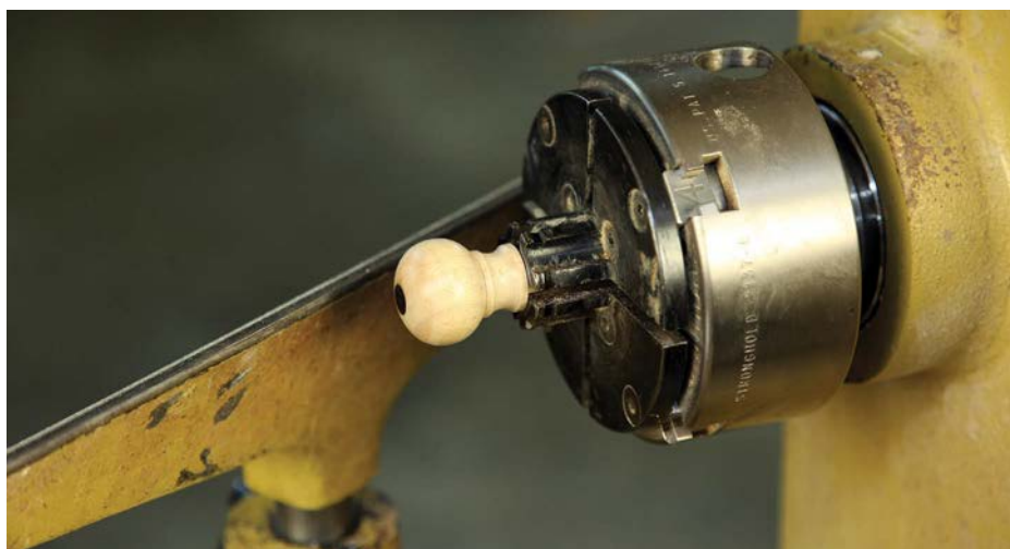
Using tower jaws to finish the front of a between centres spindle-turned knob
