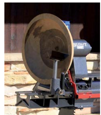
The optional bed extension gives 16" of increased spindle capacity. Used by the headstock, you can turn outboard to 21"
