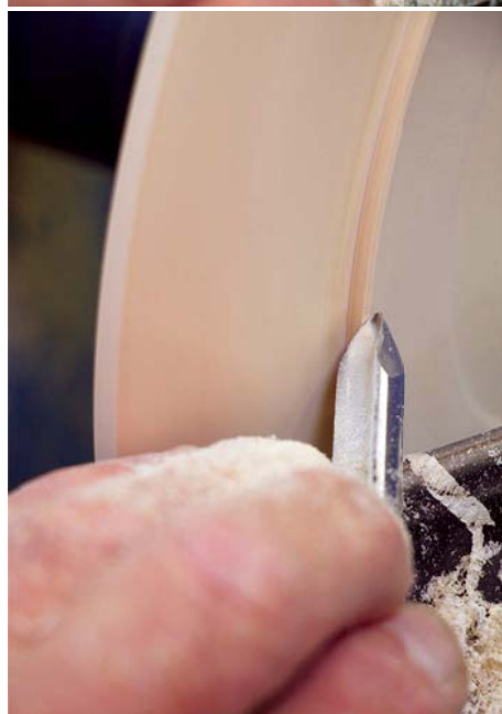
Round over the foot using a \frac{3}{8} in. (10mm) detail or spindle gouge
