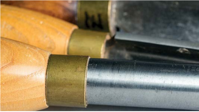
By comparison, my 25mm bowl gouge is incredibly strong throughout its length and dampens vibration wonderfully
