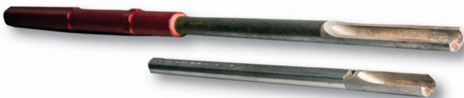
This illustrate some of the ideas for tools. Put the important steel where it needs to be. Strengthen elsewhere
