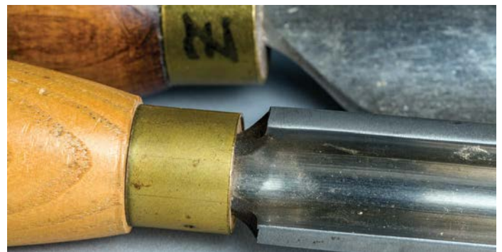
By design and manufacture, spindle roughing gouges are weakest right at the tool handle insertion point
