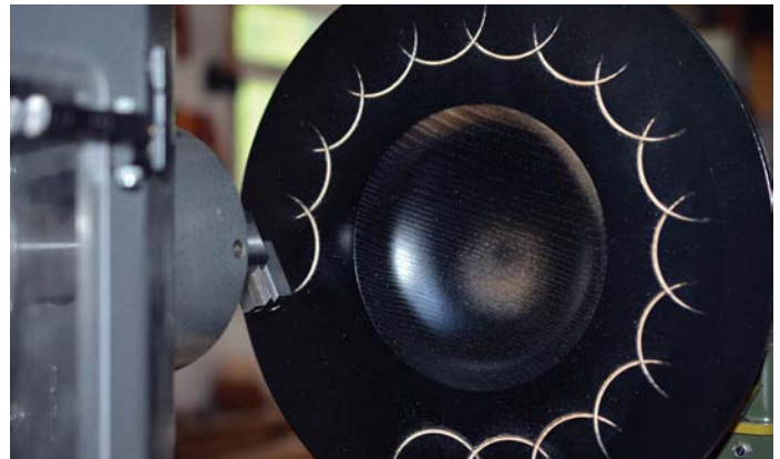
Cutting crescents on an ebonised platter, because I wanted to cut less than a full circle the work had to be rotated to present the less than half the face to the cutter
