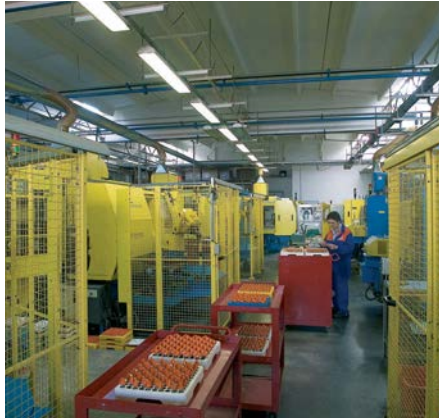
Loading the automated multi-axis CNC sharpening machines.
