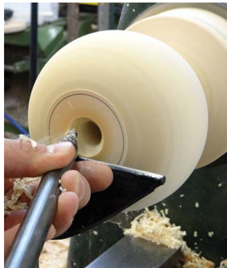
Beginning with the slender carbide tipped tool
