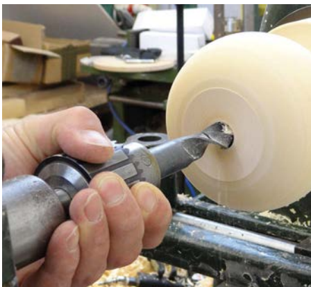
Drilling the initial hole
