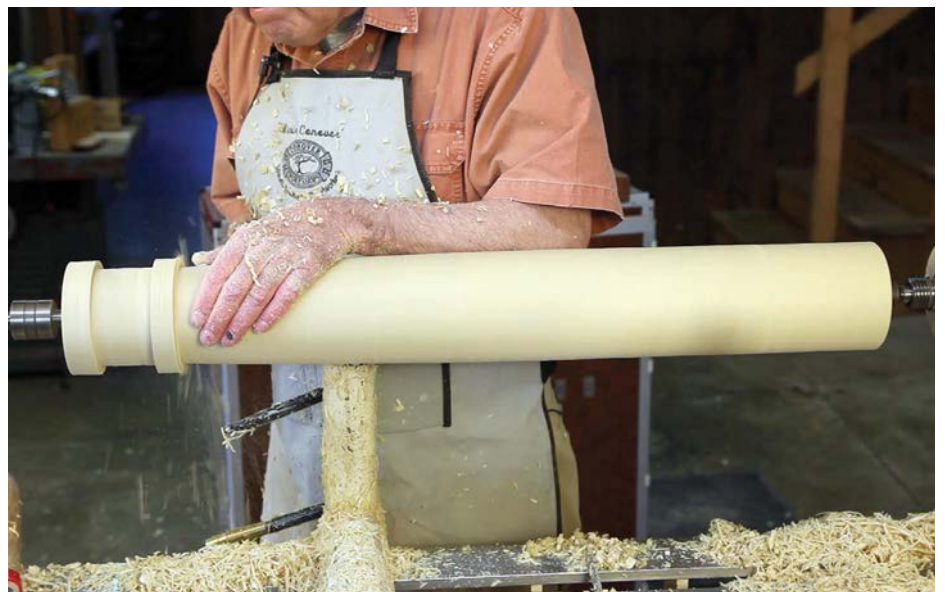
Turning architectural parts takes a heavy lathe with lots of between centre distance
