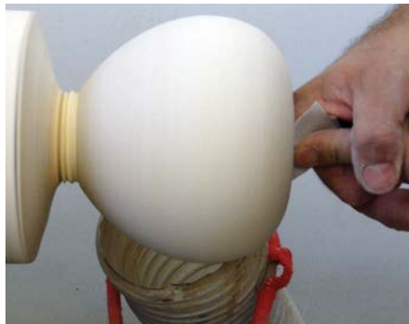
Sanding as far as I safely can inside by hand
