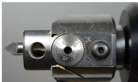
The boring bar is 2 MT and fits in the headstock, photograph shows Vernier scale for adjusting offset and a point tool in the front slot
