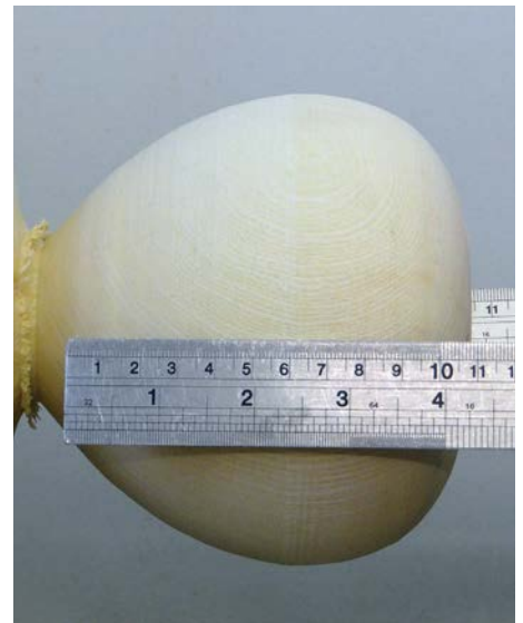
I also use rulers to check the depth
