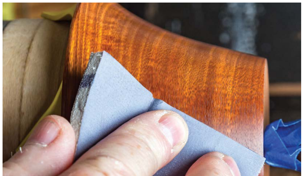
Once at the final coat, 1 or a number of them, a final sanding though the Micromesh will smooth and shine to a gloss if desired
