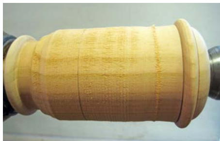
Figure 5. Support the body between the multi-purpose jig and a live centre. Start the turning with the two 10mm wide beads. Measure the position of the waistline, mark and using a spindle gouge begin the shaping to give a nice curve
