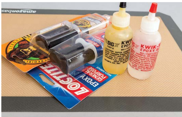
I've used the five minute structural epoxies for finishing but they are more suited to small items because of their viscous nature
