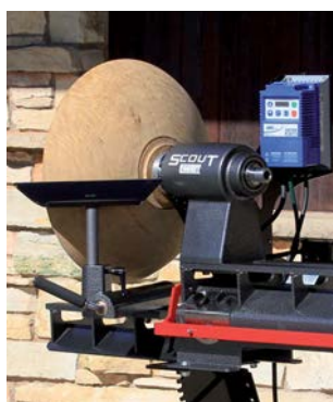
The optional bed extension gives 16" of increased spindle capacity. Used by the headstock, you can turn outboard to 21"
