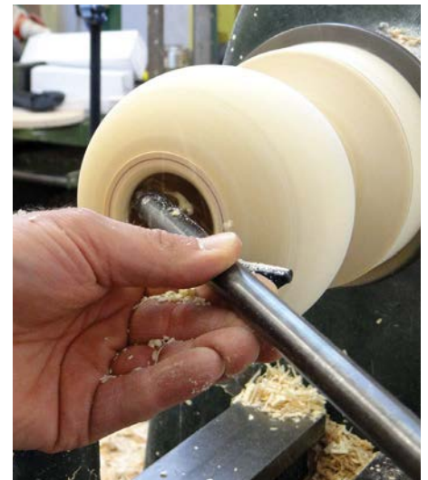
The straight tool can manage a surprising amount of hollowing before the crank is required
