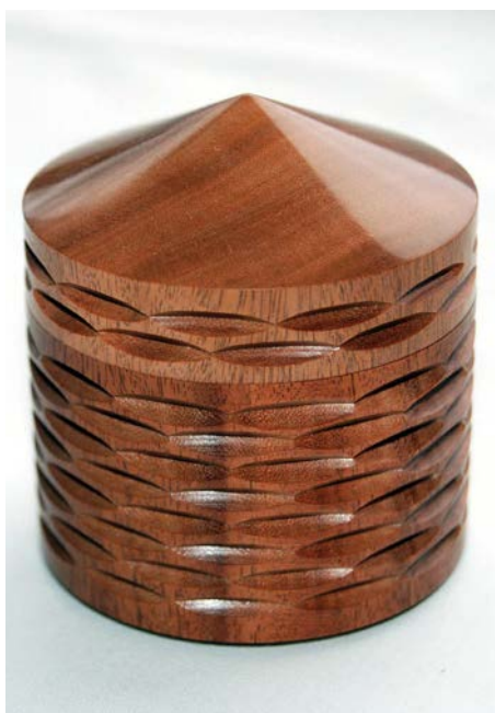
A threaded lid box in Quebracho ( Schinopsis ) with decorated cylinder. 12 divisions of 30°, the first row is cut and the work advanced forward then moved around by 15° to give the offset, this is then alternated until the pattern is complete. The cutter was a straightforward point
