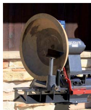
The optional bed extension gives 16" of increased spindle capacity. Used by the headstock, you can turn outboard to 21"
