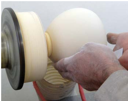
Sanding the outside of the form
