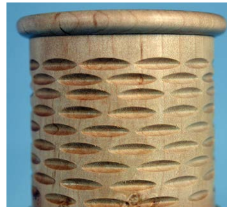
Field maple ( Acer campestre ) pencil pot with cylinder decoration 12 divisions of 30° each. Point cutter
