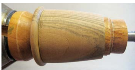
Figure 7. Multi-purpose jig fixed in the chuck jaws
