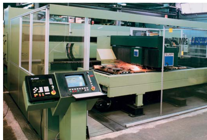
Laser cutting the steel plates.
