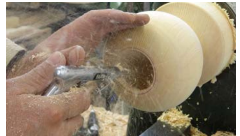
The airline easily clears the shavings from inside the form
