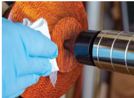
The layup epoxies, West Systems, System 3, or equivalents can be brushed on, applied with rollers, or by hand with a towel
