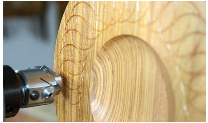
Fig. 1 – Cutting an olive ash ( Fraxinus excelsior ) platter is at right angle (90°) to the lathe bed/axis
