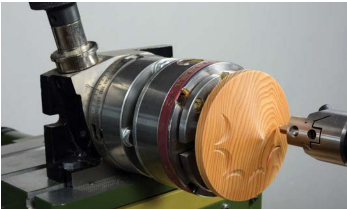
Workpiece at 90° to the lathe axis, cutting part circle or crescent finished piece
