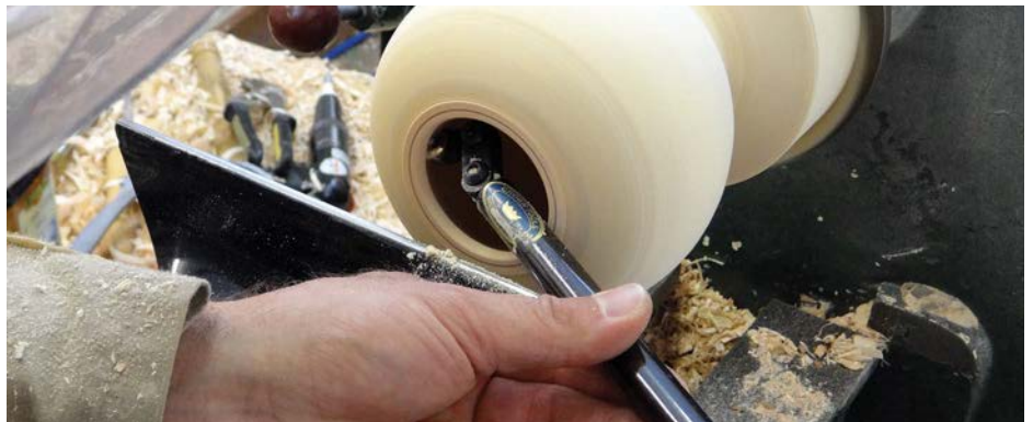
Beginning to work on the shoulder with the tool
