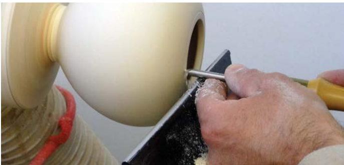
Using my point tool to cut a 'v'-groove near the rim
