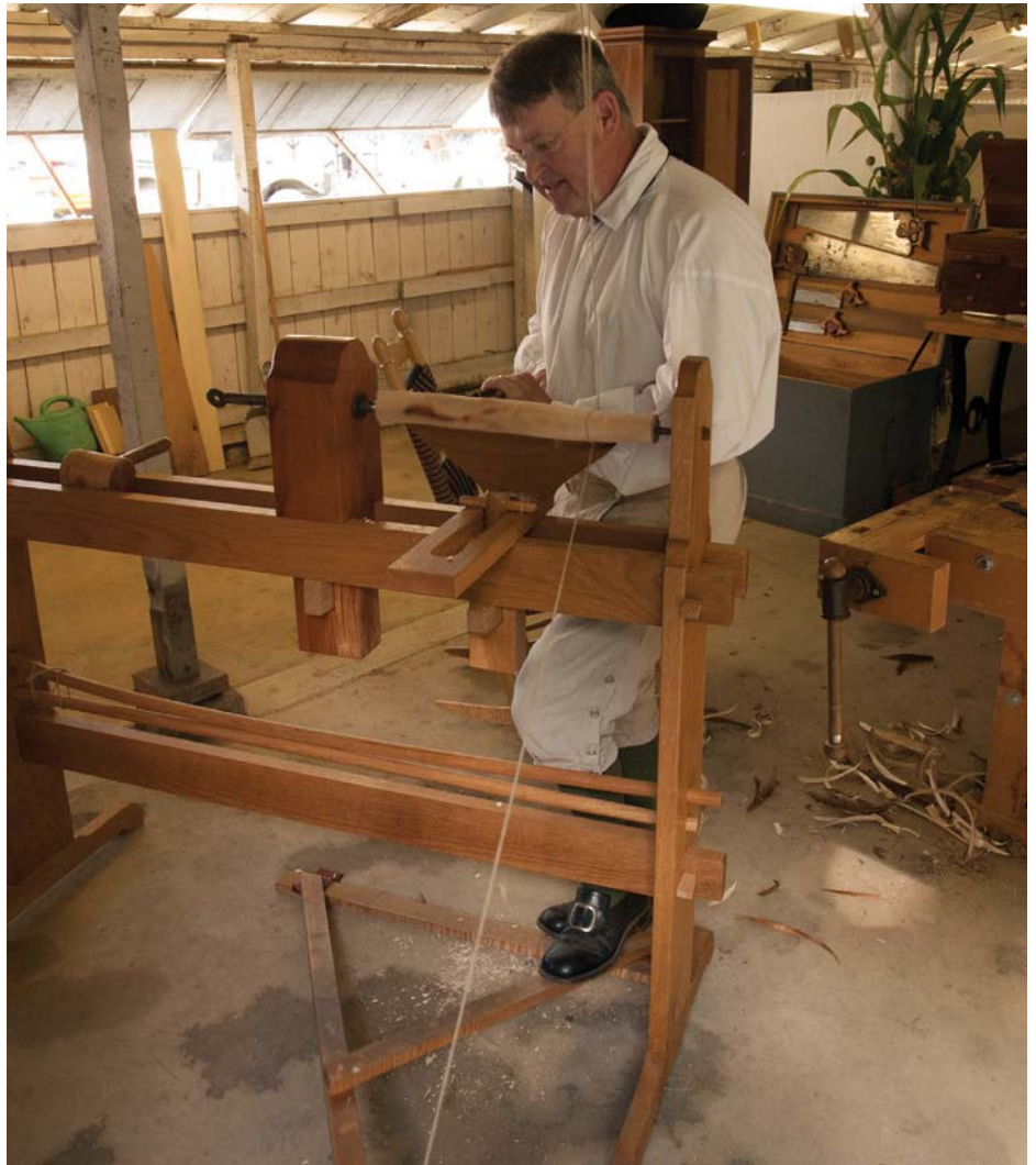
A spring pole lathe requires non-stretch cord. We made our own from linen, which yielded long-wearing, stout cord. The treadle is near the bottom of its stroke here and is about 1.1m off the ground at the top. While many think the rope ends under the lathe it actually ends far in front of it. It is pulled forward and down by the treadle
