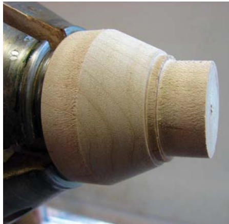
Fig 7. Multi-purpose jig awaiting the bottom of the base
