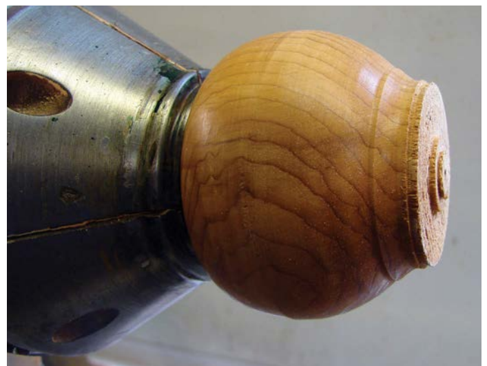
Fig 10. The top's final turning about to be completed on an earlier yew top
