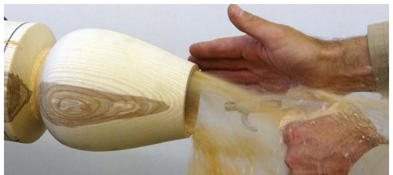
Using an air gun to clear out shavings
