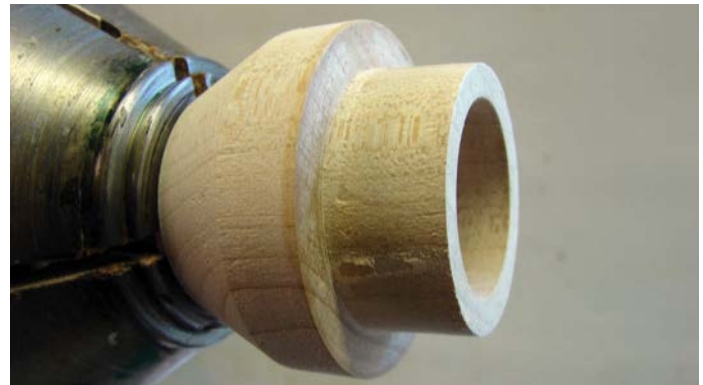
Fig 11. The multi-purpose jig held in chuck jaws
