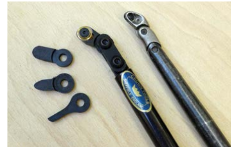
... and finally a couple of the hollowing tools available in the shielded cutter category
