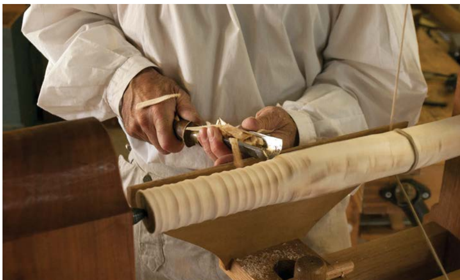
Turning on a spring pole lathe requires sharp tools to get results
