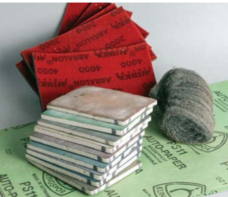
While you can level any ridges with 400 or 600 grit abrasives, you'll need finer to get to a high gloss or steel wool to matte back
