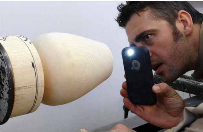
Using the torch on my phone to inspect the inside of the form
