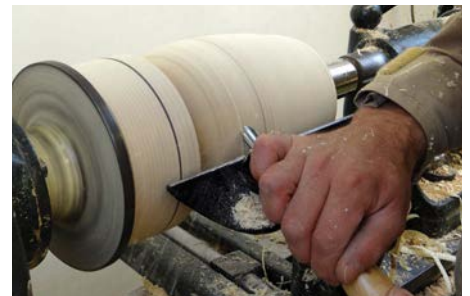
Forming the outside shape is pretty much standard spindle turning
