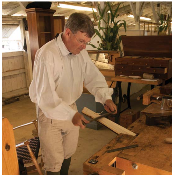
Riven billets are further shaped with a drawknife before mounting in the spring pole lathe
