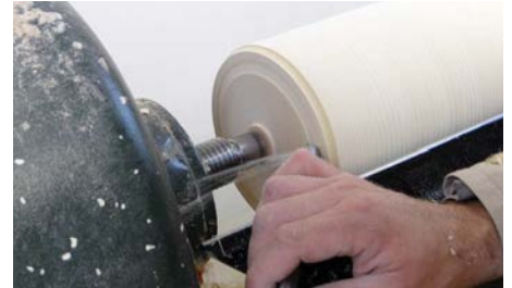
Flattening the end ready to fix the faceplate
