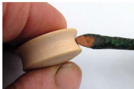
This small round-nosed scraper was made from a scrap piece of Roman bronze and used to create the cove in the stud
