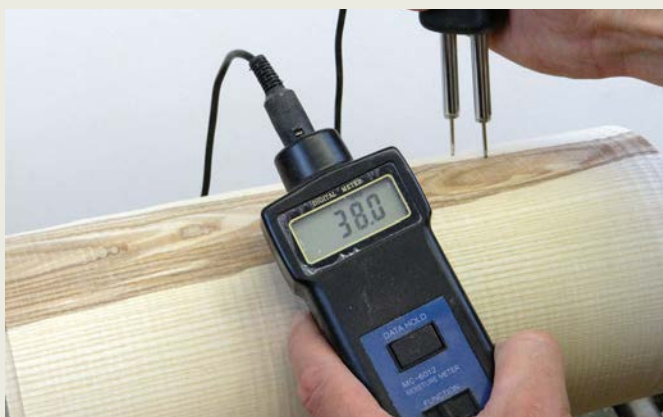
My moisture meter reads 38% on the ash blank I'm working on
