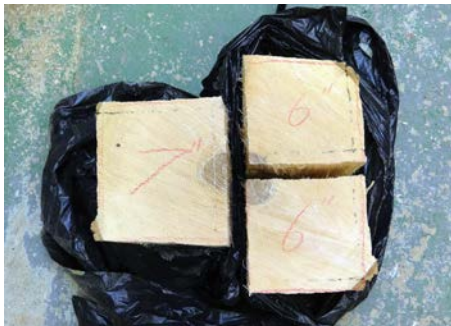
The ash log cut up, showing the larger section which may move and the two smaller pieces which should be more stable
