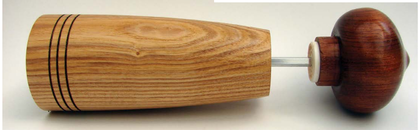
Fig 14. The top placed over the shaft to indicate the amount of shaft to be removed
