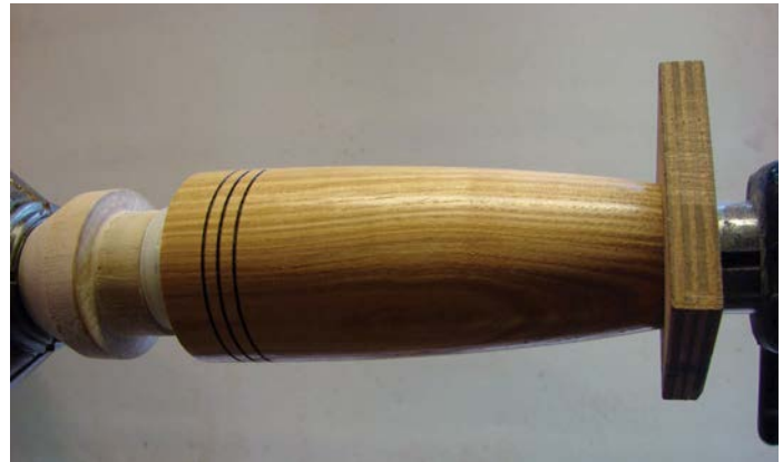
Fig 13. Everything in place and waiting for the tailstock barrel to be wound in
