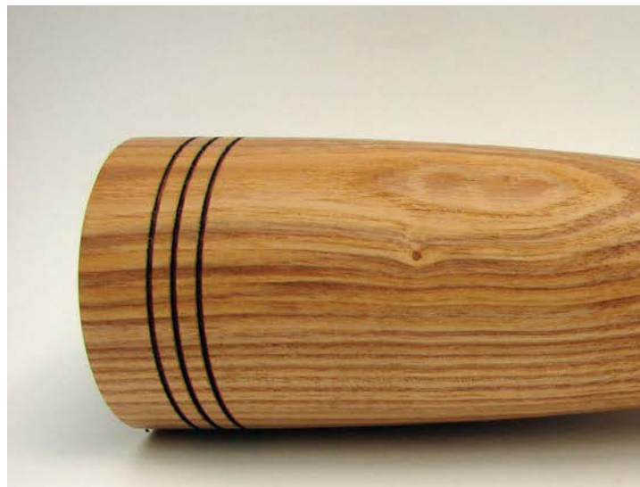
Fig 14. The top placed over the shaft to indicate the amount of shaft to be removed
