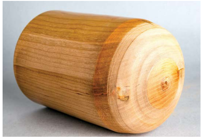
The practice piece with only six coats of Ca applied to the flat cylinder surface. No levelling, sanding or buffing yet. Imagine 20 coats
