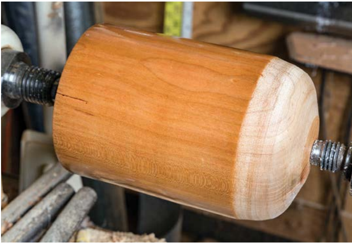
Continue to build to the desired finish. Use the same sequence of one accelerator application followed by three applications of Ca
