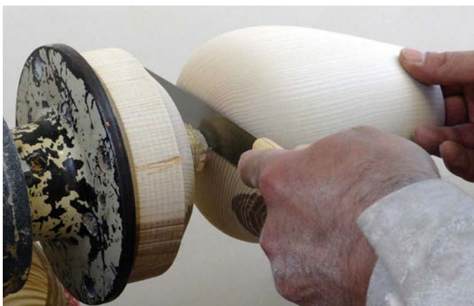
Sawing off the form
