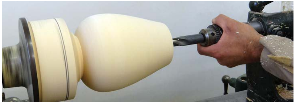
Drilling a central hole in the form
