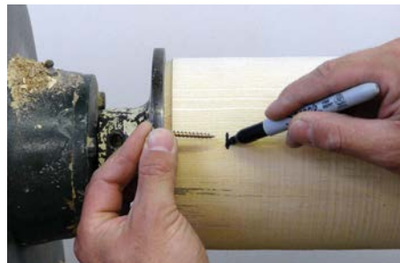
Marking where the screws are
