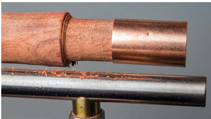
Rather than measure, I use the ferrule to test fit for size. Fast, easy and accurate. Turn until you like the fit
