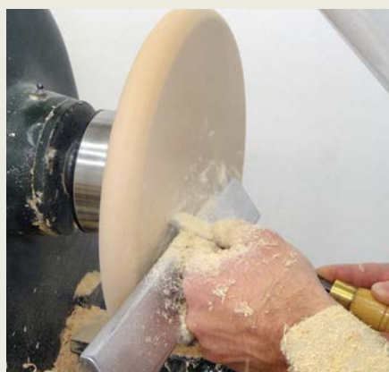
Flattening the face with a skew used as a negative rake scraper
