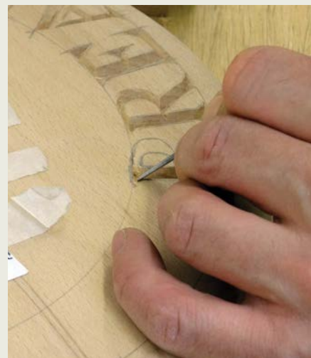
Using a tiny straight chisel to blend the two cuts together
