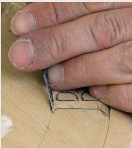
Using a small straight chisel to meet the curve of the serif
