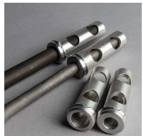
ABOVE: Your drilled size will usually fall into a couple of standard diameters but the square, rectangular and tapered vary. RIGHT: Adapters are available so you can accommodate a couple of different shaft sizes with one hole diameter
