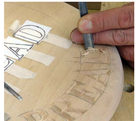
Making my way around the curve with more stab cuts
