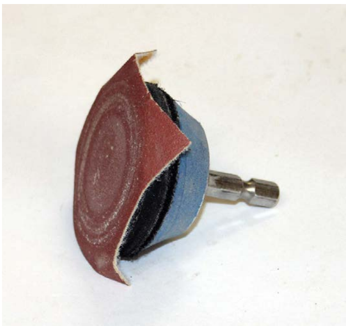
Sanding arbor for a drill
