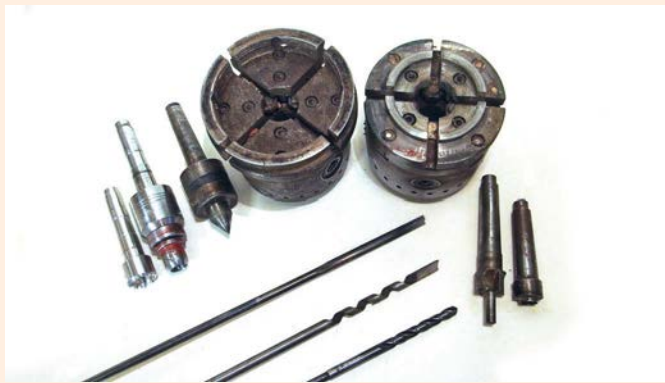
LEFT: Three standard head and tailstock drives which can be useful MIDDLE TOP: Chucks with 55–75mm internal jaws and large grip 90mm+ jaws RIGHT: Standard long hole boring centres BOTTOM: Shell auger, twist auger, twist auger
