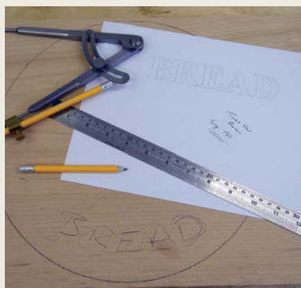
With the board marked out I sketch the lettering roughly the size I want and find a suitable font size
