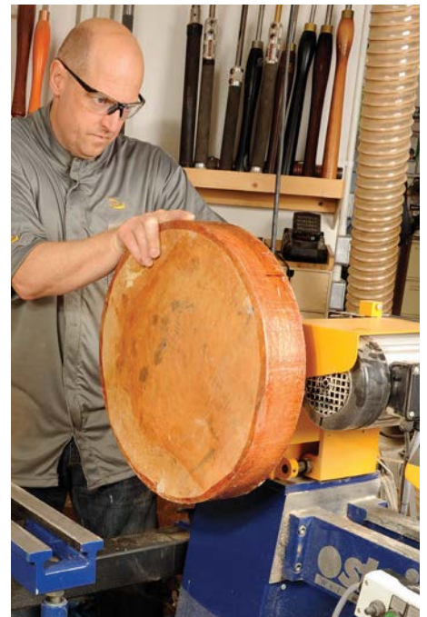
Fitting a large blank on the lathe ready to use the BTA
