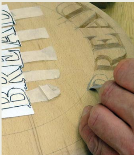
Beginning the serif with a curved gouge 'upside down', slicing with a twist of the gouge
