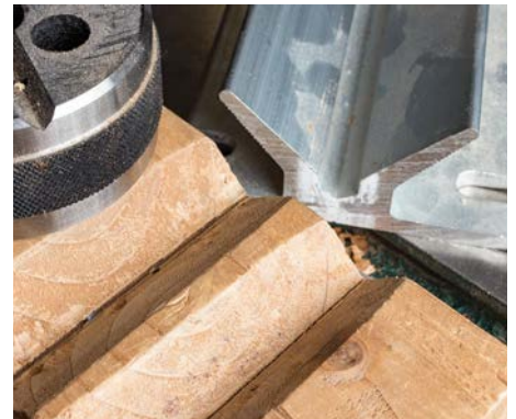
For drilling and cutting of round stock, a V block is essential. Store bought or shop made will be an asset
