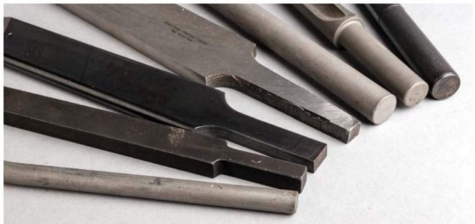
ABOVE: Your drilled size will usually fall into a couple of standard diameters but the square, rectangular and tapered vary. RIGHT: Adapters are available so you can accommodate a couple of different shaft sizes with one hole diameter
