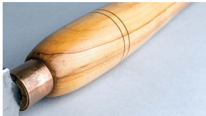
My favourite finish is Ca adhesive. After 15 years of use, this homemade tool and handle still look good
