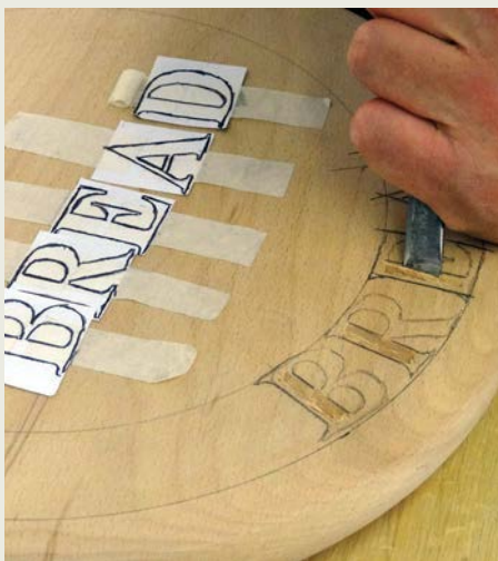
Using a straight carving chisel in a stab cut to widen the V shape
