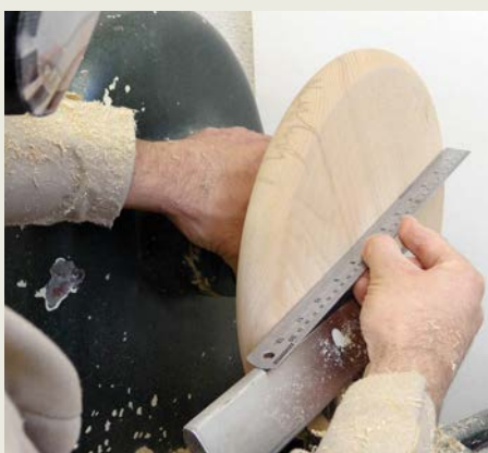
Checking it is flat with a steel ruler
