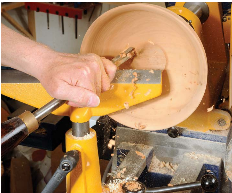
Turning a typical bowl over the lathe bed
