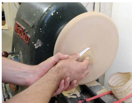
Sanding the board with abrasive wrapped around a cork block
