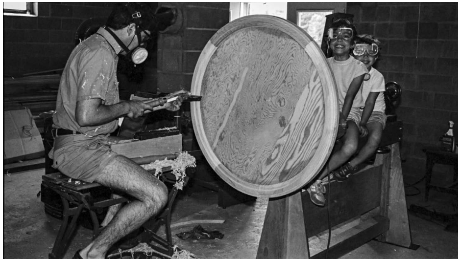
Ernie turning the ceiling medallion, with a little help from his children. Note: this is a very old image and current safety thoughts would go against doing this now
