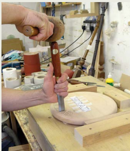
The first cut is with a mallet and bevel edged chisel
