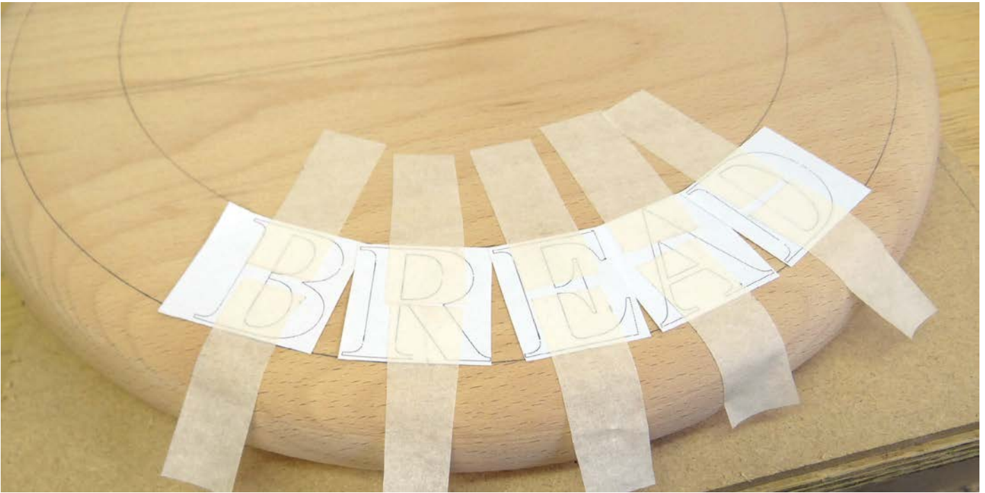
Having cut out the letters I position them around the edge of the board. Once happy, I fix them in place with masking tape
