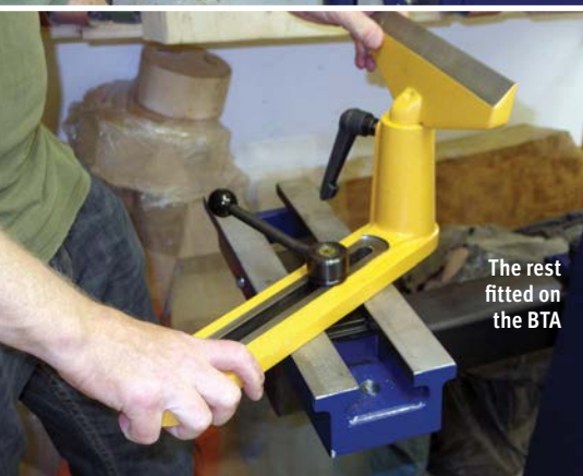
Using the bowl turning attachment, heavy duty cuts were no problem
