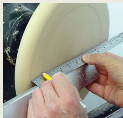
Marking out the position for the lettering
