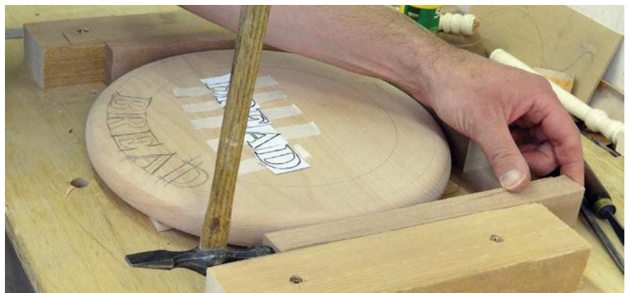
Fixing the breadboard in place with wedges
