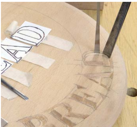
This shows how two different curved gouges make up the shape of the D
