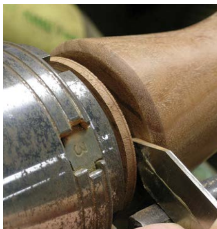
The form was cut free of the chuck with a parting tool
