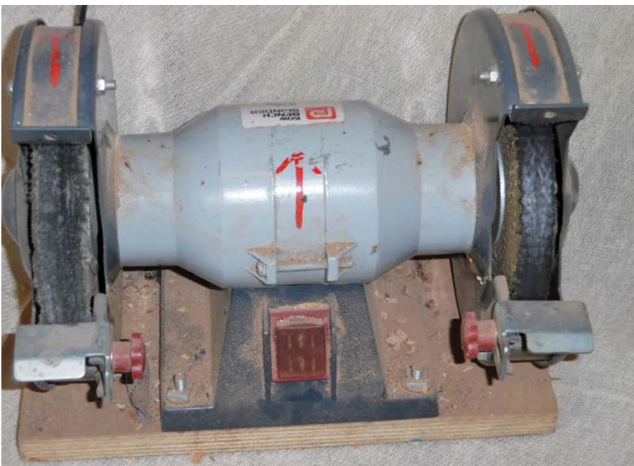
John's reverse turn grinder – one wheel is sisal while the other is sewn cotton – never fails to cause a stir at demos
