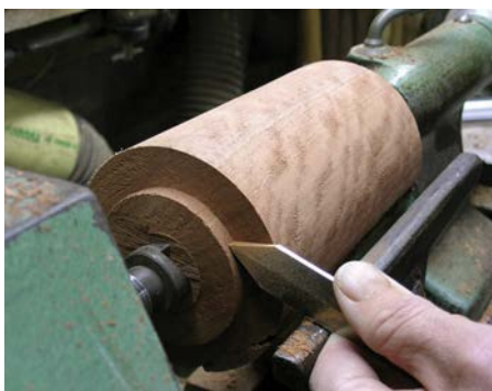
A tenon was cut so the form could be fitted to a scroll chuck
