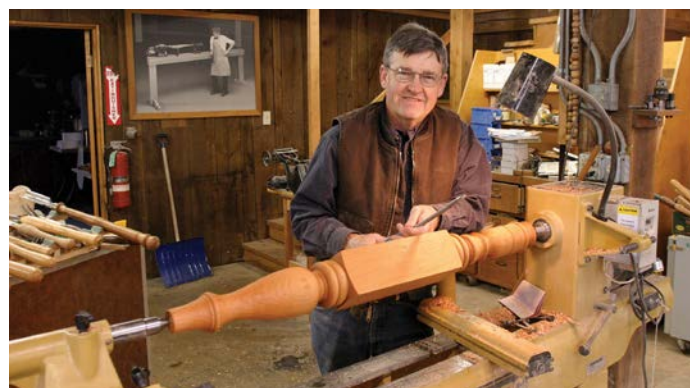
The bottom half of a finished post in my Powermatic. This is 'you are not allowed to make a mistake' turning that requires full concentration. I do not listen to music, want other people in the 'shop or to be tired. It is all about coves and beads and precise work
