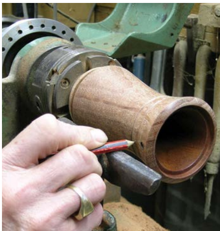
Using the indexing head of my lathe, spacing for 'buttons' were marked
