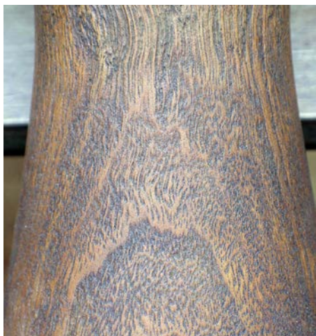
Colour was cut back with sand paper to highlight the exposed grain
