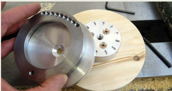
The Axminster chuck, showing its three engineered parts
