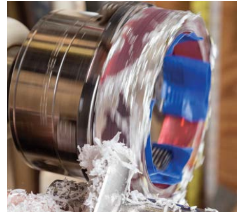
I never remove the homemade casting mould aluminium foil as it turns off easily. Note the tape on the jaws protecting the finished I.D
