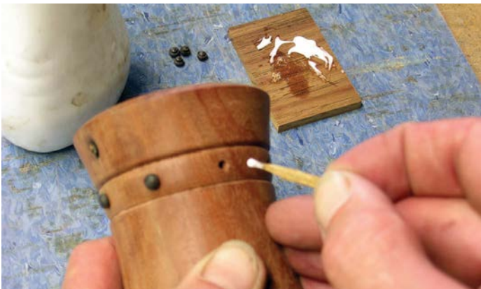
A sliver of veneer ensured just the right amount of glue was applied to fix each button into place
