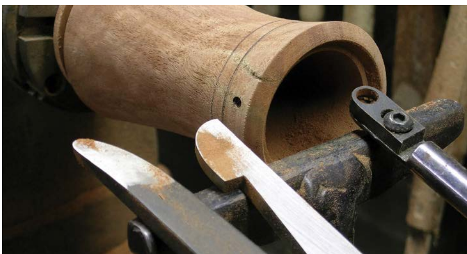
A series of tools was used to hollow the interior
