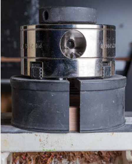
ABOVE: A tip to mounting your work flush to the jaw edges providing space behind. Lay the work and the jaws on the bed, then tighten
