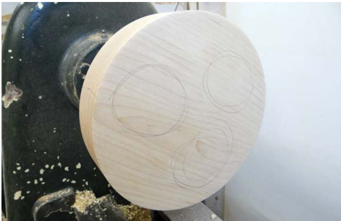
Rough circles sketched on the face of the blank
