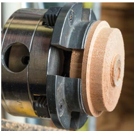
A jamb chuck turned at the moment to fit the occasion. Any scrap works, a shoulder is helpful, and tape adapts within reason
