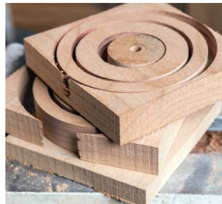
A trip to the bandsaw to separate the blanks at the desired blank widths in multiples at a time
