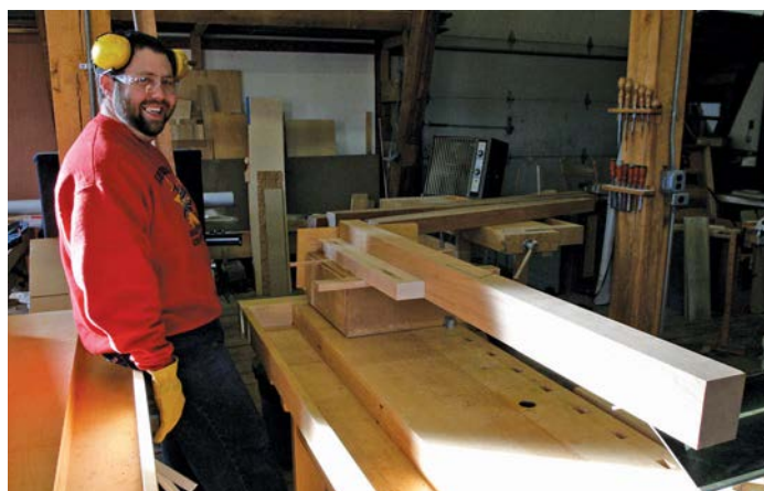
Patrick Brown with a router table and support he designed to cut the stub tenons on the posts for our beds
