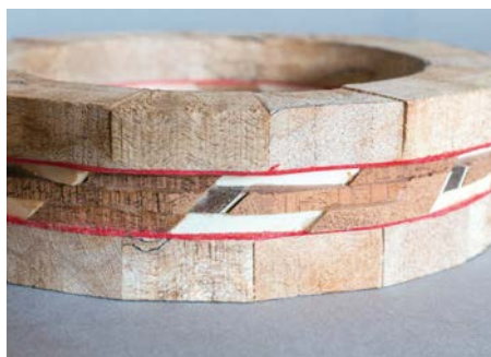
Segmented bracelet blanks taking advantage of the staggered seams. The artistic segmented blanks from my friend Nelson Cassinger
