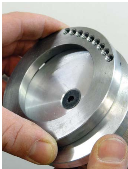
The adjustment on the outer ring of the Axminster chuck
