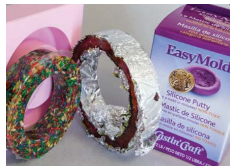
Cast blanks are easily done whether with a purchased mould, homemade mould from a kit or jerry rigged mould
