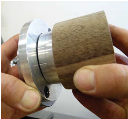
Adjusting the boss to the next position on the index
