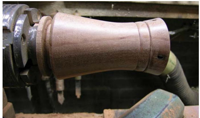
The exterior sanded and a couple of 'V' lines cut for a feature line
