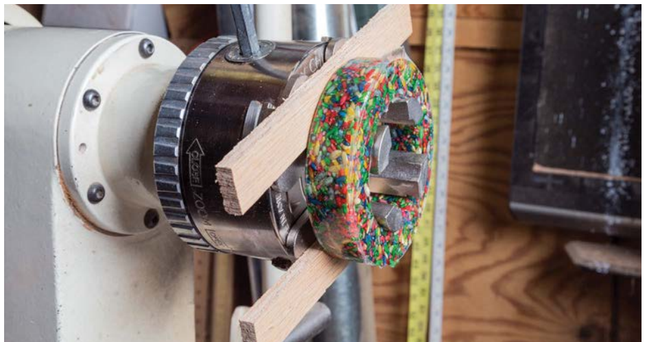
You can space your turning away from the back of the chuck by using equal sized shims as you tighten the jaws then remove shims
