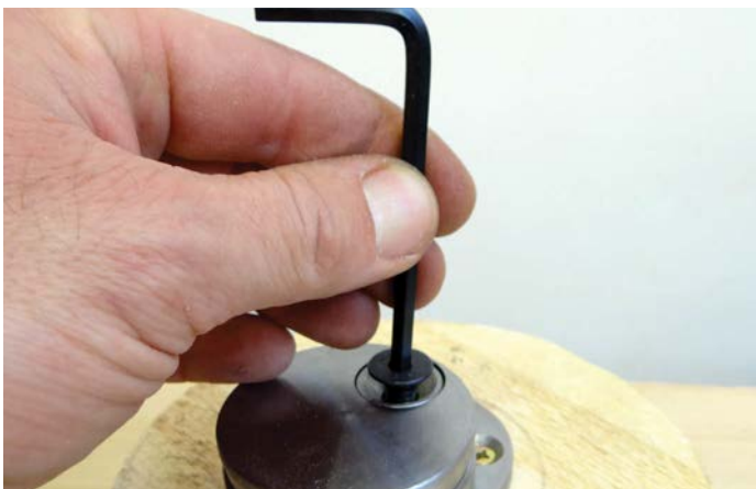
Once set, it is locked in place with a grub screw
