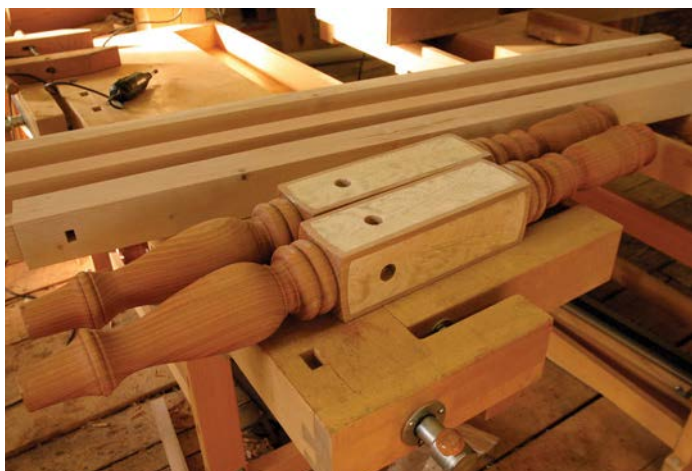
The foot posts were also inlaid after turning with crotch satinwood veneer
