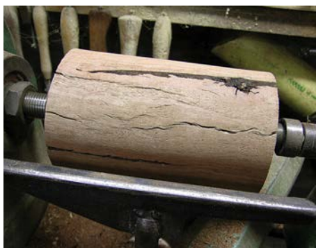
Voids needed stabilisation with CA glue
