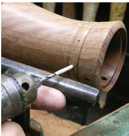
Masking tape ensured all holes were drilled to similar depths
