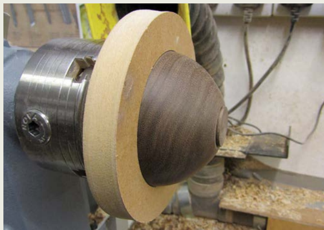
Held in jam chuck for sanding the base
