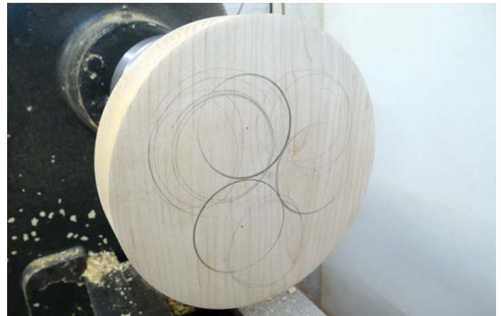
After adjusting the chuck these are the actual shapes possible
