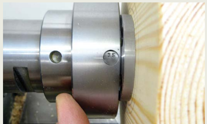
Position '35' is the largest offset available
