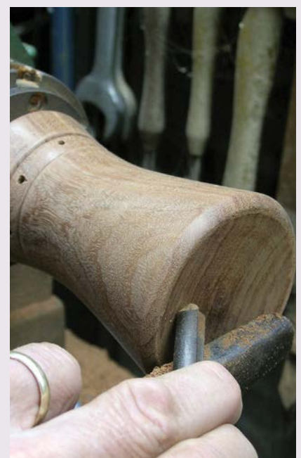
The base was cleaned up while the form was held on the chuck in its expansion mode
