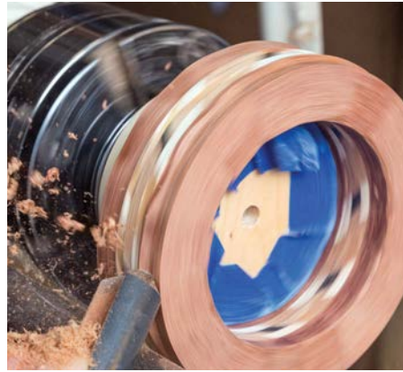
Regardless of your mount, chuck or jamb chuck, it is wise to always work towards the headstock
