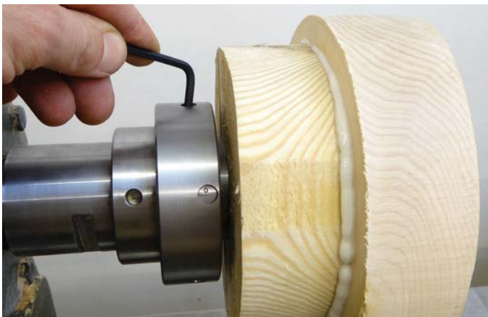
The chuck is adjusted from position '0', which is true centre to position '35'
