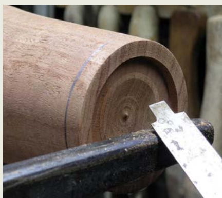
Using a 'granny tooth' scraper to create a recess for the lid to sit in
