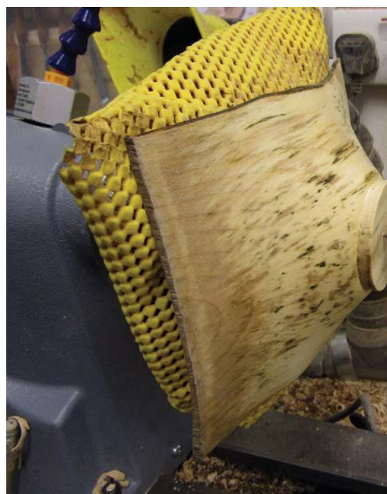
Bowl held for re-turning of the base
