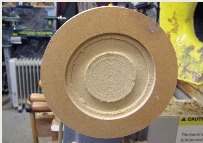
Jam chuck recess
