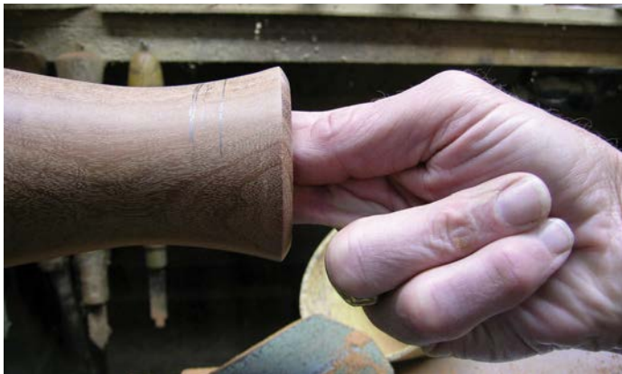
Don't hollow forms too far for fingers to fit into
