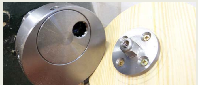
The chosen fixture, in this case the faceplate, fastens into the chuck body by a screw through the rear of the inner boss, seen in the chuck body. Notice the 12-sided hole which allows indexable rotation
