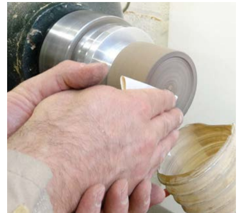
A light sand cleans up the pattern
