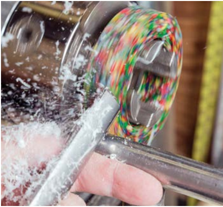
With the inside completed, you can now work the outer diameter of the bracelet to your liking
