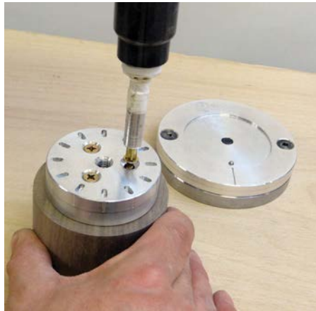
Fixing the piece of walnut to the faceplate attachment
