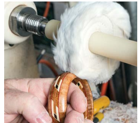
It is rare that any finish doesn't improve with some buffing. Proper speeds and feeds are important
