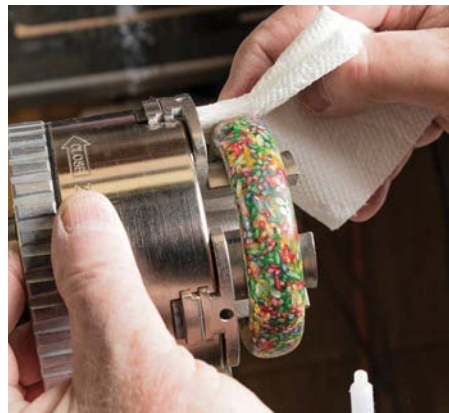
I even apply Ca finish to some of my resin cast parts. Here, the Ca seals the cut through and fractured rice grains
