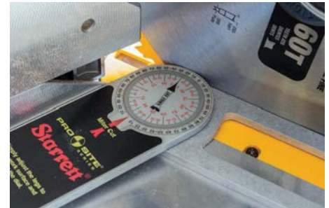
Insufficient resolution or accuracy. A tenth of a degree error times 16 cuts is a 1.6° problem
