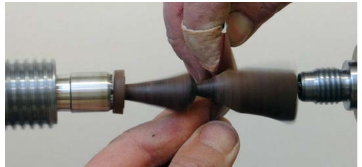
Sanding is done at each stage to minimise risk of breaking
