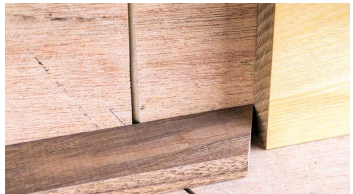
Make the initial angle cut to establish that. Flip the stock 180°, position at the stop and cut the segment
