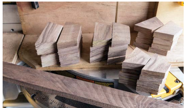
Once things are adjusted, cutting segments is quick work. Cut them all and save extra stock in case of errors later
