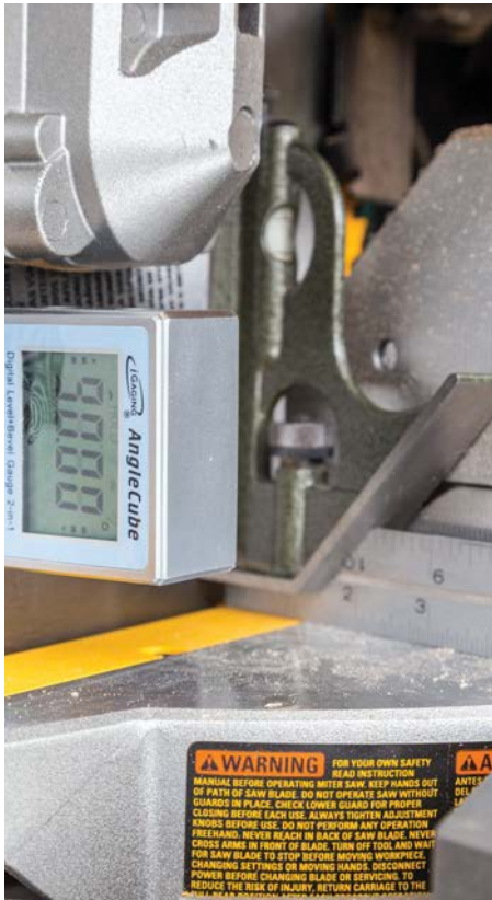
Whether using most modern electronics or an old-fashioned square, be certain you are cutting at 90°
