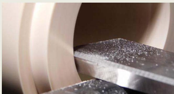
Clearance created with side grind
