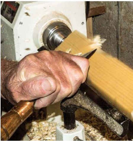
Using the convex bevel skew to make some incisions, followed by planing cuts
