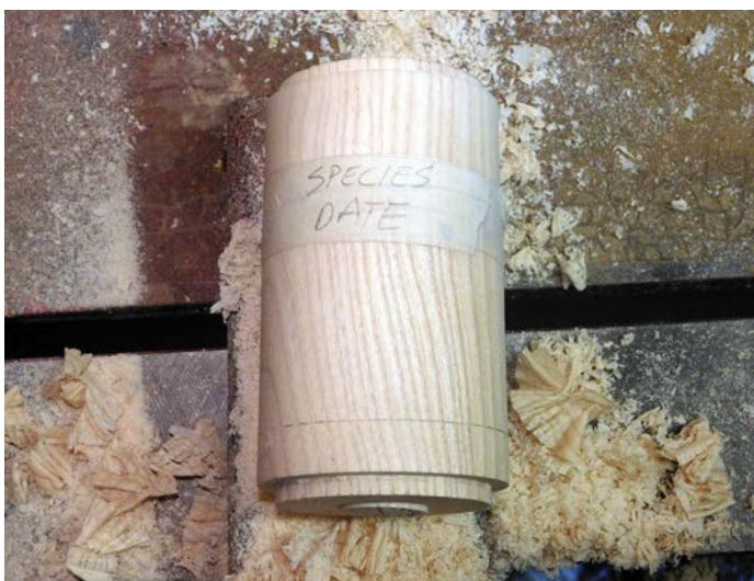
Roughed-out box taped up for drying out
