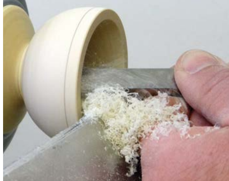
Refining the lid with my negative rake scraper
