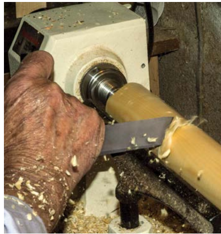
Refining the surface with planing cuts to create a smooth cylinder
