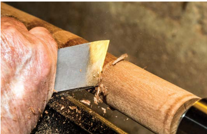
A closeup of the cutting edge making a planing cut on the timber
