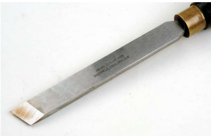
A standard ground skew chisel. The bevel is a flat grind rather than hollow grind in this instance
