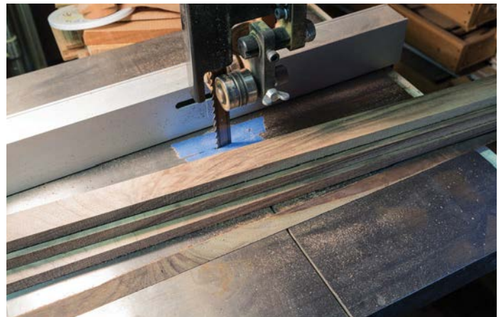
A 3 TPI resawing blade rips wonderfully but isn't always the best choice for cross cutting segments
