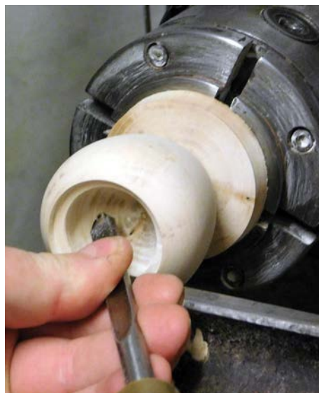
Cutting the wrong way
