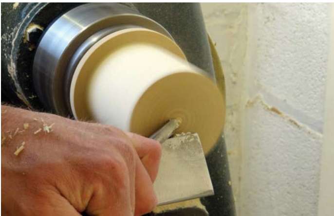
Using a jam chuck to finish the base
