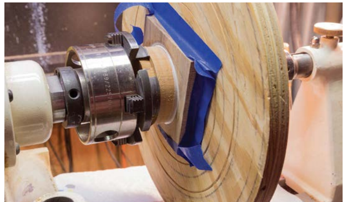
Waste block prepared, the base is glued and clamped in place using a home-made centring platten in the tail stock
