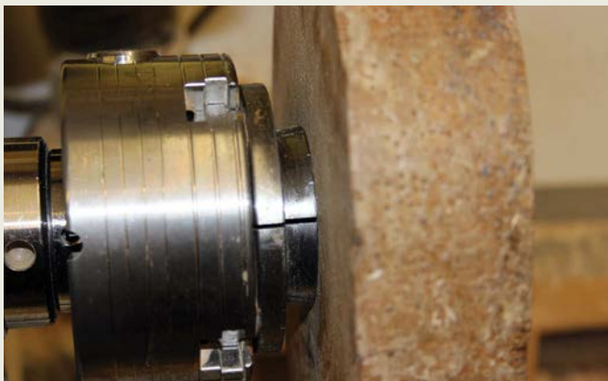
The blank securely mounted on the screw in the screw chuck
