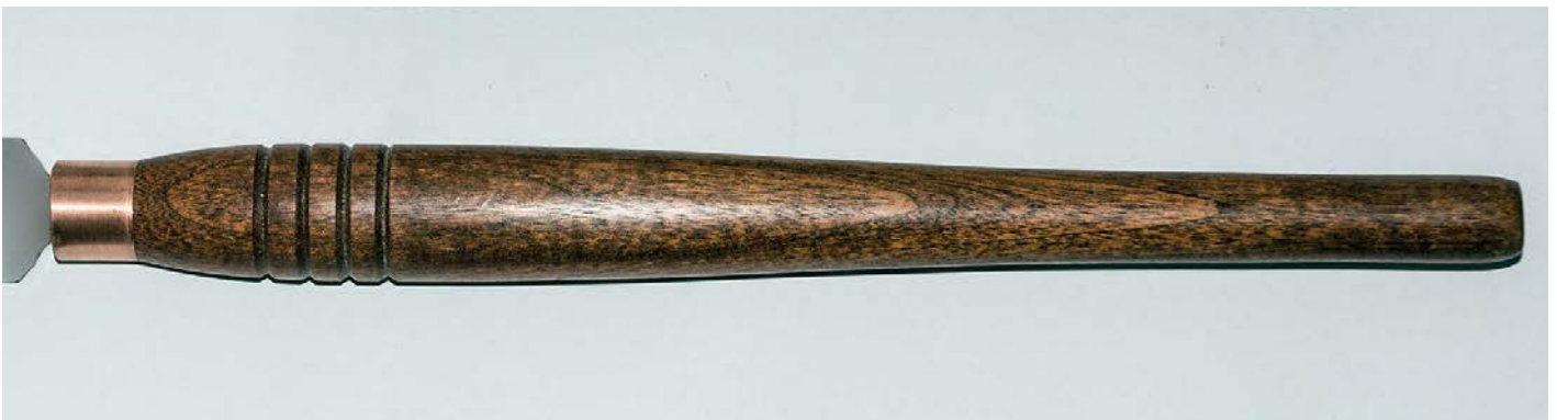
The finished handle fitted to the new convex ground skew blade ready for use
