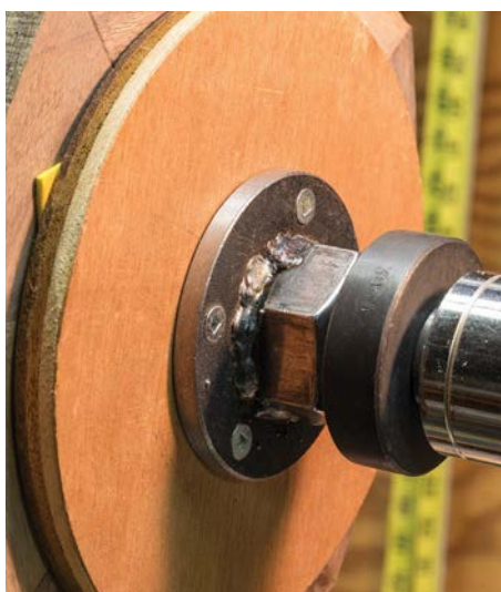
Like any bowl blank, there is value in using the tailstock for support until it needs to be removed
