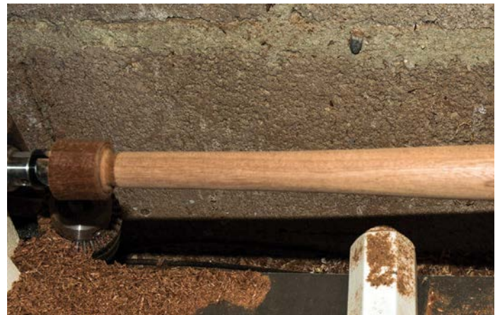
The partially shaped handle with a clean finish straight off the tool
