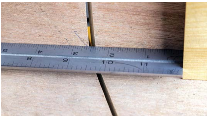
Setting the stop block accurately will help produce your planned results. Not the place for a tape measure
