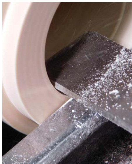
Using a scraper to cut with the grain
