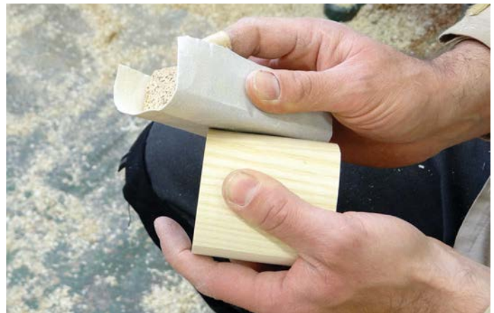
Hand sanding the sides with abrasive wrapped around a cork block
