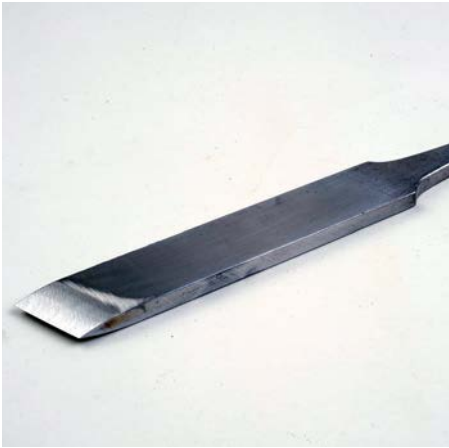
The bought HSS tool blade I ground with a convex bevel to replicate the grind I know of old
