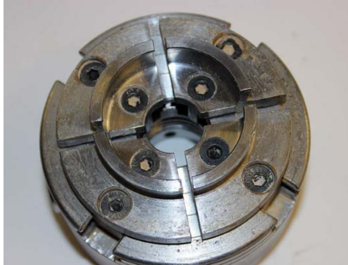
Standard jaws with dovetailed inner and outer jaw profile
