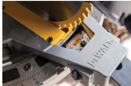
Adjustable and not accurate or repeatable enough. Don't rely on the detents on your equipment
