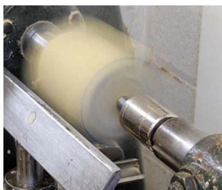
The marking out lines can clearly be seen on the spinning work
