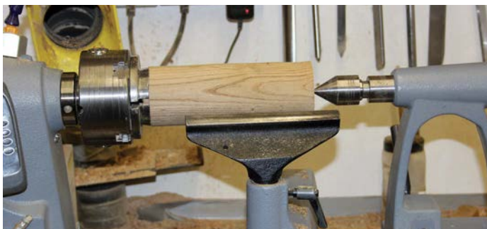
Tailstock used to support work held in a chuck
