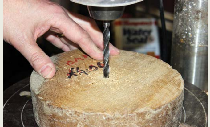
Drilling a correct size hole to suit the screw in the screw chuck
