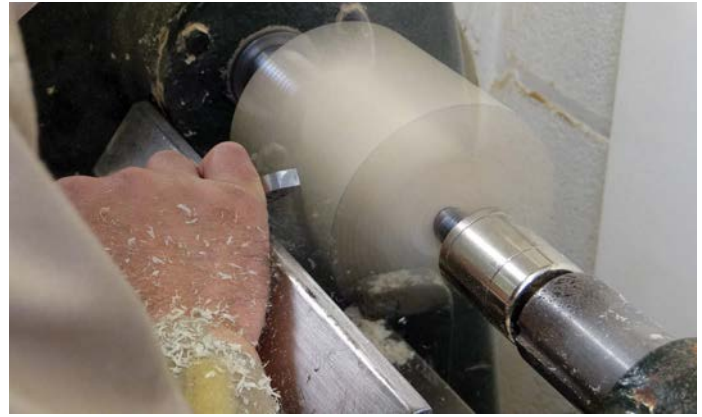
A careful skew cut leaves a clean and smooth surface
