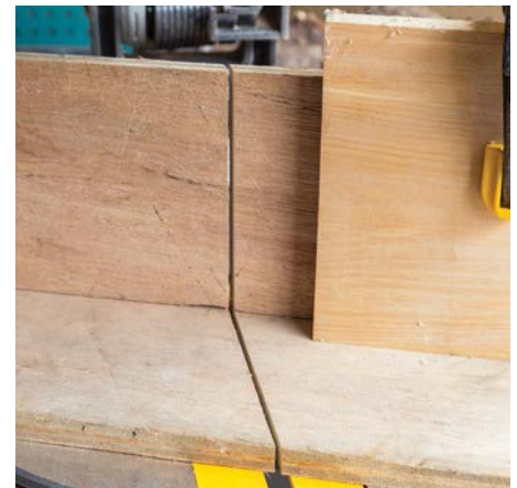
Sacrificial plywood stock is clamped on my mitre saw to create a zero clearance fence
