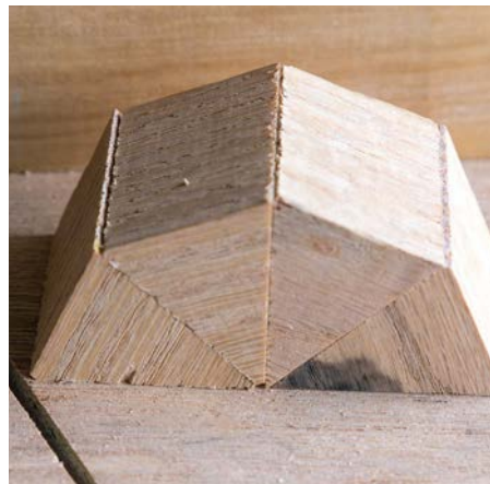
Cutting segments from scrap and checking the error stackup lets you tweak the angle setting until correct
