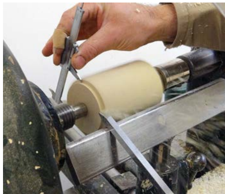
Cutting the spigot to hold the box on true centre ready for hollowing
