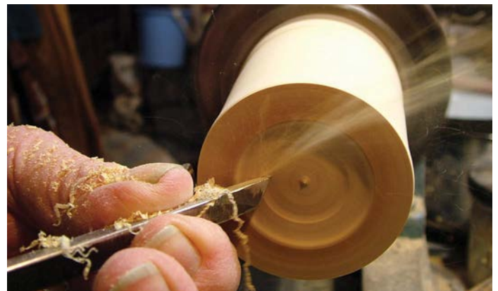
A round nosed scraper of triangular section used in 'sheer' scraping mode on boxwood end grain
