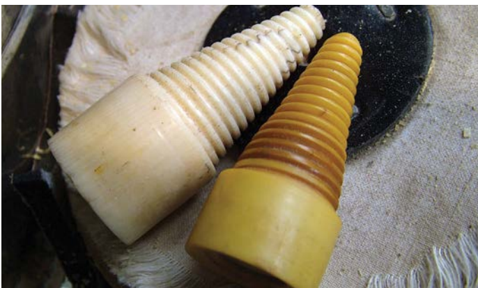
Homemade 'pig tails' for holding buffing mops. Most of Bill's pieces were buffed to a final finish
