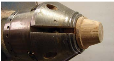
The jig held in a chuck awaiting the body of the mill
