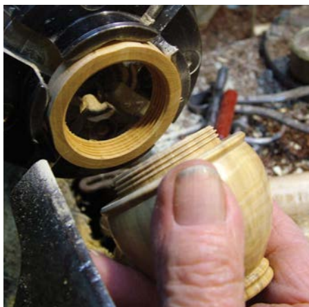
Bill often made threaded wooden chucks that were inserted in the lathe chuck to hold a threaded item. This allowed further work such as finishing the base
