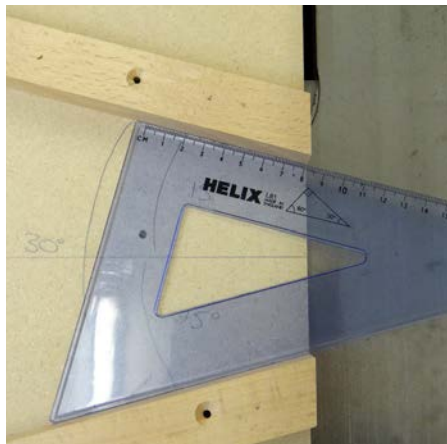
Checking the angles with a setting out triangle
