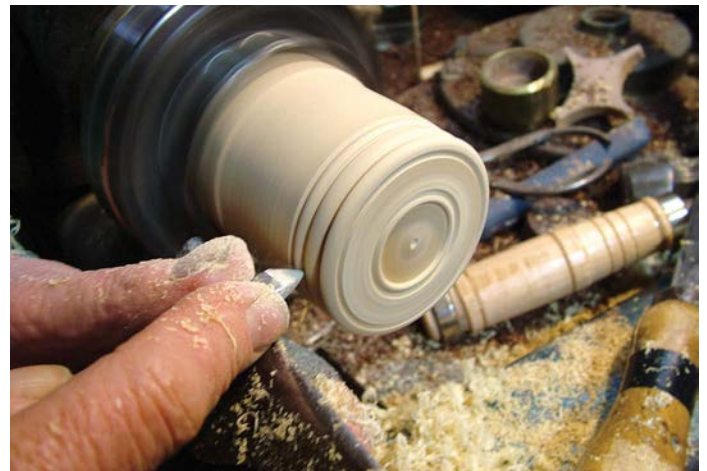
Using a homemade triangular scraper to create beads
