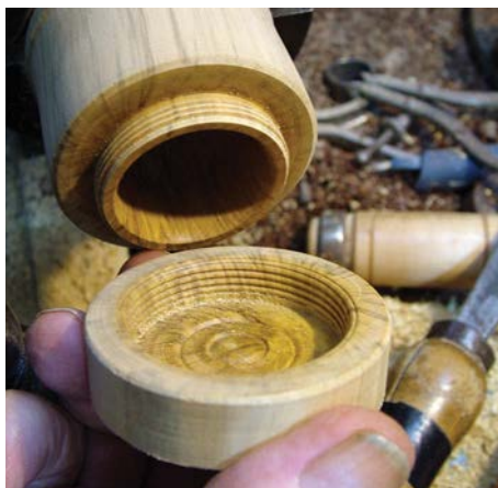
A completed male and female thread on a lidded screw-top box, turned from boxwood
