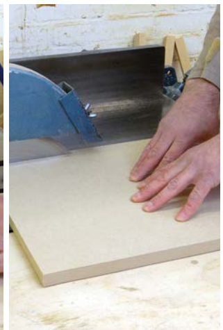
Trimming a parallel edge to the base board
