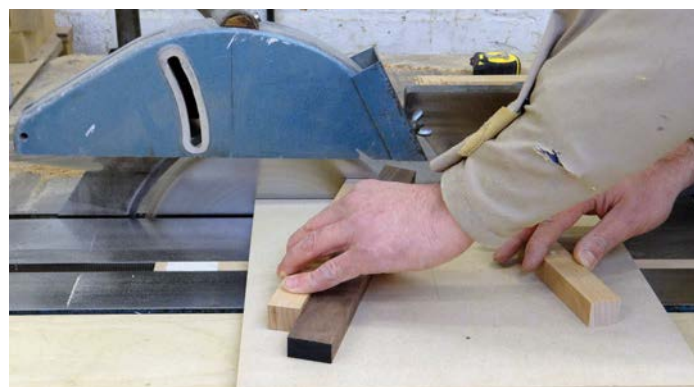
... alternating between the two positions to produce the correct angles on each segment
