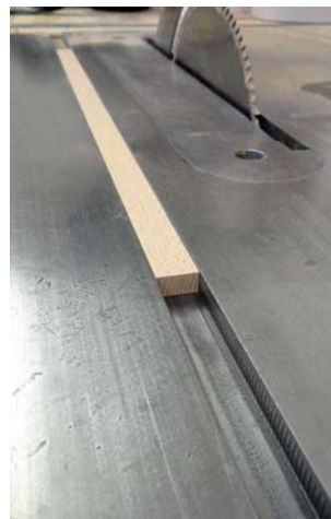
The first step for most jigs like this is to insert the beech strip in the slot on the saw bed
