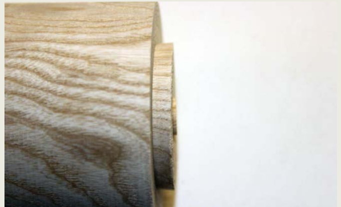
A parallel spigot is required when using micro-toothed jaws
