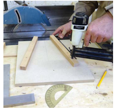
Fixing the battens to the base board using the sliding bevel as a guide
