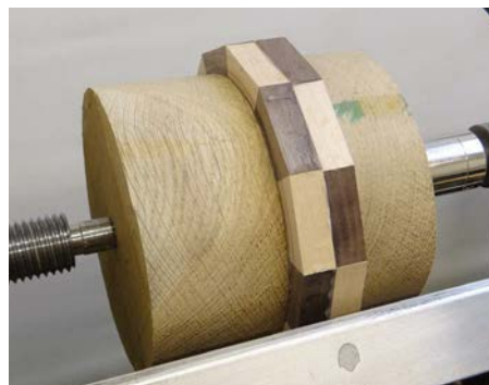
The blank held between centres to centre the rings
