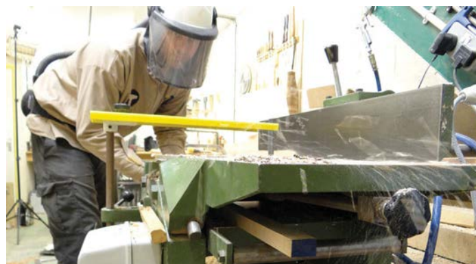
Preparing the timber with my planer-thicknesser
