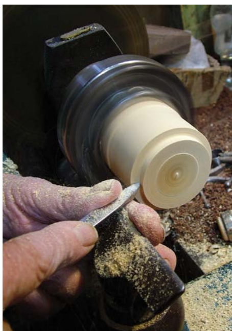
'Roughing out' using a homemade round nose scraper
