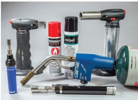
Depending on your size and dexterity needs, you can use anything from the propane torch to micro butane torches
