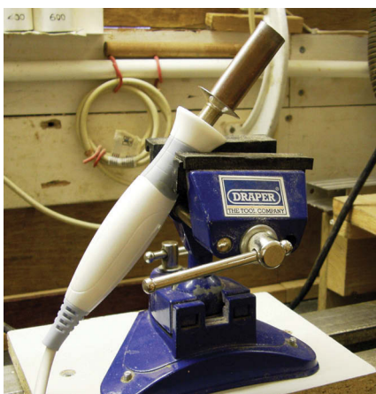
I sometimes slot a vice into the lathe bed
