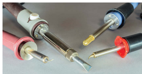
The modest woodburners lack heat recovery capability. The tips are also limited requiring your modifications
