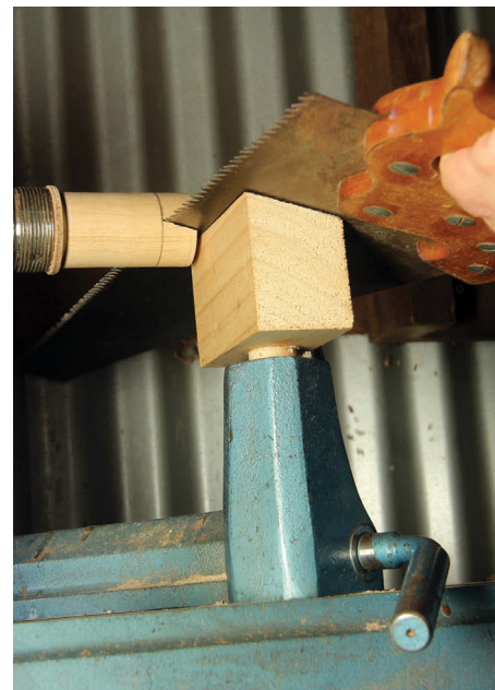
Sawing the slot in a bishop using a sloping jig that locks into the lathe banjo
