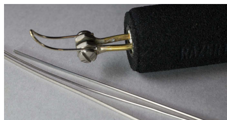
There are handles available allowing you to create your own tips from nichrome wire
