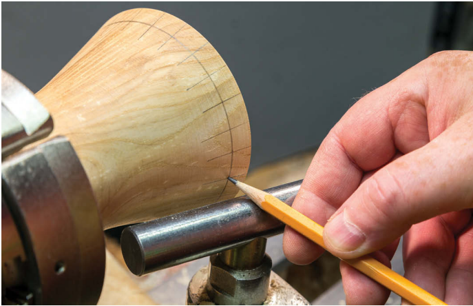
A blunted, soft lead pencil along with your indexing head will help with marking out pattern spacing
