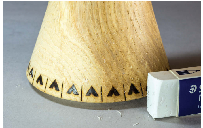
A good artist's eraser can remove layout lines provided you haven't indented the wood fibres
