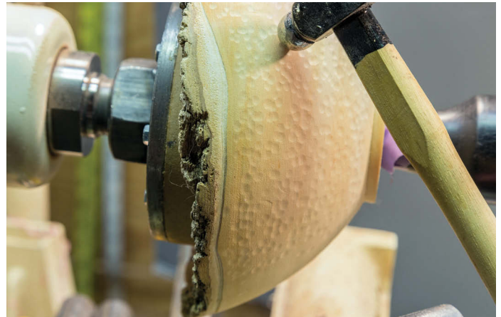
A simple ball pein hammer can be used to create that 'hand hammered' texture like metalwork
