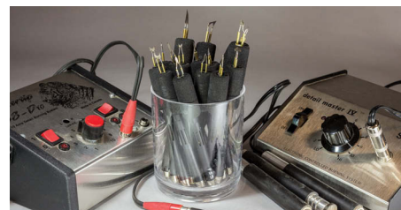
The higher-cost units feature extensive tip selections, variable temperature and fast heat recovery
