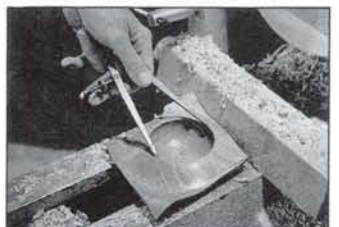
FIG. 27 The dividers are used to measure the diameter of the bowl in preparation for making the lid of the container. The waste pine can be removed from the base of the container before you proceed. If you wish to see the profile of the edges. Don't forget to add \frac{1}{8} th of a turn on dividers.
