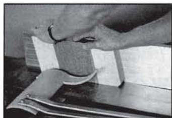
FIG. 3 Mark out container section, one for lid and one for base and label in pairs. Cut along line with band saw to minimise waste. The angle selected can be adjusted to suit individual requirements. It depends on the shape of the container.
