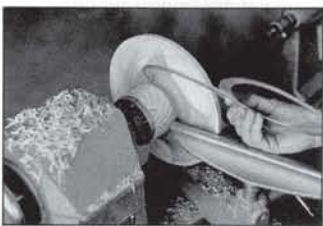
FIG. 16 Figure eight calipers are necessary to measure the thickness from the inside of the bowl to the outside of the bowl. The area is too far away to be measured with your fingers.
