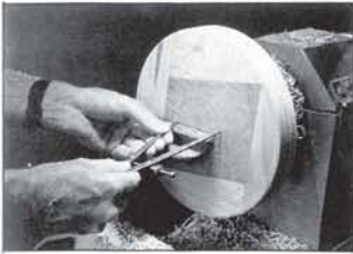
FIG. 28 Mark diameter on inside of container lid.
