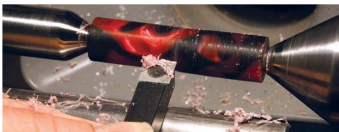
Using a TCT-tipped tool
