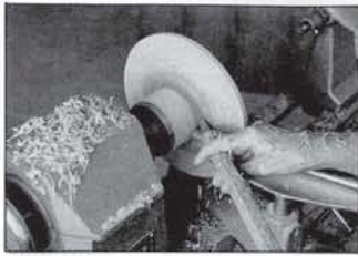
FIG. 15 Using a bar tool made from a 8mm \frac{5}{16} " tool steel bit fitting into a hexagonal bar with grub screws, remove waste from back of container (that is the base of the container). The thickness will be determined by fingers and range from 3mm x 5mm \frac{1}{8} " to \frac{3}{16} ".
