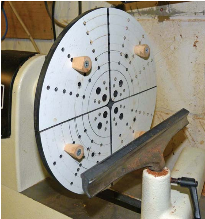
Chris' latest homemade jig is a reversing Cole-type backplate, which enables him to clean up the bottoms of bowls, etc.
