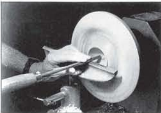
FIG. 30 Cut out shape of lid with 10mm \frac{3}{8} " bowl gouge spinning at 1200 rpm.
