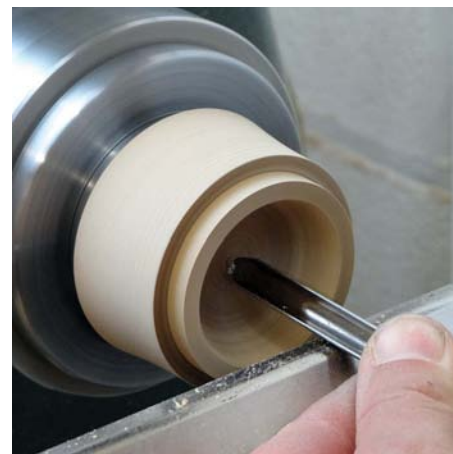
Removal is simply a case of cutting dead on centre with the gouge or scraper
