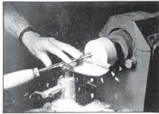
FIG. 33 Excess material in the carrier should be cut with a 10mm \frac{3}{8} " bowl gouge inside the divider line. When marking the carrier, this time remember to measure the step of the lid and close dividers by \frac{1}{8} th of a turn.
