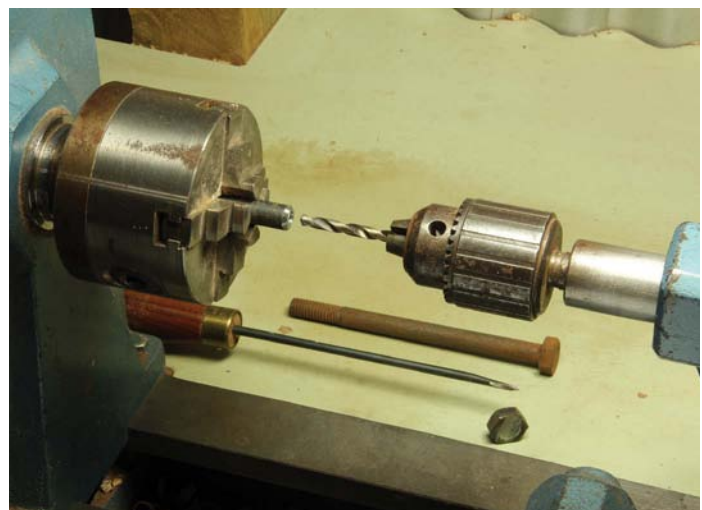
Boring a shaft cut from a bolt. After inserting the tip, a crisp hammer tap on the tip end of the shaft locks the tip in
