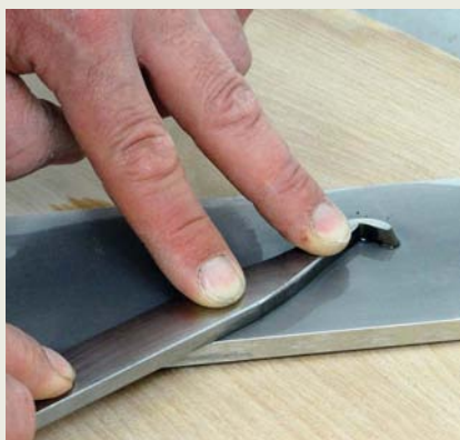
To sharpen my scrapers, I polish the top surface on a diamond plate
