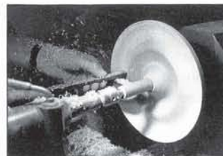
FIG. 39 Scrape the top surface and refine the line. Always scrape downhill with the dowel support in revolving centre. Do not remove dowel until you are ready to finalise shape of centre.
