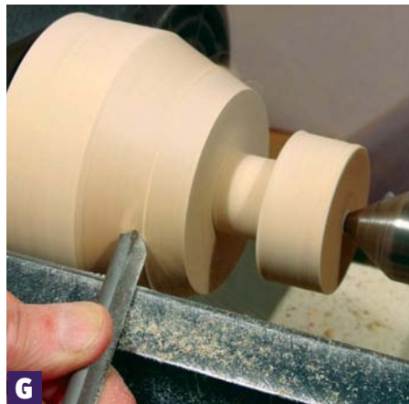
G Turning the sloping side. Note that there is plenty of 'waste' wood close to the tailstock
