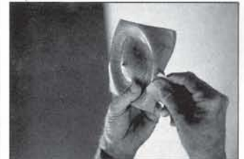
FIG. 38 Use sandpaper on edges and corners to remove excessive sharpness.
