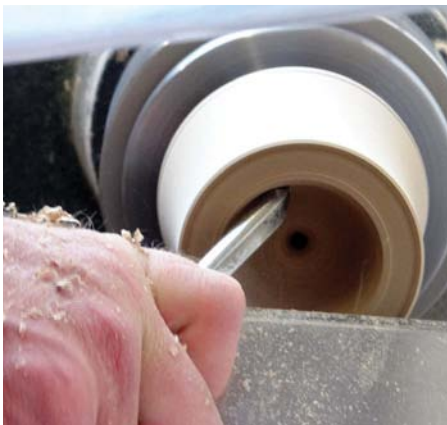
The 'Raffan' hollowing cut
