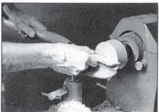
FIG. 19 Alternative method to remove container from waste block is the use of a tenon saw or combine both parting tool then saw. THE LATHE MUST NOT BE GOING WHEN USING THE SAW.
