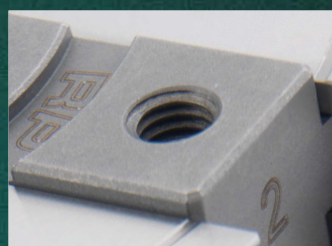
Heavy Duty Jaw Slides The improved and enlarged jaw slides give unsurpassed holding power and load bearing ability. They are made from high tensile steel, reinforced with nickel and copper and heat-treated to ensure superior strength.
