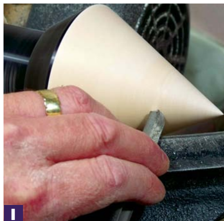
I The sloping side of the cone is turned to a point
