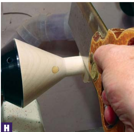
H The excess wood is sawn off
