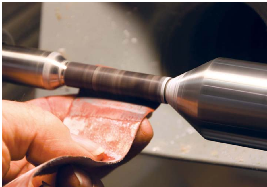
Wet sanding keeps the blank cool
