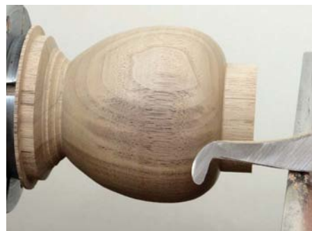
You can see how the cranked scraper will easily reach parts that straight tools can't
