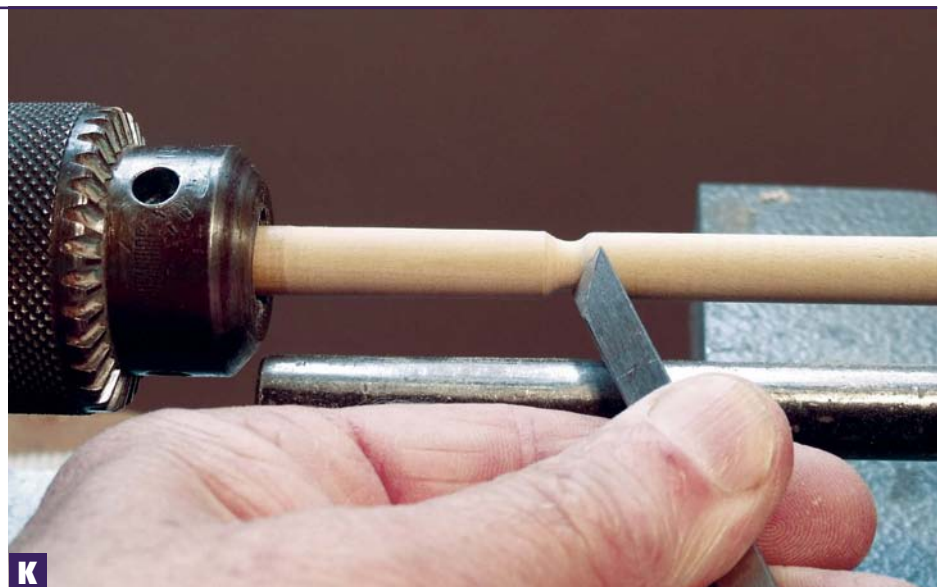
The cove in the spindle is turned out using a skew chisel
