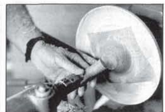
FIG. 24 Use of a wooden dowel with end covered with leather to protect base of container. This stays in position until you are ready to refine bottom of base.
