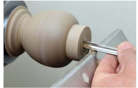
Drilling with the spindle gouge
