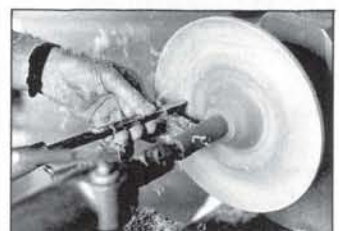
FIG. 25 With 12mm \frac{1}{2} " scraper refine the shape of the container on the outer edge while dowel keeps container on carrier. Again scrape downhill spin at 2000 rpm. Do not go any faster as the pine can break off by the force of spinning too fast.
