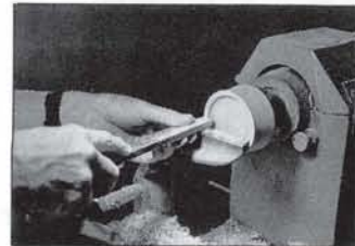
FIG. 21 Testing for flatness with edge of tool.
