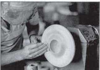
FIG. 17 Sand top surface and bowl of container with 150, 180, 220, 240, 280, 320, 360, 400, 500 grit. I use linen-backed J weight flexible resin bond material up to 240 grit followed by A weight open coat free cut paper backed to 400 and wet and dry to 500.
