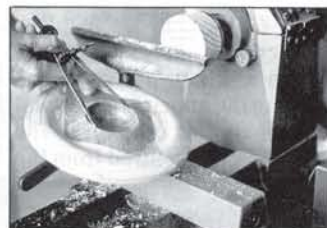
FIG. 21 Testing for flatness with edge of tool.
