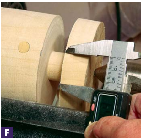
F Measuring the 25mm tenon. Note the dowel filling the 'stick' hole
