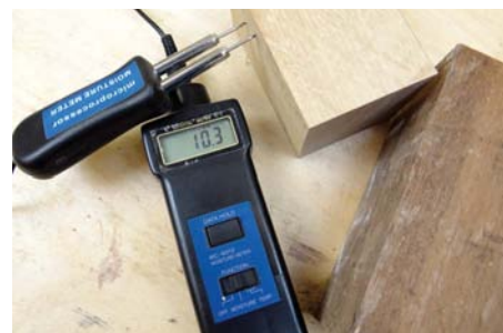
Using my digital moisture meter shows that the walnut ( Juglans nigra ) is 8.6% and the oak ( Quercus alba ) is 10.3% – both are suitable for box-making
