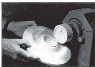
FIG. 34 With the step tool, remove the excess creating a right angle cut 5mm \frac{3}{16} ".
