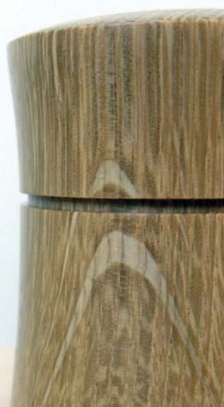
The box is not seated correctly here, so the chances of it staying there as you work the base are slim at best, even if the fit is tight
