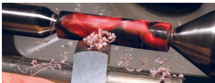
Using a Robert Sorby hardwood scraper – negative-rake scraper
