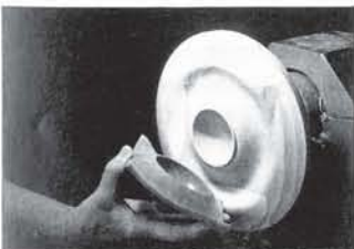
FIG. 32 Check fitting of base to lid. This should not be a tight fit, as you do not want to lift up the base when you pick up the lid. Before removing the lid from the waste block, shape the lid as we did before on the base section with the bar tool.
