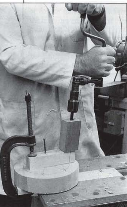
12 Boring jig in use. Note the G-clamp and depth stop.
