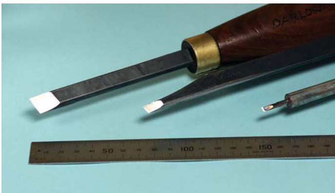
Left, a 12mm wide skew; centre, a 6mm wide skew ground from a 12mm wide skew; right, a 3mm wide skew tip ground from the stub of a HSS twist drill and mounted in a 9.5mm diameter shaft cut from a bolt
