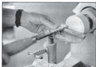
FIG. 23 Cut step 5mm \frac{3}{16} " deep to divider line and check for fit. If slightly loose chalk can be applied to step of carrier. You can even wet the step with saliva. Another method is to use sorbent tissues which are very soft and follow the contour of the step. If you have to fold the tissue more than four times cut a new step.
