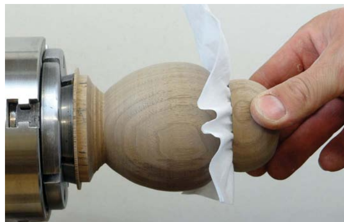
If you find the lid is not quite tight enough to rework it safely, a piece of paper towel can give that bit of extra grip
