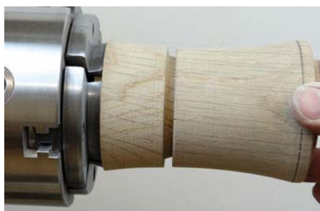
The first step is to cut a taper; this is slightly over emphasised for clarity
