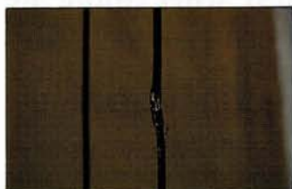
Driving belt ends joined with 'hook and eye'. Original gut belt
