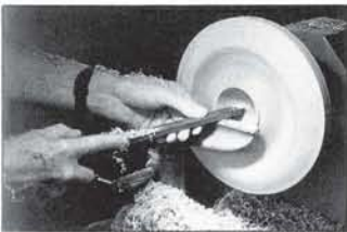
FIG. 31 Use half round nose scraper to refine line at 2000 rpm. Cut step at this time with step tool so as to get a better cut. (See illustration 34 for grinding of step tool profile.)
