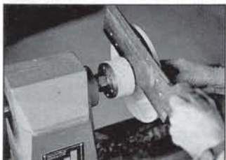
FIG. 19 Alternative method to remove container from waste block is the use of a tenon saw or combine both parting tool then saw. THE LATHE MUST NOT BE GOING WHEN USING THE SAW.
