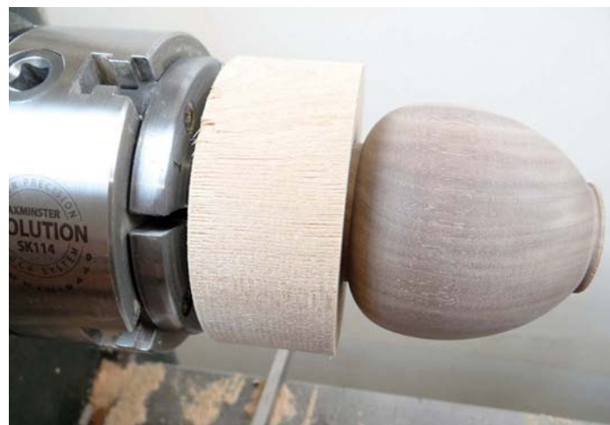
The box is not seated correctly here, so the chances of it staying there as you work the base are slim at best, even if the fit is tight
