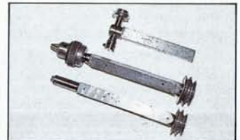
Top: Original drilling instrument. Middle: Contemporary drilling instrument with Jacob chuck. Bottom: Vertical cutting frame.
