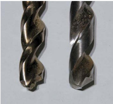
Bullet tipped – left – and jobber – right – drill bits
