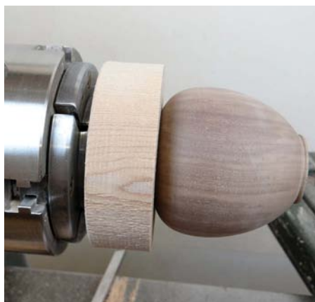
The box is now correctly seated and so, in combination with a tight fit, will stay in the jam chuck while you rework the base
