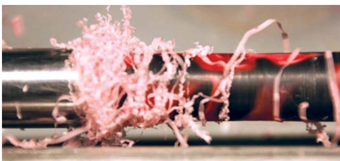
Swarf will begin to accumulate once the blank is turned to a cylinder
