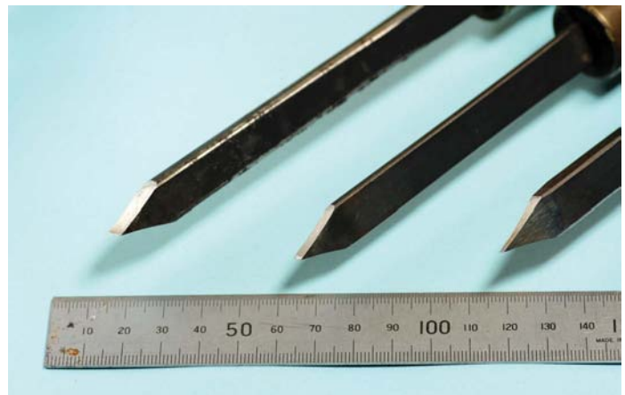
Parting tools, from left to right: 6mm wide, 3mm wide, 1.5mm wide ground from a 6mm wide parting tool
