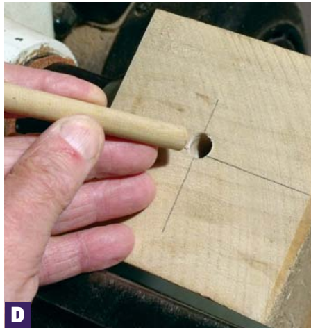
D A temporary, but tight, dowel is fitted into the 'sword' hole preventing edges breaking out while being turned
