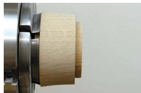
Removing material towards the shoulder and creating a slight dome gives you the best chance of a tight fitting lid
