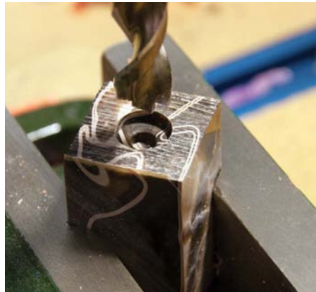
Bullet tip bit drills its own pilot hole
