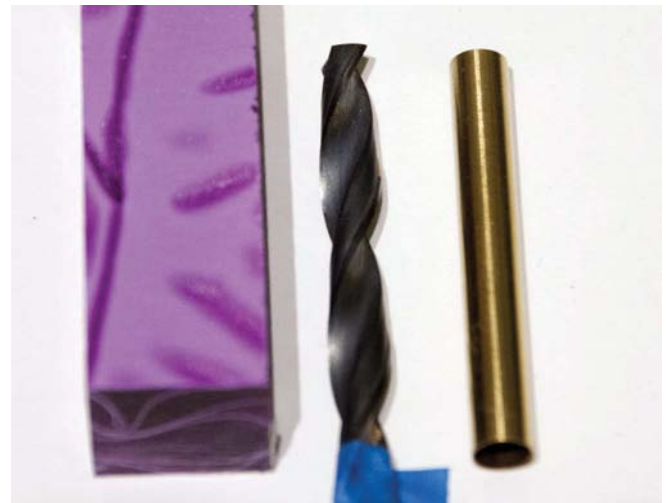
Drill bit and blank prepared to drill short of breakthrough
