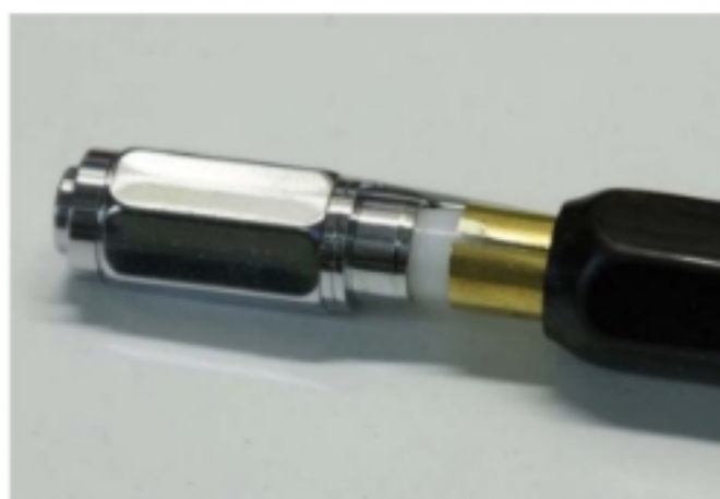
The slit tube slips over the plastic parts but is still able to contact the end of the metal components
