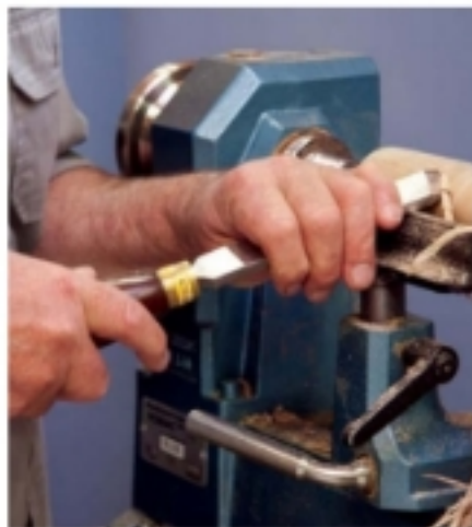
Good working stance: hold the tool near the ferrule to avoid cramping your arm and keep the handle in close to your body. Use your whole body – not just your arms – to move the tool
