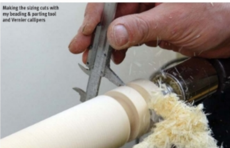
Having a good line of sight and sharp tools when making sizing cuts will help to ensure details stay where you want them
