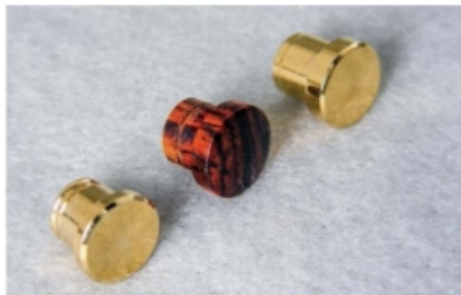
Because the wooden end cap can't be a hard press fit, it needs to be adhesively bonded but is susceptible to squeeze out
