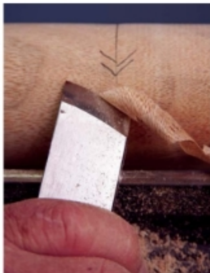
Ideal cutting angle: hold a skew chisel or gouge so that the part of the edge that is cutting is about 45° to the oncoming wood
