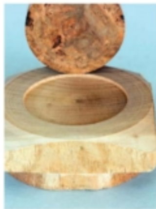
While the burl may not vary in expansion rates based on orientation, any grained substrate will move dramatically
