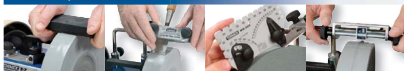
Stone Grader grades the stone for a 1000 grit finish
