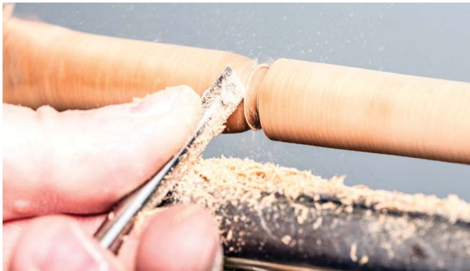
A round skew can be used exactly as any other skew chisel. The size and shape lends itself to smaller detailing and bead work
