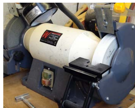
My sharpening setup, a 200mm slow-running grinder with a 120 grit white wheel and an adjustable platform fitted
