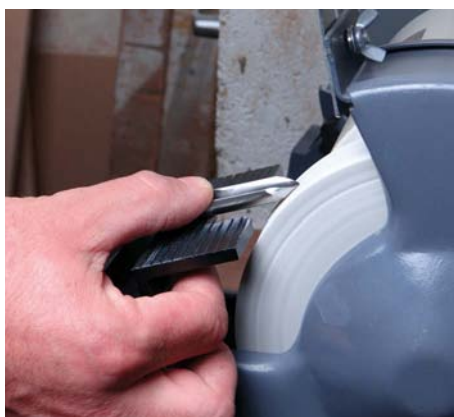
My method for sharpening spindle gouges is to start at the tip ...
