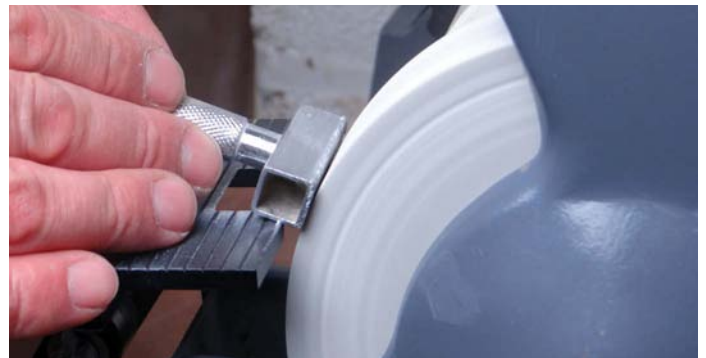
Dressing the wheel with a diamond T-bar dresser
