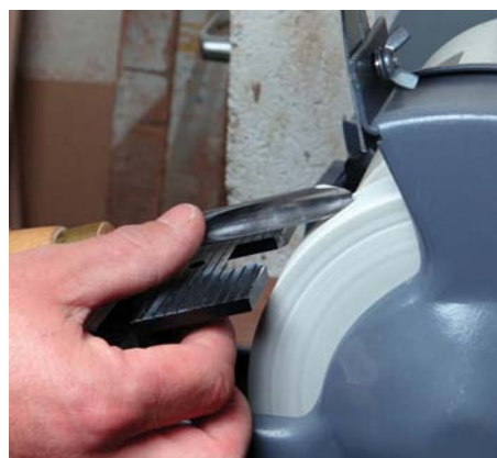
... then roll the tool as I ride it up the stone
