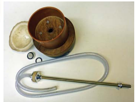
Andrew's latest homemade vacuum chuck with a bought bearing set
