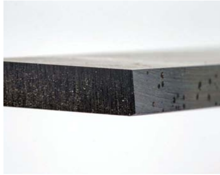
Any tool edge that doesn't create the wood contact edge is a candidate for softening
