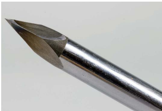
I favour mine hollow ground rather than the more common commercially available flat ground because I can use the honing method of sharpening more easily
