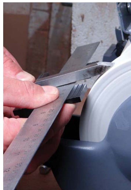
My method for sharpening my beading & parting tool to a longer angle without adjusting my platform
