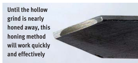
Skews, bedans, parting tools and any other skew-like edge that is hollow ground lends itself to sharpening via honing
