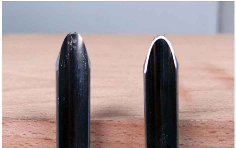
Touching the top of the gouge to the grinding wheel shows you a perfect profile that the tool 'wants' to be
