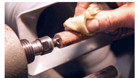
Cleaning away sanding dust between grits prevents scratching from any remaining coarser grit particles
