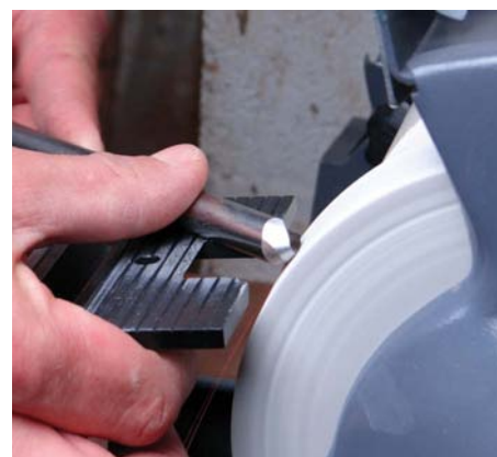
Sharpening my bowl gouge, keeping it flat on the platform and rolling while I swing the handle to one side
