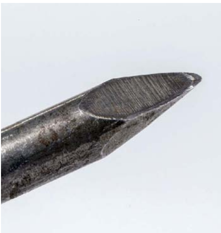
Not certain of the lineage or name but this detailer is hollow ground across the face allowing for diamond hone touch up
