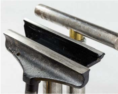
Other than the hardened edge rest in the centre, tools will slide easier on soft rests once the tool edges are broken
