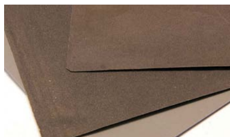
Silicone carbide abrasives are useful for wet sanding man-made materials
