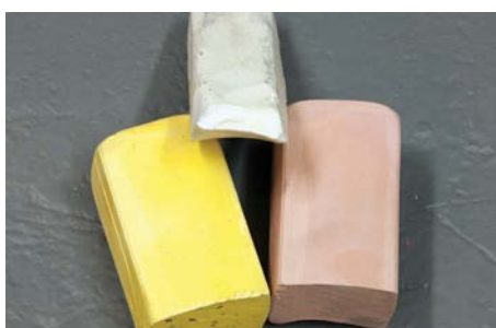
Compounds for buffing wheels come in a variety of grades from coarse to very fine. A separate buffing wheel should be used for each grade
