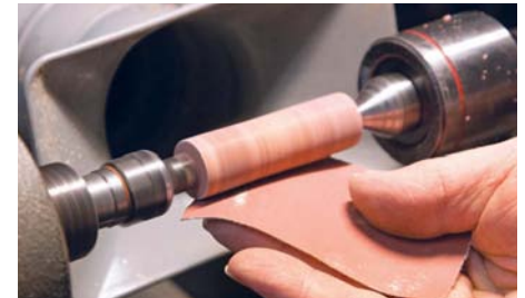
Sanding with the lathe running should be followed by hand sanding along the grain
