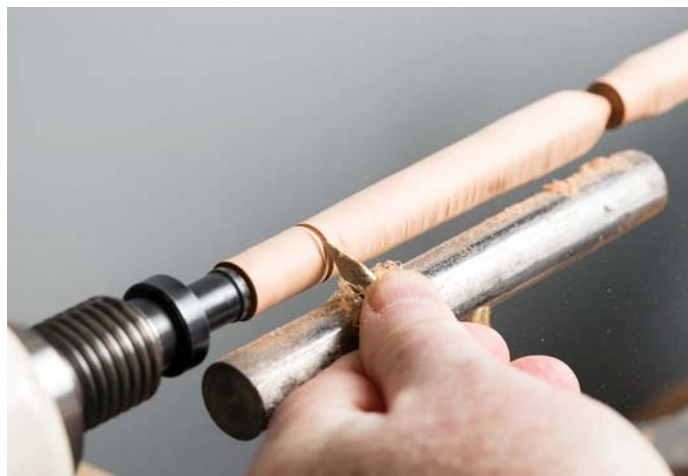
The tri-point tool is not only capable of V cuts and corner detailing but also rolling beads. Keeping the point clear is critical
