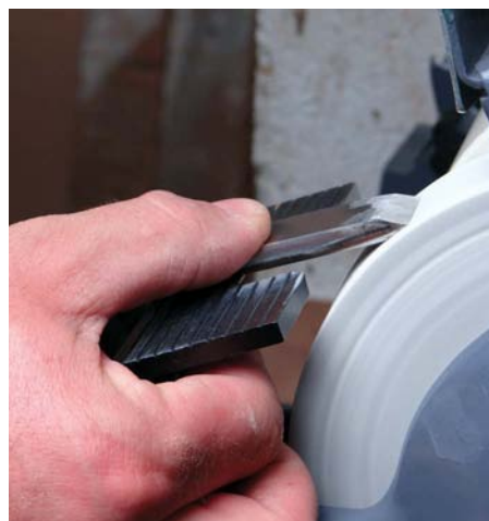
Skews and parting tools are simple to sharpen, just by laying them on the platform and gently moving them across the stone
