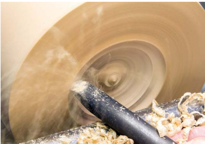
Don't start your deep hollowing learning process working through small openings. Begin practising in the wide open to learn tool control
