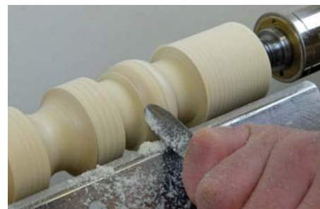
Rolling a bead with a gouge. Notice the shaving is coming from the sweet spot
