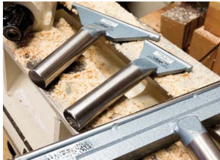
Forces on a toolrest when hollowing demand sturdily built equipment. Be certain your toolrests are up to the task
