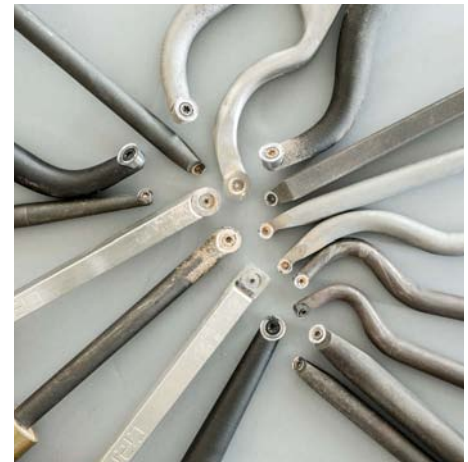
Just a few of the available carbide cutter hollowing tools for hand-held use. All feature replaceable cutters when the existing has been rotated until spent
