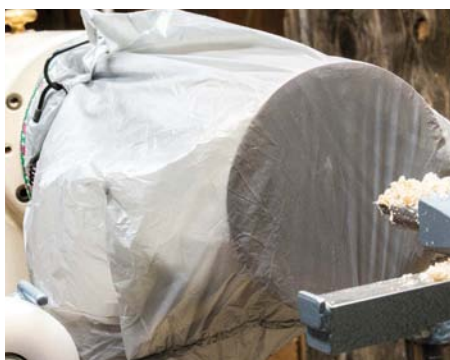
When turning green wood, deep hollowing or not, keeping it sealed and wet is important when leaving even for the briefest time
