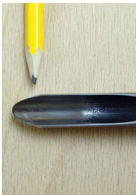
You can just see that the top of the wing, how the cutting edge is slightly rolled within the diameter of the bar, which I have found prevents some accidental catches in confined areas
