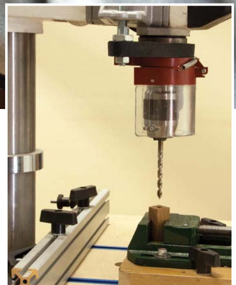
A pillar drill and vice will ensure accurate drilling
