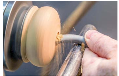
Do a bit of outside shaping to help with your hollowing but leave plenty of strength for the workholding until later. It is easily cut away after hollowing
