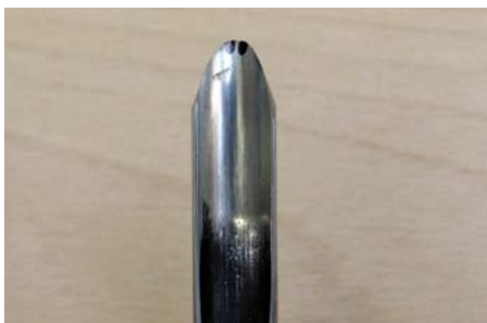
The sweet spots marked on the gouge, either side of the centre point
