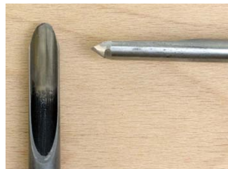
This shows the profile and grind on my spindle gouges
