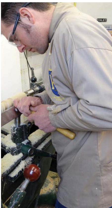
My stance at the lathe. Notice the tool handle is by my side, as are my arms, which means it is my body movement that creates the shapes in the wood
