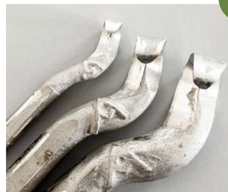
Superb at hollowing end grain green wood, the Martel hook tools are not for newcomers
