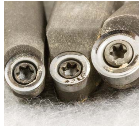
Most modern carbide cutter tools support the cutter as completely as possible. The cutter is exposed only in the areas of potential use
