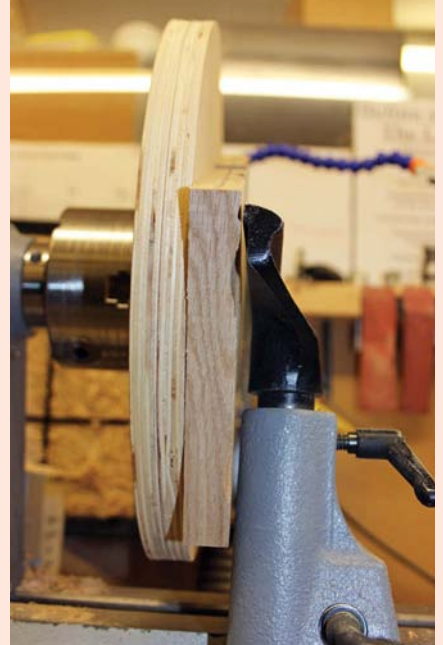
Always make sure your blank is mounted securely
