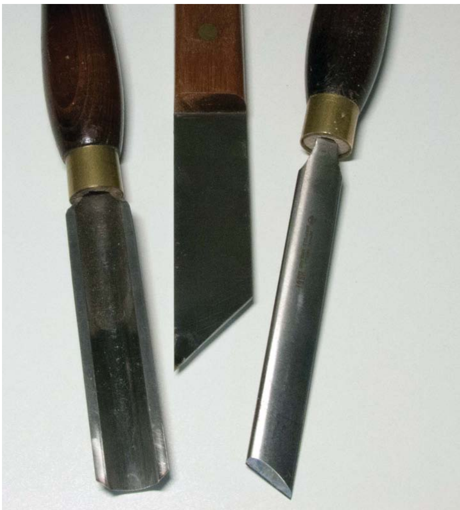
Only basic turning tools are needed to begin with. I use full-size tools but some turners, especially those with smaller lathes, prefer to use smaller tools
