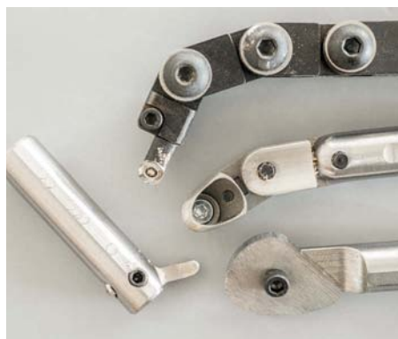
The mainstays of the hollowing tools for both the hand-held and the hollowing bar systems
