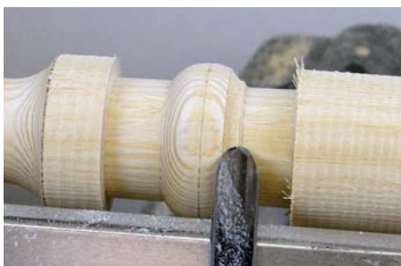
Using the wrong part of the edge will result in a large catch
