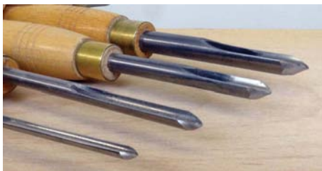
My standard round bar spindle gouges are all Ashley Isles in sizes of 3mm, 6mm, 10mm and 12mm – all have the same profile and grind
