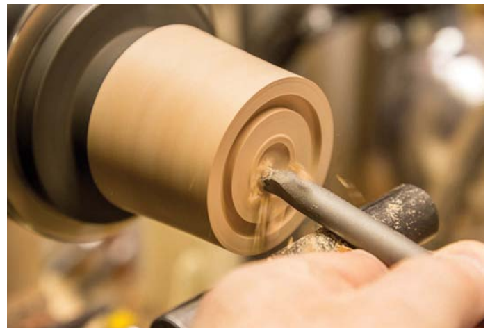
Hollowing lidded boxes is great practice. Notice the desired finished wall surface to work towards
