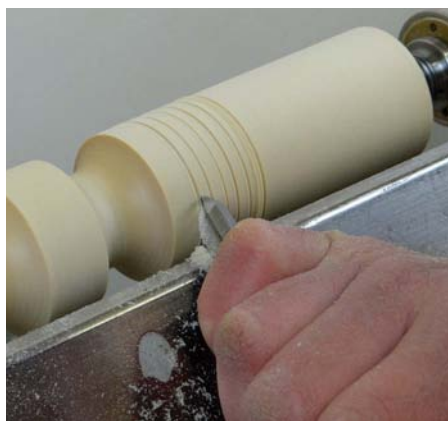
Practising the entry cut by making a series of lines with the tip of the tool
