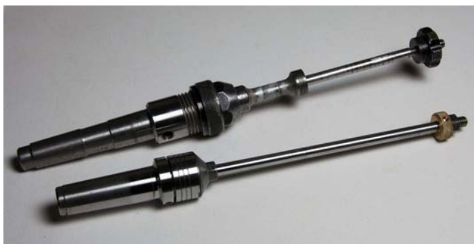
Mandrels come in many different forms but my preference is for colletted adjustable types such as these
