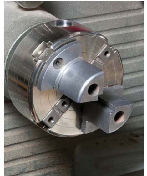
Dedicated pen jaws can be used to hold the blank for drilling on the lathe
