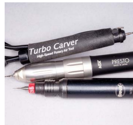
A machine tool grade die grinder and my two favourite high-speed tools. The die grinder is used with thicker materials and the high-speed tools with shell and thin stock
