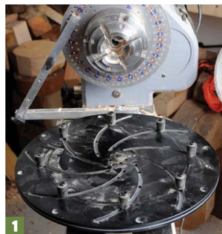
1 Fluting of any sort requires that the work be held in such a way that it is stable while you cut it
