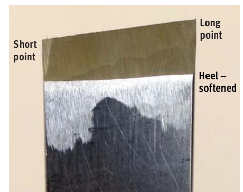
Parts of a skew. Notice my skews are not very skewed in angle compared to some that you might see, which is simply my personal preference
