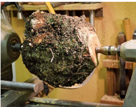
Balancing a burr lump between centres. The burr was about 250mm long x 225mm. Plan B was a light pull!
