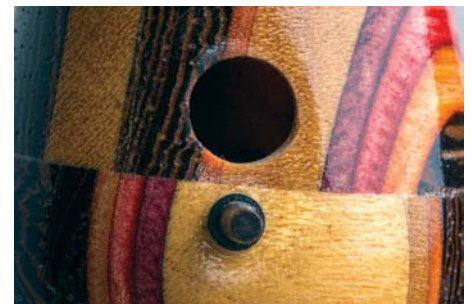
Lots of effort creating a unique blank. Far too little effort in layout and drilling the holes. Attention to detail isn't that difficult and it pays dividends
