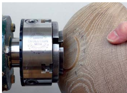
The base of the bowl shows I have marked the position of each jaw, to enable accurate remounting
