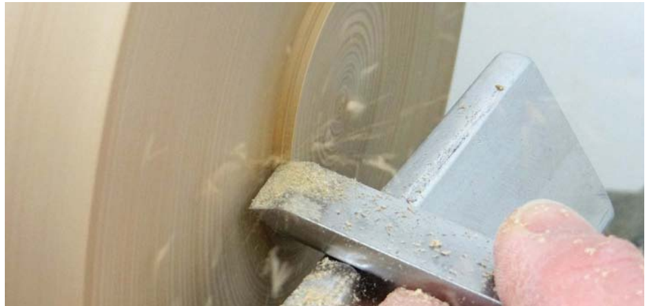
Cutting the spigot with a skew, used in scraping mode
