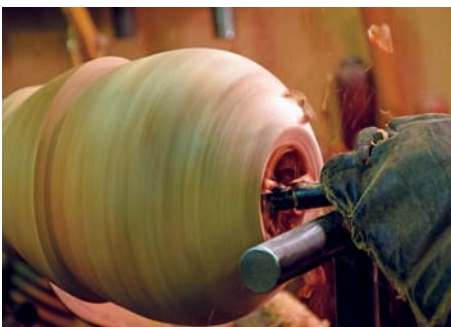
Outside shaping is done in stages as the hollowing progresses
