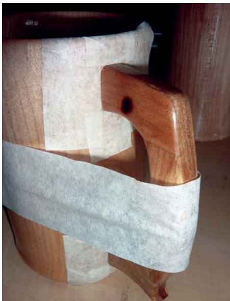
The handle taped into place
