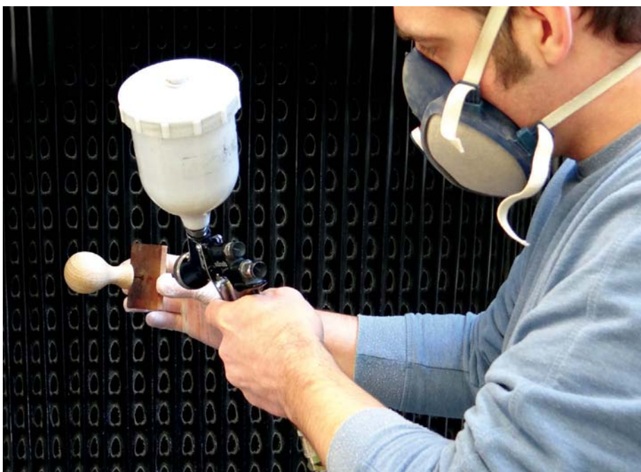
Spraying the coffee tamper with gloss lacquer in the spray booth
