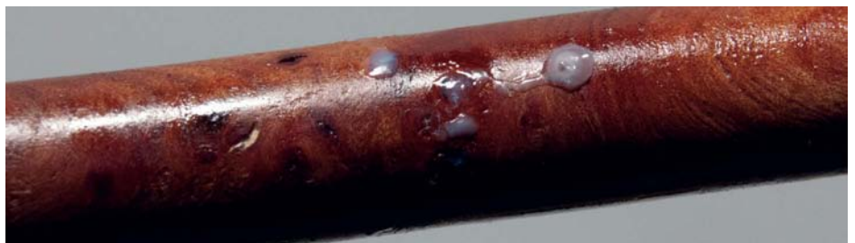
Too much accelerator can cause the CA to go white
