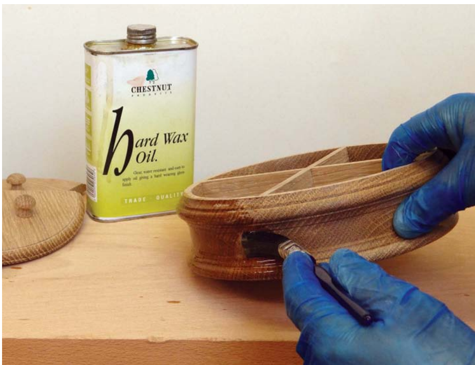
Applying oil with a brush
