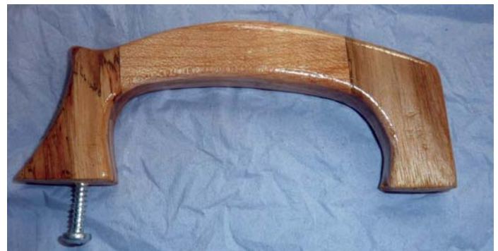
Screw a long small diameter screw into one end of the handle
