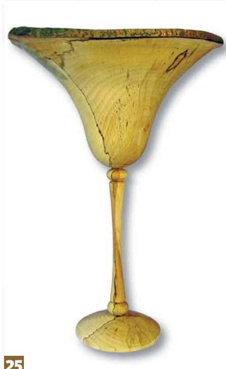
Step 25: apply oil to the entire goblet, allow to soak in and wipe away the excess. Place in a cool, draught-free location in your workshop for a couple of weeks before moving to a cool, draught-free location in your home. After a week, your goblet can be moved to a warm location for display. Here is the finished piece
