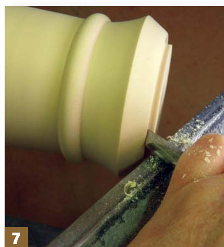
Step 7: with the outside of the chimney pot shaped, true up the front edge using a 10mm fingernail spindle gouge and sand to a finish using your usual sanding grits
