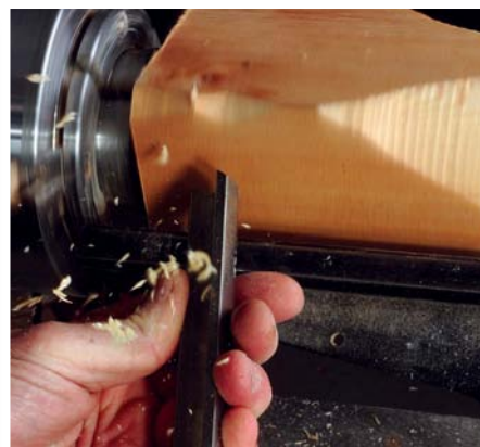
... reverse the tool and the direction of the cut and start to smooth or shape the rest of the piece, stopping often to see how you progress
