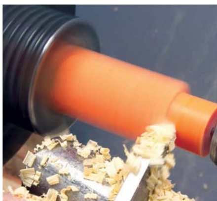
A sharp parting tool will work very well, not only on tight spaces, but also in the open. Basically a skew chisel, it will create very nice straight sections
