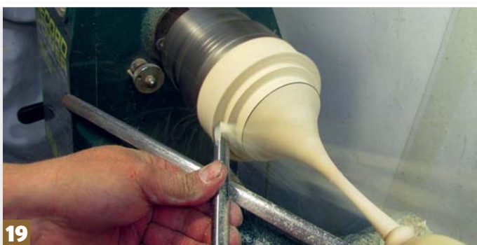
Step 19: mark the final diameter of the foot onto the face of the waste section and turn down to this line using a 10mm bowl gouge
