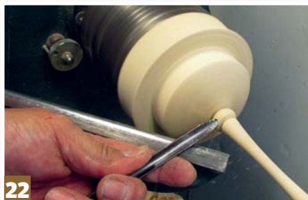
Step 22: using a pencil and rule, mark the width of the bead onto this section. Continue using the spindle gouge to shape the bead as before
