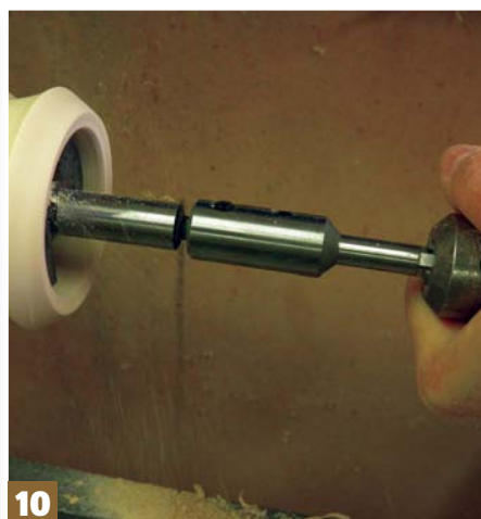
Step 10: an alternative method is using a Forstner bit fitted into a Jacobs chuck. Starting with approximately 25mm diameter and increasing in size until the required diameter is achieved
