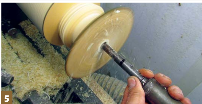
Step 5: measure the eventual depth of the bowl from the rim using the line previously marked. Subtract 10mm from this and mark accurately onto the shaft of a 20mm sawtooth bit held in the tailcentre. Drill out to this line and withdraw the drill regularly to remove the shavings
