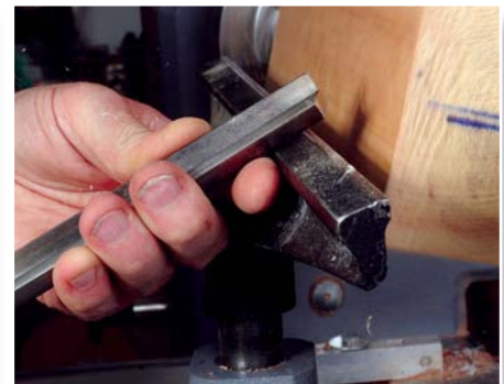
... then raise the handle until the cutting edge makes contact with the wood
