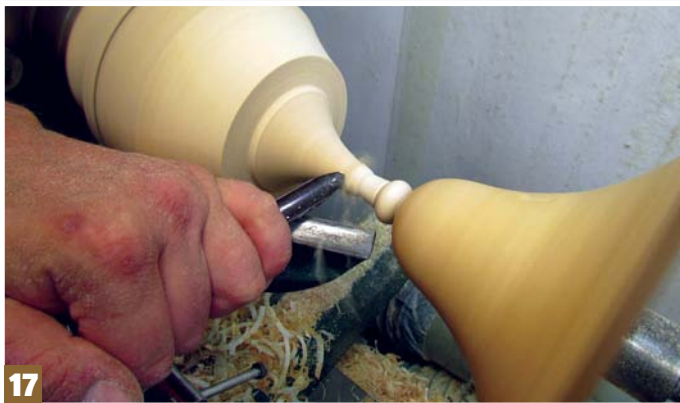
Step 17: blend to final shape and thickness using the 10mm spindle gouge, always working with the grain downhill
