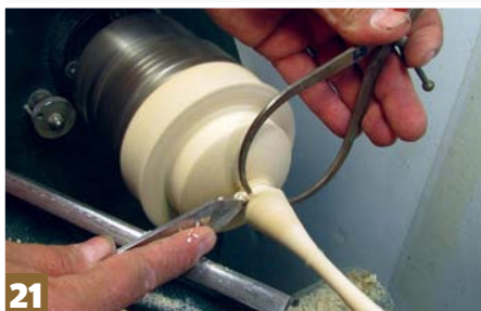
Step 21: using the first bead, set your callipers to size and part in above the foot with a 6mm parting tool, opening out along the stem to a width of 15mm
