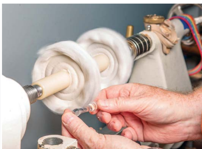
Every plastic I've worked with can benefit from buffing once the sanding and Micromesh process has been completed
