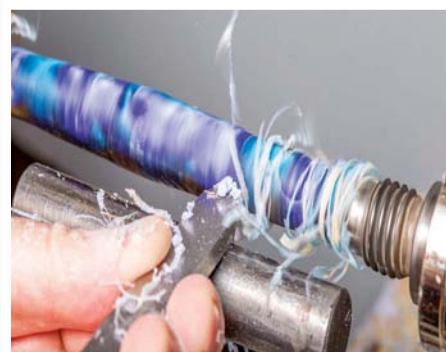
Scraping can be done on both thermosets and thermoplastics, but only as needed. The best use of scraping is brittle, chippy materials. Light touch and with minimal burr
