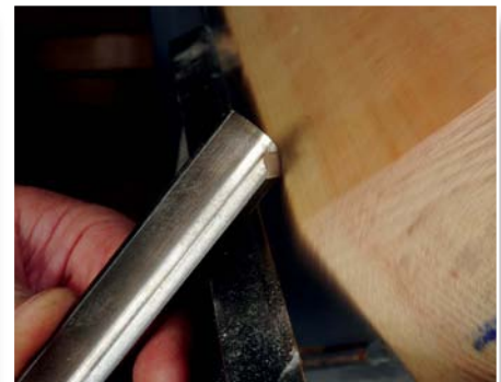
As you raise the handle, the ticking noise you hear is the heel making contact with the corners of the wood
