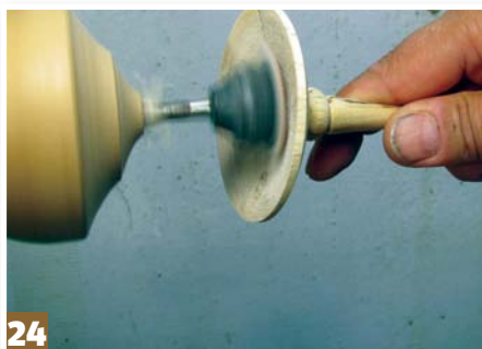
Step 24: blend the base with a sharp chisel or power carver, always cutting away from your body. Blend with abrasive attached to a small sanding arbor held in the chuck of the lathe
