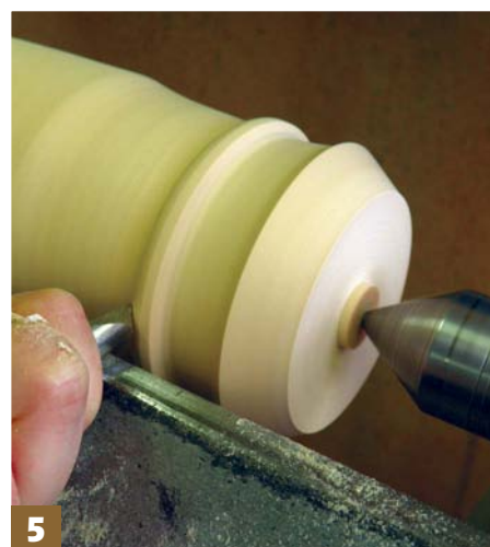
Step 5: create the bead section using a 10mm fingernail profile spindle gouge
