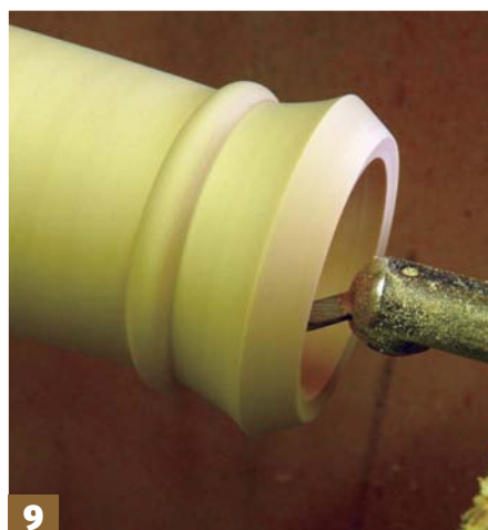
Step 9: using a swivel-tipped hollowing tool or similar, hollow the centre of the chimney pot to a diameter of 55mm
