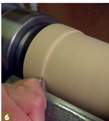
Step 6: create a step at the base, approximately 20mm long and round over the top. Taper the remaining timber from the step to the base of the bead; this section should be a flat gentle taper, which can be checked with a straightedge
