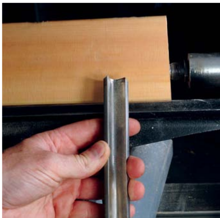
Using the gouge square-on to the work, cutting right at the bottom of the flute of the gouge...
