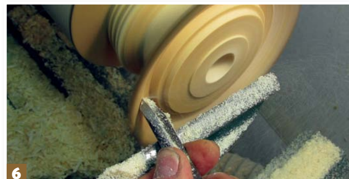
Step 6: using a 10mm bowl gouge, hollow out the first section by cutting gently into the end grain from the rim inwards. Continue until you have cleared the joint with the wood and bark by 25mm and reached a final wall thickness of 4mm. Cutting against the grain here helps to maintain the bark around the rim
