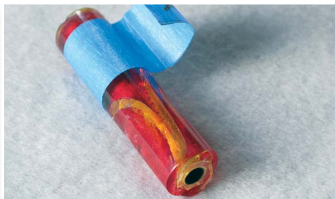
With care, embedded material plastics can be turned and finished. High speed, light touch and cool processing will be the keys to success
