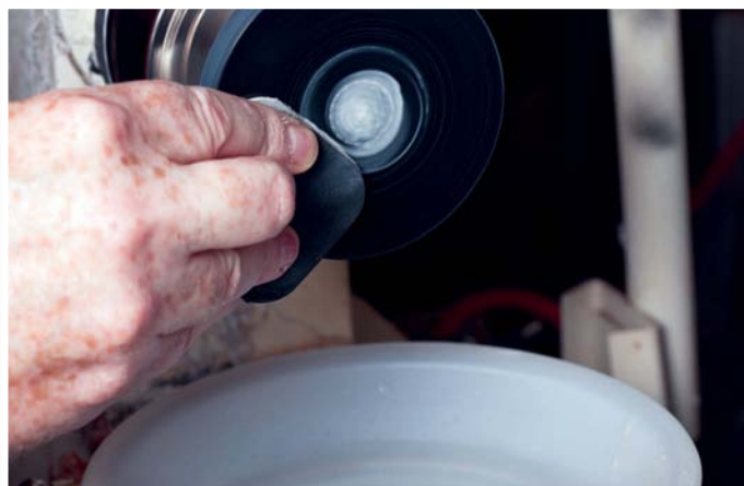
Wet sanding works well with plastics. While I don't wet sand with standard abrasives, I find it beneficial when using the Micromesh or very fine auto papers
