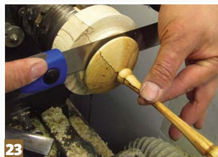
Step 23: mark the thickness of the foot on the outside and part in to the left of this using a 2mm parting tool, leaving around 10mm waste remaining. Stop the lathe and cut through the remaining waste using a fine-bladed saw. Apply oil to the stem, bead and foot and finish with abrasives from 120-320 grit
