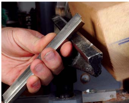
With the heel touching, raise the handle and bring the bevel into contact with the work...
