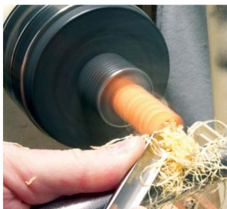
Depending on the hardness, plastics will hold good detail – especially thermosets. A sharp detail gouge will work quite well to cut in features
