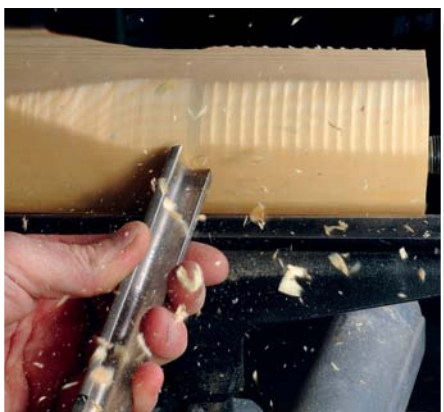
When you have smoothed down the area you are working and reached about two-thirds of the way along the work and the shape you require ...
