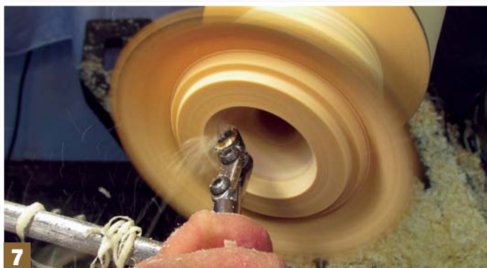
Step 7: using an end grain hollowing tool, continue hollowing and change direction to cut from the inside out, slightly thicker than required at this stage
