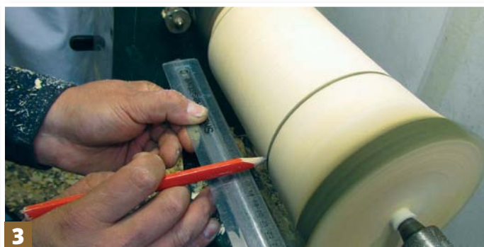
Step 3: clean up the front face with the bowl gouge up to the tailcentre, then mark the measurements of the bowl section, stem and foot onto the outside
