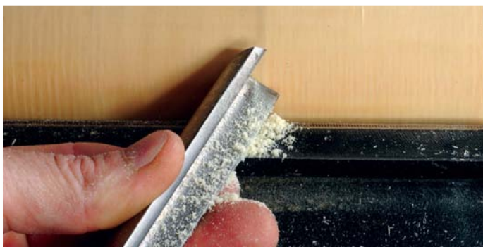
The refining cut is best used as a finishing cut or when you are cutting timber that splinters and fractures easily
