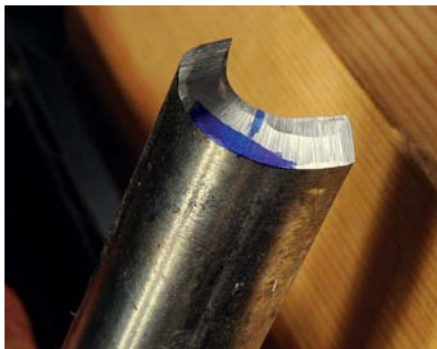
The heel of the bevel marked in blue is the area that should be the first to touch the spinning wood
