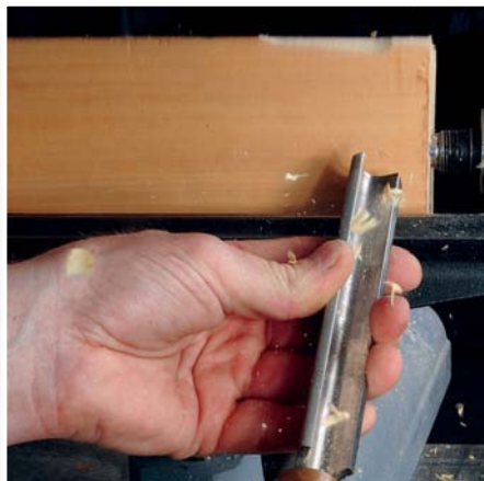
... or better still, you can shift your body so the tool is at a slight angle to it and cut on the lower wing
