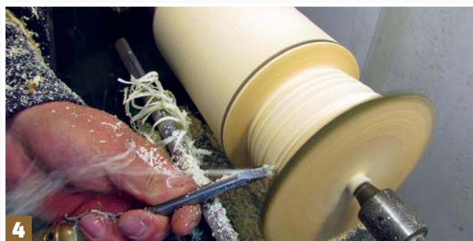
Step 4: using a 10mm bowl gouge, profile the first half of the bowl section, always working downhill from the outside in
