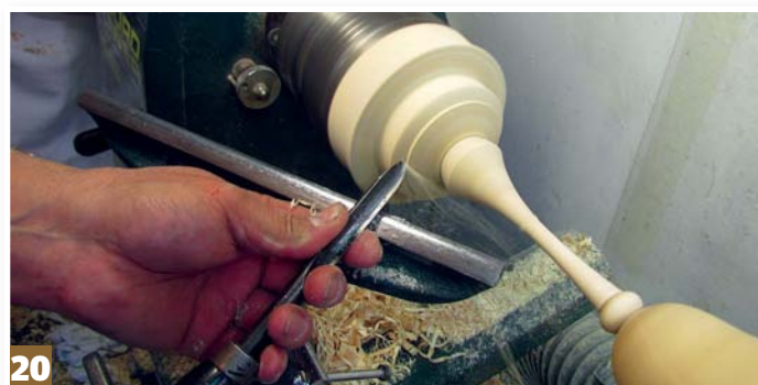
Step 20: refine the profile of the base using a 10mm spindle gouge, reducing the section for the bead as you progress
