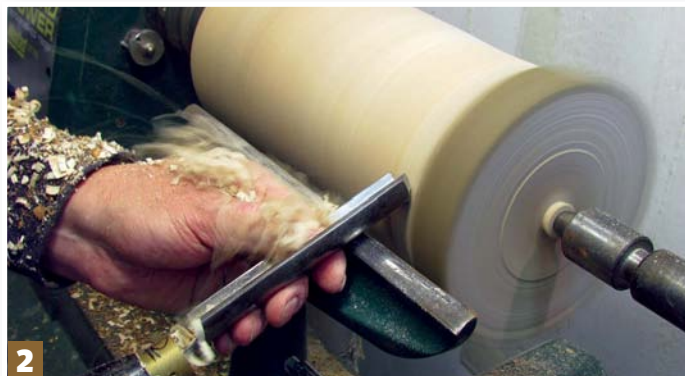
Step 2: reverse and tighten into the chuck bringing up the tailcentre for support. Using a 25mm spindle gouge, clean up the outside of the log to balance, leaving approximately 25mm width of bark on the rim
