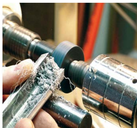
Thermosets are easily worked with cutting tools. The material cuts well with whispy curls possible, which creates a very good surface finish
