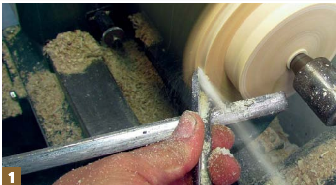
Step 1: mark the centre on both ends of the log and mount between centres. Using a 10mm bowl gouge, produce a spigot to suit your chuck jaws. Reduce the diameter of the log and produce a waste section around 50mm wide next to the spigot
