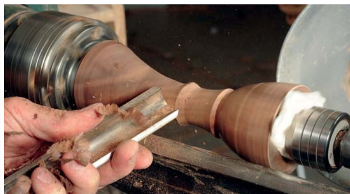
You must never cut uphill when spindle turning
