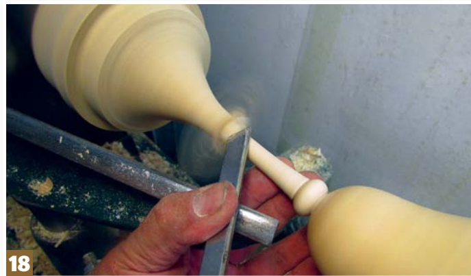
Step 18: refine the surface using a 12mm skew chisel. If the stem flexes, support it with your fingers as shown in the close-up at the start of the article, taking note of the safety precautions mentioned. If you are not confident in doing this, reduce the spindle speed further and refine with very light cuts. Finally, finish the bead and stem with abrasive from 120-320 grit
