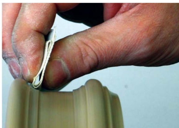
Carefully sanding the outside of the box
