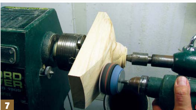
Step 7: stop the lathe and lock the spindle. Finish the underside of the wings using 120-240 grit abrasive attached to a 75mm sanding arbor in a drill. Finish by hand using the sanding pad with 320 grit abrasive and rub in line with the grain
