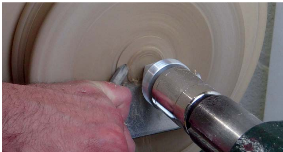
Turning the base of the box
