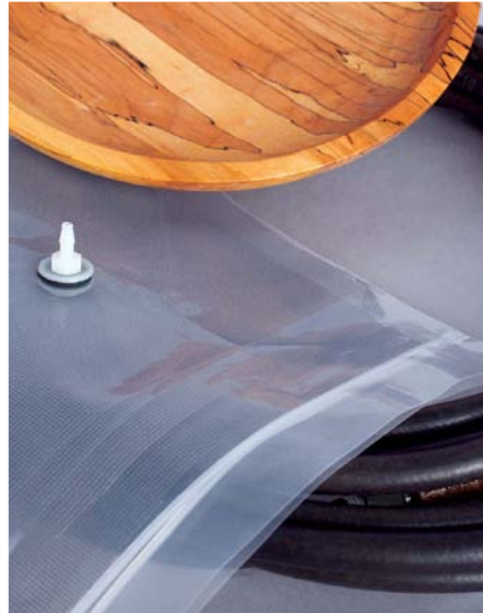
Help yourself with vacuum bagging by creating a cradle to minimise bag filling dimensions. My air line coiled up works nicely
