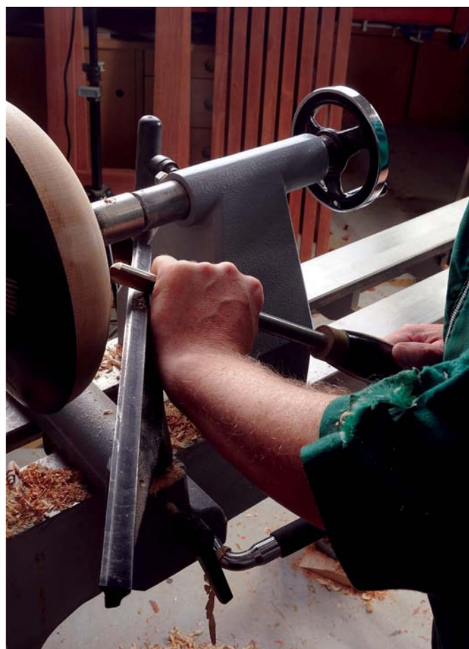
A typical stance that is a good starting point when spindle turning. Here, the overhand grip is being used
