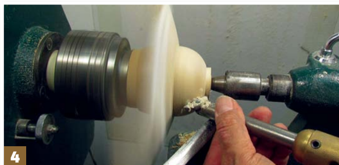
Step 4: using a 25mm square-end scraper, refine the finish of the bowl section being careful not to catch the corner of the scraper on the wing. Do not attempt to use the scraper on the wings. Or, miss out this process and go straight to...
