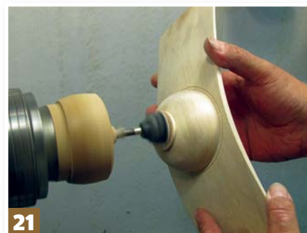
Step 21: blend the base with abrasives from 120-320 grit using a sanding arbor held in a friction drive
