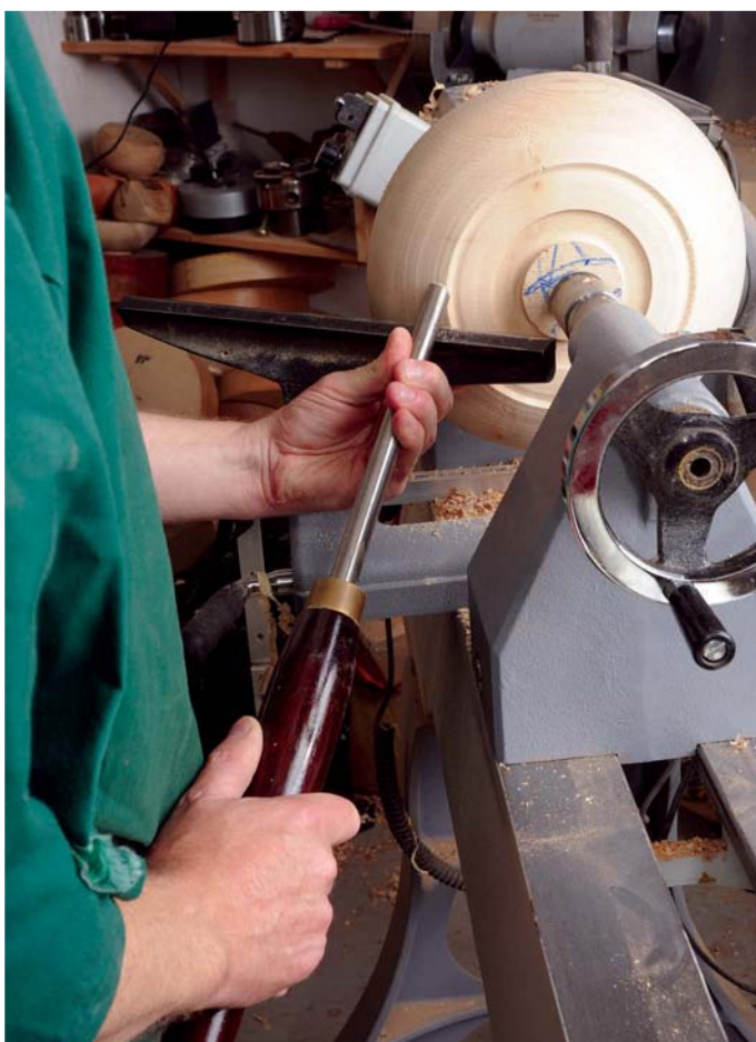
Underhand holding position with the thumb pointing along the handle in line with the tool blade
