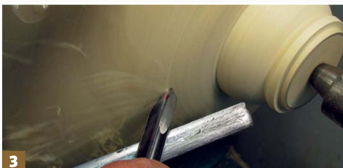
Step 3: once profiled, take several fine cuts traversing the tool slowly across the base of the wings; this will allow you to remove any tooling marks
