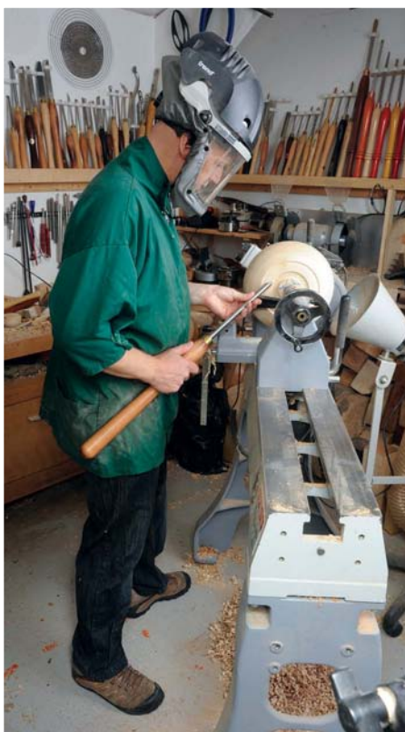
Underhand holding position with the thumb pointing along the handle in line with the tool blade
