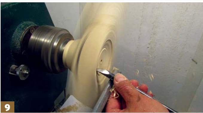
Step 9: using a 10mm bowl gouge, start to reduce the thickness of the bowl while following the curve of the base line – see cutting sequence diagram for more information
