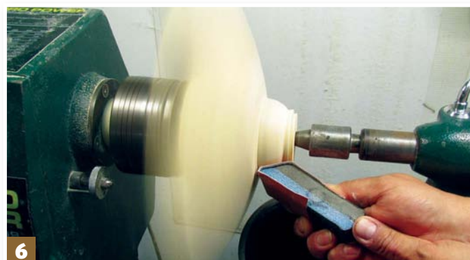
Step 6: finish the bowl using 120-320 grit abrasive attached to a sanding pad; this will keep your fingers away from the wings
