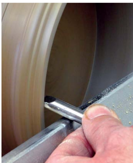
Using the round 'skew' as a shear scraper on the inside of the box
