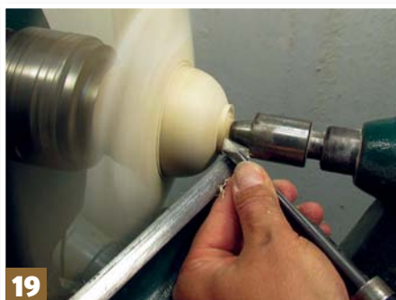
Step 19: concave the base using a 10mm spindle gouge to a safe distance from the tailcentre
