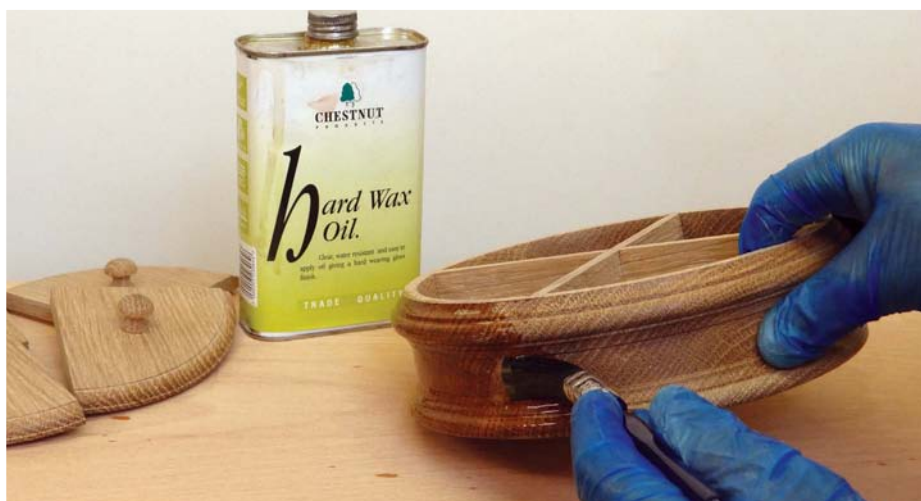
Applying the hard wax oil to the box
