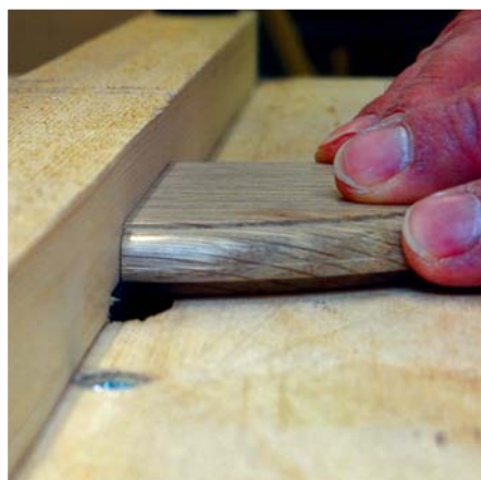
Routing the rebates on the lids
