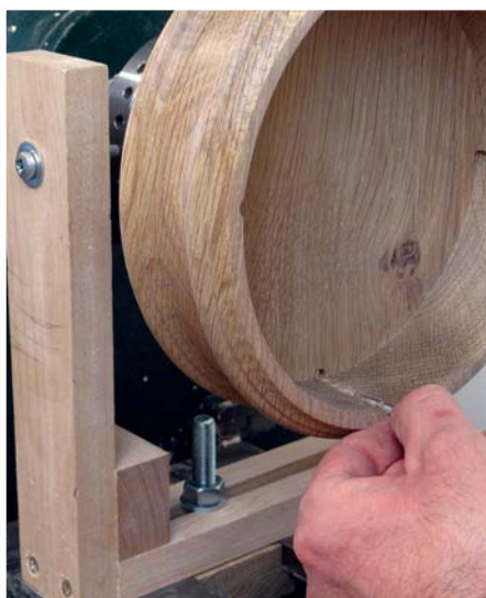
Paring the housings square while the box is held on the lathe
