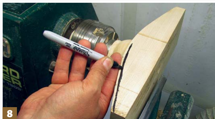
Step 8: reverse into the chuck and mark the intended thickness of the wing onto the edge using a marker pen or dark pencil. This mark will be visible as the blank spins, which will help you to gauge thickness
