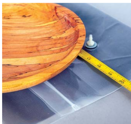
The larger bag from TMI Stick Fast is 510mm square. It is large enough for the work most of us are involved with
