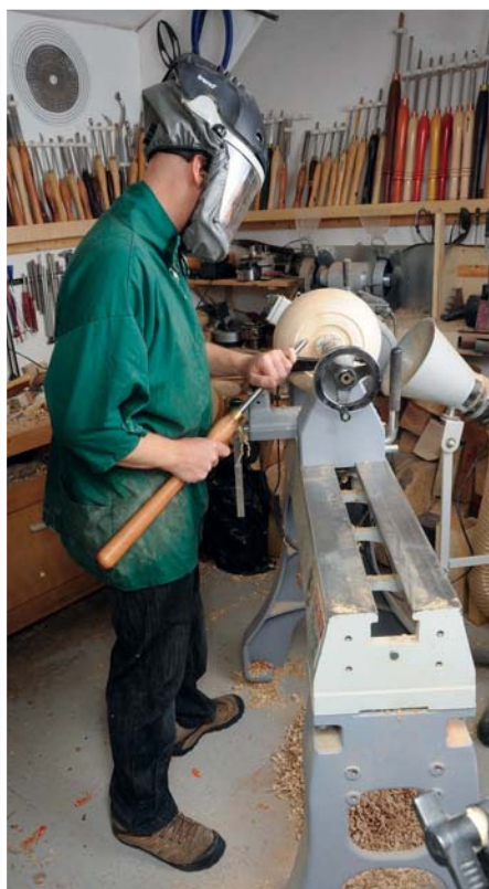
Holding the handle with a 'round the handle' grip
