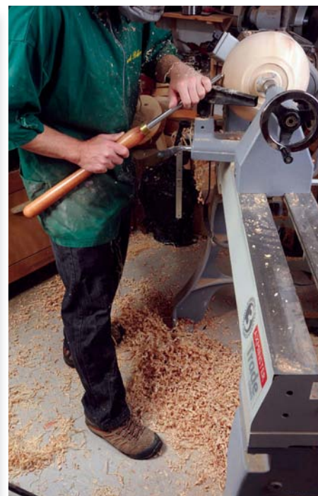
... gradually moving so that I am upright and square on to the upper edge of the work
