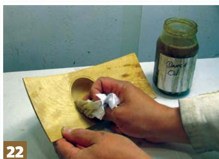
Step 22: you can now apply several coats of Danish oil and wipe away the excess with kitchen towel
