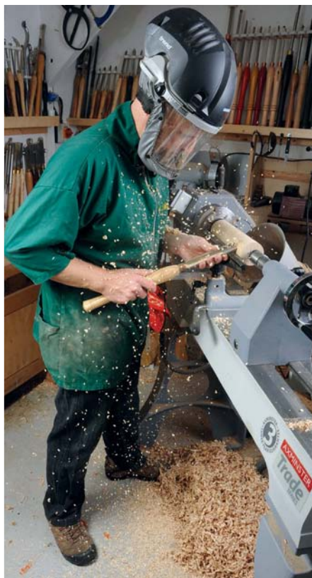
A typical stance that is a good starting point when spindle turning
