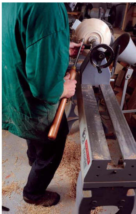
As you can see, my feet are at the 9 and 12.30 o'clock positions and I am leaning slightly on my right-hand leg at the start of the cut
