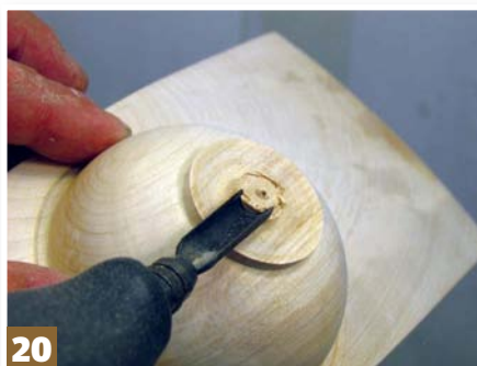
Step 20: remove from the lathe and cut away the waste using a power carver, ensuring to always cut away from your body
