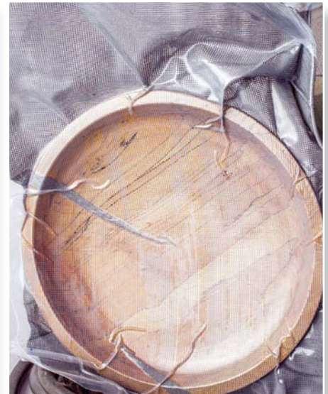
With sufficient resin for absorption, the bag is pulled to full vacuum with care to provide for a liquid trap
