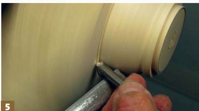
Step 5: ... using a 6mm point tool to produce a groove at the join between the bowl and wings, plus a second 3-4mm outside/next to this
