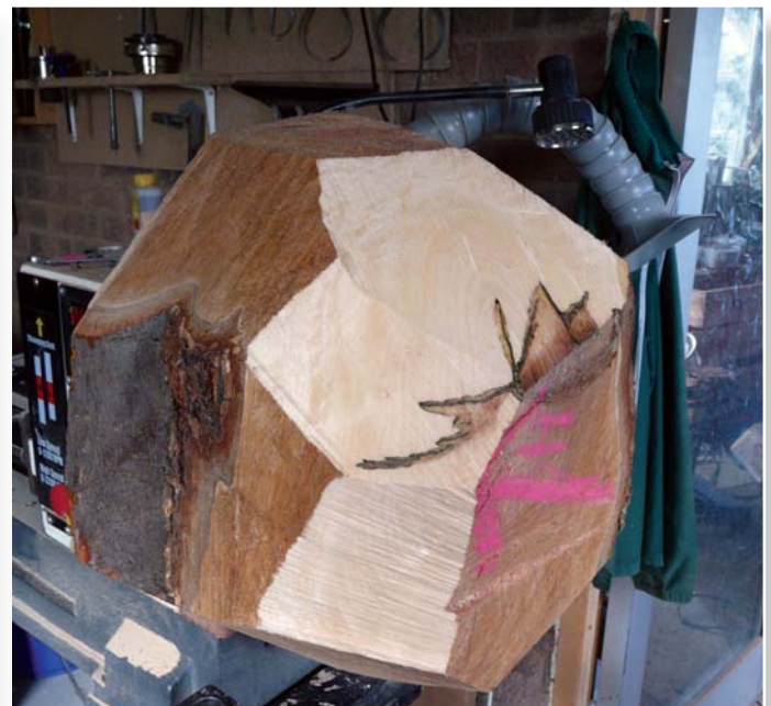
Wood cut away to reduce initial out-of-balance loads
