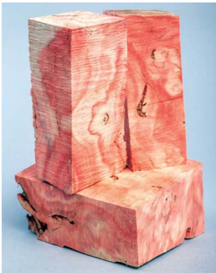
Boxelder ( Acer negundo ) burl cut to size for processing. The stabilisation will toughen it for turning and also help keep the colour from fading
