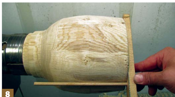
Step 8: using a depth gauge, measure from the front face to the final location of the base...
