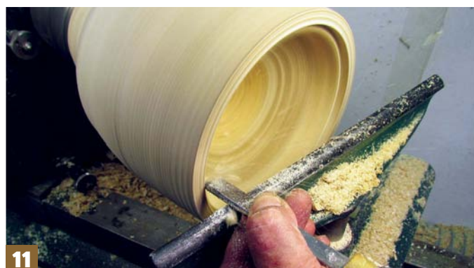
Step 11: use the toe of a 12mm skew chisel, presented horizontally on the toolrest in trailing mode, and plunge gently in to produce a shoulder; this will allow you to accept the remaining spigot on the top section previously parted
