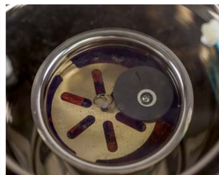
Maintain the vacuum until the rate and size of bubbles diminishes to a minimum. At that point, the vacuum can be released
