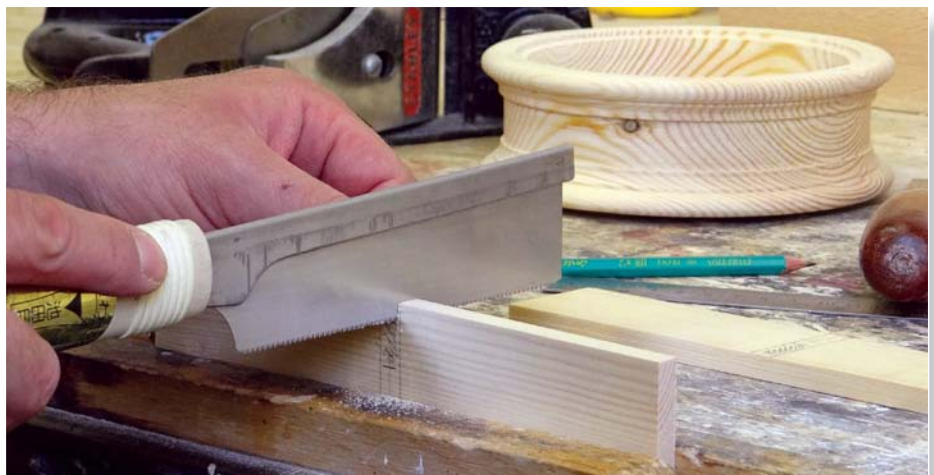
Cutting the halving joint on the dividing sections
