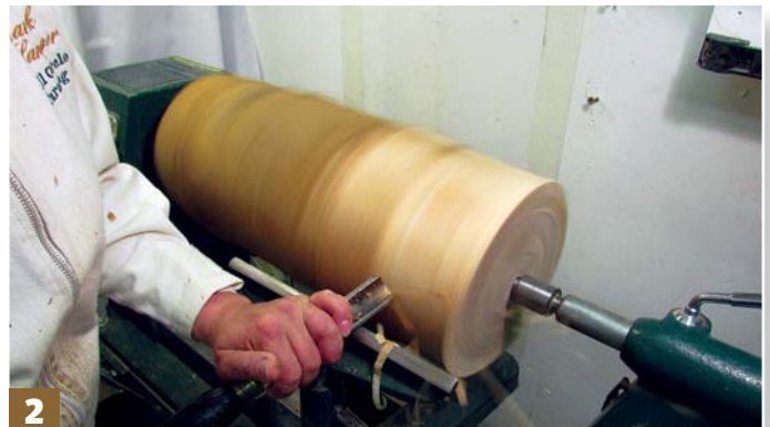
Step 2: using a 25mm spindle roughing gouge with the lathe set to slow, start to rough to the round
