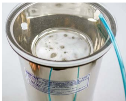
The chamber is evacuated but done slowly to prevent foaming over the rim. Use any vacuum limits, as per your chamber manufacturer specs
