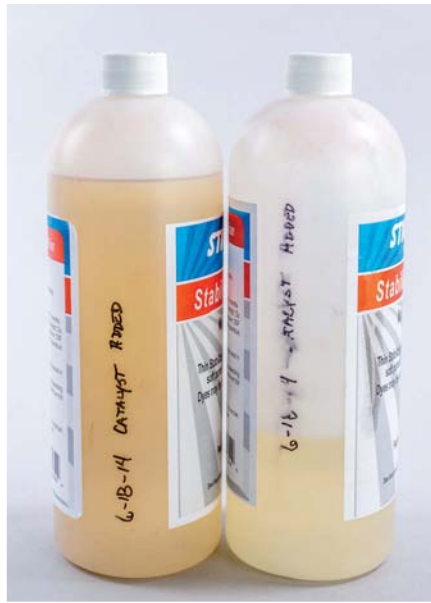
The dozen very porous blanks stabilised for this column consumed only 24oz of resin. All of the rest was reclaimed for future use
