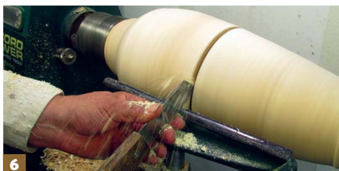
Step 6: use a 2mm parting tool to part in slightly to the right of the shoulder left by the previous parting tool. You want to leave a register on the front face. Continue parting through and stop with around 25mm wood remaining
