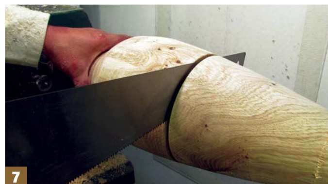
Step 7: stop the lathe and cut through the remaining using a hand saw
