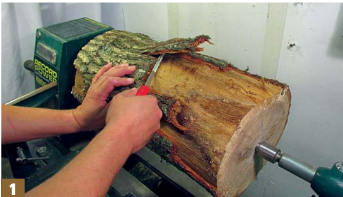
Step 1: mount the blank between centres and remove the bark using a screwdriver to initially lift the loose sections. Always ensure to push away from your body
