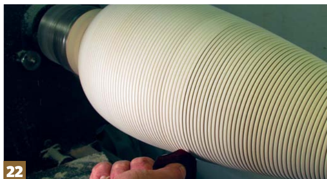
Step 22: with the lathe stopped, texture the outside using a 50mm round wire brush fitted in a power drill by running it perpendicular across the beads. Using a thin piece of Formica or a medium wire burner, burn lines in the base of each
