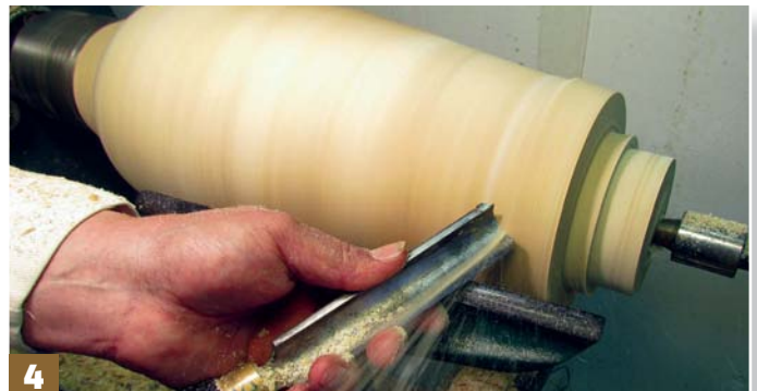
Step 4: mount in the chuck and bring up the tailcentre, using a 25mm spindle roughing gouge to rough down the general shape, always working from large diameter to small towards the tailcentre and chuck. At this stage, leave oversize
