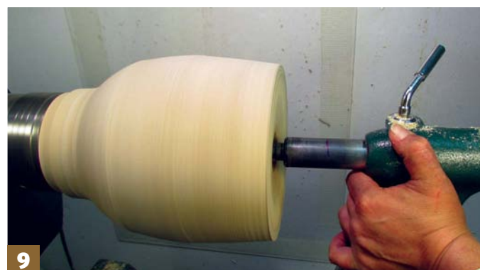
Step 9: ... mark this onto the shaft of a long series 50mm sawtooth bit or the quill of the tailcentre, then drill out to depth. It is important to measure and drill out accurately to depth, so measure twice and cut once
