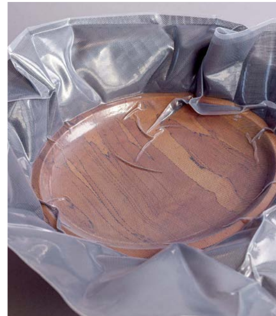
Using a cradle for support and a vacuum bag, much larger work can be stabilised without large quantities of extra resin
