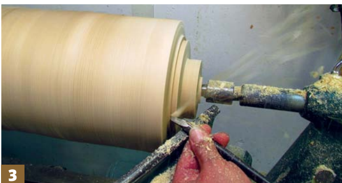
Step 3: using a 10mm bowl gouge, produce a spigot and waste section at each end to suit the jaws of your chuck. Here I am using 100mm gripper jaws for maximum security as standard ‘C’ jaws do not offer enough security
