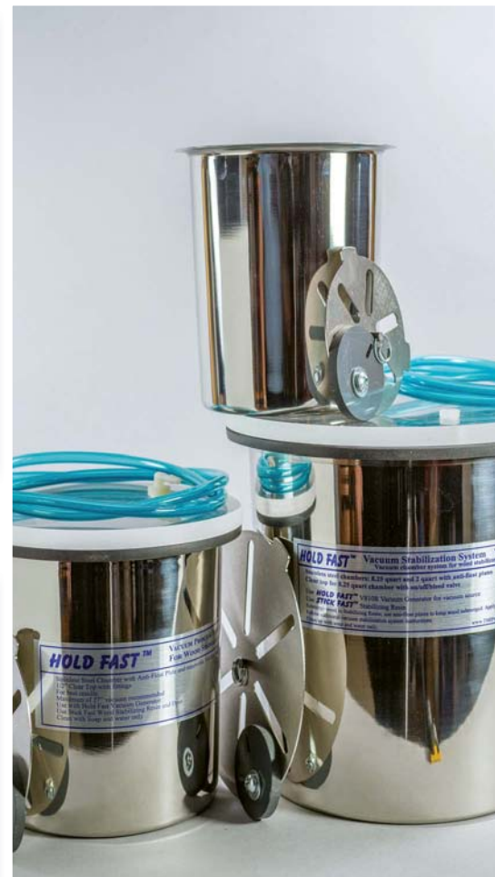
The TMI Hold Fast vacuum chambers are stainless steel with clear plastic lids. They recommend 27inHg maximum for their use
