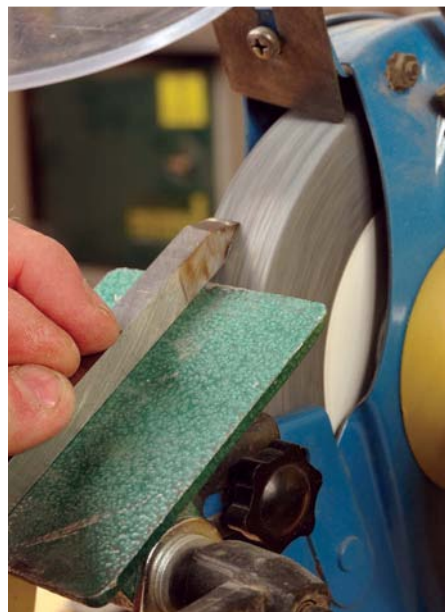
Moving the beading & parting tool along the toolrest to access the full width of the wheel or belt
