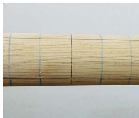
The spindle showing the pitch lines in pencil and pitch dividing lines in blue
