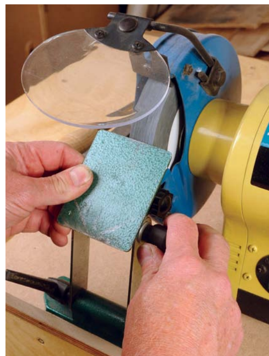
An adjustable rise and tilt table
