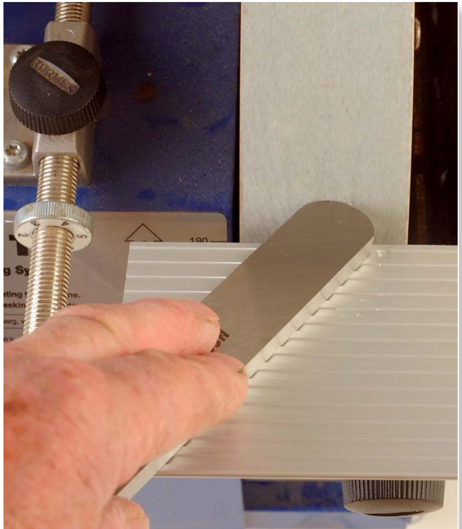
Start with the blade flat on the toolrest with the table set to the right angle. Present the blade to the wheel or belt and...
