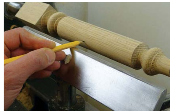
Drawing the start lines along the spindle, level with the corners of the pommel
