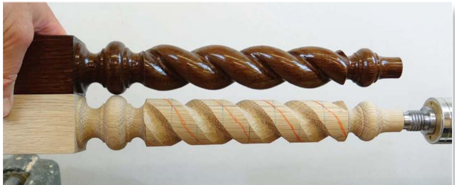
Comparing with the original again after the groove is cut
