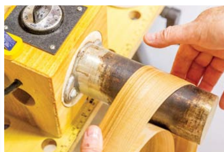
Work the wood! This is a progressive process of wetting, heating, wetting, heating, coaxing the form and repeat until it gently yields to your wishes
