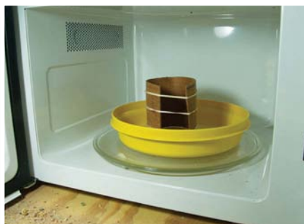
A household type microwave will work. Do not ever use for food service again once you've used it for drying or bending wood
