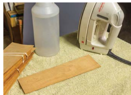
A spray bottle of plain tap water and a household iron will work to bend wood. Although it doesn't provide form, it can make the wood pliable to work with
