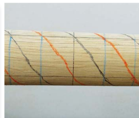
The setting out is complete with the valleys drawn in pencil and the bines marked in orange
