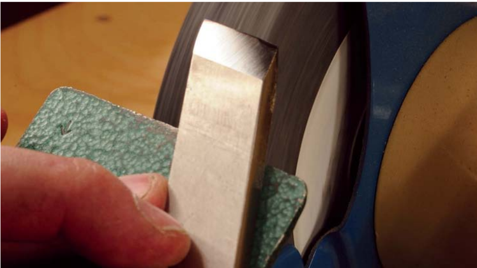
The skew chisel being sharpened on a bench grinder
