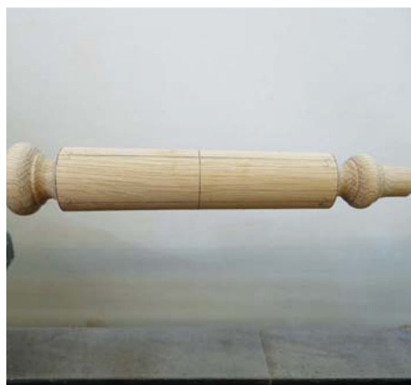
The pitch lines drawn on the spindle
