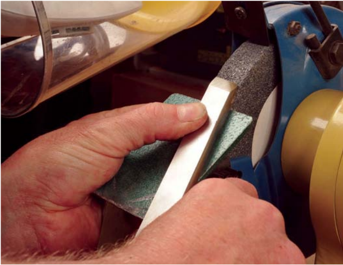
Adjusting a rise and tilt table for the skew chisel – bevel contact required
