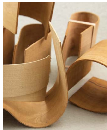
Regardless of the material and the ultimate shape, if the grain isn't perfectly orientated to the surface of the wood it is likely to fail, now or later
