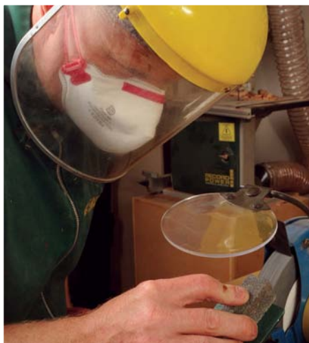
Cleaning a grinding wheel with a devil stone
