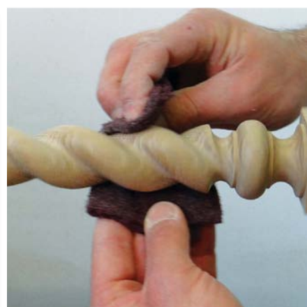
Final sanding with the lathe running at 200rpm
