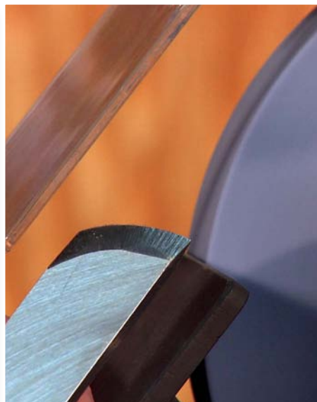
The edge was rough-shaped on a coarse wheel. Note the grooves on the bevel from this process. The finer the wheel used, the better and more refined the cutting edge will be
