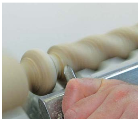
The final tidying cut in the cove, to crisp the end of the twist
