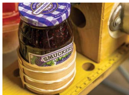
If you want to ensure that the coil is perfectly round, use a form of some sort. This jam jar works nicely and creates a perfect circle of 75mm in diameter
