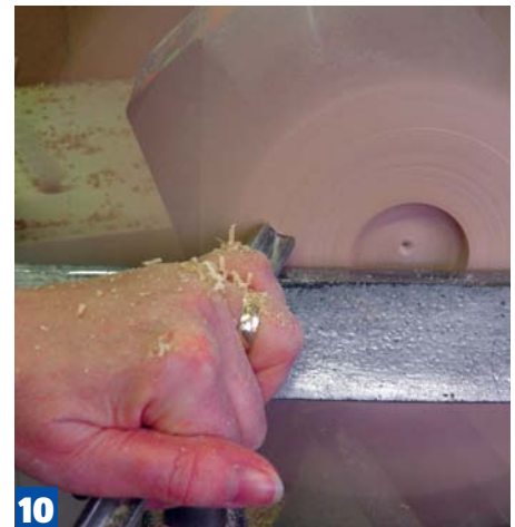
Bevel cutting the bowl shape
