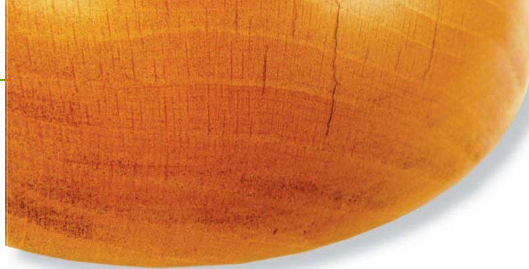
Heat checks running across the end grain. A stained wax was used to show them more clearly for the photo
