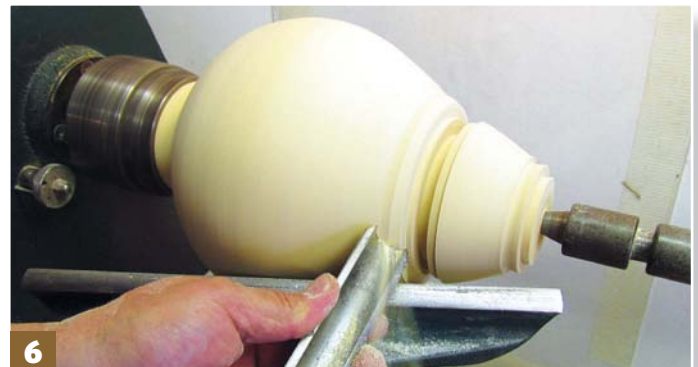
Step 6: use the spindle roughing gouge to shape down to the previous 95mm sizing cuts, continue towards the tailstock, reducing and shaping the lid profile
