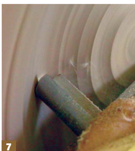
Step 7: using a 10mm standard-grind bowl gouge, remove the centre of the bowl creating the correct profile at the bottom to fit the brass candle holder. Try for fit before sanding to a finish and avoid removing the crisp detail
