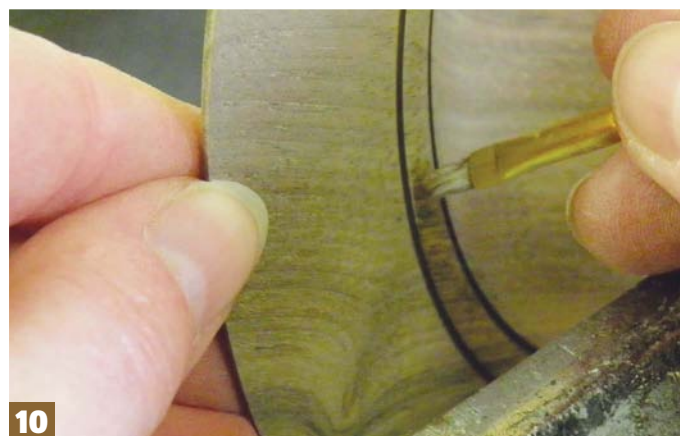
Step 10: with the bowl still mounted on the lathe, use a small paintbrush to seal the surface of the ring and, when dry, apply a thin coat of leaf size. Allow to stand until the size becomes tacky to touch
