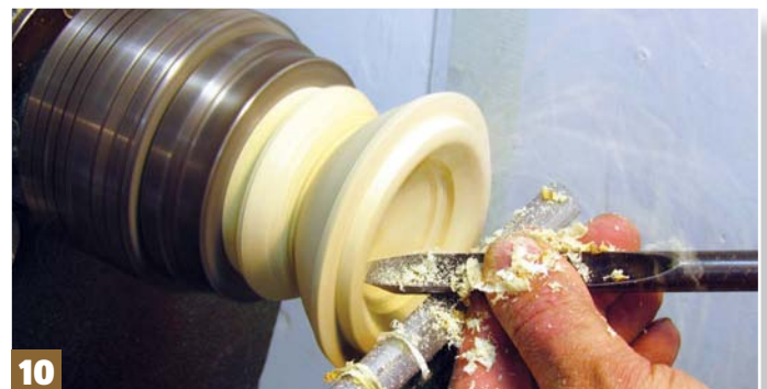
Step 10: place the lid into the chuck and use a 10mm spindle gouge to hollow the underside, taking into account the final profile. If you're using unseasoned wood, produce the wall thickness to a constant 15mm all the way around. There will be some thicker areas, such as that of the spigot and waste, but cut in to these as much as possible while leaving enough material for rigidity when finishing later
