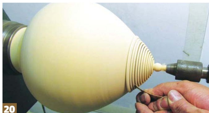
Step 20: using a small piece of Formica with the lathe speed set to around 1,000rpm, burn a line at the base of each bead. Alternatively, a sharp graphite pencil can be used to add definition
