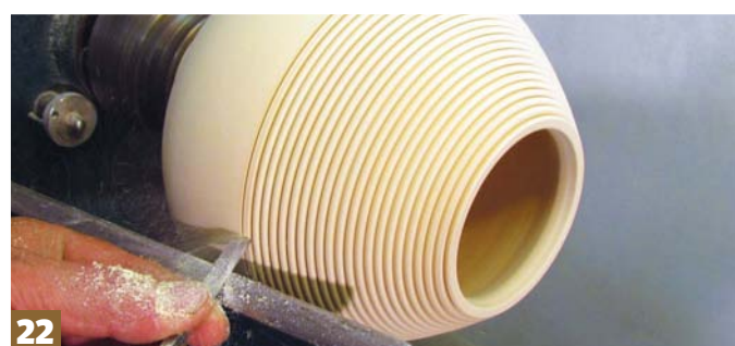
Step 22: remove the lid and bead the main form as before to a safe distance from the chuck. Finish and define the beads with a burn line or pencil
