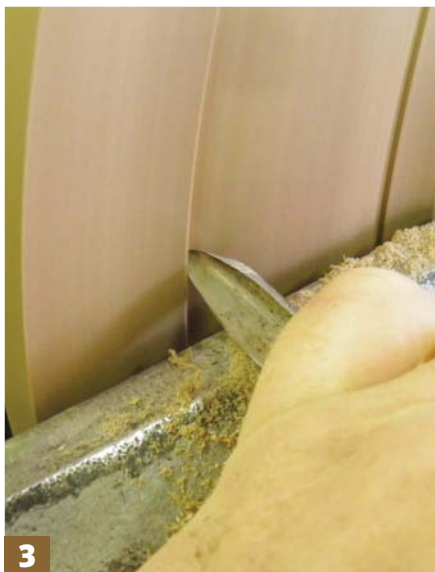
Step 3: continue with the shape creating a step approximately 31mm from the outer edge. Here I am using a 10mm fingernail profile spindle gouge to cut a crisp undercut where the two surfaces meet
