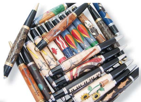
I use a CA finish on my turned pens almost exclusively. It is simply wiped on in very thin coats and repeated until the build thickness desired is achieved
