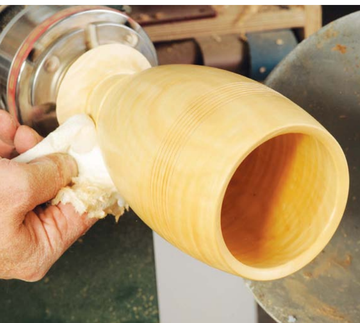
A wax finish being applied with paper kitchen towel
