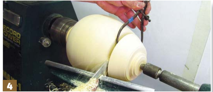
Step 4: using callipers set to 80mm and a 6mm parting tool, part in centrally to the line sizing the lid spigot that will fit into the main form. Open this out to 12mm wide by parting in a second time towards the tailstock, again using the callipers for sizing
