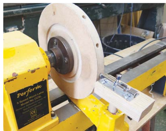
The indexer on my Perform demo lathe
