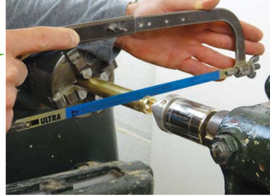
Sawing off the ring with a hacksaw
