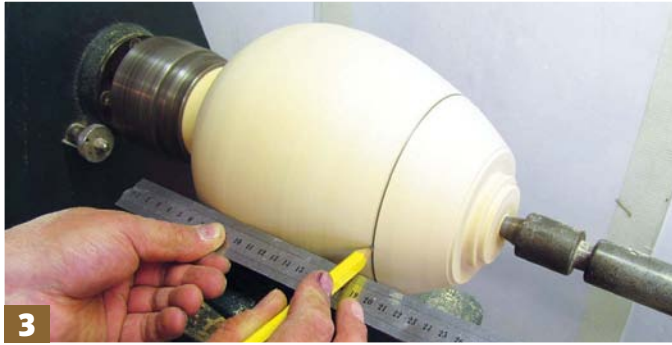
Step 3: using a rule and pencil, mark 180mm up from the base, this being the join of the lid
