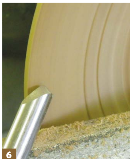
Step 6: using a 10mm long-grind bowl gouge, refine the shape, reducing the thickness on both sides of the grooves to create a slightly raised ring
