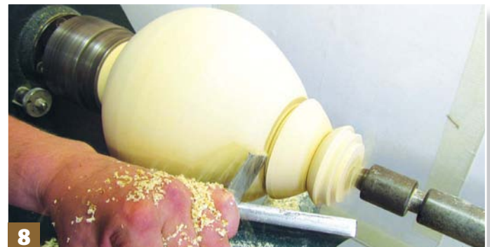
Step 8: use a 2mm parting tool to part in just right of the rim of the main form to leave a registration mark for fitting of the lid. Stop short without parting all the way through and stop the lathe
