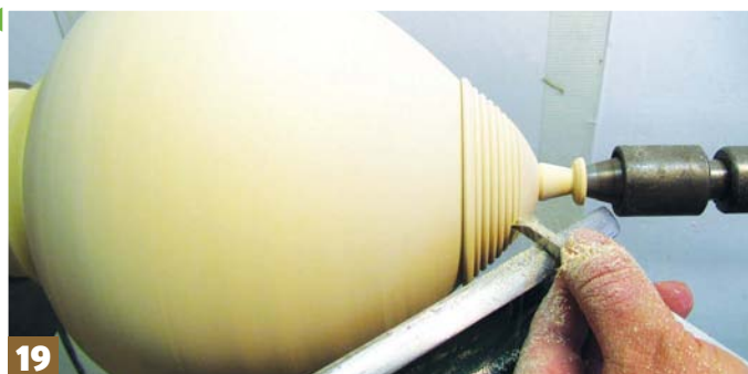
Step 19: produce beads from the base of the lid up using a 3mm beading tool, stop short of the button. Once complete, finish the beads with 240-grit abrasive folded tightly in half, being careful not to alter the profile of the form with the abrasive
