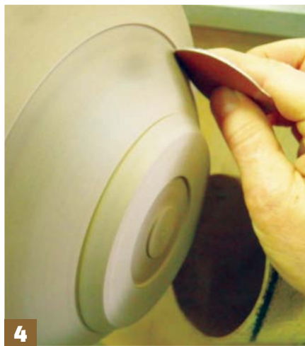
Step 4: sand the underneath of the bowl. A rotary sander can be used for the bulk of the surface, but the crisp edges will need to be hand sanded. Keep the abrasive moving against the rotation of the lathe; this will minimise scratch lines. Work through your usual grits checking the surface before progressing to the next grit
