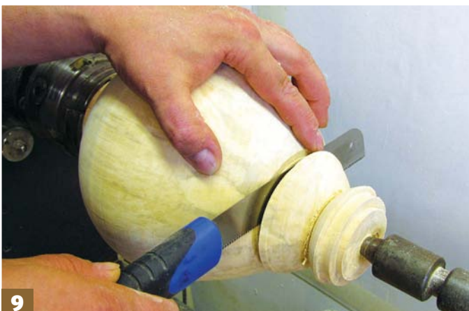
Step 9: cut through the remaining waste using a fine-bladed saw
