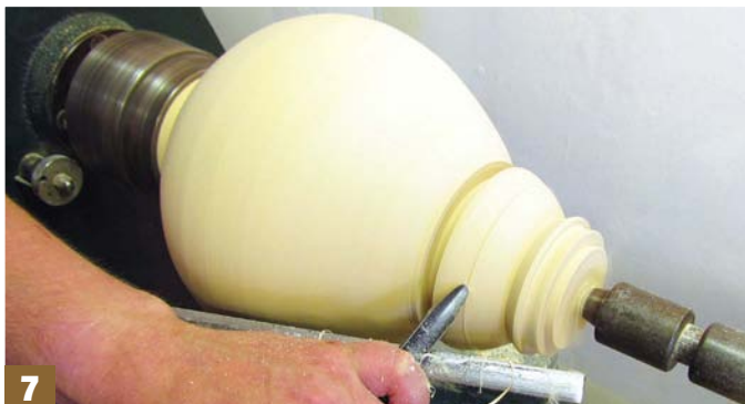
Step 7: using a 10mm spindle gouge, refine the main form and lid reducing the waste at the tailstock end leaving the waste section and spigot in place
