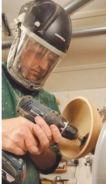
Power sanding with a drill fitted with a sanding arbor loaded with abrasive
