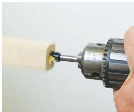
Drilling the wooden collar with the router cutter mounted in the Jacobs chuck
