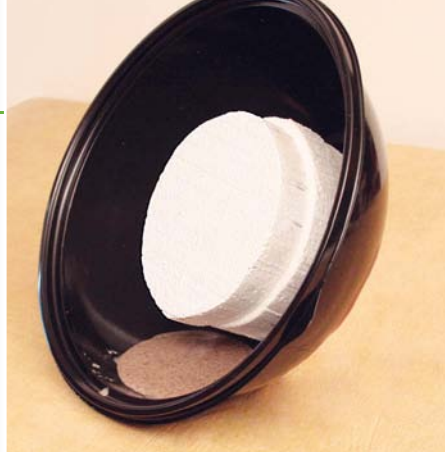
Hemispherical mould showing Styrofoam used to reduce resin volume
