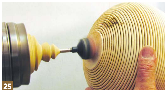
Step 25: Refine the base with abrasive on an arbor driven via a waste piece of wood in the chuck of your lathe
