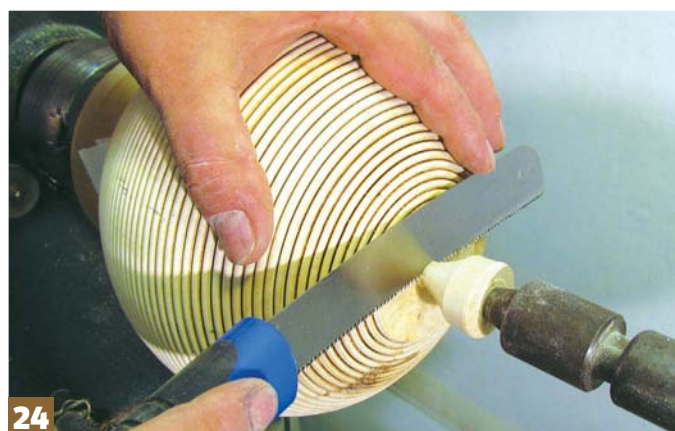
Step 24: cut through the remaining waste with a fine blade saw, cutting away the remaining on the base with a sharp chisel or power carver, always making sure you cut away from your body
