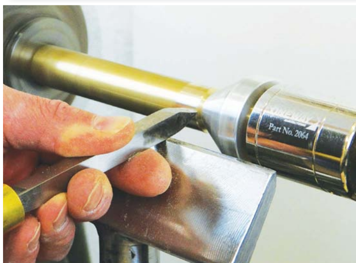
Cleaning and truing up the brass rod
