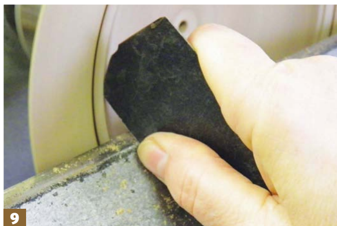
Step 9: using a strip of Formica, burn the 'V' grooves either side of the ring. Use the toolrest for support and apply adequate pressure to create the burn
