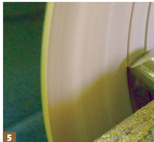
Step 5: you can now remount the bowl using the chucking recess cut earlier. True up the front face and roughly create the rim. 31mm from the outer edge cut two 'V' grooves to create a ring approximately 7mm wide. This ring will receive the metal leaf enhancement. Here I am using a 10mm bead former to create the ring
