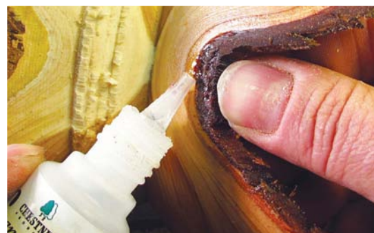
Bark being secured in place with CA glue
