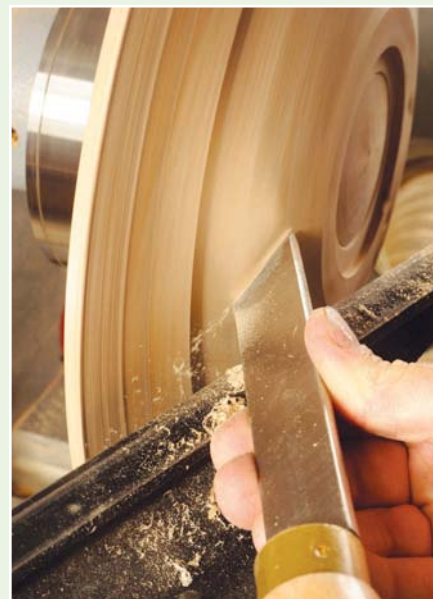
Shear scraping with a traditional rectangular-blade scraper. Again, the cut occurs on the lower half of the cutting edge
