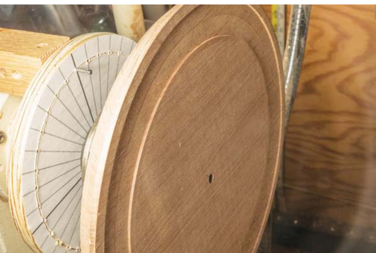
Indexed assembly, drilling, marking, slotting or whatever is easily done on the lathe. Shop-bought or home-made indexing works well
