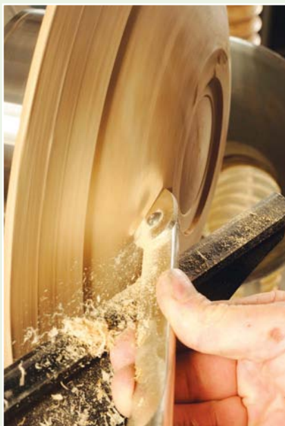
Shear scraping with the cut occurring on the lower half of the cutting edge
