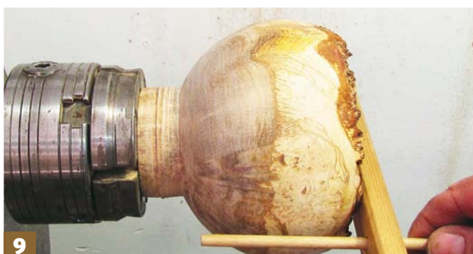
Step 9: finally, refine the lower section with the scraper
