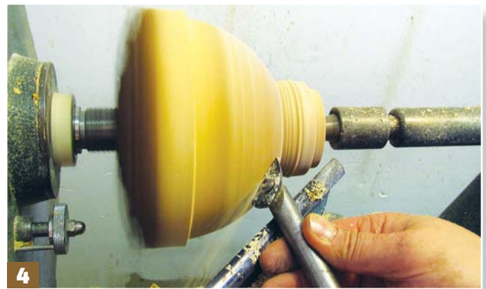
Step 4: refine the profiled area with a 25mm square-end scraper
