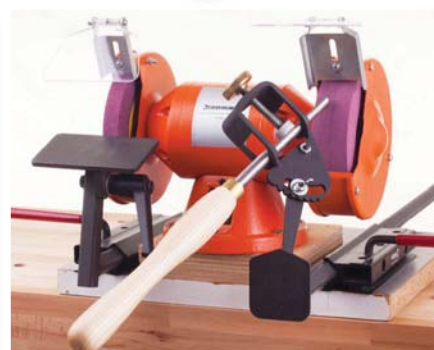
The fingernail/adjustable grind jig for creating swept-back grinds
