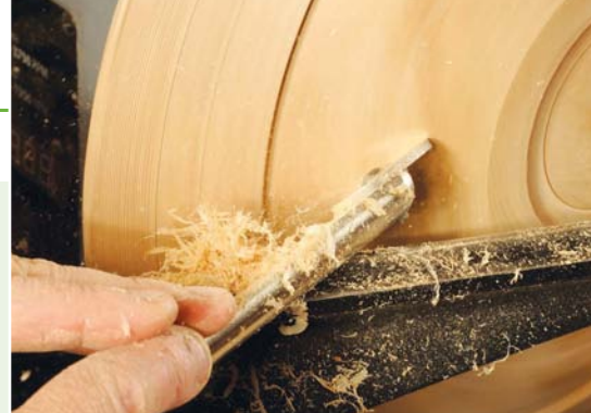
Shear scraping with a multi-tipped tipped tool
