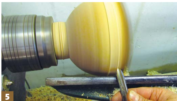
Step 5: reverse into the chuck, cut from the rim into the lower section with the bowl gouge and blend the two areas together. Refine as before using the scraper, taking fine cuts and again working from the rim down, which will prevent the bark from being pulled from the rim
