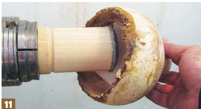
Step 11: reverse the bowl onto a friction drive that fits down into the base of the bowl, protecting the surface with several sheets of kitchen towel. Bring the tailcentre up for support and apply moderate pressure
