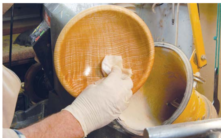
Finishing ash with an oil finish
