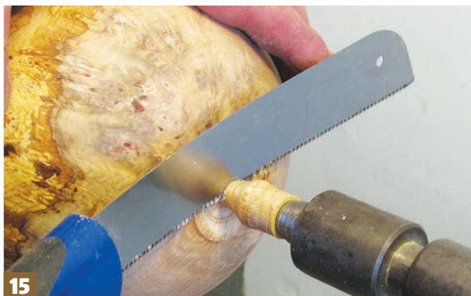
Step 15: stop the lathe and cut through the remaining waste with a fine-blade saw
