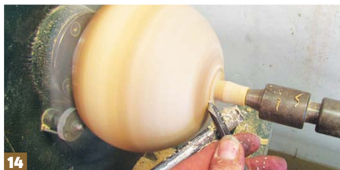
Step 14: using a 10mm spindle gouge, further reduce the waste and profile the foot, making sure it is slightly concave. Finish the base with abrasive by hand from 120-320 grit
