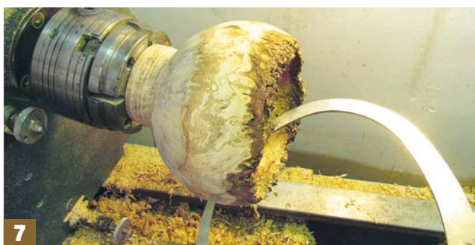
Step 7: continue reducing the wall thickness to 3-6 mm. Check regularly with callipers and refine using a 25mm round-nose scraper as required remembering to cut from the rim in; this will prevent breakout of the bark or edge
