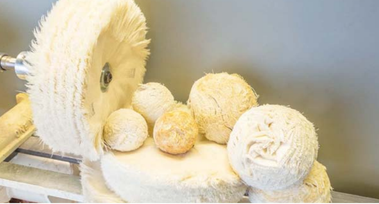
The Beall Buffing System includes three buffs for different compounds and has inside buff sets of different sizes
