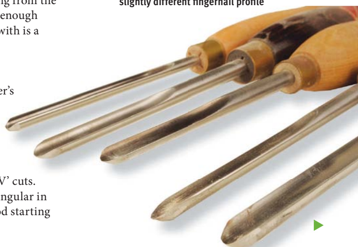
Spindle gouges ranging from 6mm on the left to 13mm on the right, each with a slightly different fingernail profile
