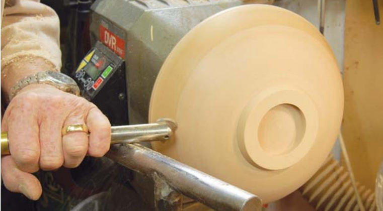
Shear scraping ash
