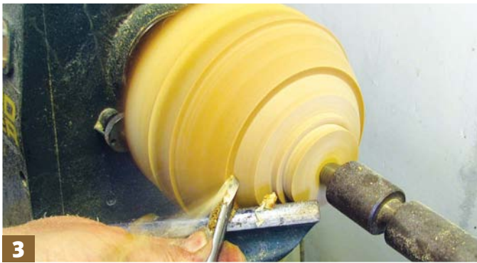
Step 3: using the bowl gouge, continue to shape the base profile of the bowl. Cut from the tailcentre towards the headstock stopping around 20mm from the bark/natural edge. See the cutting sequence diagrams for clarity
