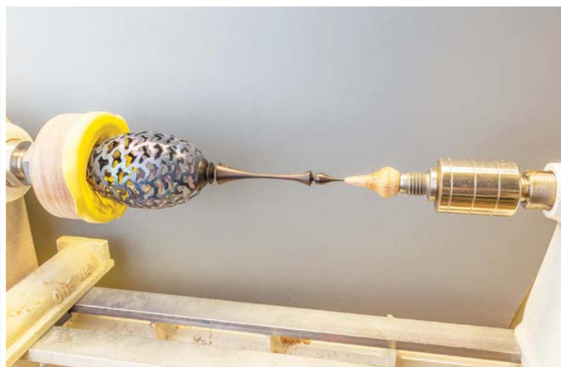
A nicer gluing clamp is hard to find. A pierced and painted goose egg has the finial glued in place and clamped until cured
