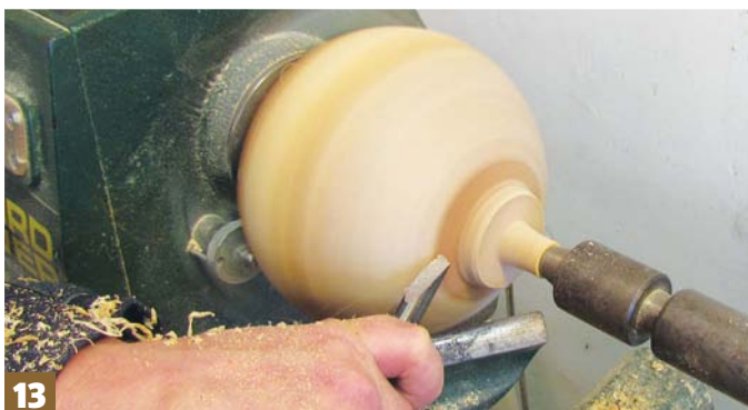
Step 13: refine the surface with the gouge in shear scraping mode, or alternatively, use a standard 25mm square-end scraper
