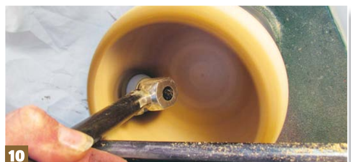
Step 10: due to this bowl being relatively shallow, enough rigidity remained with the walls and the inside and outside was finished after hollowing. For this step, carefully use an inertia sanding arbor with abrasive from 12-320 grit to sand near the rim and bark. For the rims of deeper vessels, finish with abrasive and work down in stages after refining with the gouge and scraper. Forms with voids or excessively uneven rims should be finished with the lathe stationary using a 50-75mm diameter sanding arbor held in a battery powered drill/driver, which was covered in the previous article
