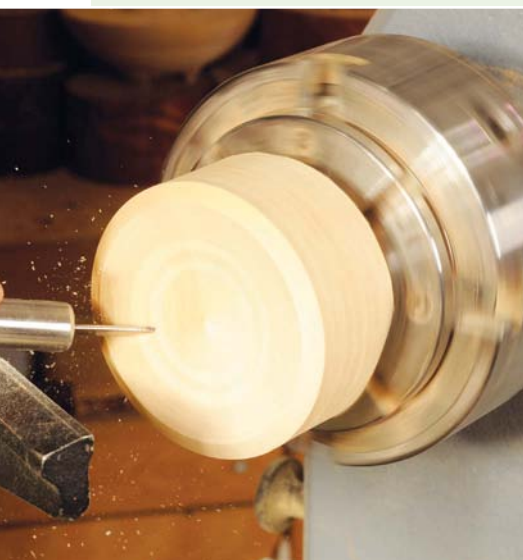
A chatter tool being used to create a chatter effect on dense close-grained hardwood
