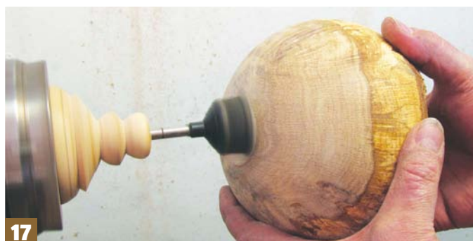
Step 17: finish the base with abrasive on an arbor held in a scrap piece of wood in the chuck
