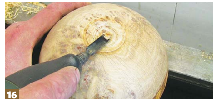
Step 16: refine with a power carver or sharp chisel, working away from your body as you cut
