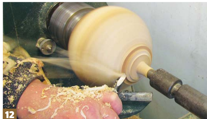
Step 12: using the 10mm bowl gouge, refine the base profile and reduce the waste section and spigot
