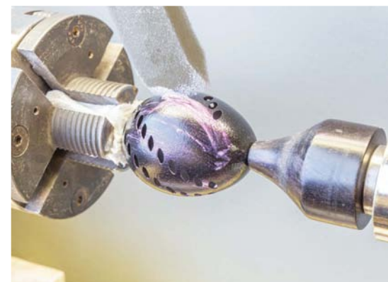
Capable of an incredibly light touch, here a pierced chicken egg is painted and rotated using the handwheel
