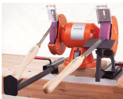
Adjustable arm and table can be used to sharpen various tools
