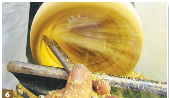
Step 6: start hollowing out the inside with the 10mm bowl gouge to a depth of 50mm. You should keep going until you have cut below the join of the natural-edge and bark
