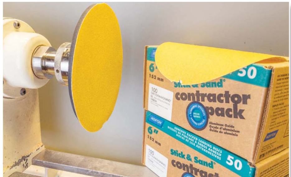
Creating a disc sander is as easy as adding a stiff sanding pad. You can go as large as your swing will allow
