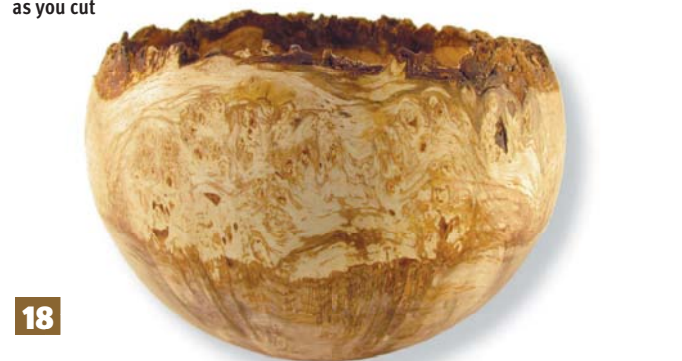
Step 18: apply several coats of finishing oil and wipe away any excess. Set aside in a cool draught-free location for several weeks to season. Weigh with digital scales weekly until the weight stabilises for two weeks, at which point the moisture level will be equal to that of your workshop. Introduce into a cool location in your home to settle. Apply more oil if required or a top coat of your desired wax. Once seasoned, if the bowl rocks, place 180 grit abrasive on a flat surface and place the foot of the bowl onto this, gently twisting back and forth until the bowl is stable ●
