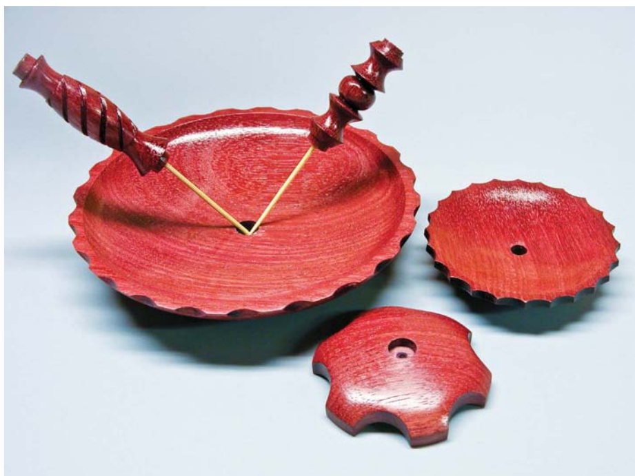
When there is no need for precision, parts can be indexed as needed for sanding, grinding or other processing. The candy dish rim scallops are sanded with an air die grinder
