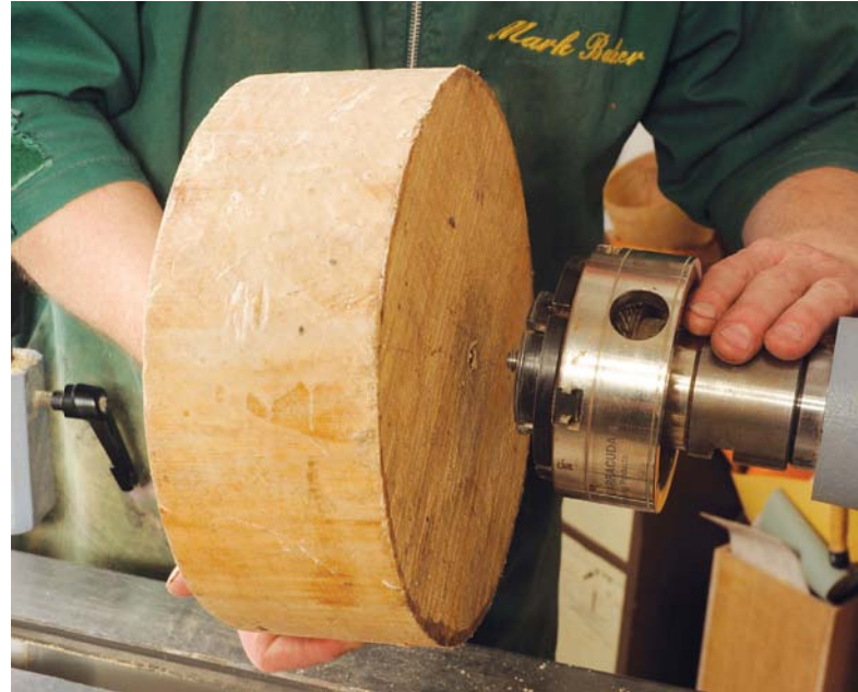
A bowl blank about to be mounted onto a screw held in a chuck
