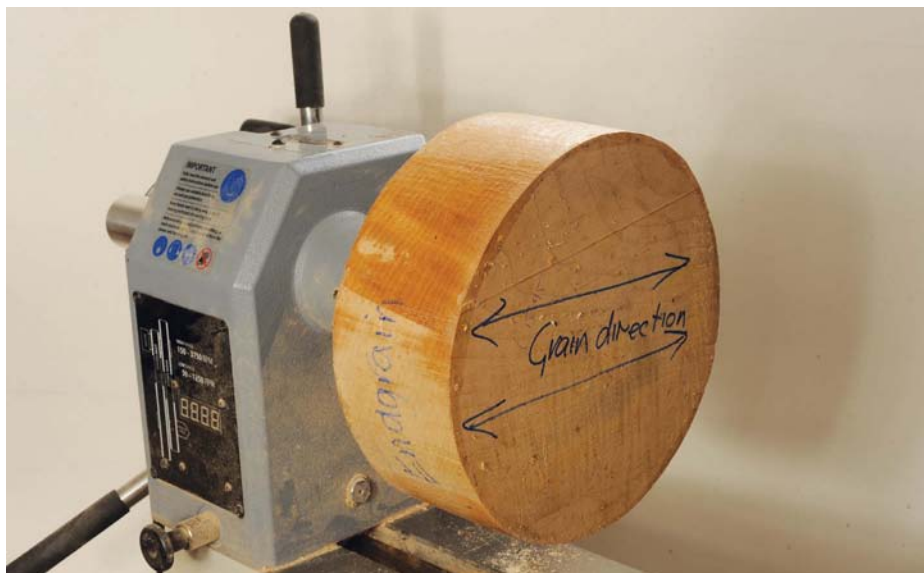
Faceplate blank mounted on the lathe ready for turning
