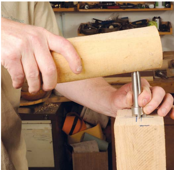
A drive spur being knocked into the centre of a spindle blank
