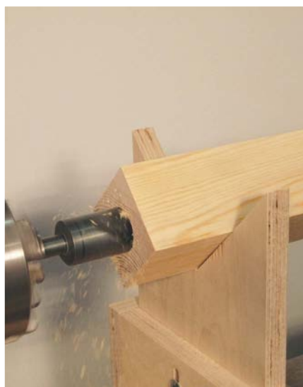
Drilling a long spindle using the pair of cradles for support
