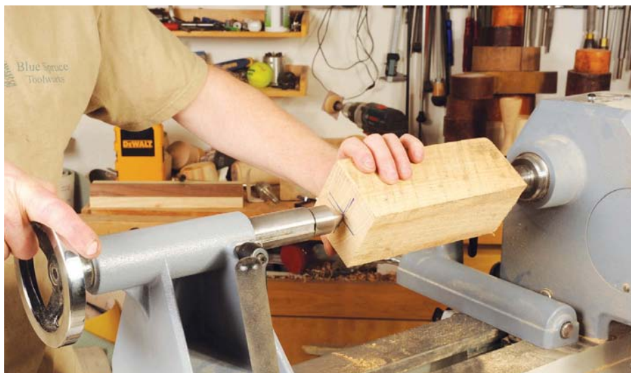
Mounting a spindle project between centres
