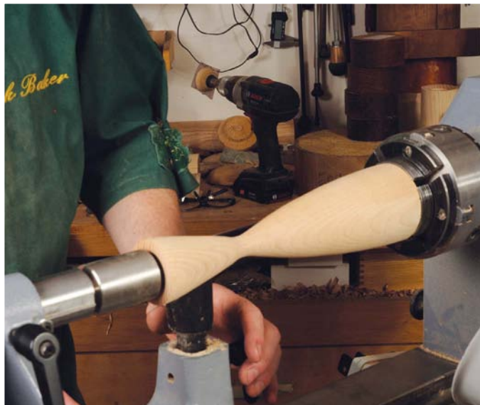
A spindle project: a candlestick held in the chuck via a spigot
