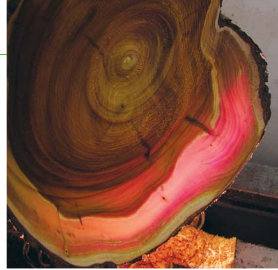
Using a light positioned close to the vessel, which is turned to shine through the wall when it becomes thin
