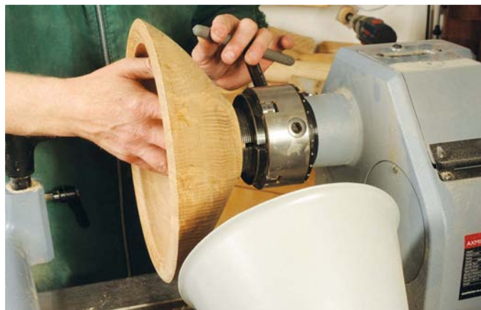
Bowl with a spigot being fitted in the chuck
