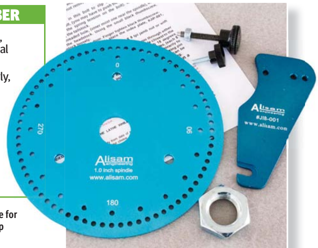
The generic model has even more resolution with holes every 3° and a method of interpolation. The locking pin mechanism is mounted with rare earth magnets
