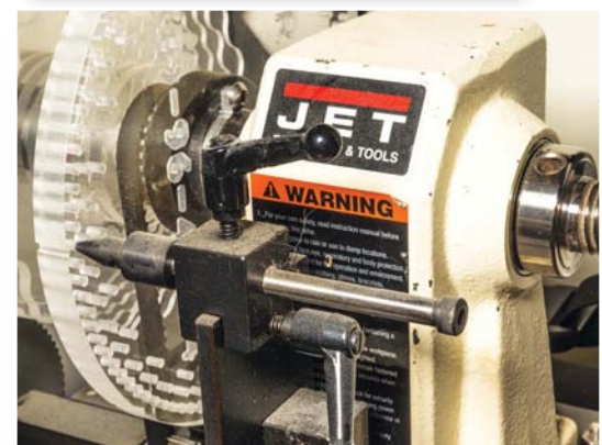
The indexing wheel can be mounted on the inboard or outboard side of the headstock spindle. The locking pin arrangements vary from quite simple to complex
