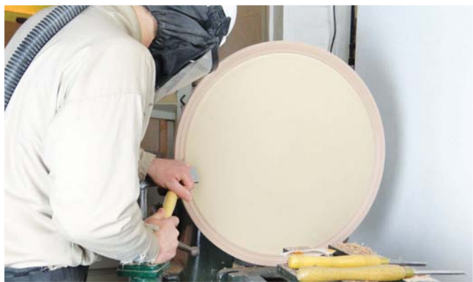
Turning the large moulding
