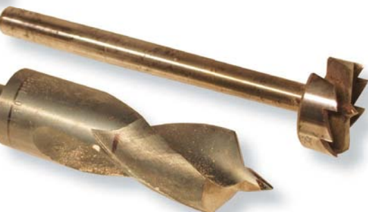
The drill bits used to form a turned mortise and tenon joint
