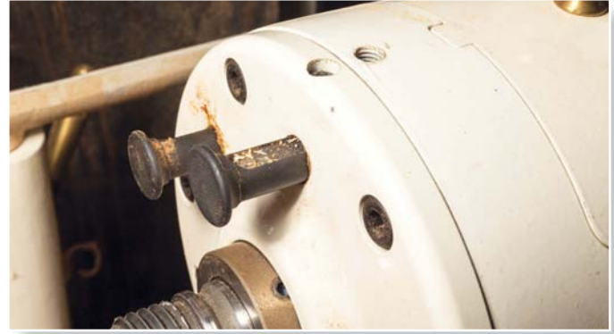
The engagement pins on my lathe represent two different measurement methods. While sturdy and well built, it is good practice to not stress the locking mechanism
