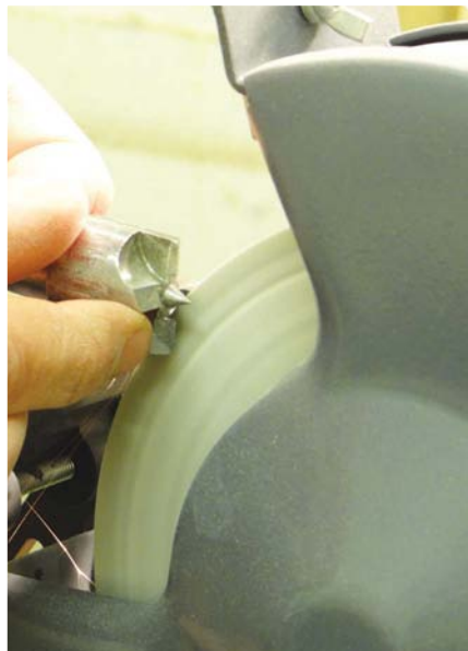
Sharpening a four-prong drive
