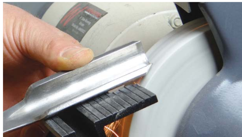
Sharpening my spindle roughing gouge
