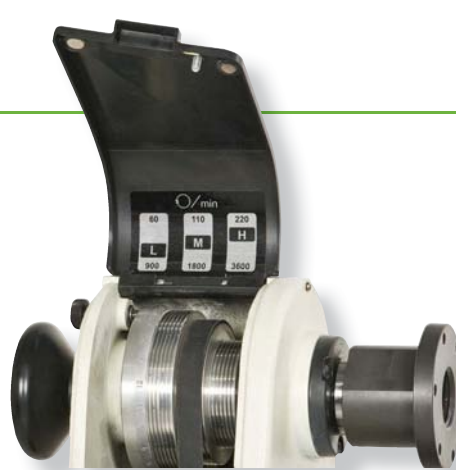
Speed ranges as shown on this three pulley lathe setup
