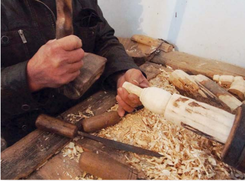
The toolrest doubles up as a mallet for driving a plug into the blank
