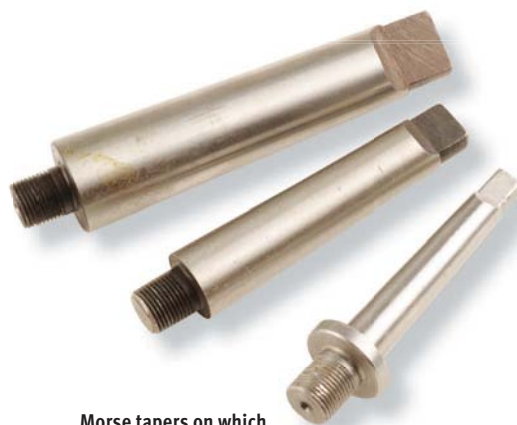
Morse tapers on which can be fitted various types of head
