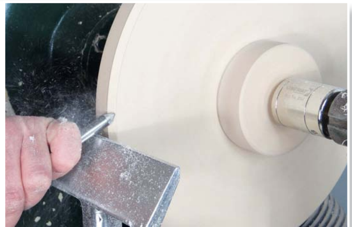
In action, turning the edge detail on a baseboard
