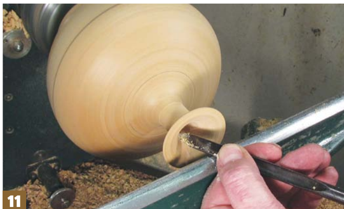
Step 11: blend the inside profile of the neck to the rim using a 6mm spindle gouge and working from inside out, as in step 7. You are working on a glue join here so take small cuts; this will ensure the tool is trailing slightly and is less likely to catch
