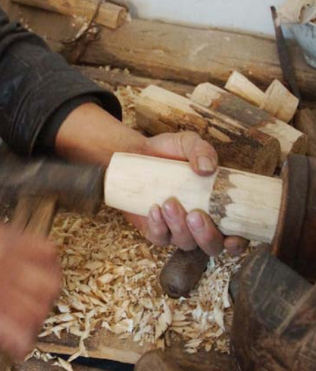
Mr Wang hammers a pre-cut blank into the jam-fit chuck using a hammer
