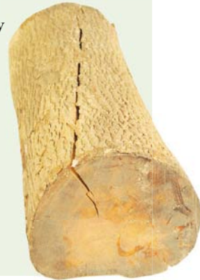
Boxwood ( Buxus sempervirens ) branch section showing a radial crack
