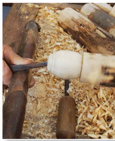
This underhand grip is familiar to traditional turners all over the world
