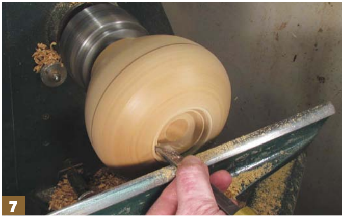
Step 7: using the toe of a 10mm skew chisel set horizontal/trailing on the toolrest, produce a parallel recess 10mm deep to accept the neck previously parted. Check regularly with the neck as you proceed, aiming for a snug fit
