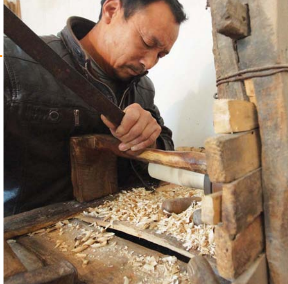
With the toolrest in a horizontal position, Mr. Wang rounds the blank
