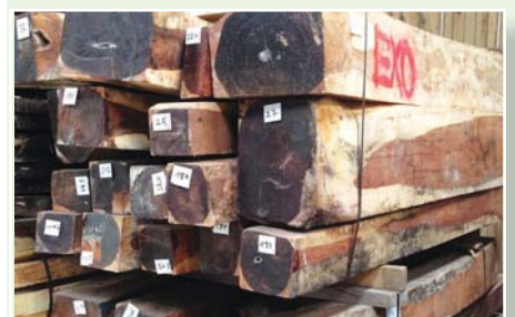
Ring shake on a squared-off log
