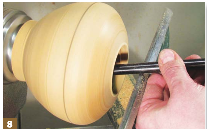
Step 8: hollow out the form using an end grain hollowing tool. Make sure you do not cut away the face within the base of the recess
