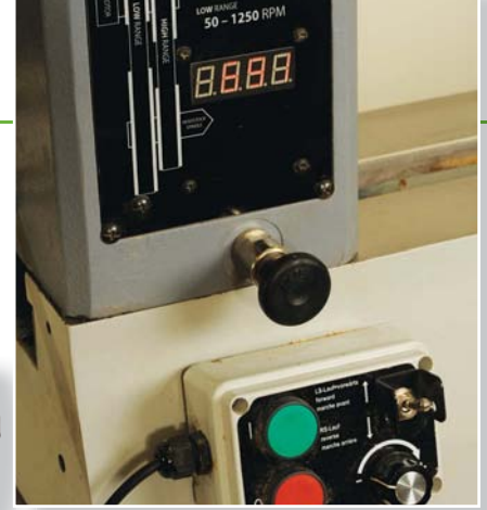
Electronic variable speed control
