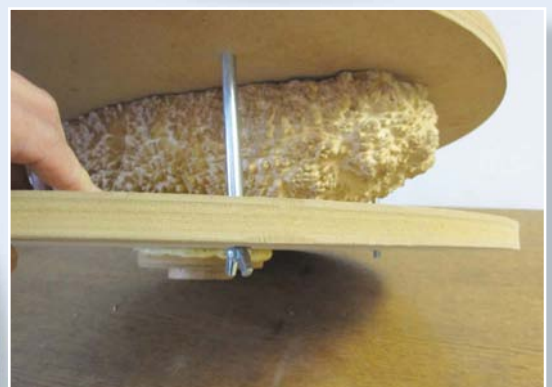
This home-made jig is ideal for holding burls
