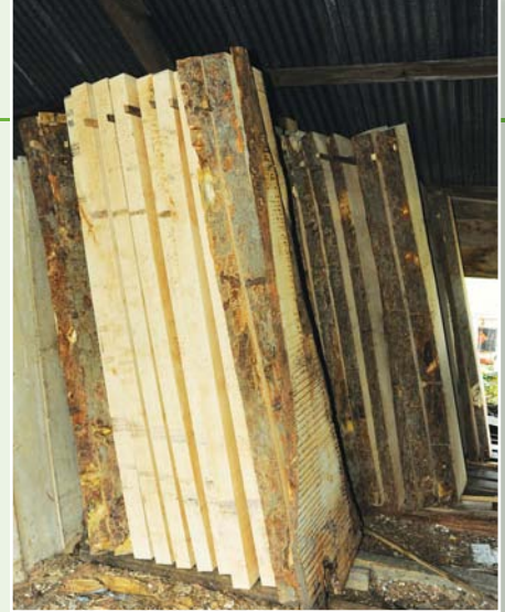
Storing boards vertically instead of horizontally
