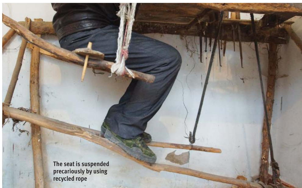
The frame over the lathe was originally secured with wedges, but over the years a quick-fix of wire and nails has sufficed
