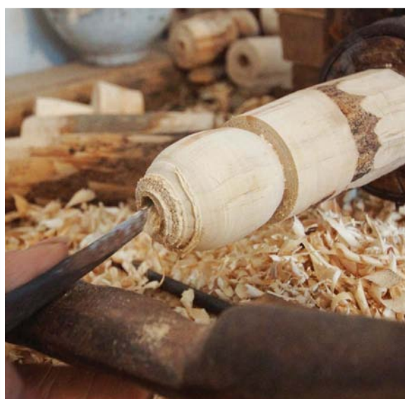
A hook tool is used to hollow out the blank
