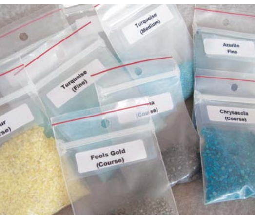
These examples are just a few of the crushed stone fillers that are available. Depending on the material and application, you may need different size particles
