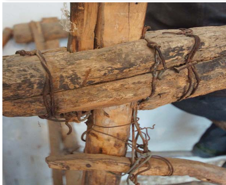
The frame over the lathe was originally secured with wedges, but over the years a quick-fix of wire and nails has sufficed
