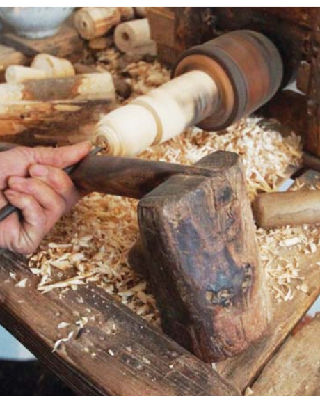
The toolrest is repositioned for hollowing
