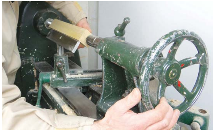
Placing the timber between centres
