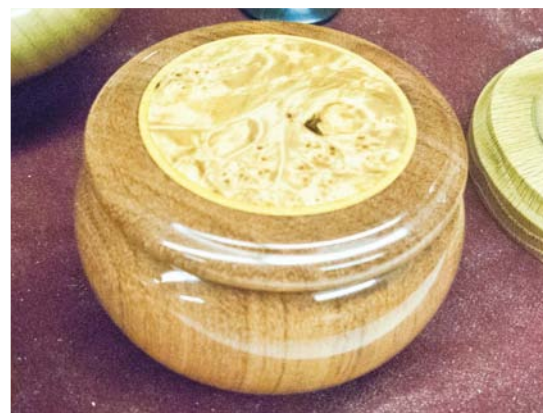
Forgive the alignment error of the top to bottom for grain match. The point of the image is that the burl is more forgiving in the differing expansion rates. It is pretty uniform in all directions
