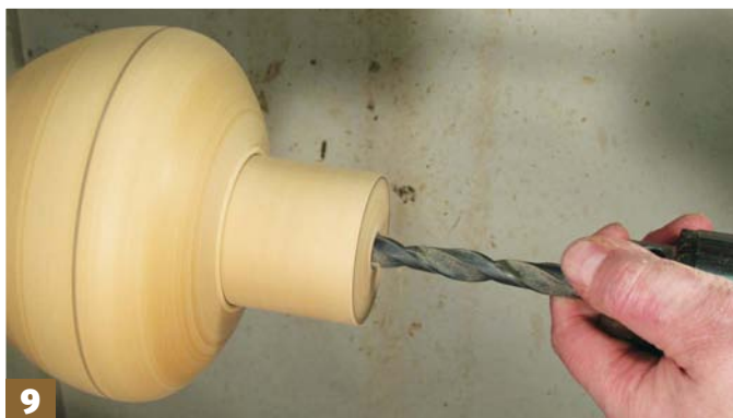
Step 9: apply medium viscosity CA glue into the recess, then line up the pencil lines on the neck and body of the form to align the grain and press the neck into place. Bring up the tailcentre to apply moderate pressure. Once set, drill through the neck into the form with a 12mm drill bit held in a Jacobs chuck
