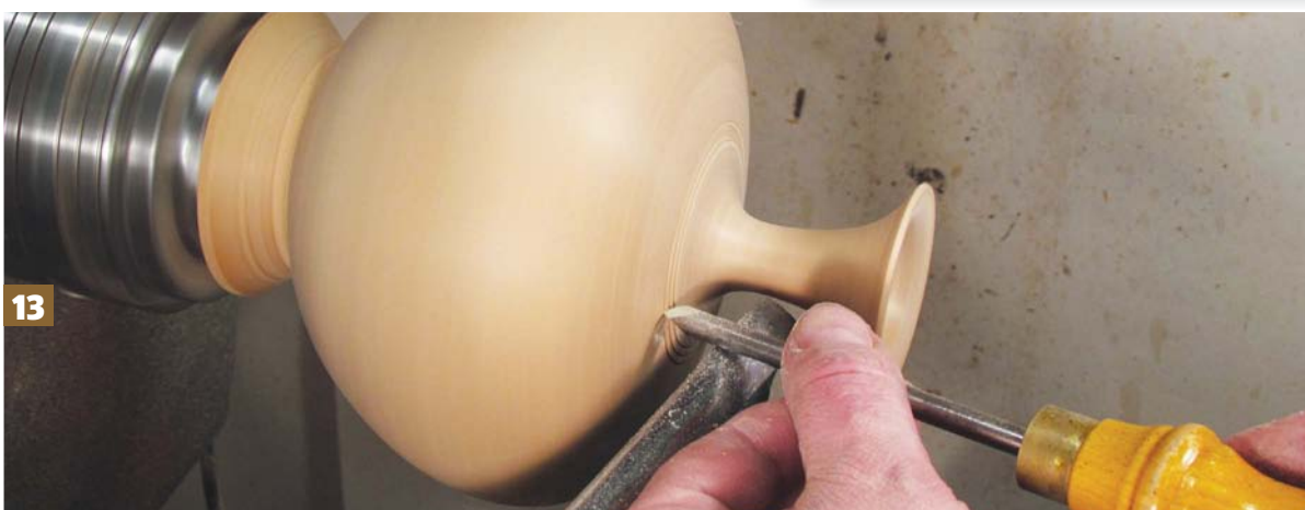
Step 11: blend the inside profile of the neck to the rim using a 6mm spindle gouge and working from inside out, as in step 7. You are working on a glue join here so take small cuts; this will ensure the tool is trailing slightly and is less likely to catch
