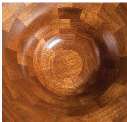
The same species used as a solid bottom. Because of the glue joint it is more forgiving. Another method is to 'float' the bottom piece like a rail and stile door
