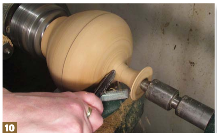
Step 10: using a 10mm spindle gouge, blend the top of the form into the neck producing the neck profile and always working from large diameter to small
