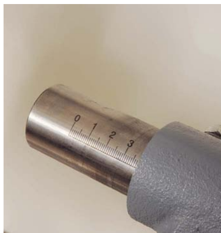
Tailstock quill with rule markings
