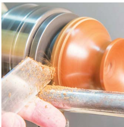
A pocket to receive the dry particles is created in one of a variety of ways. Here the parting tool is used to create parallel channels to be filled with turquoise
