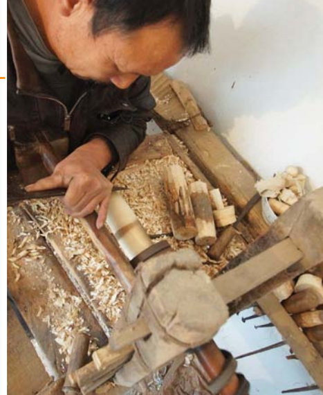
The underhand grip is used in rounding over the end
