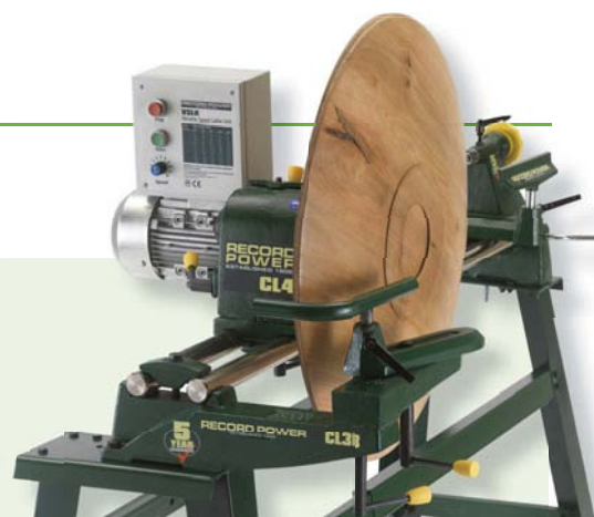
Record Power CL4 lathe with the headstock swivelled and fitted with an outrigger – an optional extra to help with large diameter faceplate work
