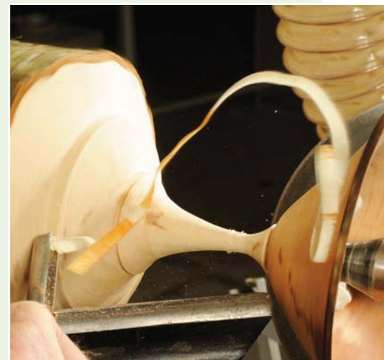
Wet turning a piece producing ribbon-like shavings
