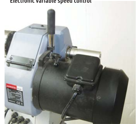
Motor attached to headstock with locking lever assembly
