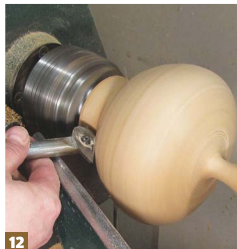
Step 10: using a 10mm spindle gouge, blend the top of the form into the neck producing the neck profile and always working from large diameter to small
