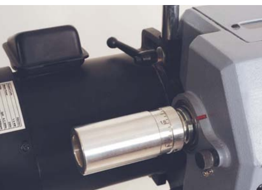
A handwheel with indexing and indent pin
