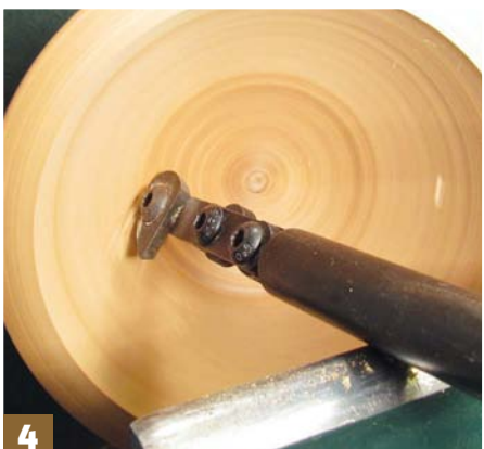
Stage 4: one of many finishing scraper attachments being used at a steep shear angle
