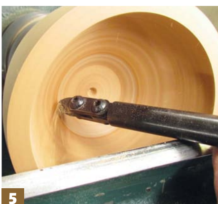
Stage 5: sweep the tool out in a smooth curve from the base into the shoulder
