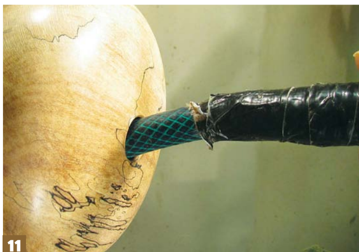
Stage 11: a small home-made attachment can be used to fit a small pipe on a vacuum for smaller openings
