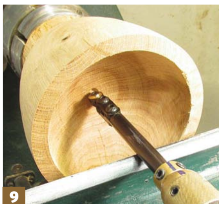
Stage 9: position a locking screw at 12 o'clock and use this mark to monitor the angle of the cutter as you hollow
