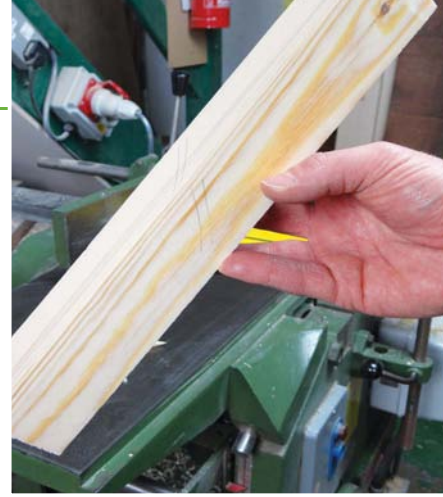
A piece of timber planed with face edges marked, ready for thickening
