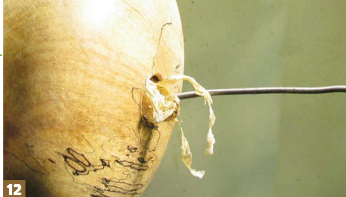
Stage 12: ribbon shavings will have to be pulled out using a bent piece of wire or similar
