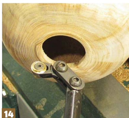
Stage 14: the greater the cutter offset, the greater the twisting forces
