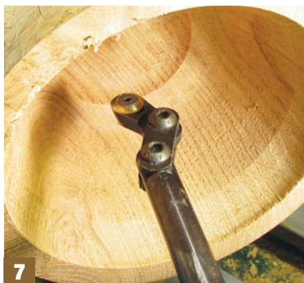
Stage 7: when using an articulated tool, make sure the cutter is positioned in line with the shaft – this will reduce the twisting forces
