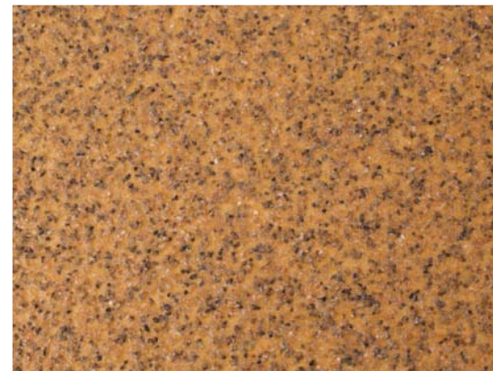
Think of sandpaper as a cutting tool, much like your lathe tools. Each particle of abrasive works the same as your tools
