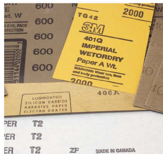
There is a wealth of information printed on the back of the sandpaper including measuring system, grit, backing type, backing weight, manufacturer, abrasive, lubrication and more
