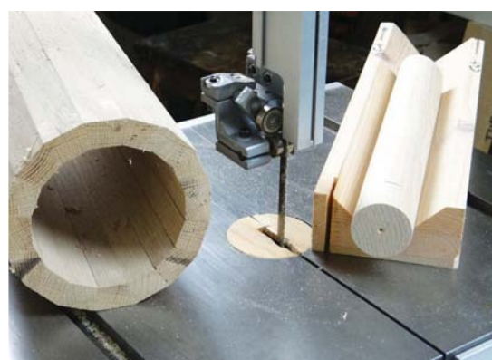
The 'V' shaped cradle I use for supporting round objects
