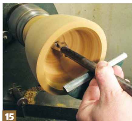
Stage 15: lathes with a swivelling headstock allow better access into the form
