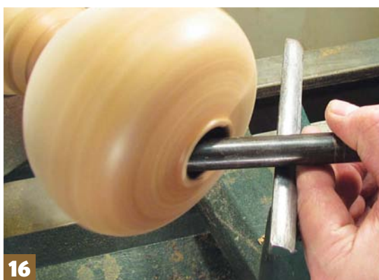
Stage 16: alter the toolrest to maximise support and keep the shaft as perpendicular as possible on the rest
