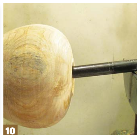
Stage 10: make sure the tool handle trails slightly into the form from the toolrest
