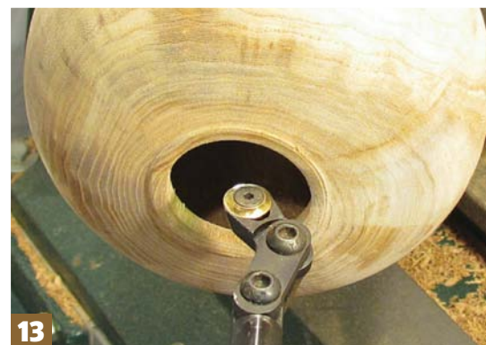
Stage 13: make sure the cutter projects just enough from centreline of the shaft to cut the wood without being excessive
