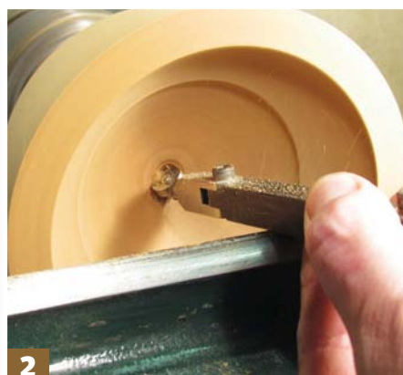
Stage 2: a ring tool being used to hollow out the parallel/end grain form from centre out to the rim
