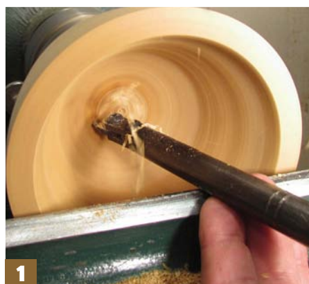
Stage 1: a hollowing tool with a scraping tip cutting within a parallel/end grain form
