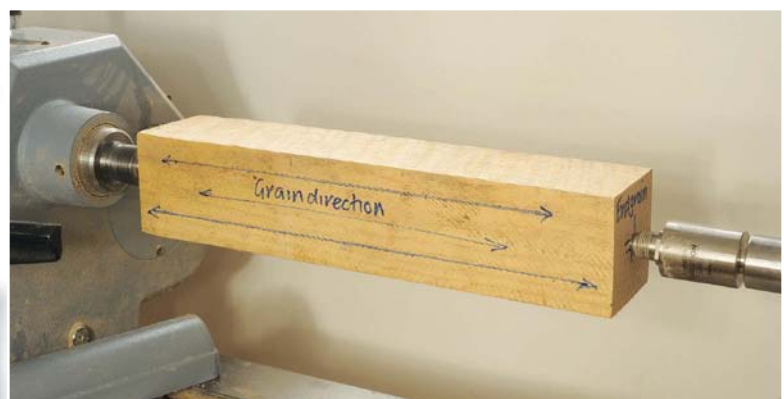
Spindle blank mounted on the lathe – between centres – ready for turning. Arrows denote grain direction
