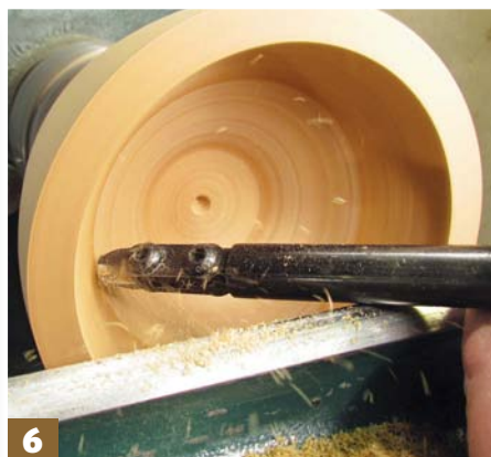
Stage 6: use the tool and toolrest as a fulcrum – this keeps the cut perpendicular to the surface of the wood
