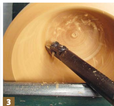
Stage 3: a scraping-type cutter presented at 9 o'clock for maximum material removal
