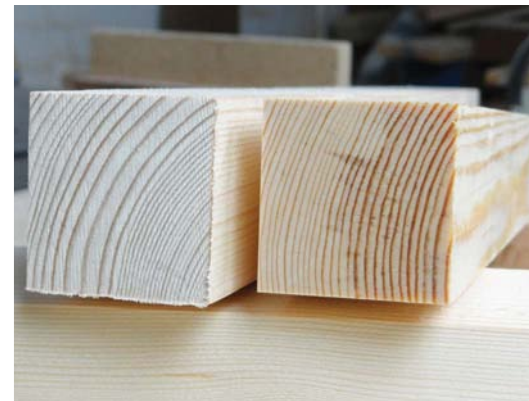
Comparing a bandsaw cut and a circular saw cut on end grain
