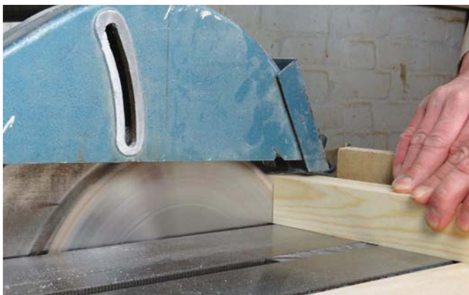
Ripping on the saw bench
