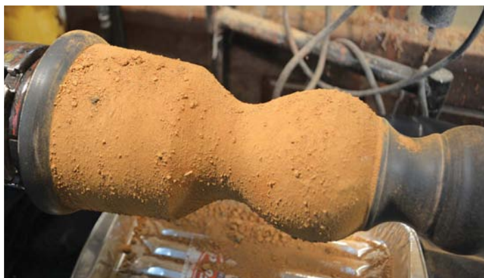
Step 4: smothering the wet paint in dry clay
