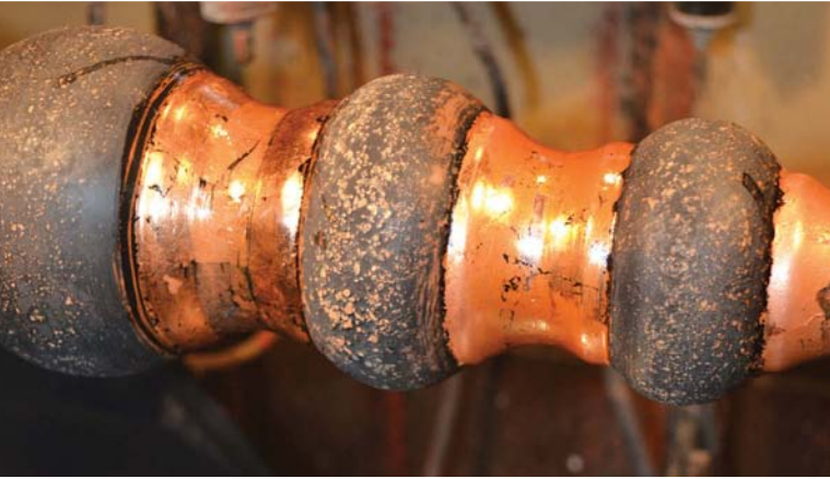
Step 10: applying the gilding size
