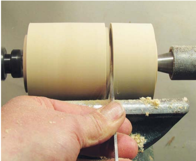
Step 3: using a 2mm parting tool, part in just left of the right shoulder to leave 5mm waste in the centre of the blank. Open out the groove as you proceed to stop the tool from binding by parting in at stages of 6mm. Withdraw the tool, move over to the left and part in past the previous cut by 6mm. Remove the tool and part in again at the first cut deeper again, continuing back and forth until you reach the correct depth
