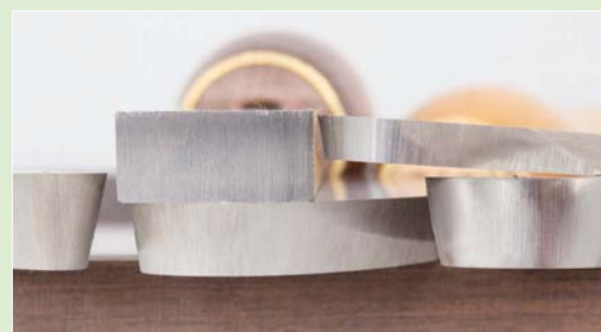
The advantage of the Sorby ProEdge and Tormek is their ability to deliver finely ground edges. Take a look at 60, 200, 1,200 and a mix or 60 and 1,000. The time and investment cost difference is your call
