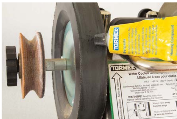
Both the Sorby and the Tormek offer buffing or honing. More applicable to the skew chisel than other turning tools, a cotton wheel with jeweller's rouge or leather stop with honing compound is used
