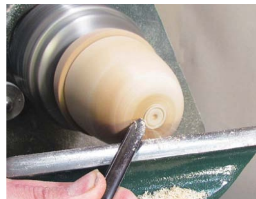
Step 19: jam the base over a jam chuck made from waste wood, placing kitchen towel between to protect the internal finish. Using a 6mm spindle gouge, refine the base profile, working down towards the base. Finally, concave the base so the box will sit stable in use. Finish and blend with 120-400 grit, using your chosen finish as before...
