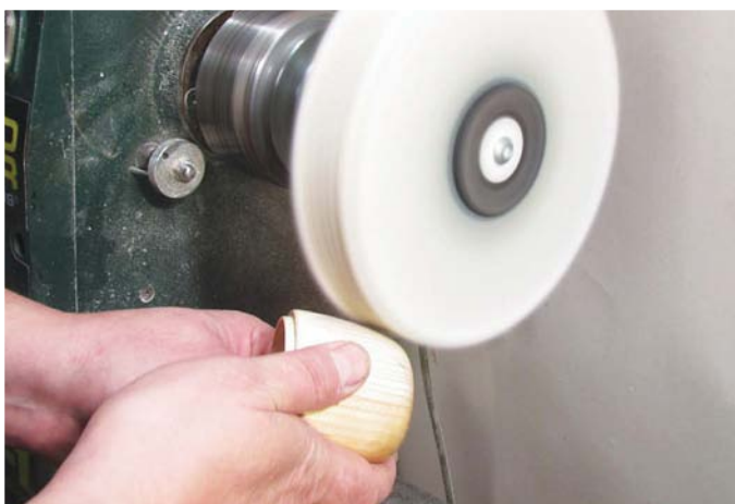
Step 20: ... alternatively, the finish can be applied off the lathe and buffed with a buffing system, as shown here
