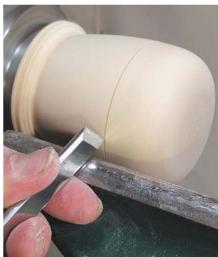
Step 18: using the toe of a skew chisel, produce a small groove straddling the join. Finally, finish the box lid and body as before with abrasive and sanding sealer
