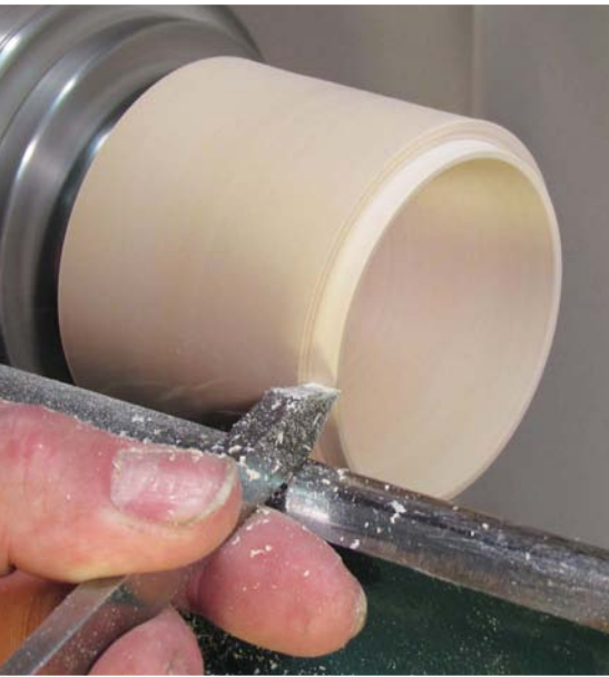
Step 14: refine the spigot using a 6mm parting tool, taking fine cuts. Check the fit with the lid until you have a fit too tight for everyday use. Finally, finish the inside of the box from 120-320 grit
