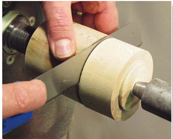
Step 4: stop the lathe and cut through the remaining waste with a fine blade saw
