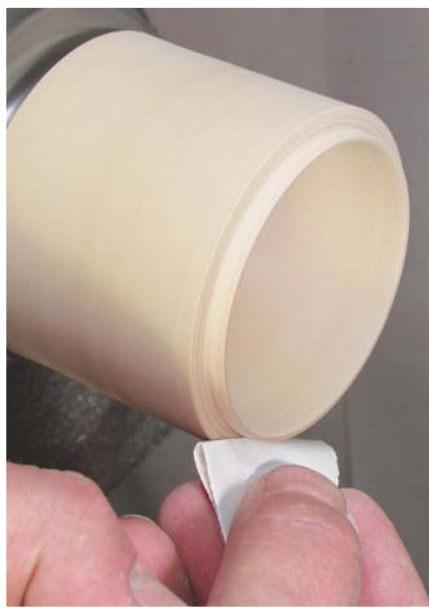
Step 15: using 240-320 grit abrasive, finish the spigot continually checking with the lid until you have achieved a snug fit. Finish the inside with sanding sealer and buff as before
