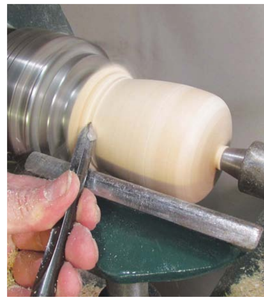
Step 16: place a piece of kitchen towel between the base and lid, jamming the lid on. Bring the tailcentre up for extra security and profile the external shape using a 10mm spindle gouge, working downhill to a safe distance from the chuck and tailcentre as shown in Fig.C
