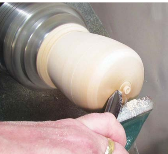
Step 17: remove the tailcentre and remove the remaining waste with the spindle gouge. Make sure you gently rub the bevel on the face of the lid prior to starting the cut
