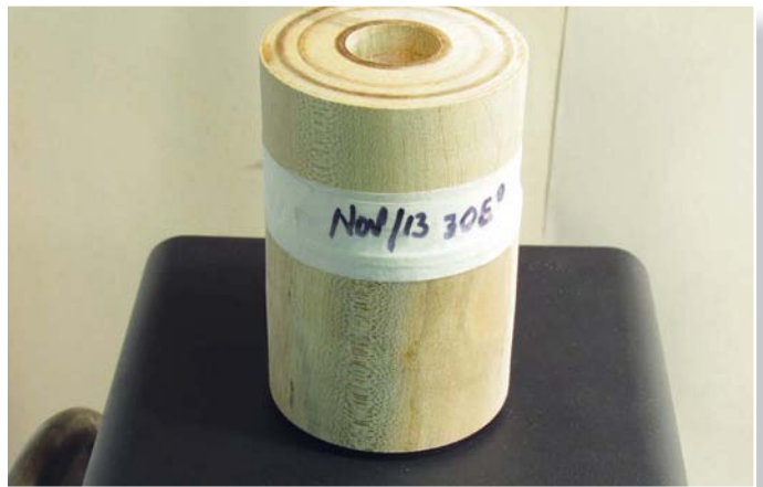
Step 6: tape together with masking tape so that the drilled sections are facing outwards. Weigh the item and write the date, species and weight on the tape. Store and monitor as previously discussed in 'processing wood'. Part-seasoned wood can be left unsealed, depending upon your region and time of year. If the climate is hot and dry, then it is best to seal the end grain as a precaution
