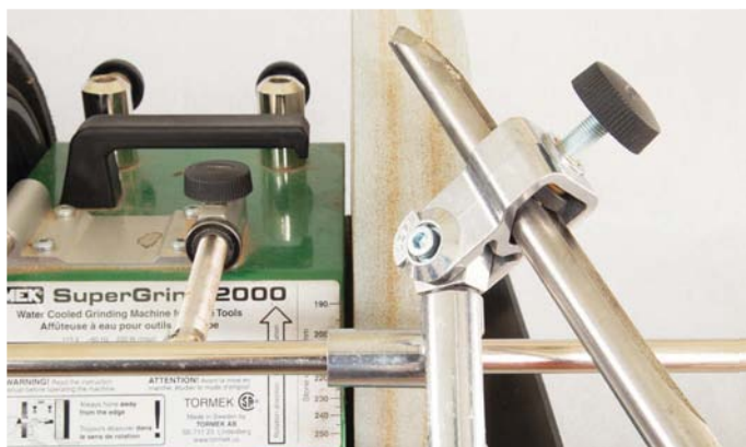
The Irish grind is possible using the Tormek jig. Once the user finds their favourite, the extension in the jig and guide-bar measurements are recorded and used over and over. It takes some easy measurement
