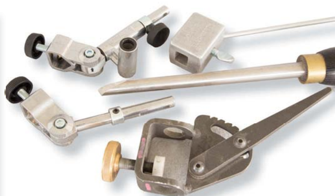
All of the bowl grind jigs work similarly. The tool extension, the angle setting when available and the jig pivot point all interact to create the nose angle, sweep length and sweep contour
