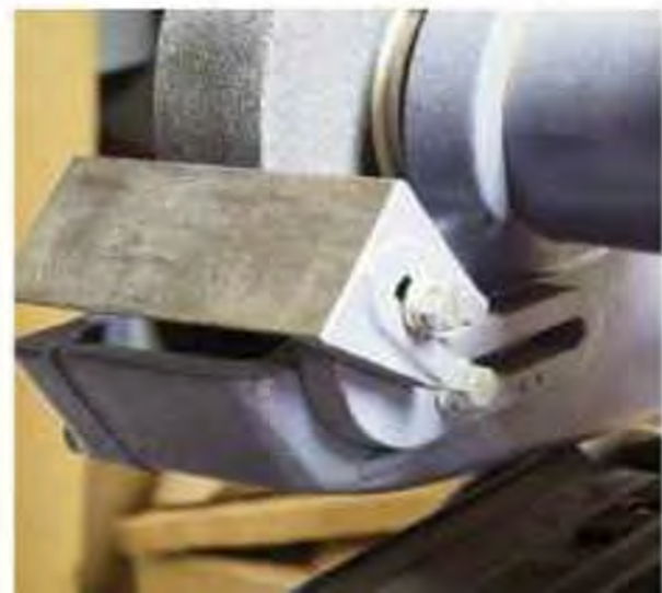
Regardless of the rests that are installed on the grinder, a sharpening system benefits from having an after-market grinding fixture system. This accommodates those special needs effectively.
