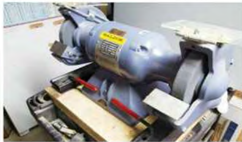
Regardless of the rests that are installed on the grinder, a sharpening system benefits from having an after-market grinding fixture system. This accommodates those special needs effectively.
