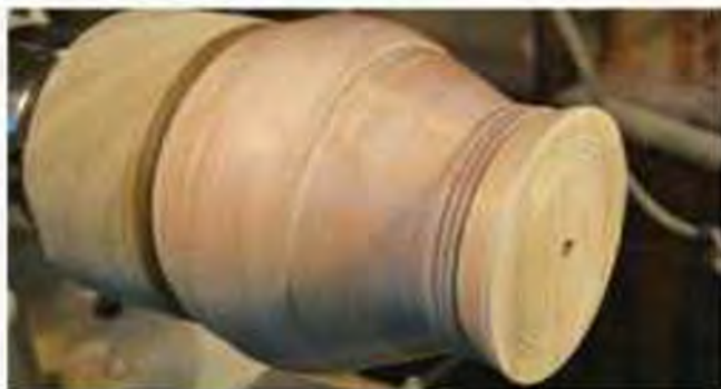
The piece placed on a fabricated jam chuck
