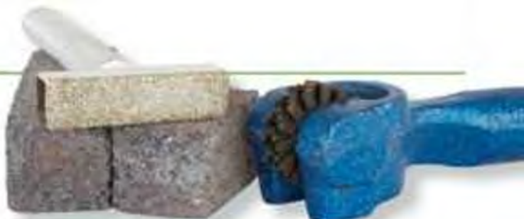
Wheel dressers from old to new. The 'devil stick' – lower left – is from another time – with the star wheels – right – not far behind. The most modern and effective diamond dresser is in the upper left
