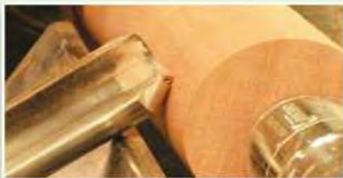
Presenting the tool to the wood to make a cut, rotating the wood by hand
