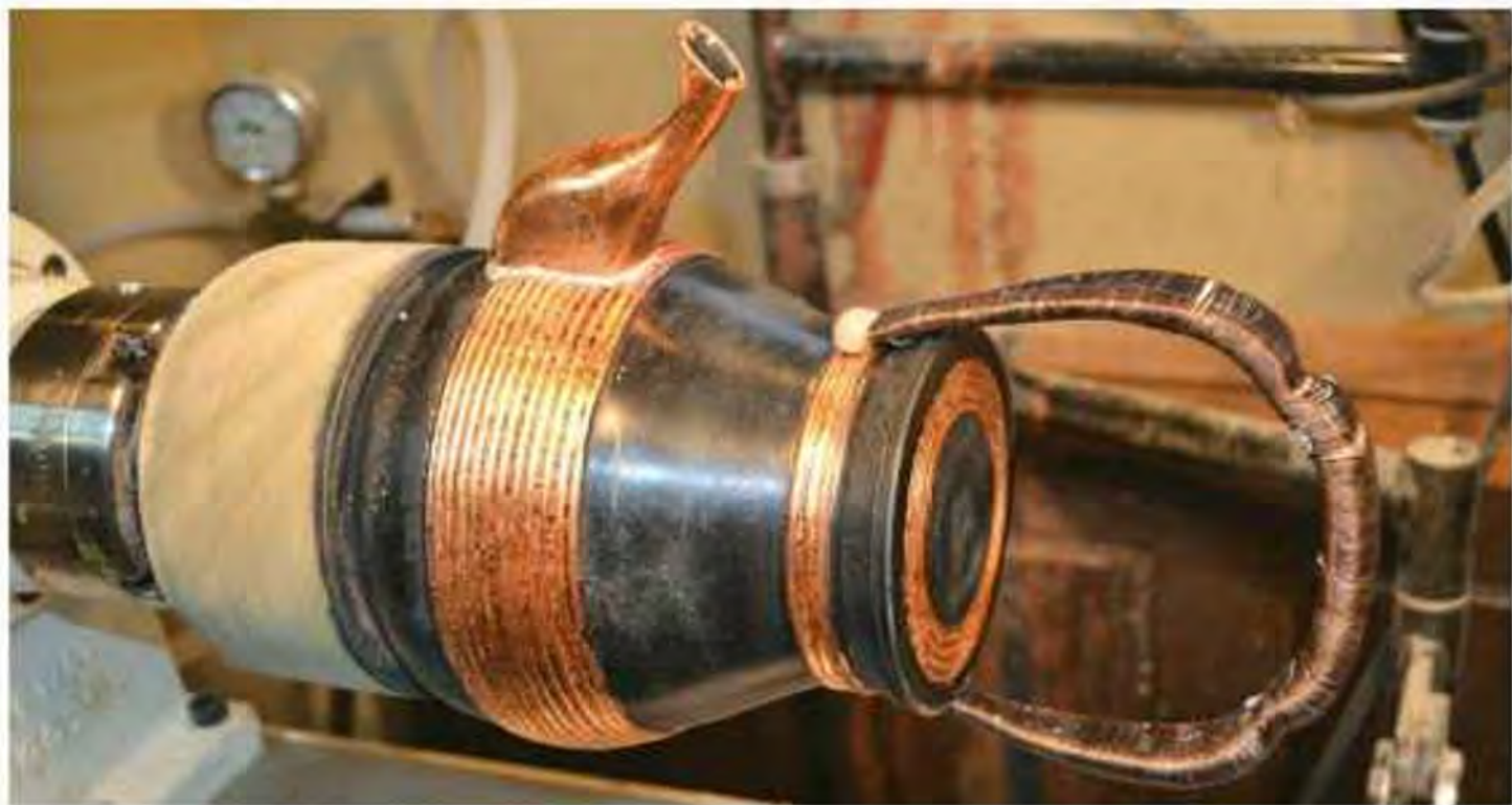
Applying copper leaf to the beading
