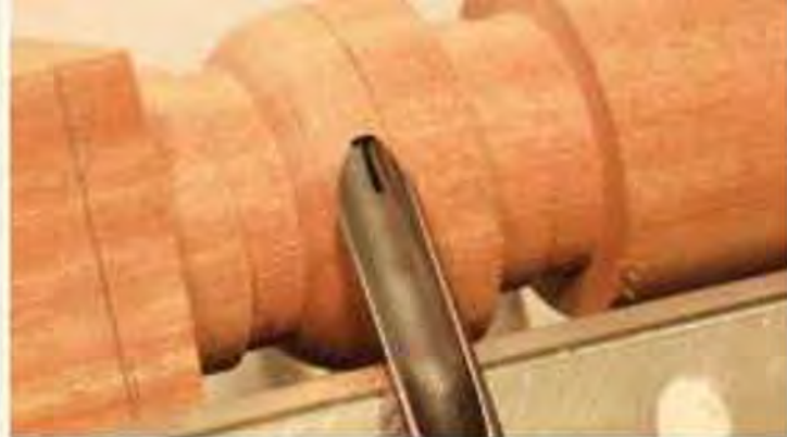
This photo shows the area on the tip of the tool that is being used
