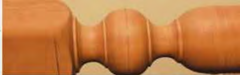
Finished bead and cove combination, including the curved pommel, all cut with the spindle gouge
