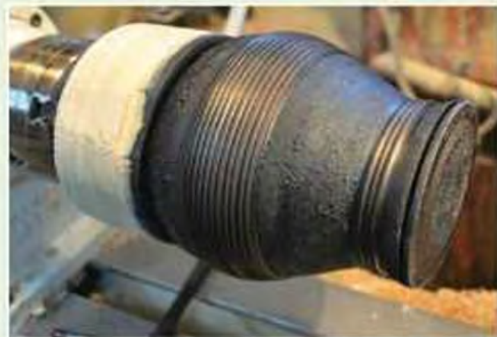
Building up layers of glaze mixed from spar varnish and black paint...
