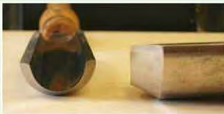
The profiles of my spindle roughing gouges
