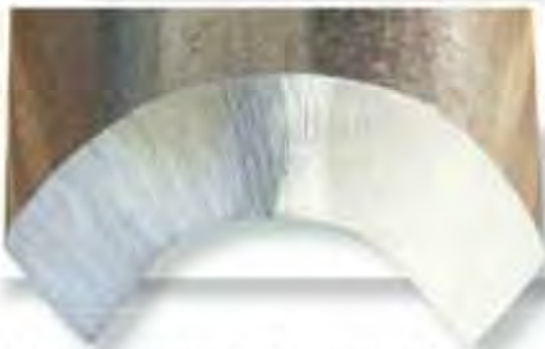
Grit selection is a balance of steel removal capability and fineness of ground edge. A look at the end of the tool will tell what grit grinding wheel was used.
