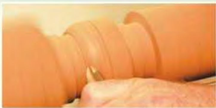
The bead being fully finished
