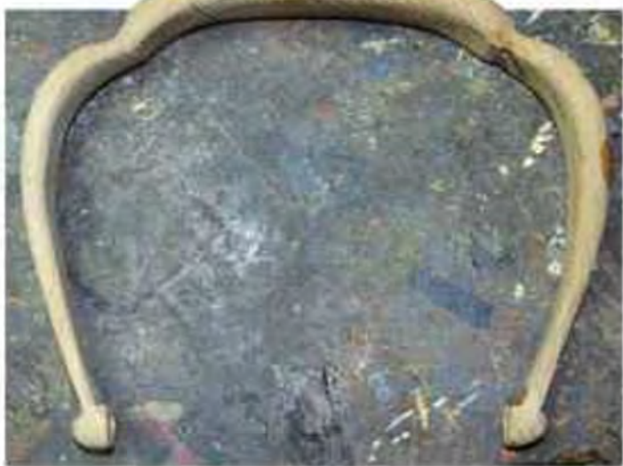
The handle, once cut out on the bandsaw and carved.
