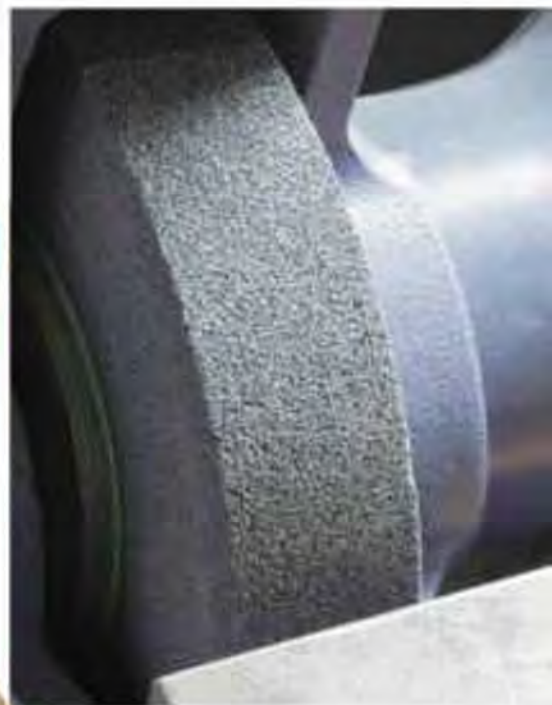
A properly dressed wheel will be flat across the face with the colour being 'dull'. The absence of shiny spots, embedded steel and the dullness indicates fresh sharp cutting particles ready to work
