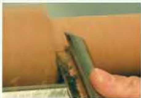
The spindle roughing gouge on its side, working up to the pommel
