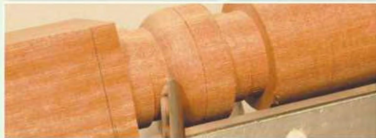
TOP TO BOTTOM: Here you can see the flute position as the cut progresses
