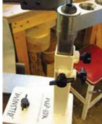
The rear assembly with comprehensive height adjustment locking nuts
