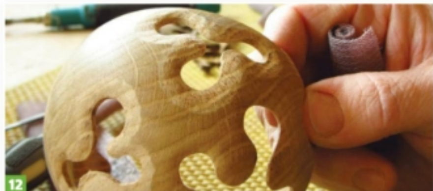
Here you can see the difference between the shaped and sanded areas
