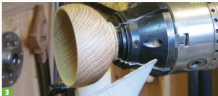
The interior of the bowl was then sanded and finished with lacquer, to give a glossy finish
