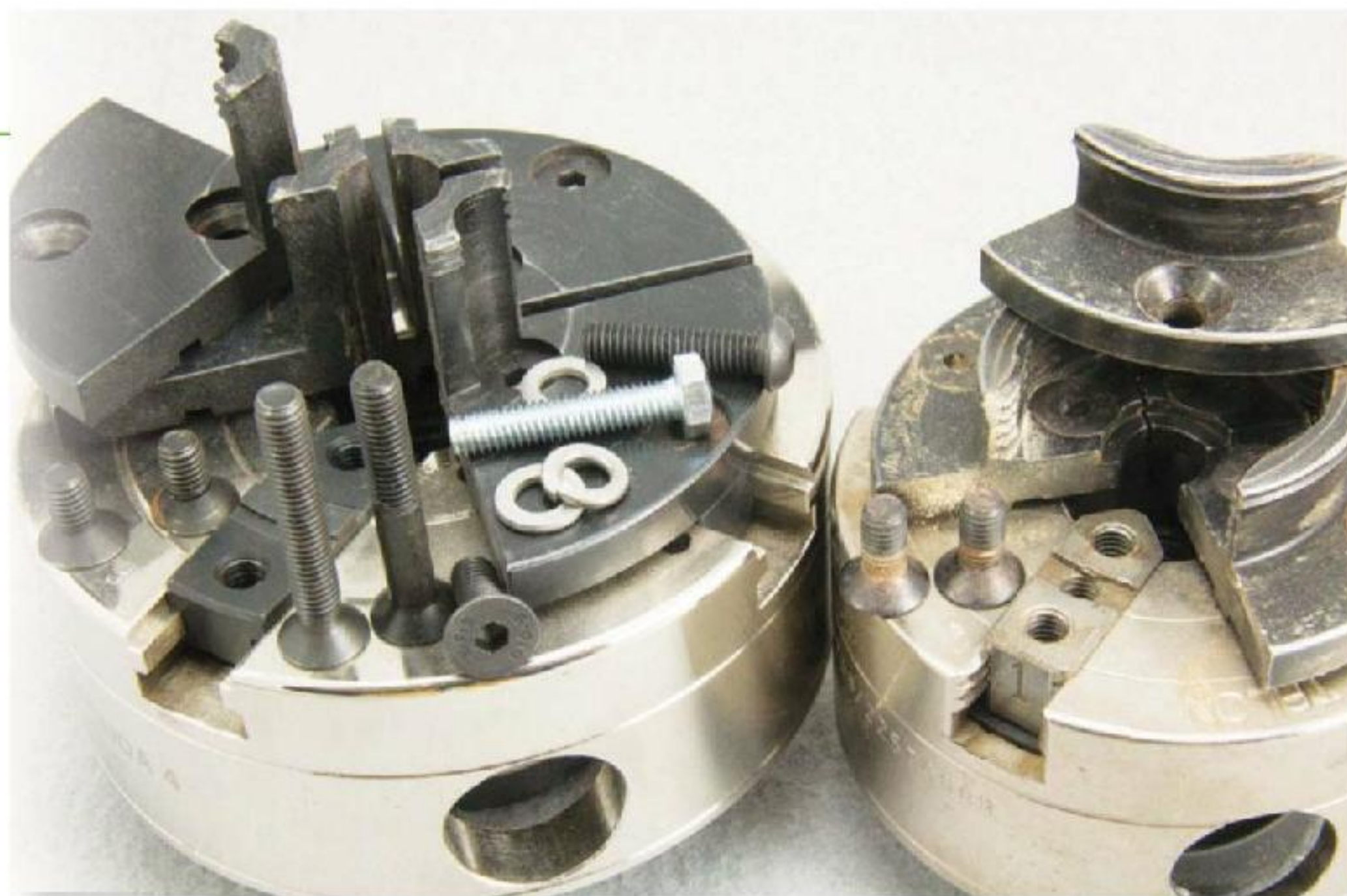
If you venture into the area of wooden jaws and custom made interfaces for your chuck, be certain you have the correct and proper strength fasteners. An assortment of 6mm fasteners shown
