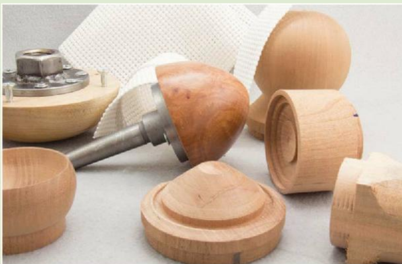
Headstock creations allow you to make those custom drives that help solve your workholding problems. Low cost, easily made, and tuned to fit, take advantage of the creative possibilities
