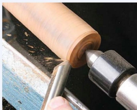
ABOVE: Making a spigot on the middle spindle
