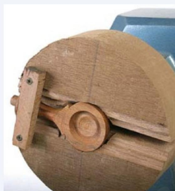
ABOVE: Held in the wood jaws while turning the first side of the handle
