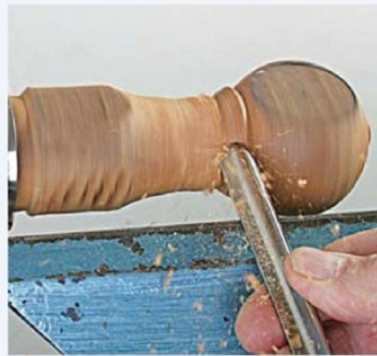
ABOVE: Shaping the stem with the shallow fluted gouge
