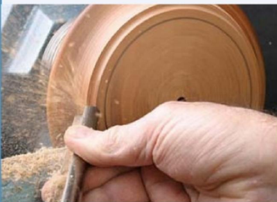
ABOVE: Shaping the rim with the deep fluted gouge
