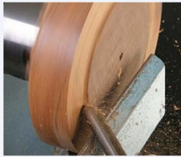
ABOVE: Trimming the top face of the discs with the deep fluted gouge
