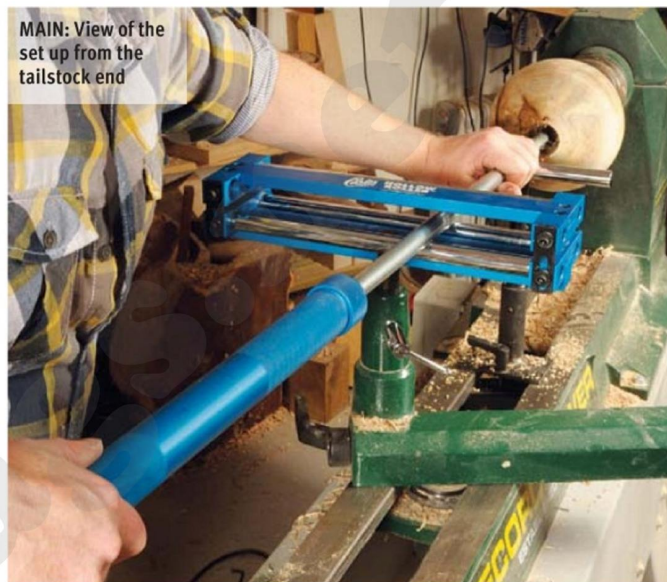
MAIN: The tip can be set to any angle required to reach the work
