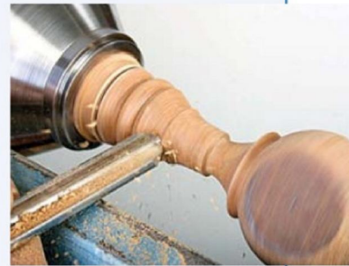
ABOVE: Finishing the spindle shape with the deep fluted gouge
