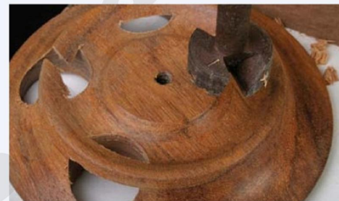
ABOVE: Stopping the drilling early will avoid damaging the feet
