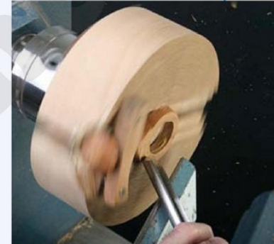
ABOVE: Turning the second face of the egg stand's handle with the deep fluted gouge
