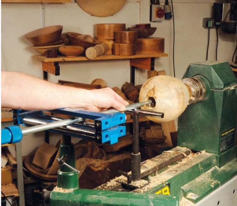
ABOVE: Side view showing how everything is supported
