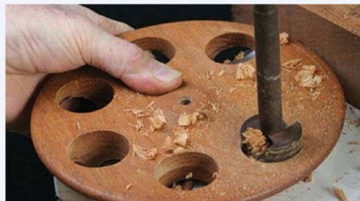
ABOVE: Drilling the holes for the eggs on a pillar drill
