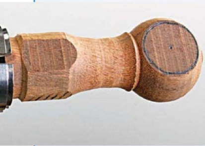
ABOVE: A circle drawn on the flat area helps to visualise turning the end spherical
