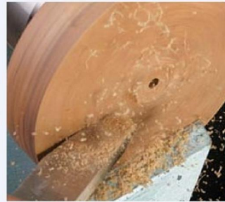
ABOVE: Refining the top surface of the discs with a large left-hand, curved side-cut scraper
