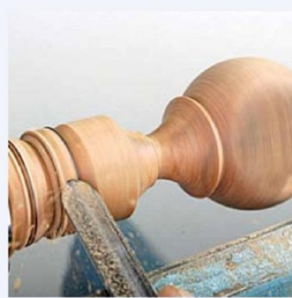
ABOVE: Rolling the bead with the shallow fluted gouge
