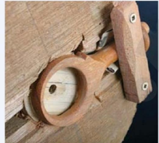
ABOVE: Held in the wood jaws to turn the second side of the handle. Note the disc inserted behind the handle and the paper behind the stem; this helps to position it correctly
