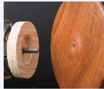
ABOVE: Reversing the disc with a recess spacer; this will make the disc stable
