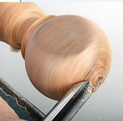
ABOVE: Removing the mark left by the tailcentre
