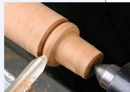
ABOVE: Rolling the bead with the shallow fluted gouge
