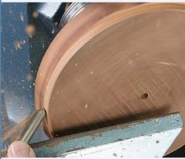
ABOVE: Trimming the rim of the discs with the deep fluted gouge
