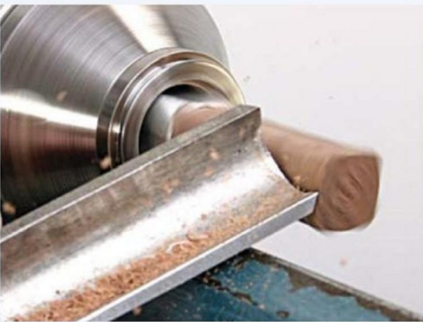
ABOVE: Individual pawn being shaped with the spindle roughing gouge
