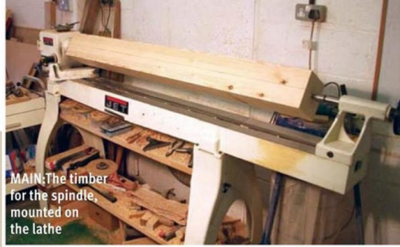
MAIN: The spindle mounted on the lathe with the barley twists marked, ready for carving
