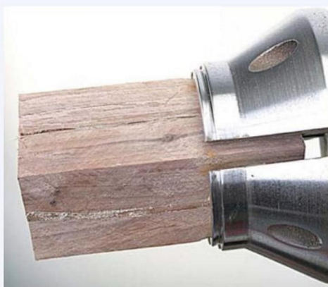
ABOVE: Four pieces fixed together with double-sided tape, held in 50mm (2in) O'Donnell Jaws
