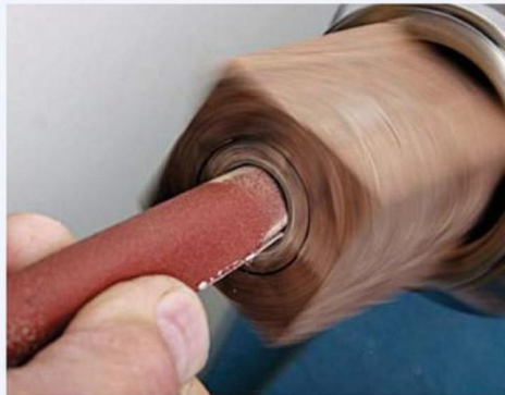
ABOVE: Sanding the inside of the hollow
