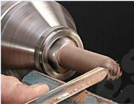
ABOVE: Rounding the end of the pawn with the shallow fluted gouge
