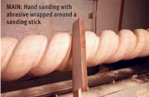
MAIN: Hand sanding the spindle with abrasives
