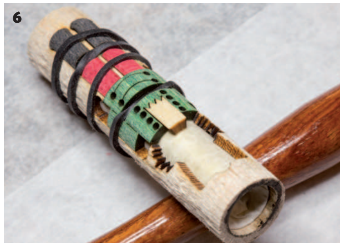
6 Lightly tack the pieces in place with CA as you go. Use the provided rubber bands to help position and hold the pieces as needed
