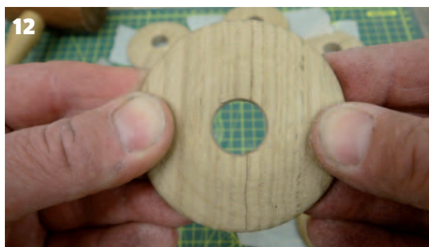
10 Turning the pipe covers 11 The cover deliberately snapped along the grain 12 Pressed back together, the join is virtually invisible
