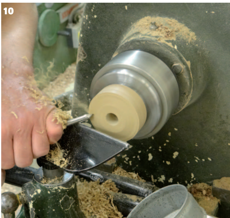
10 Turning the pipe covers 11 The cover deliberately snapped along the grain 12 Pressed back together, the join is virtually invisible
