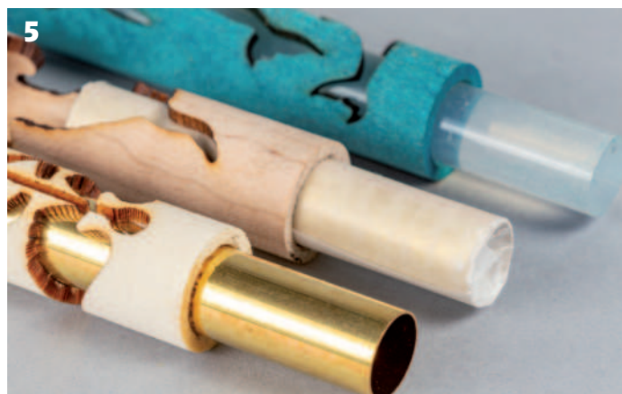
5 Rather than use the raw brass tube as your depth control device, wrap it in waxed paper or use the available silicone assembly dowel
