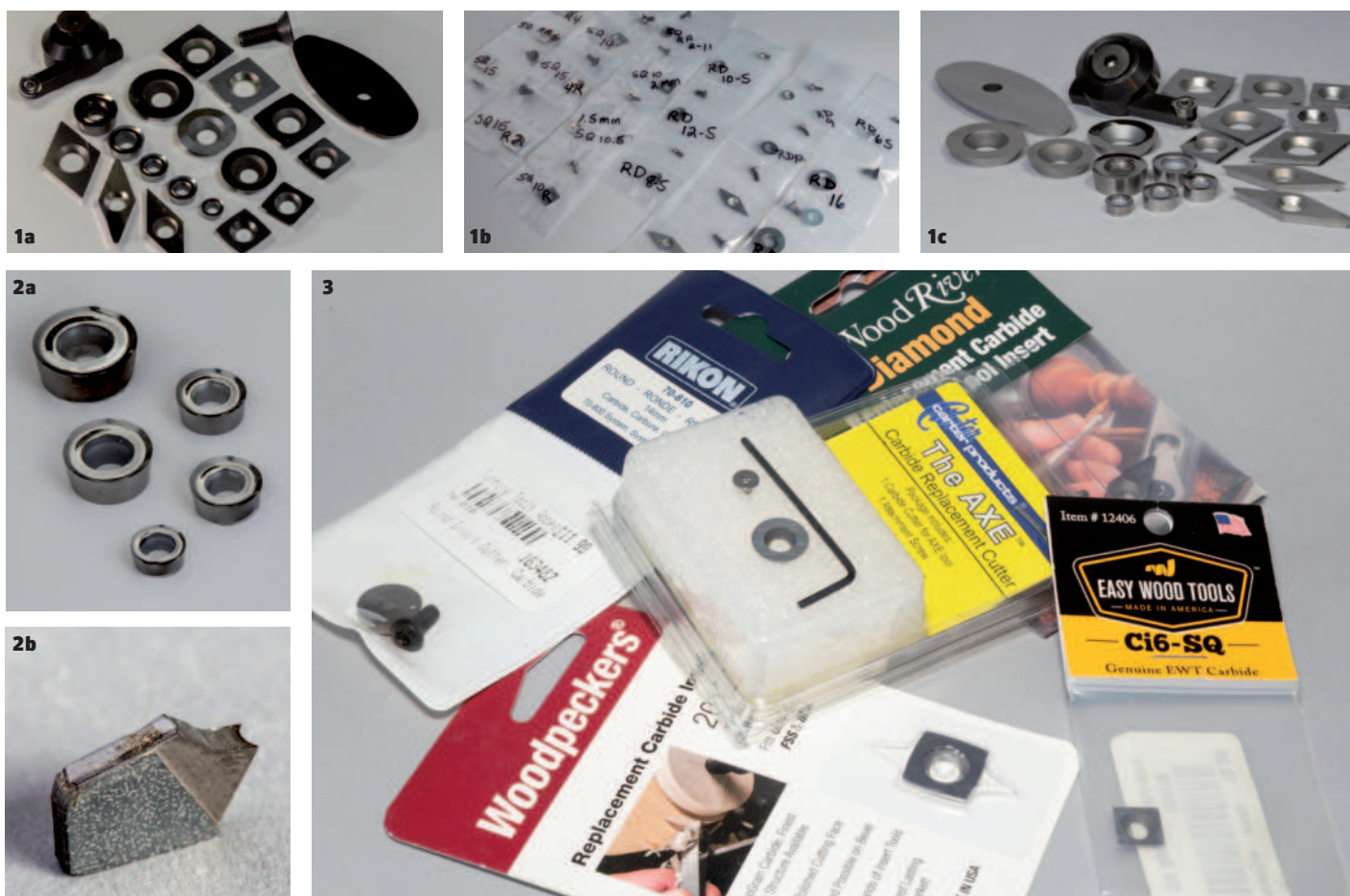
1 Just a small sample of the various carbide replacements available. You need to be certain any replacement nests like the original. 2 The design and fabrication of the carbide cutters is far more complex than perhaps you give it credit. 3 Retail packaging adds cost to your product. It can vary from the simple poly bag to more exotic visual or theft resistant.
