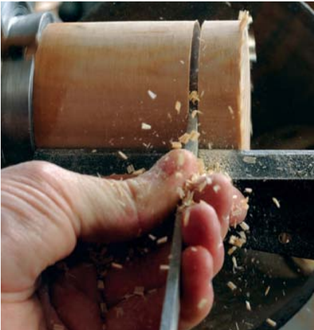
A parting cut can be made all the way through or stopped to create what is known as a fillet
