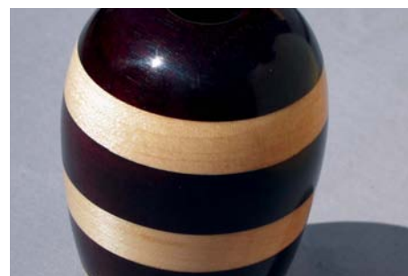
The purpleheart was cut into 75mm square pieces and glued up with maple ( Acer saccharum ) and turned into a hollow form
