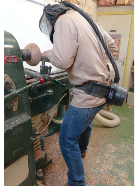
My end position when turning the inside of a bowl – notice my feet haven't moved, but my weight is now over my left leg, which allows full body movement while maintaining balance
