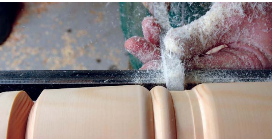
A plunge cut without the bevel rubbing works well but the surface is not as clean as with the bevel rubbing
