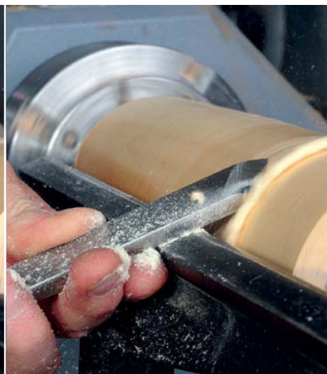
Raise the handle until the cutting edge is on contact
