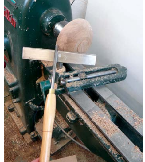
The finish point, turning the base of the bowl – notice how far the handle has had to swing to produce the simple curve on this bowl
