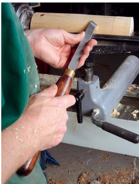
The body support is vital for full control
