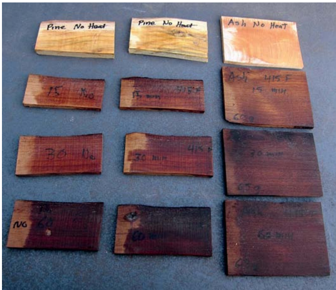
10mm-thick pine and ash ( Faxinus excelsior ) wood heated to 213°C for 0, 15, 30 or 60 minutes
