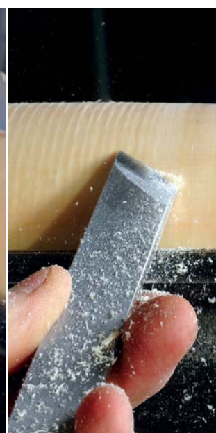
Different cutting angles create varying degrees of finesse on the surface
