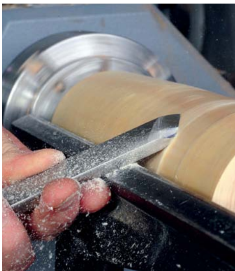
Only cut on the lower half of the blade for full cutting edge support
