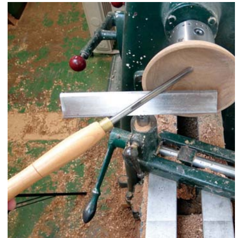
The end point turning the inside of a bowl – again notice the amount of handle movement required to produce the curve
