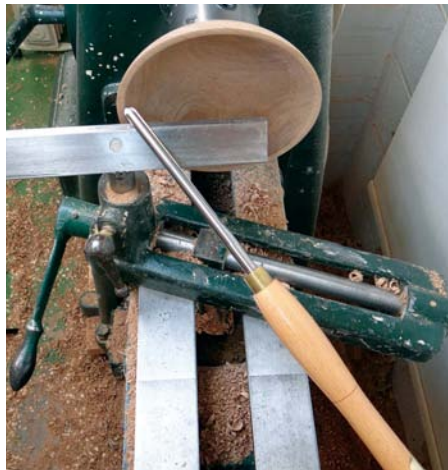
The start point turning the inside of a bowl
