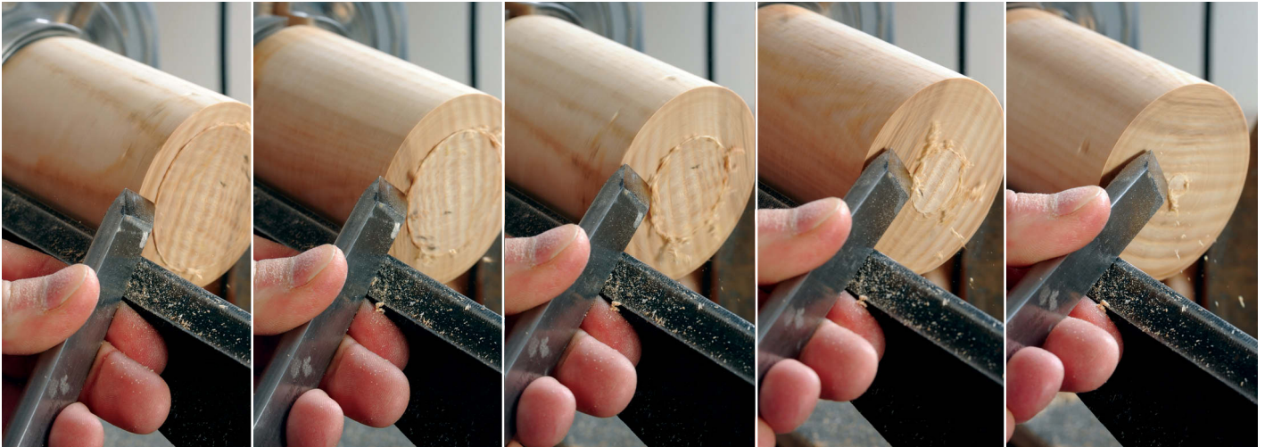
Gently raise the handle as you cut, so you gradually arc into the wood and finish dead on centre
