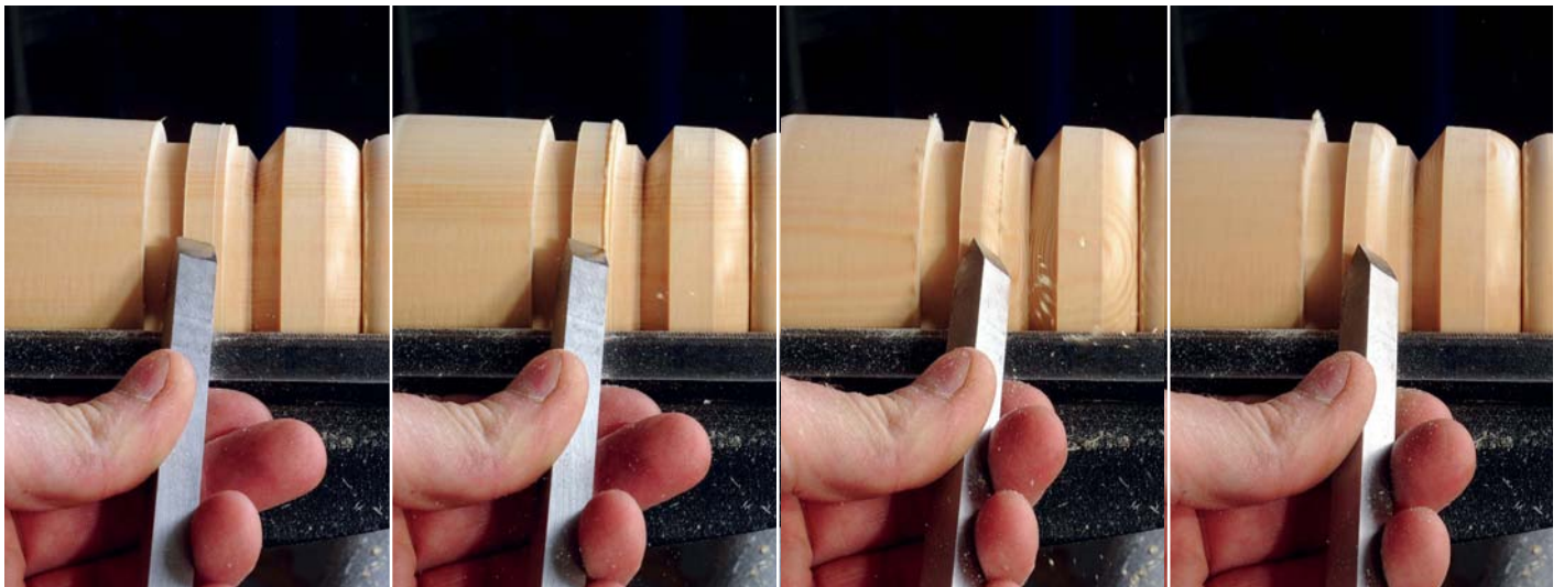
When viewed from a turner's side you can see how far the blade has to tilt to almost vertical to reach the lower section
