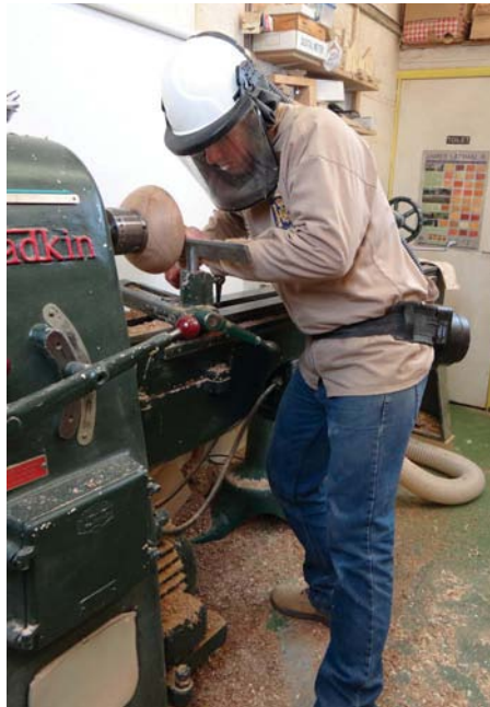
My start position when turning the inside of a bowl – note the wide stance and my weight over my right leg
