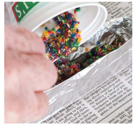
Mixing your filler to completely wet the surface will help create a good blank. Materials with a longer open time let any trapped air escape to the surface
