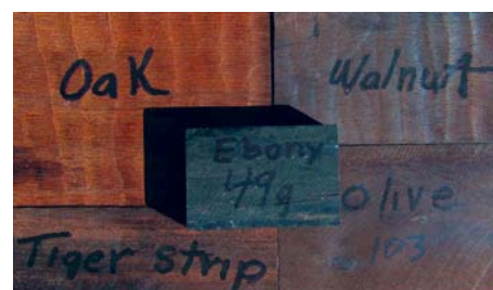
The oak and tiger stripe woods were put back in the oven and cooked at 232°C for 30 minutes more to yield a darker colour
