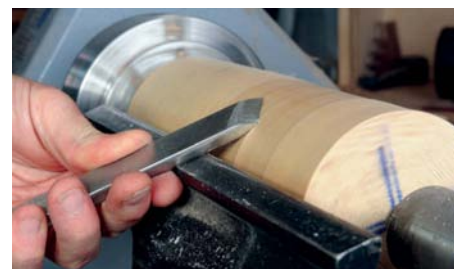
Raise the handle until the cutting edge is on contact
