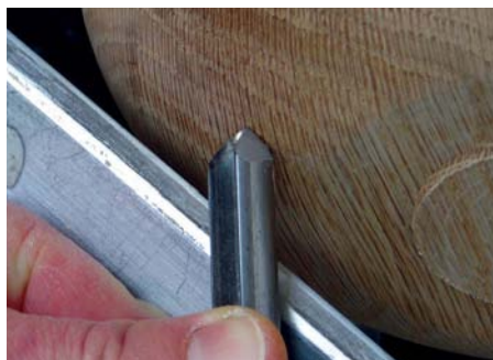
Close up of the bevel pointing in the direction of cut
