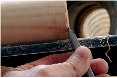
Cut with the tip only and enter in line with the bevel
