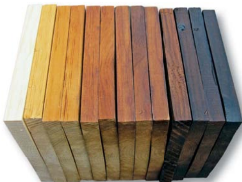
20mm-thick pine boards heated to temperatures up to 288°C
