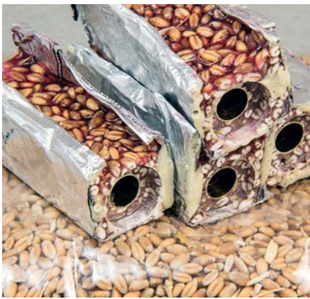
What you use to fill your resin with is your choice. If the resin will bond to it and it cuts decently, pick anything. This filler is winter wheat seed
