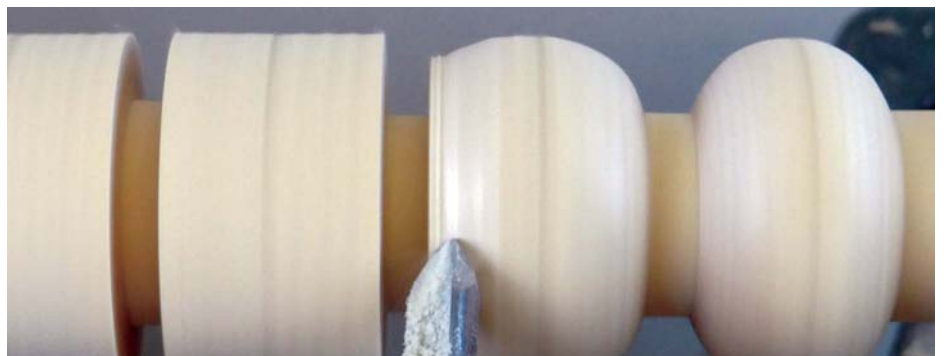
Having a full view of both the shape being turned and the tool gives the best chance of success
