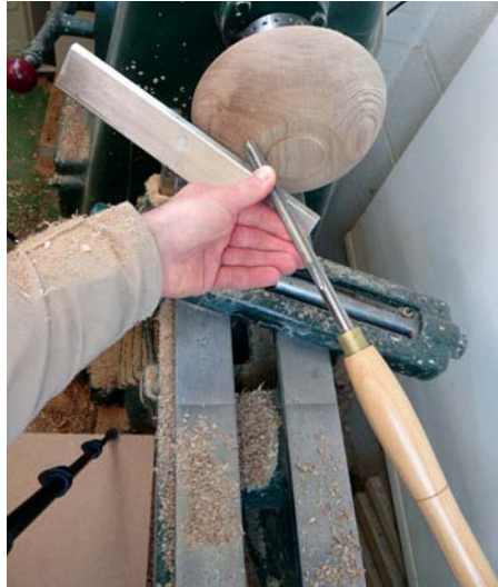
The starting point, turning the base of a bowl. Here you can notice the handle is out to the right side and over the lathe bed
