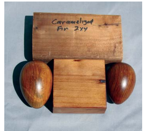
50mm-thick woods after heat treatment
