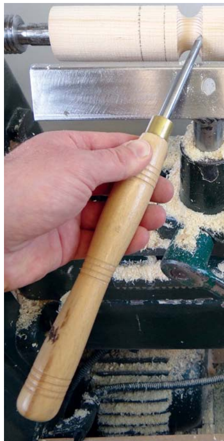
The start position when turning a cove
