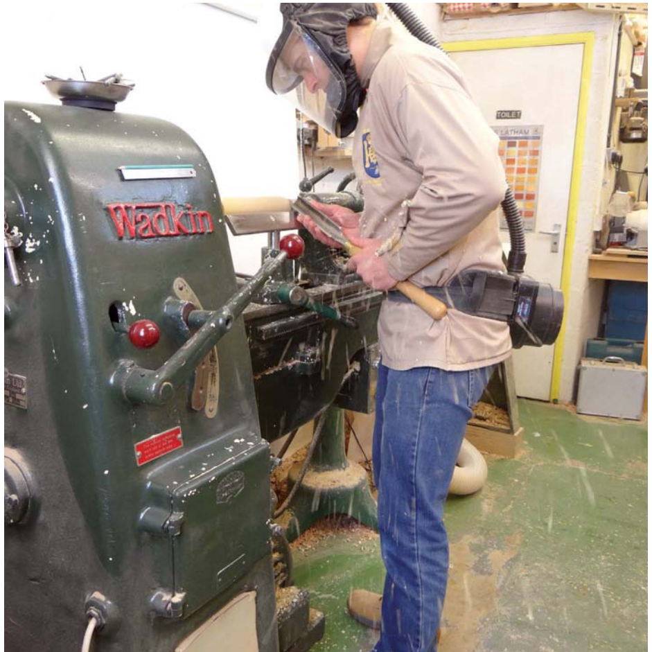
My stance when spindle turning – note the tool handle is by my side
