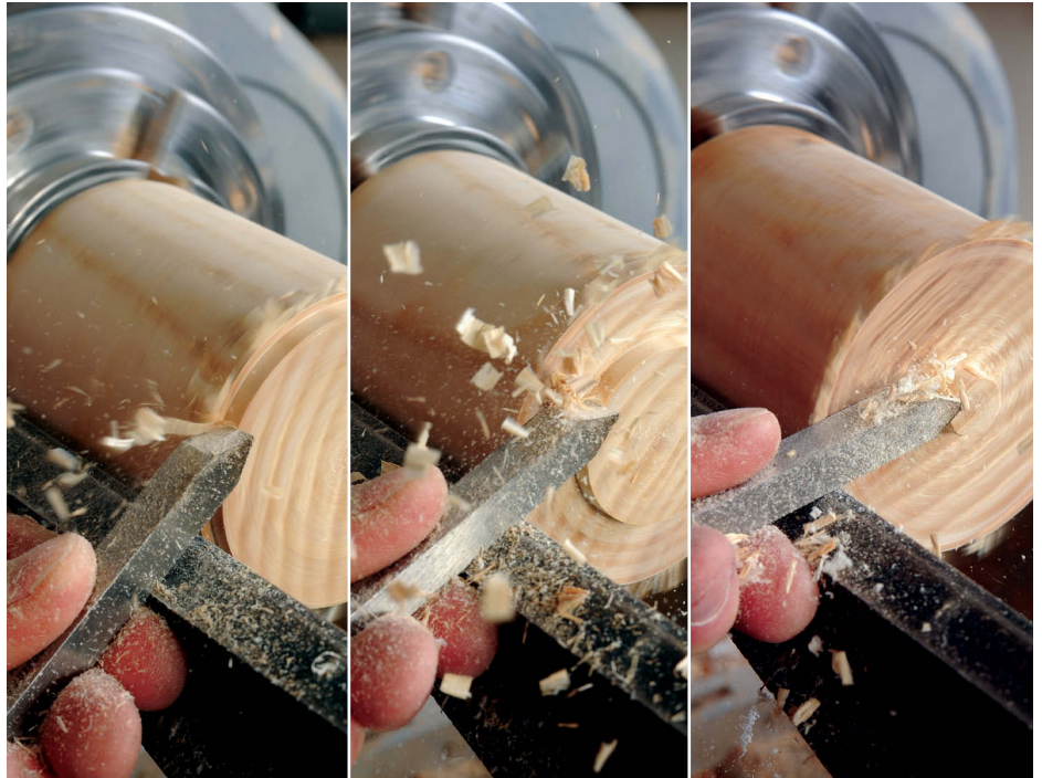
This sequence shows the tool being arced into the wood, so the bevel is rubbing all the way through for the cleanest cut possible
