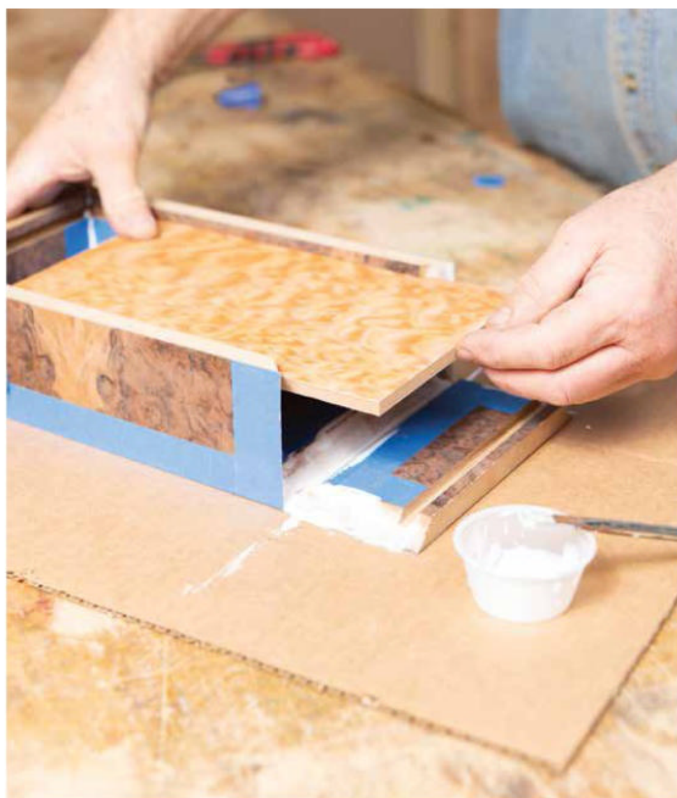
Dado for bottom panel. After cutting the dado, the veneered bottom panel should fit snugly in its slot.
