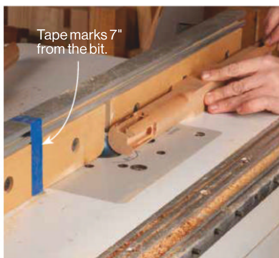
Rout round. Set a \frac{3}{4} " roundover bit into a router fence and round the ends of the leg stock into 7" long, 1\frac{1}{2} " dowels, leaving a square section in the middle for safety.
