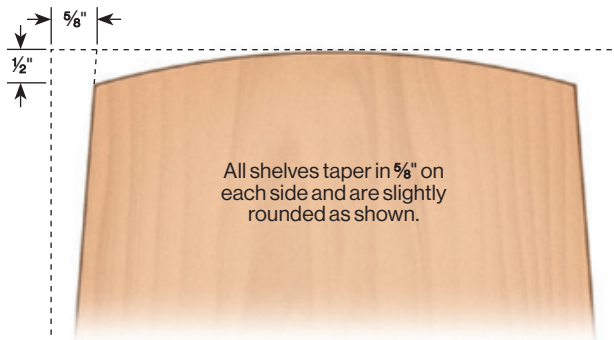
Lay out the final shape. Lay out the tapers on each shelf. At their widest, they should be \frac{1}{8} " inside the taper lines on the trunk. Then draw the end curves with help from a flexible drawing spline. I used the same curve for all eight shelves.
