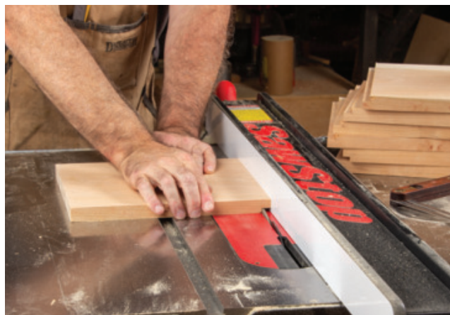
Fix the shoulder. Switch to a regular blade and tilt it to match the trunk taper angle. Recut the shelves' shoulders at this slight angle, positioning the cut with the fence. On my left-tilt saw, I had to put the fence to the left of the blade.
