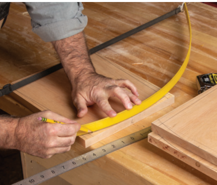
Lay out the final shape. Lay out the tapers on each shelf. At their widest, they should be \frac{1}{8} " inside the taper lines on the trunk. Then draw the end curves with help from a flexible drawing spline. I used the same curve for all eight shelves.
