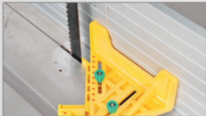
Set fences for resawing and transfer measurements.
