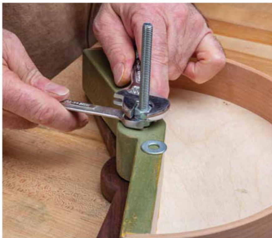
Two wrenches to tighten. Add lock nuts and washers to space the drawers apart. Tighten the nuts against each other and try the drawer. Reposition the nuts and/or add more washers to adjust the space under the drawer as needed.
