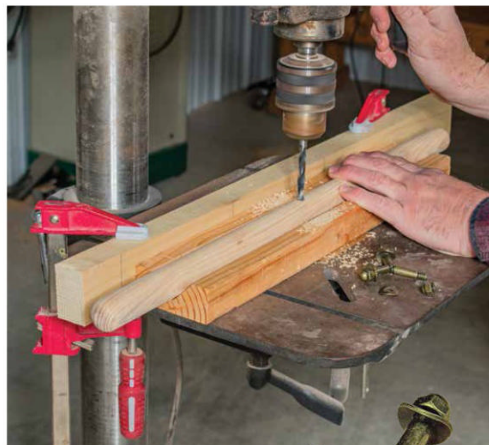
Drill for the bolt. Cradle the legs in a V-block clamped to your drill press table. Drill a \frac{5}{16} " diameter hole at the midpoint of each leg. ■
