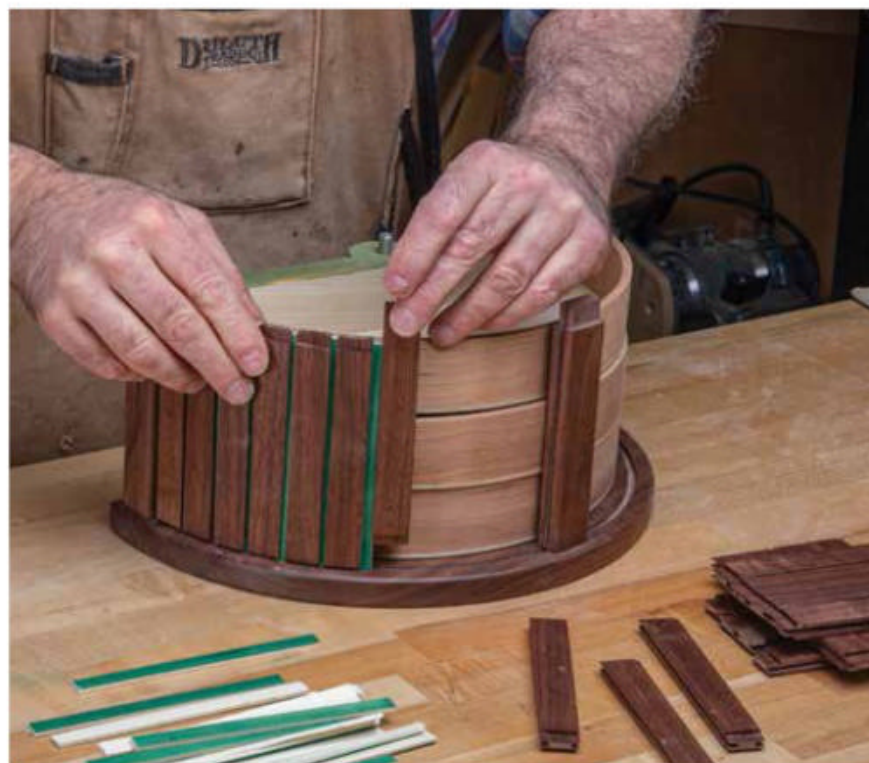
Assembly. Once the drawers are spaced correctly, fit the columns, staves and splines, trimming the width of the splines if necessary to keep the spacing consistent. Dry fit all, then glue up. ■
