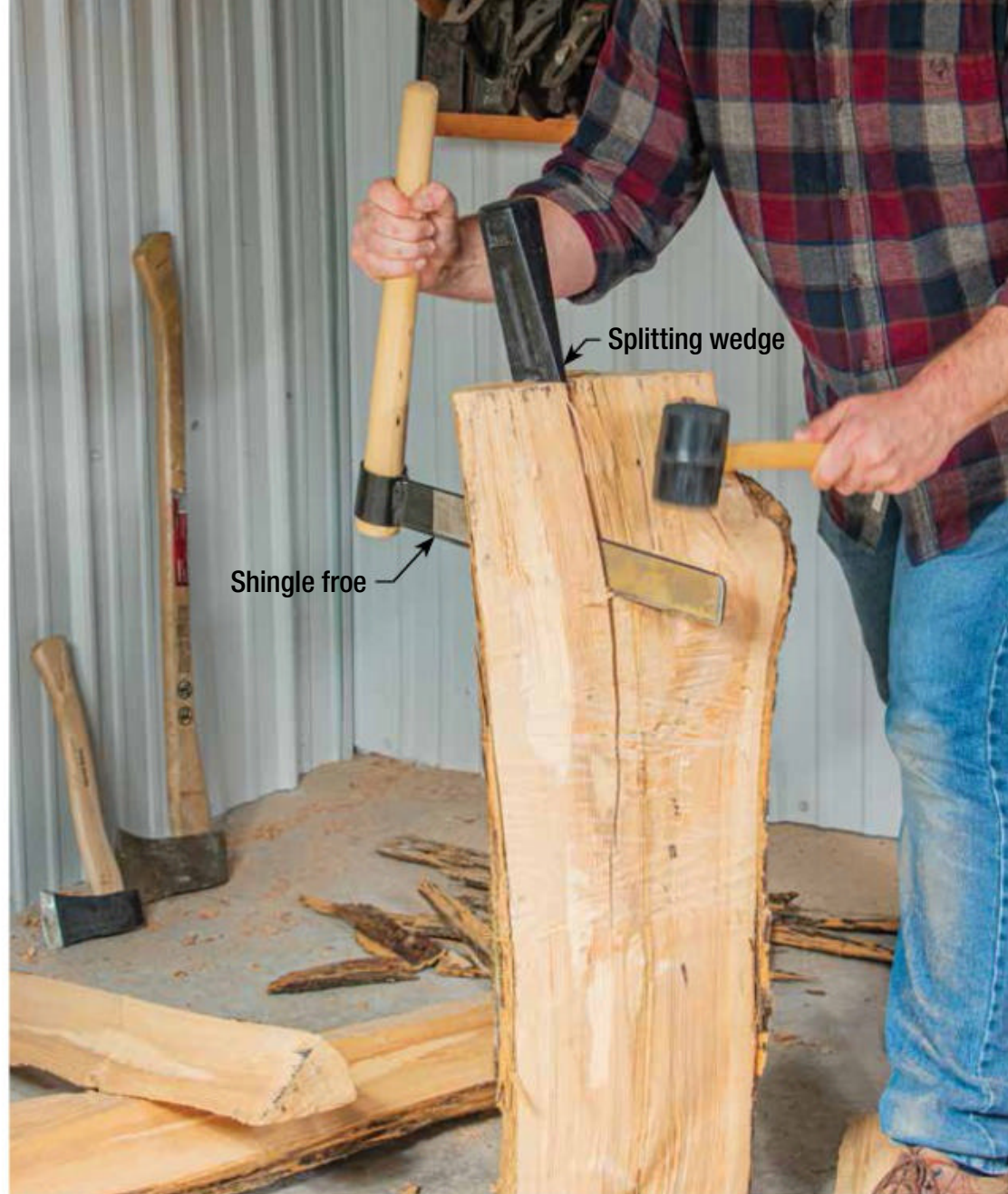
Split the log. Split the log in half using a froe and mallet. Use a splitting wedge to capture your progress as you drive the froe. Then split one half into three triangular billets, each of which will become a stool leg.
