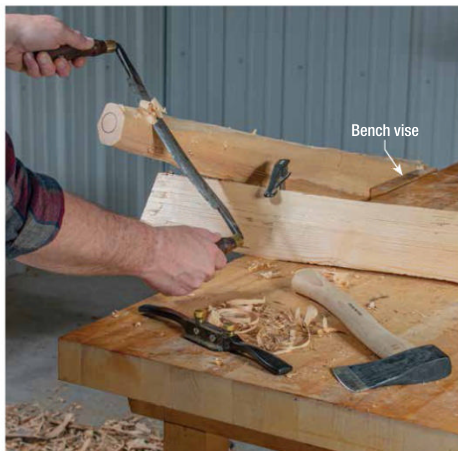
Round the legs. After trimming away the corners, securely clamp the rough leg blank to your bench and mark the ends with the final leg shape. Round it with a draw knife and spokeshave. If desired, smooth away any facets with a concave cabinet scraper.
