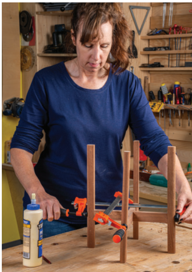
Pull it together. Get your glue-up supplies ready first, then draw the joints together with clamps. Wipe away any glue squeezeout.
