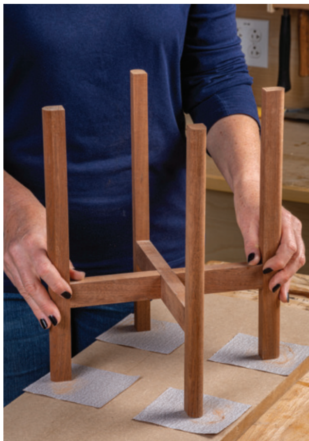
Level the legs. If you find your stand rocks slightly, level the legs by taping squares of sandpaper to a piece of MDF and scrubbing the stand back and forth across them. ■
