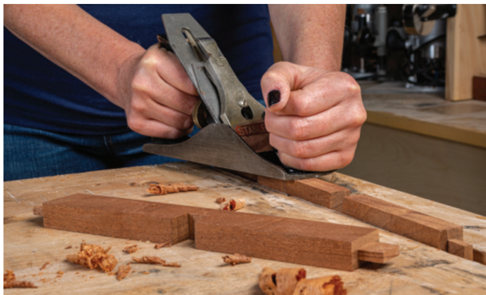
Plane to perfection. Making the rails dead flush to each other may require a swipe or two from a hand plane.
