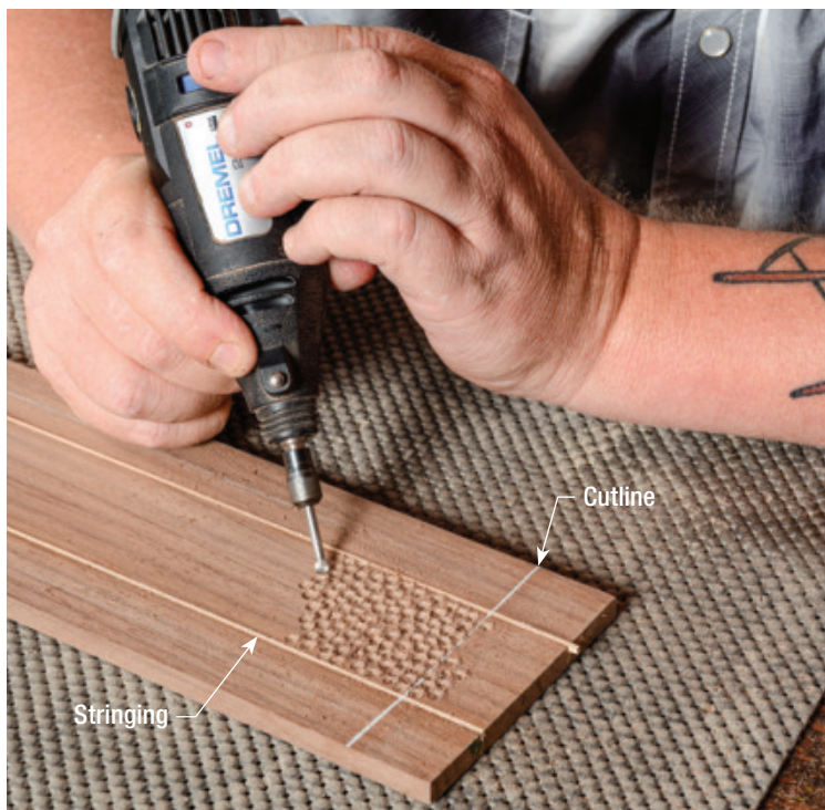
The dimple dip. Steadying the rotary tool with both hands, dip the cutter quickly into the wood surface, lifting it straight up afterward. Have fun practicing on scrap, creating a random pattern with dimples of slightly different depths. Stay close to your inlay lines without straying into them. Maintain the same angle of attack throughout so light reflects evenly on the surface.
