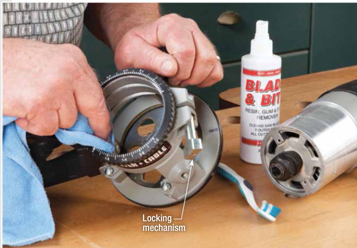
Metal hygiene. Clean the spiral height-adjustment grooves using a toothbrush and rag dampened with pitch remover.
