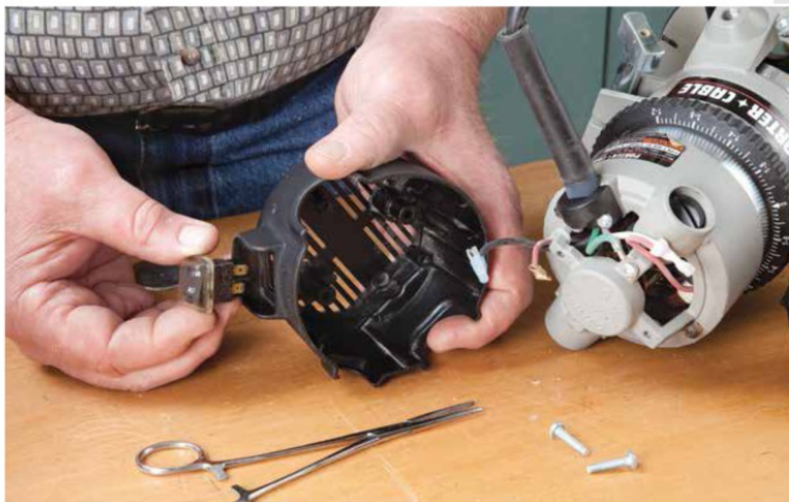
Switching out a switch. To install a new switch, orient it properly and reattach the wires in their original configuration.
