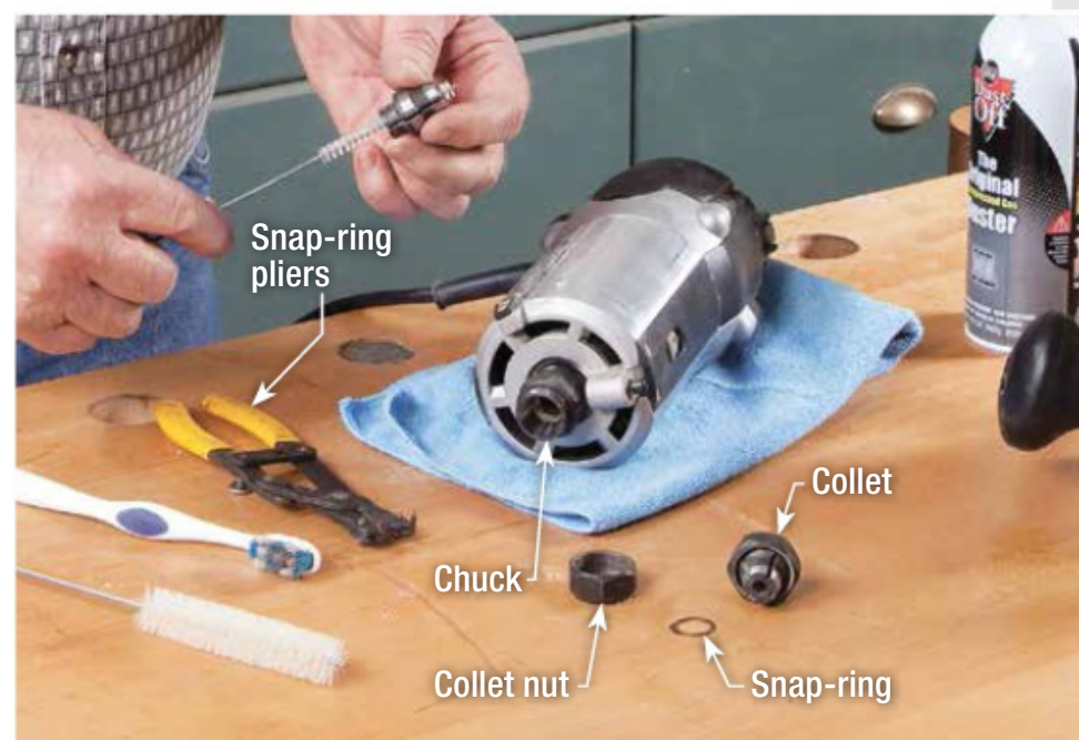
Cultivate crud-free collets. Clean the collet and nut to remove dirt and debris and keep them trouble-free.
