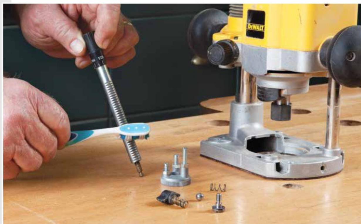
Plunge bath. Disassemble a depth-stop rod and turret to properly clean and lubricate them, ensuring smooth plunging operation.
