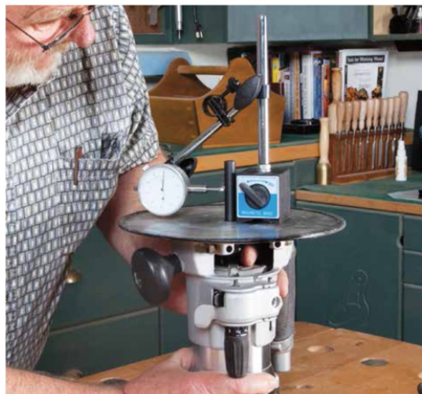
Turning true? Use this setup of a dial indicator, saw blade, and drill rod to check collet runout.
