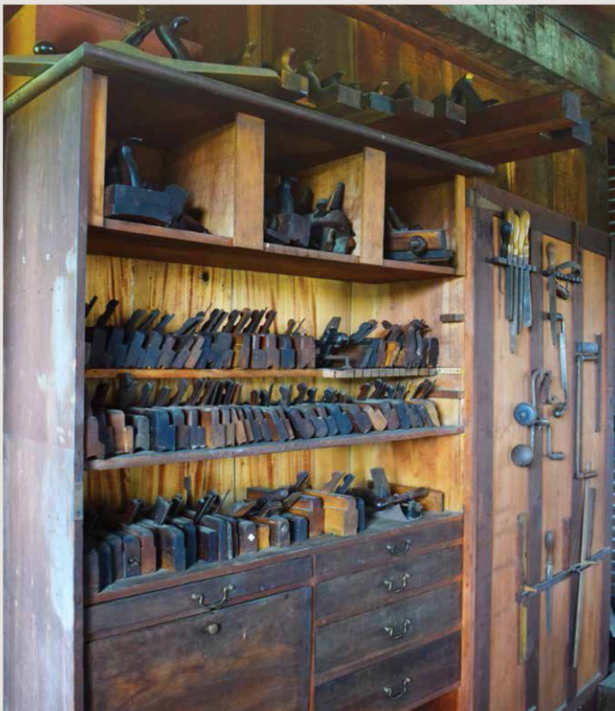
The plane life. Like other 19th century woodshops, the one at Hancock Shaker Village has a large complement of handplanes—small ones on the shelves for decorative moldings and rabbets, larger ones atop the cabinet for flattening and smoothing boards.
