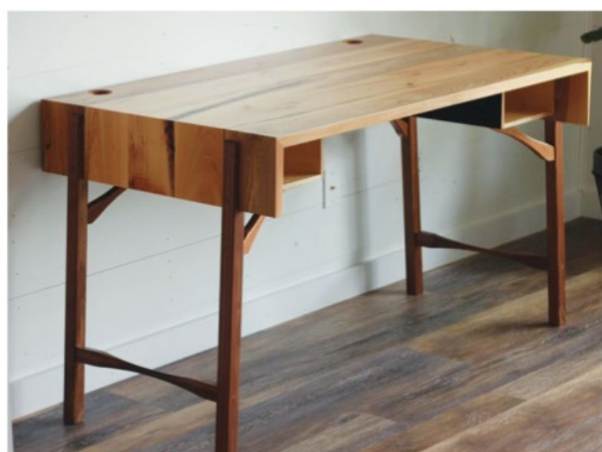
JAY DORROUGH, SEGUIN, TX Crisply made corners. Waterfall edges distinguish this desk, which has a pecan top supported by black walnut legs, stretchers, and braces. Dorrough used loose tenons to assemble the mitered edges.
