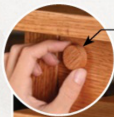
Magnet (embedded in dowel) held over catch area opens left-hand apron compartment.
