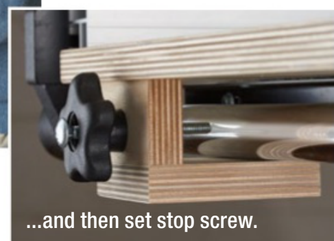
Stop initial cut at slot centerline...
