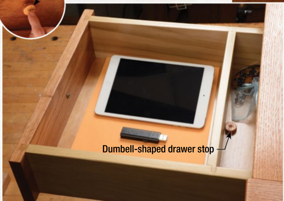
Raising dumbbell stop from underneath allows full retraction of drawer to expose hidden section at rear.
