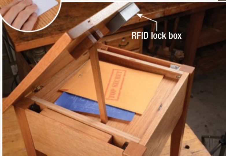
Magnet (embedded in dowel) held over catch area opens left-hand apron compartment.
