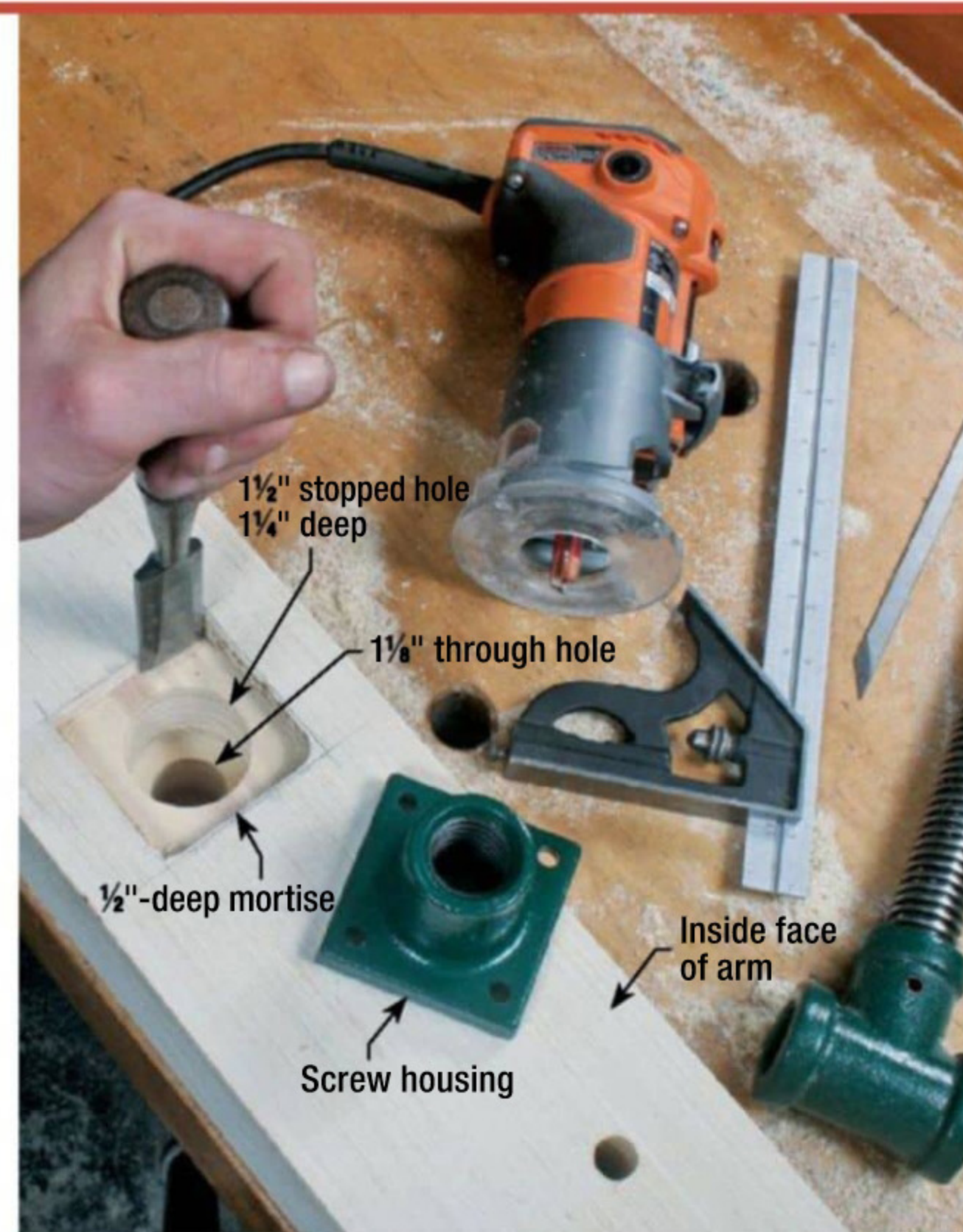
Install the vise screw housing. After drilling a stopped hole for the shoulder vise screw housing and a through hole for the screw, rout a mortise and then square the corners with a chisel.
