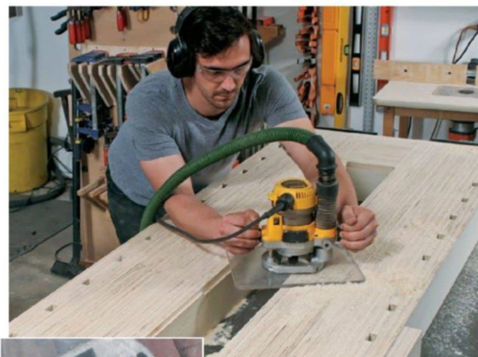
Cut a center ledge. Rout a \frac{1}{4} \times 1 "-deep rabbet around the perimeter of the interior for the centerboard using a bearing guided rabbeting bit, taking two or three successively deeper passes. An oversized baseplate steadies the cut.
