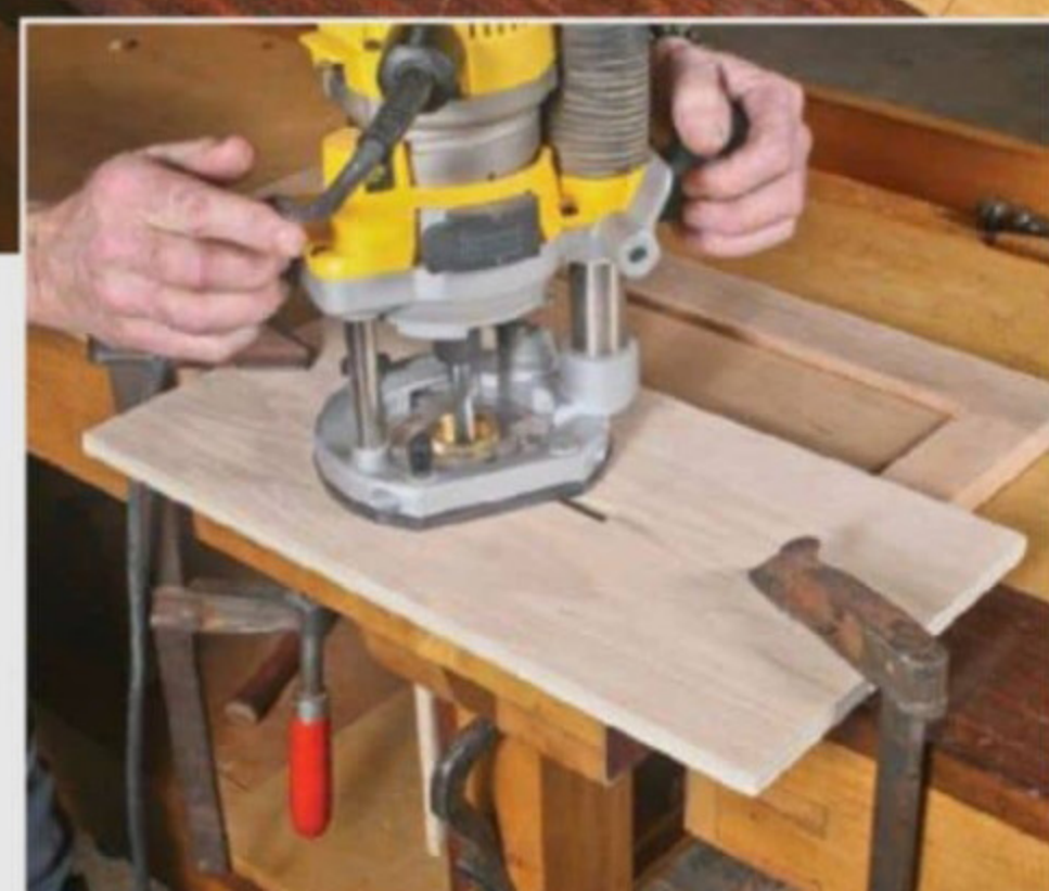
Rout the bar recess. Align the bar recess jig with the layout lines on the stile, reset the bit, and rout the \frac{3}{32} "-deep recess for the brass bar. Chisel the ends square afterward.
