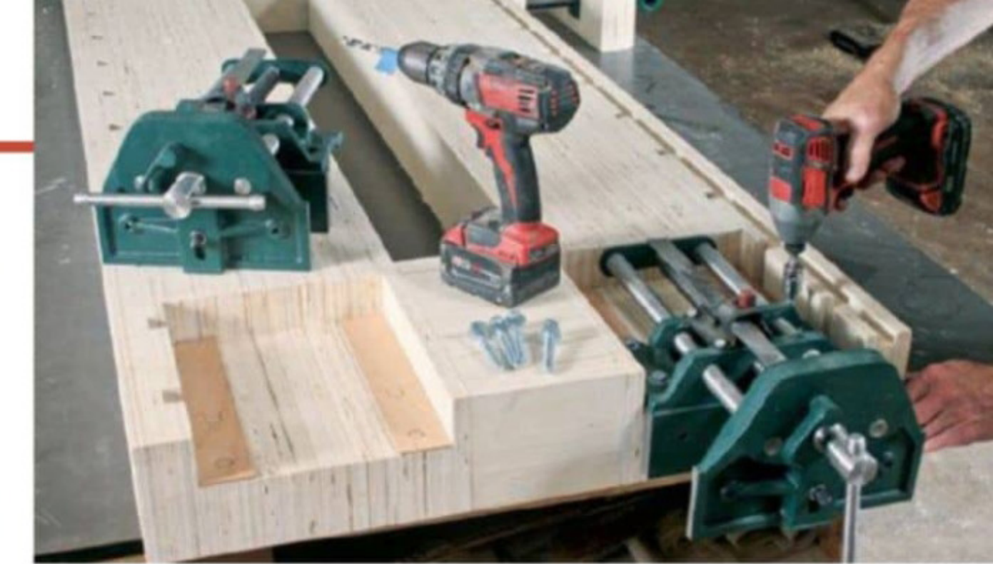
Set the vise height. Install a couple shims under each inverted end vise to locate the fixed jaw about \frac{9}{16} " from the top surface of the bench. Then secure each vise with four lag screws.
