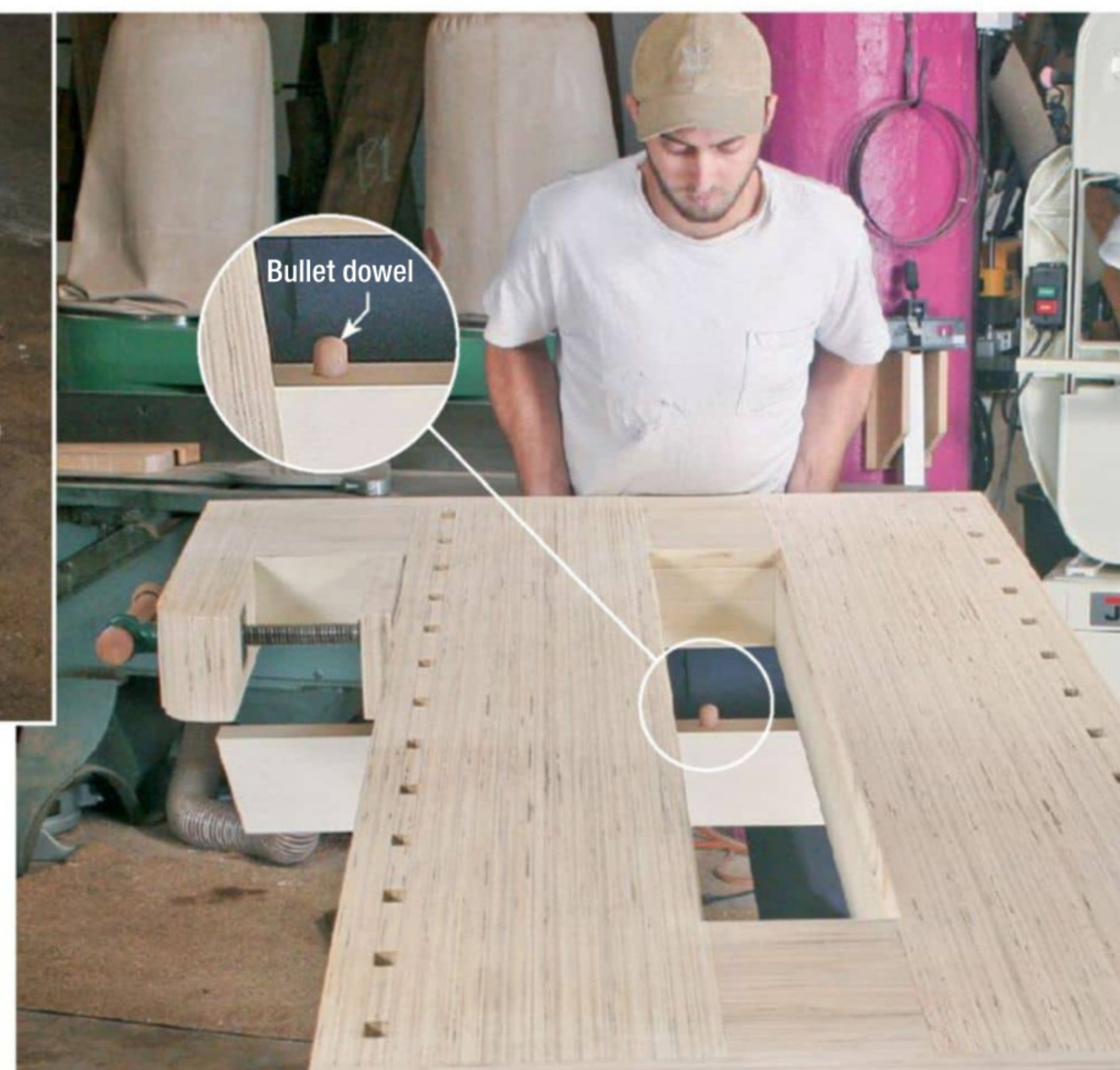
Aiming for a bullet. Make a drilling guide by boring a 1"-dia. hole in a board with a Forstner bit on the drill press. Clamp the guide flush with the front of the end assembly and use the guide and the same bit to drill a 1\frac{1}{4} "-deep hole for the bullet dowel. Use the guide again to drill the hole in the other end assembly, and two matching holes in the top's underside. Insert the dowels in the base, and then then lower the top in place. ■
