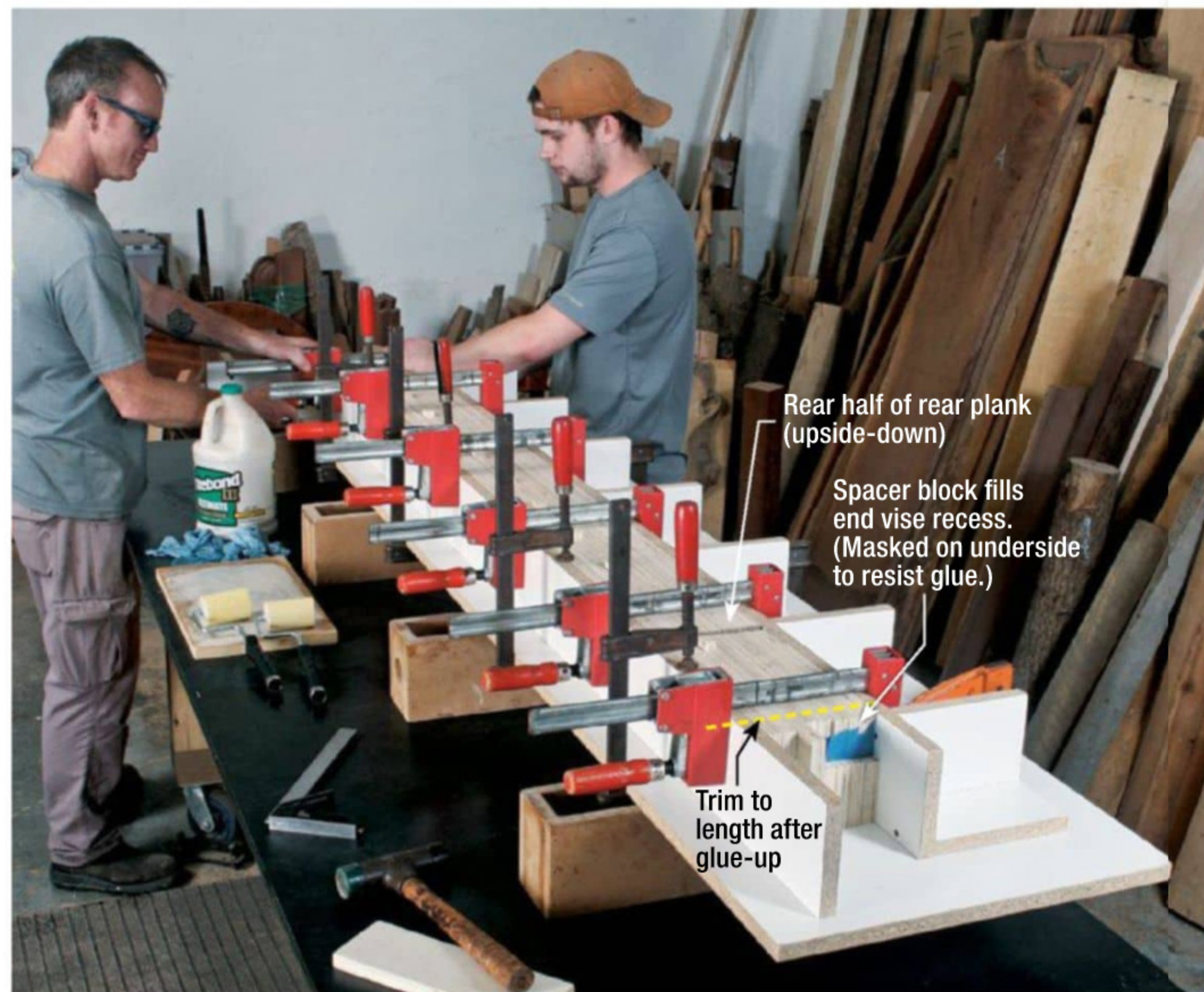
Glue up the planks in stages. Stack a half-plank's worth of strips upside down in the assembly jig, with glue-resistant plywood spacers filling any cavities. After rehearsing your assembly procedures, apply adhesive with a thin-nap paint roller to the strips, and clamp them to the jig. Wipe or scrape off the wet excess glue immediately.
