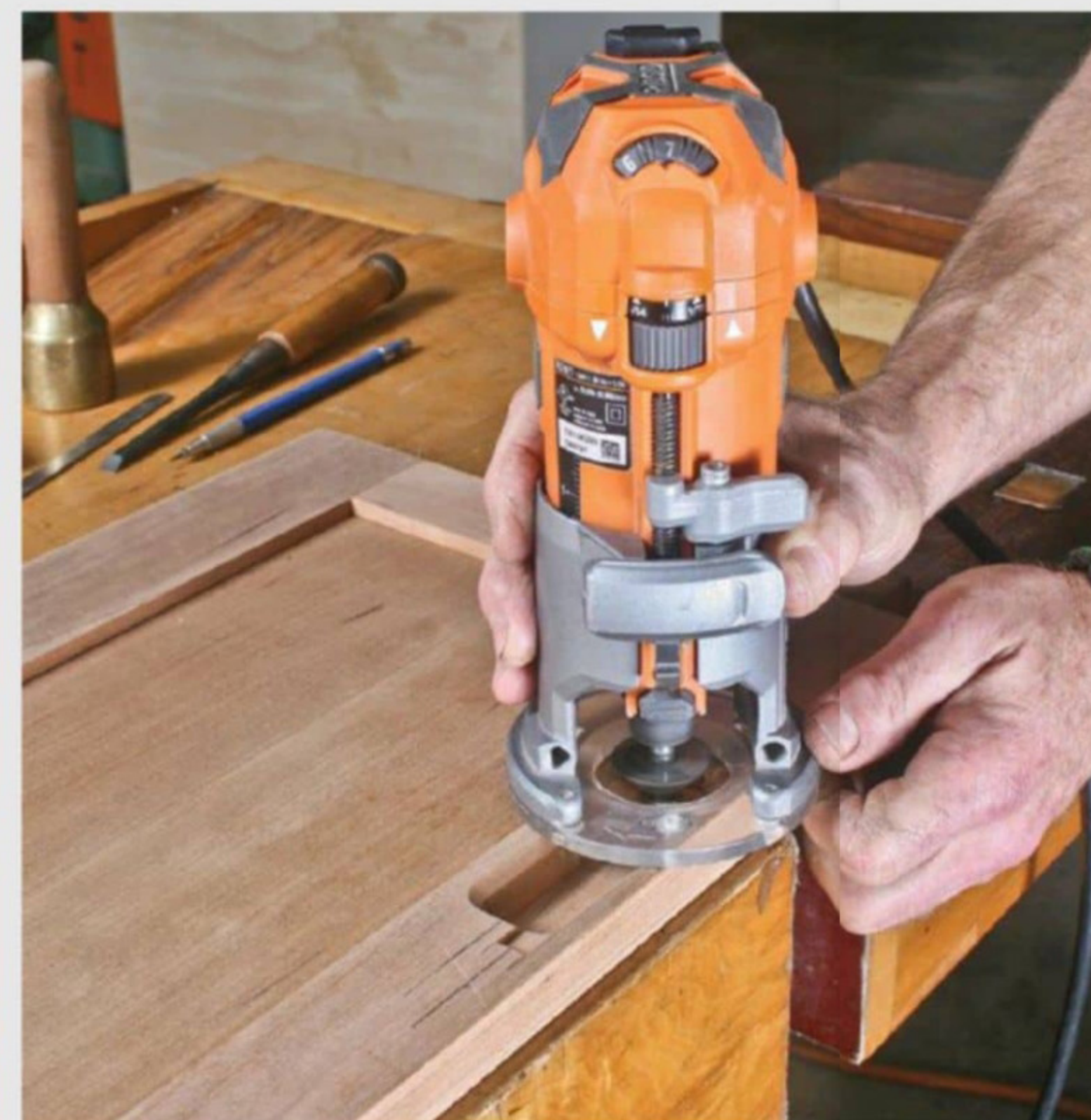
Stop that chamfer. Set a bearing-guided chamfer bit for a \frac{3}{16} "-wide cut, and then rout a bevel around the three walls of the pocket, being careful to stop at each edge of the bar recess to avoid beveling this area.
