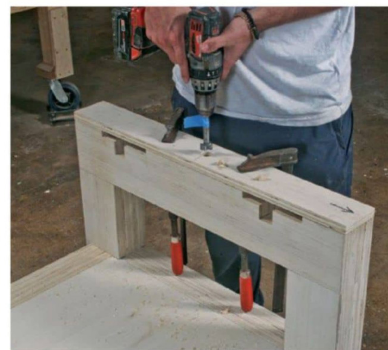
Aiming for a bullet. Make a drilling guide by boring a 1"-dia. hole in a board with a Forstner bit on the drill press. Clamp the guide flush with the front of the end assembly and use the guide and the same bit to drill a 1\frac{1}{4} "-deep hole for the bullet dowel. Use the guide again to drill the hole in the other end assembly, and two matching holes in the top's underside. Insert the dowels in the base, and then then lower the top in place. ■
