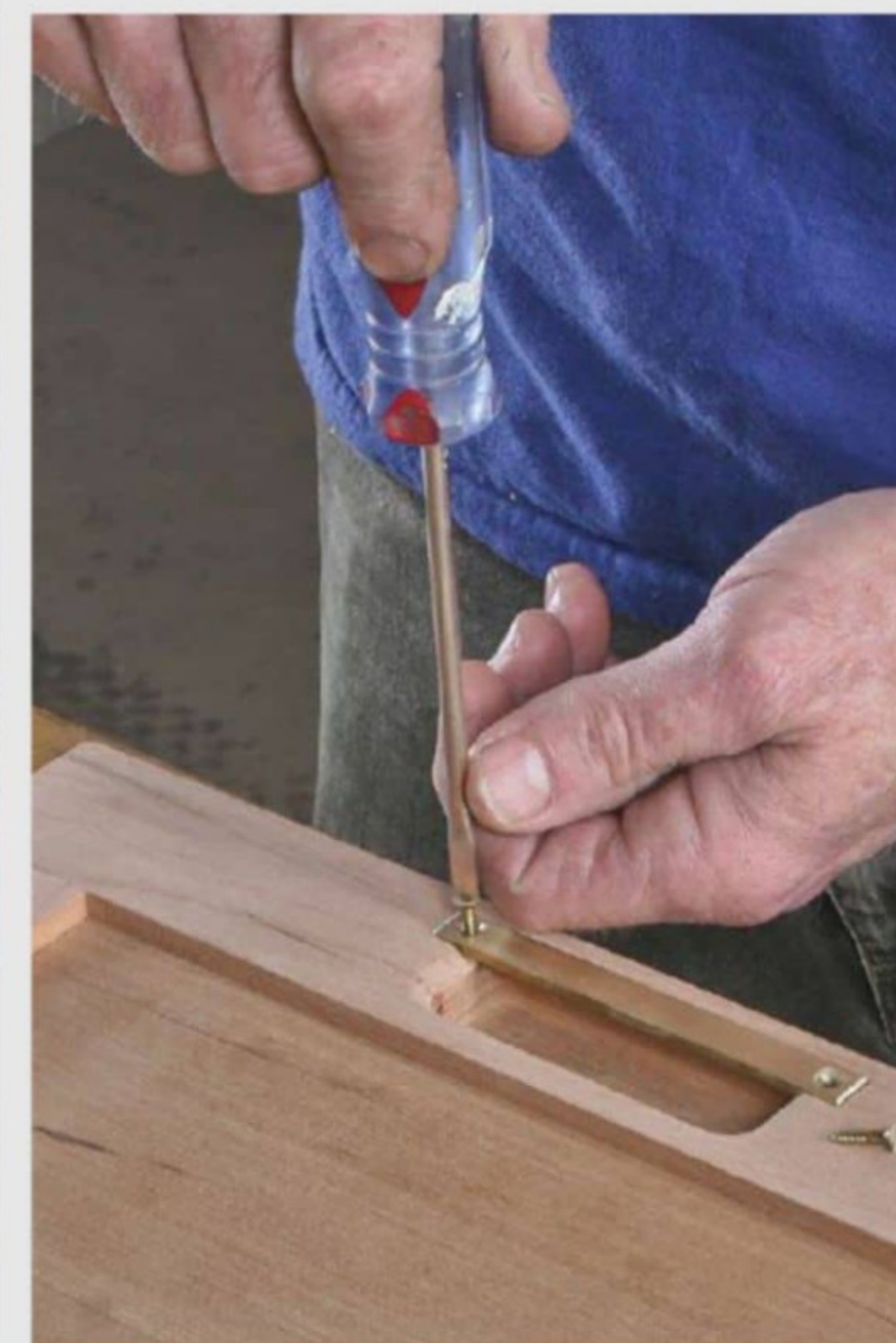
Slightly proud. Lightly ease the upper edges of the brass bar using 400- and then 600-grit carborundum paper before screwing the bar into its recess. It should project about \frac{1}{32} " above the surface of the door.
