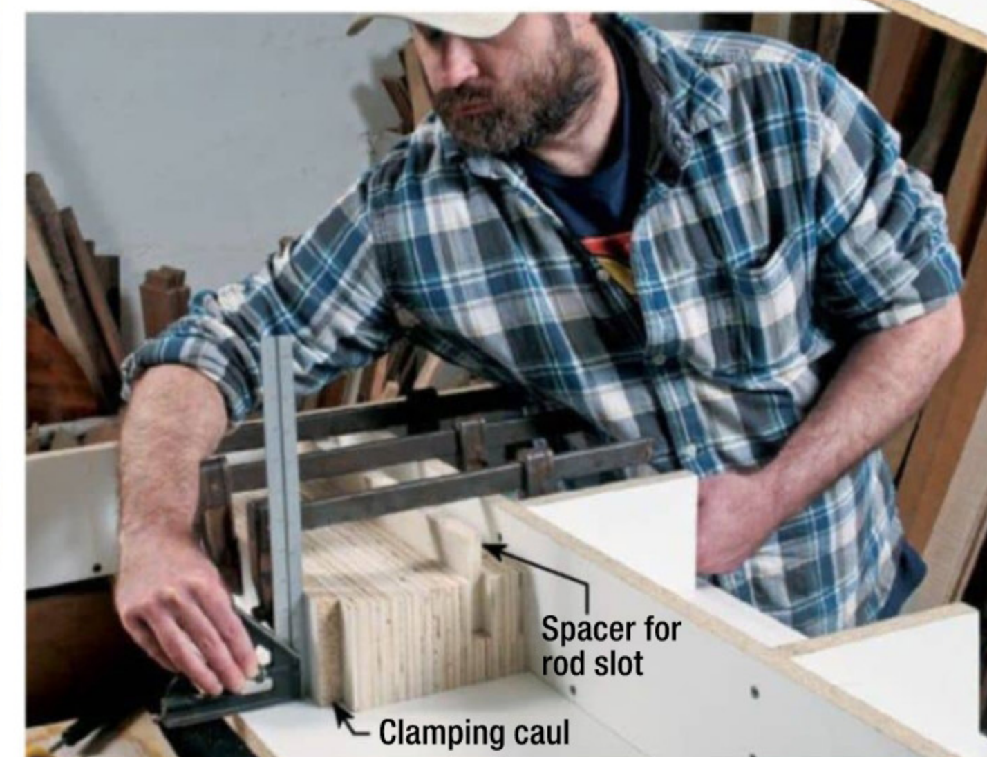
Assemble the shoulder in stages. Glue together the wide and narrow strips (shown) separately, and then join the two halves. Set a waxed plywood spacer in the rod slot to equalize clamping pressure.
