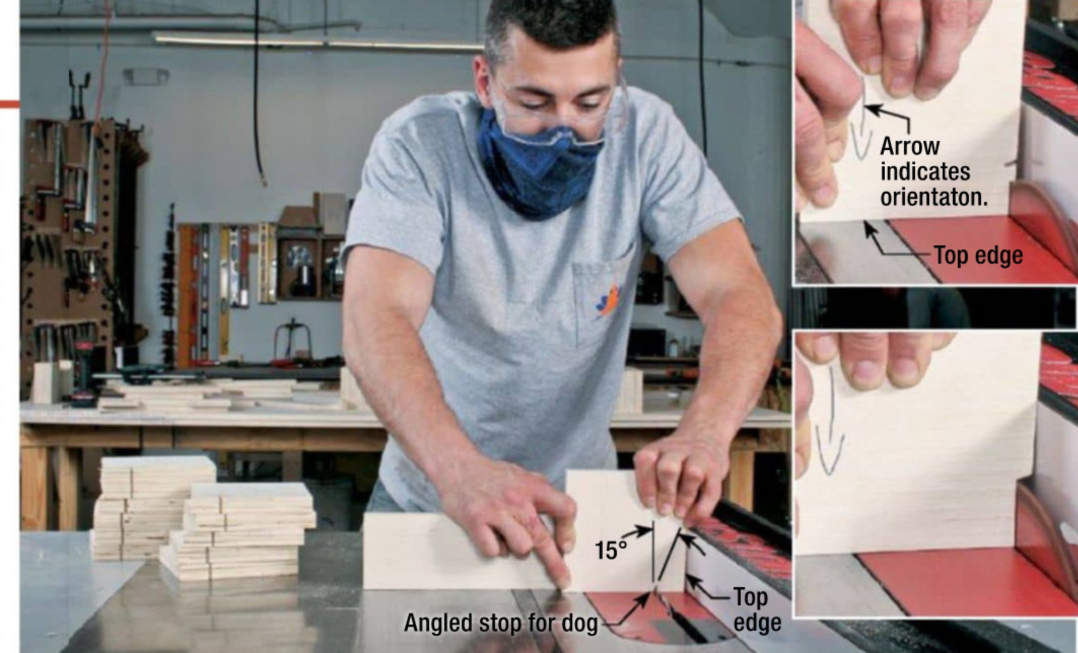
Make 26 dog blocks. Set the blade to 15^\circ , stand the dog block with its inner edge against the fence and cut the angle for the notch. Then, flip and rotate the block 90^\circ and make the long notch cut by first removing a saw kerf of material (inset, top) and then butting the block against the fence to complete the cut (inset, bottom).
